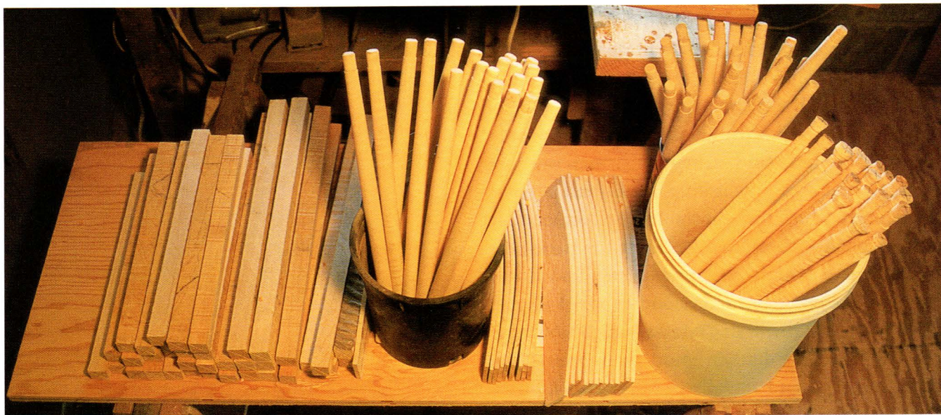
Turning blanks are stacked on the right. Turned, tenoned, and sanded rungs are stored in buckets until they're needed at assembly. Steam-bent slats are curled around the black bucket, while band-sawn and sanded (but unbent) slats are leaning against the white bucket.
