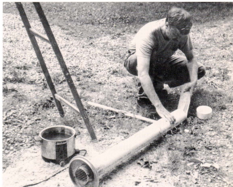
In this photo, I'm loading a set of chair slats into my steamer. Notice that the length of PVC passes through the deep-fat frier's metal lid. Notice, too, the hardware cloth that laps the bottom of the PVC.
