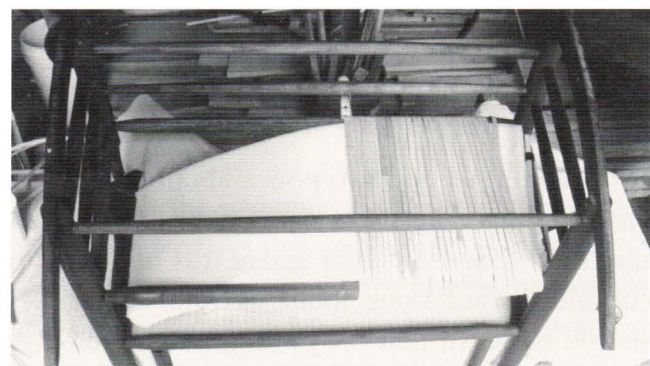
When the warp has filled approximately half the area to be seated, a 1" foam cushion cut to the contour of the seat is slipped between the warp layers. This cushion helps the woven splint maintain its shape. Additional warp is then wrapped around this cushion.
