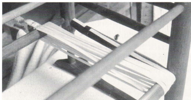
The beginning of the first strand is taped to the side seat rung. A spring clamp is used to hold the warp in place while a new warp strand is attached to the end of the first warp strand with three staples located along an eight-inch lap.
