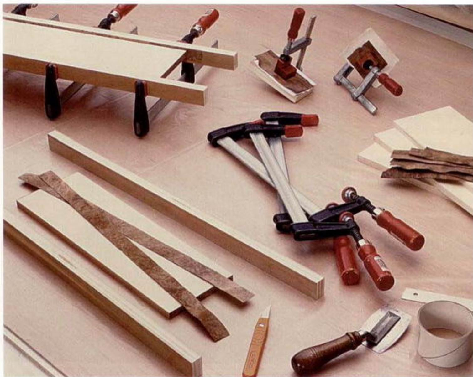
Photo B: Pressing veneer on the small corner blocks and drawer front edges can be done easily with cauls and clamps. Apply veneer larger than the substrate surface, and trim to fit later.
