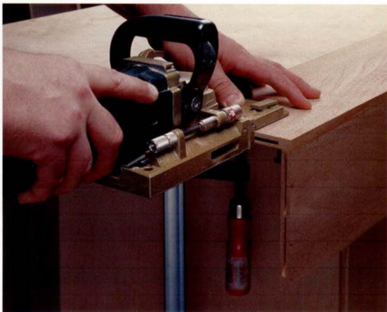
Photo E: Cut four biscuits in the end of each V-shelf, registering the joiner off the shelf backs. Leave the layout lines.
