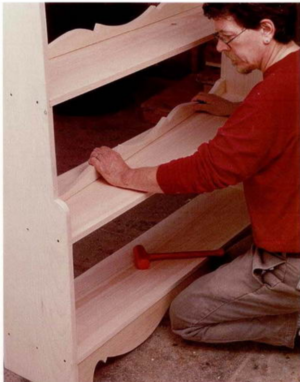
Photo G: Position and glue the decorative members flush with the back edge of the shelf and nail in from the sides.
