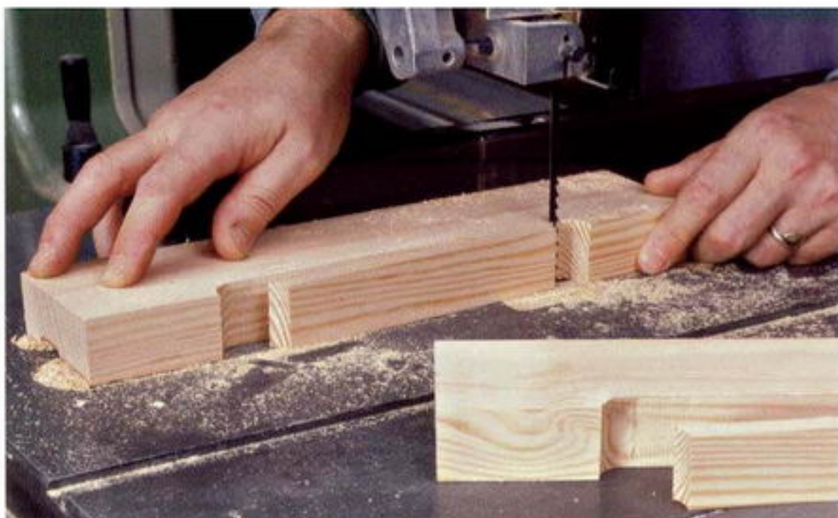
Photo I: Bandsaw the waste between the half-rounds to create the base detail.
