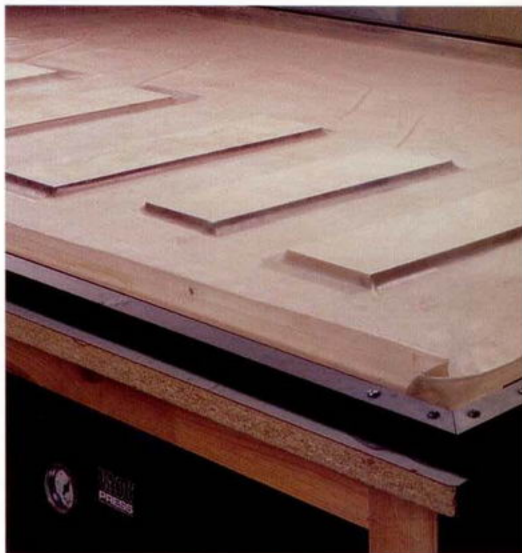
Photos D and E: Vacuum presses make applying veneer to the drawer fronts and side panels a cinch. Just position the pieces on the veneer in the press (left). Lower the membrane top and start the vacuum pump. The bag exerts perfectly even pressure over the parts (right).
