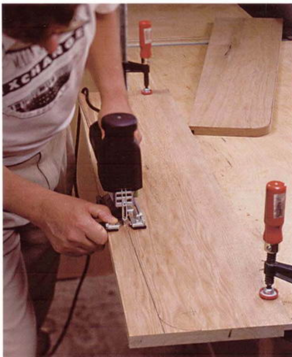
Photo F: A jigsaw is the quickest and simplest way to cut the taper and the radius in one operation.
