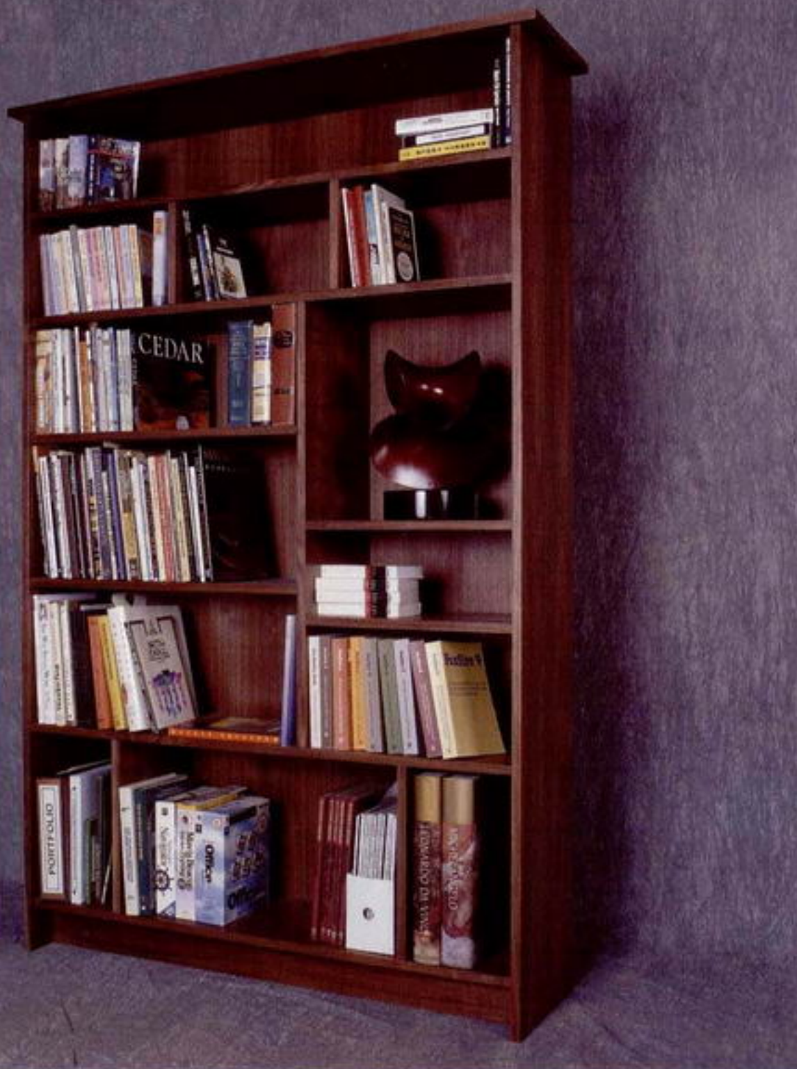
Fixed intermediate supports spread the load across these 48-in.-long shelves and keep them from sagging. (Photo by Joe Romero.)
