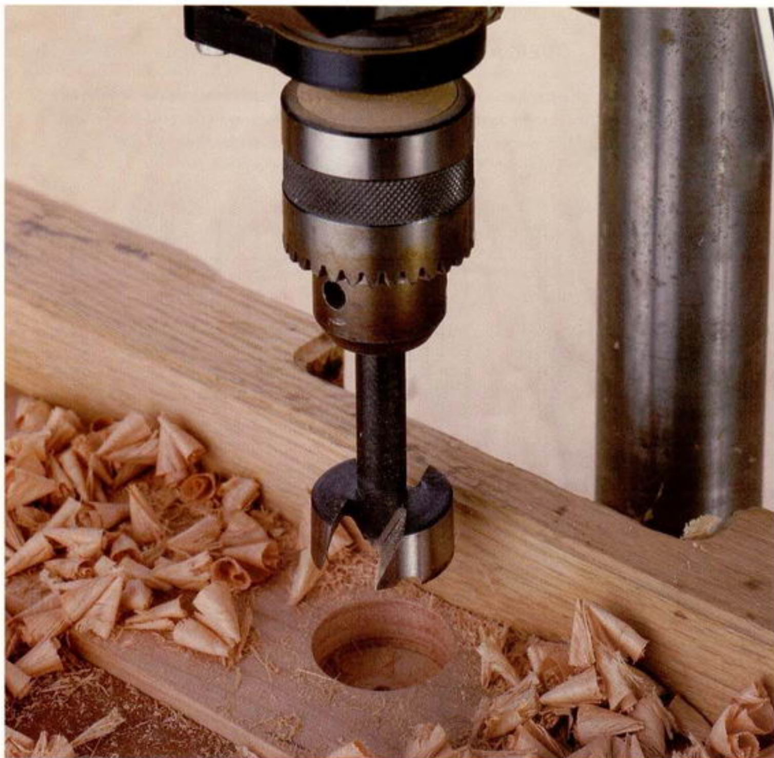
Photo I: Drill the hinge cup hole in the door stile on a drill press to ensure that the hole is not skewed.
