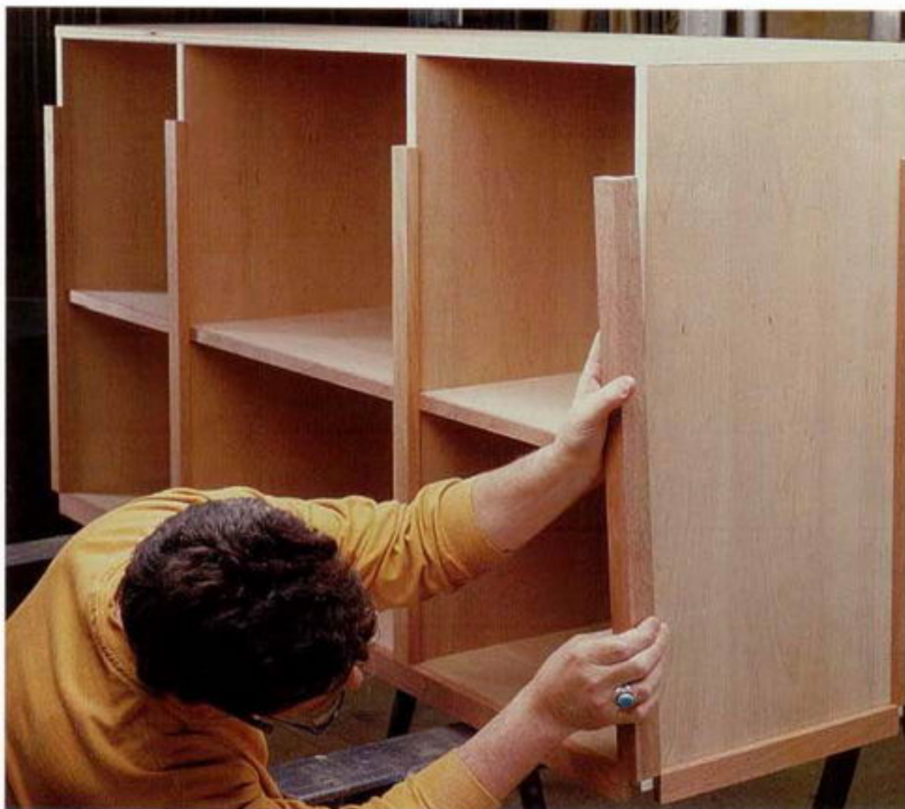
Photo A: Attach the corner piece of the face frame \frac{3}{4} in. shy of the bottom. This leaves a space for the corner block.
