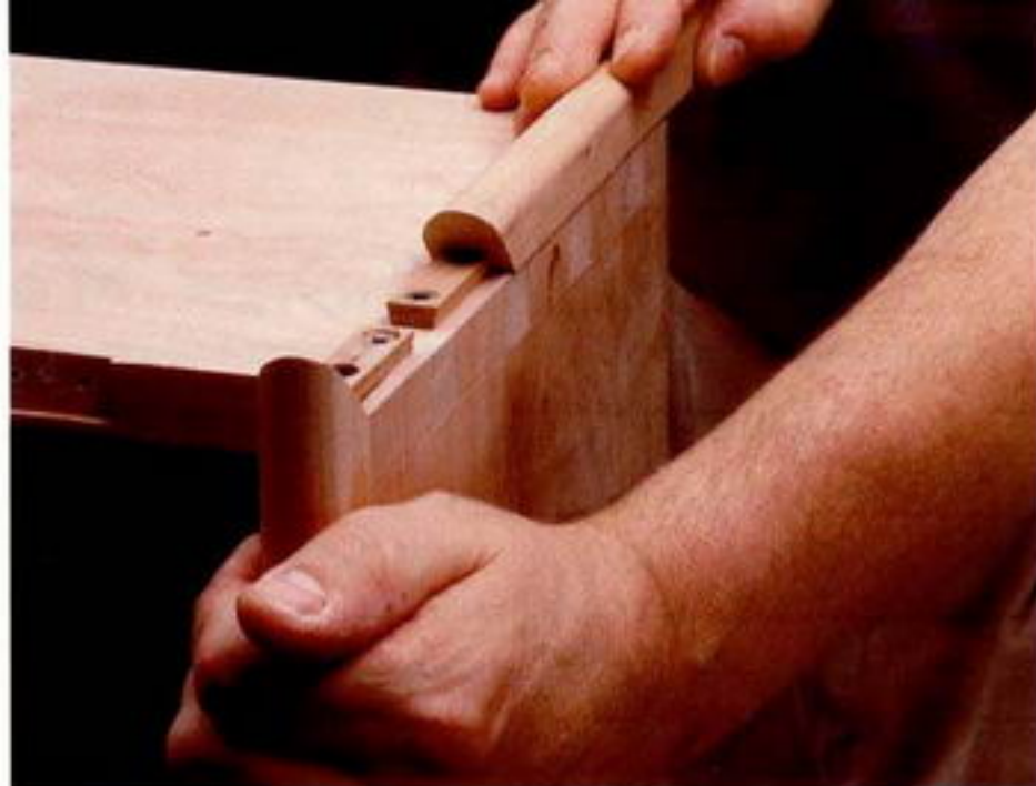
Photo O: The thumbnail molding shouldn't slide on too easily but shouldn't need to be hammered into place.
