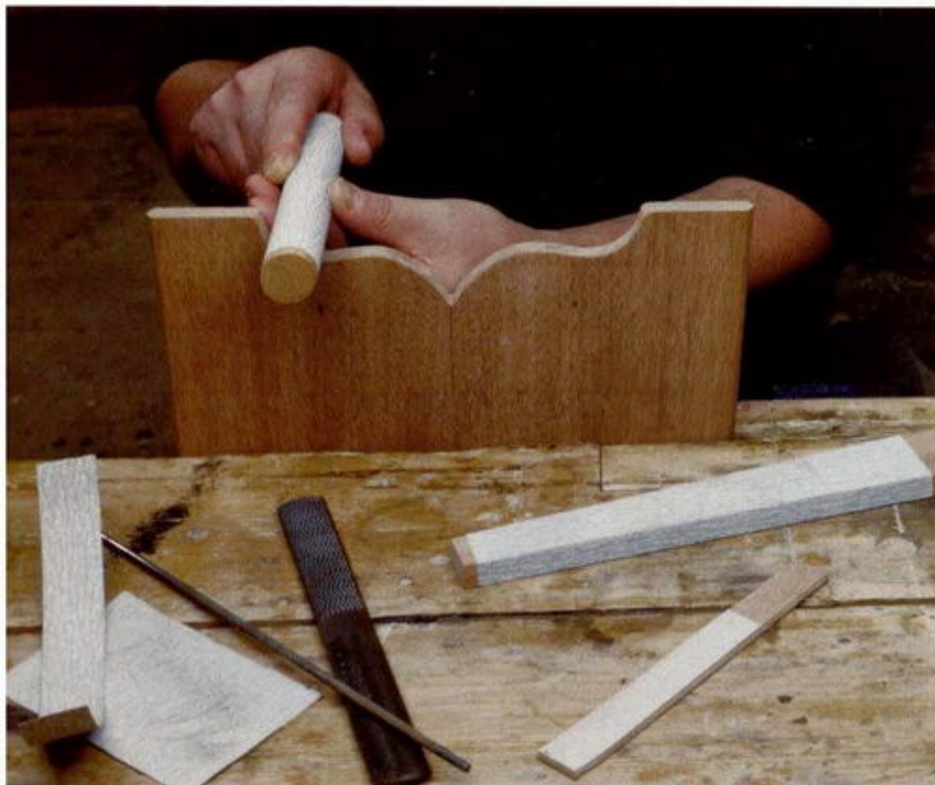
Photo C: Smoothing the whale-tale detail can be accomplished with files, rasps, and an assortment of sandpaper and blocks.
