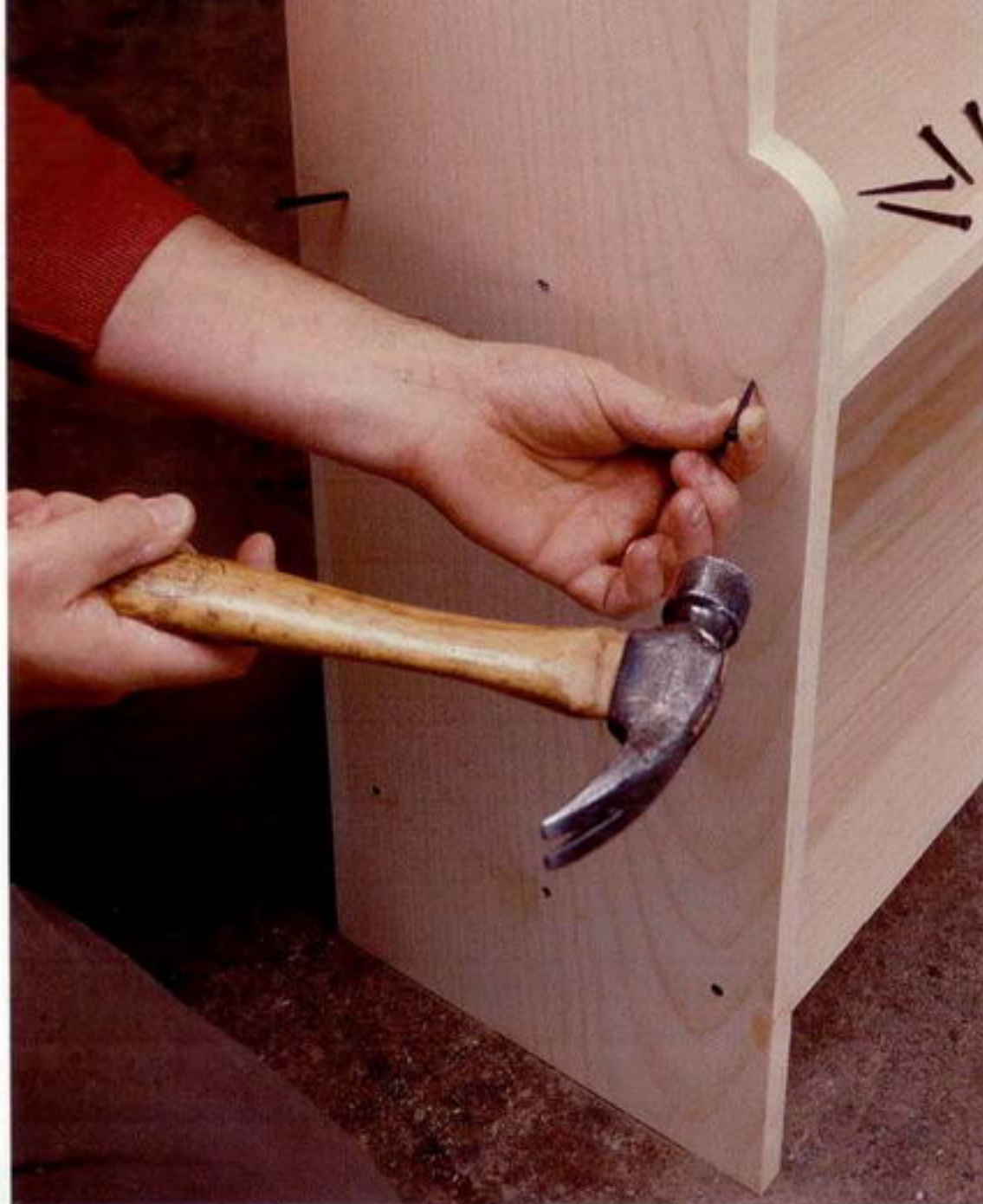
Photo C: Alternate the angle of the nails into the shelf ends to give the joint greater strength and to prevent them from pulling apart.
