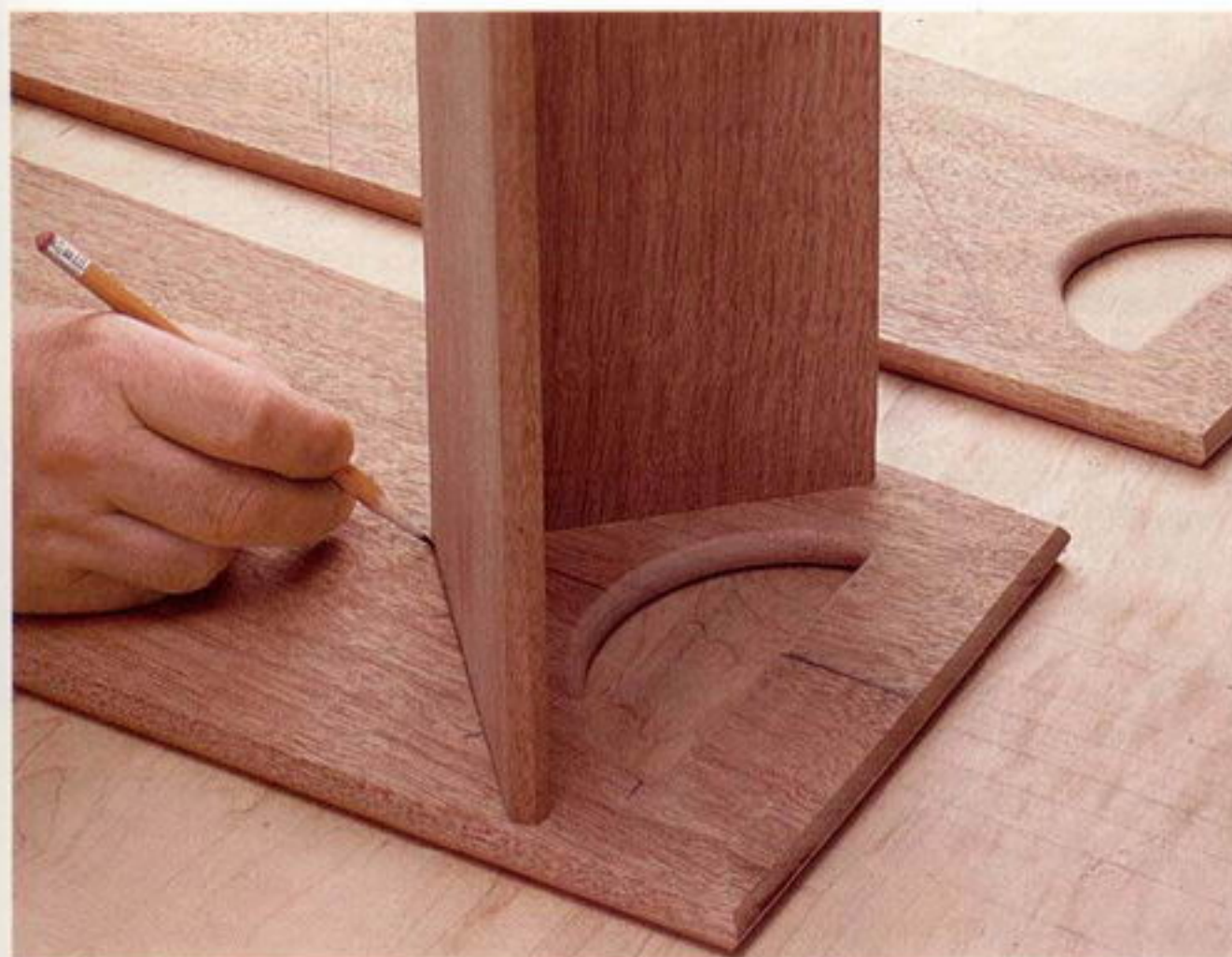
Photo F: Use the assembled V-shelves as marking guides. Scribe a line around the bottom of the shelf to help you align the biscuit joiner in the cut.
