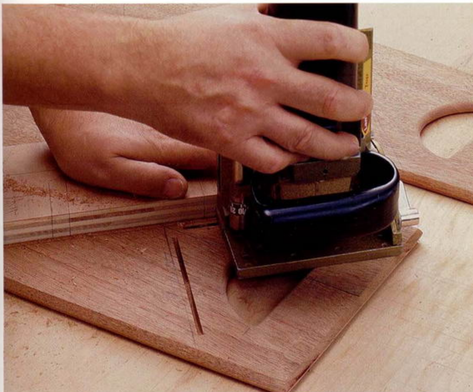
Photo H: A \frac{3}{4} -in.-thick scrap of plywood aligned on the reference line makes an excellent guide for the biscuit joiner when making the V-shelf cuts.
