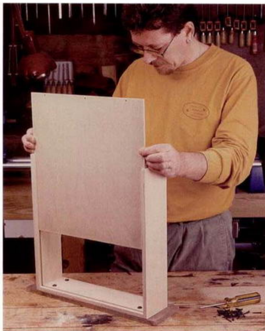
Photo G: Slide the drawer bottom in last, and attach it with three screws at the back. It will get in the way when attaching the drawer fronts if it's put in earlier.
