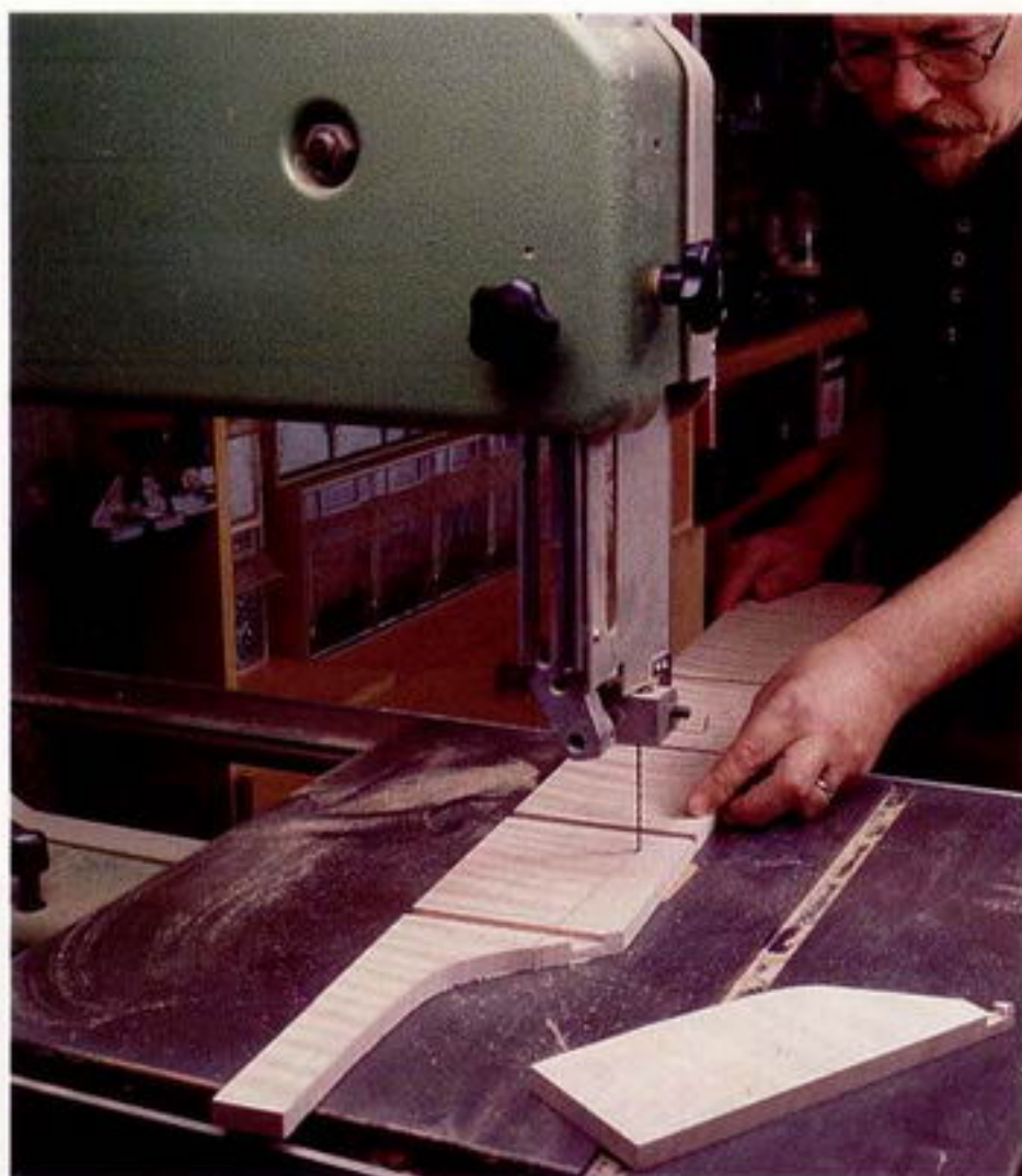
Photo C: Rough out the profile of the sides on the bandsaw after you've cut the joinery. Try to cut as close to the line as possible without going over it.
