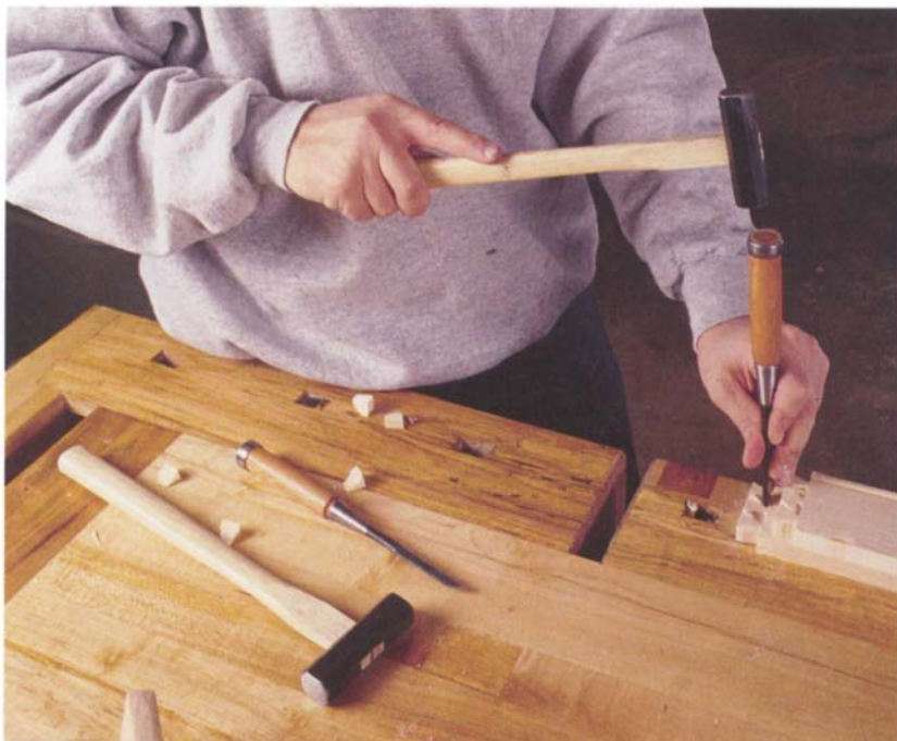
Photo M: To make the initial baseline cuts on the tails, tap the chisel straight downward.
