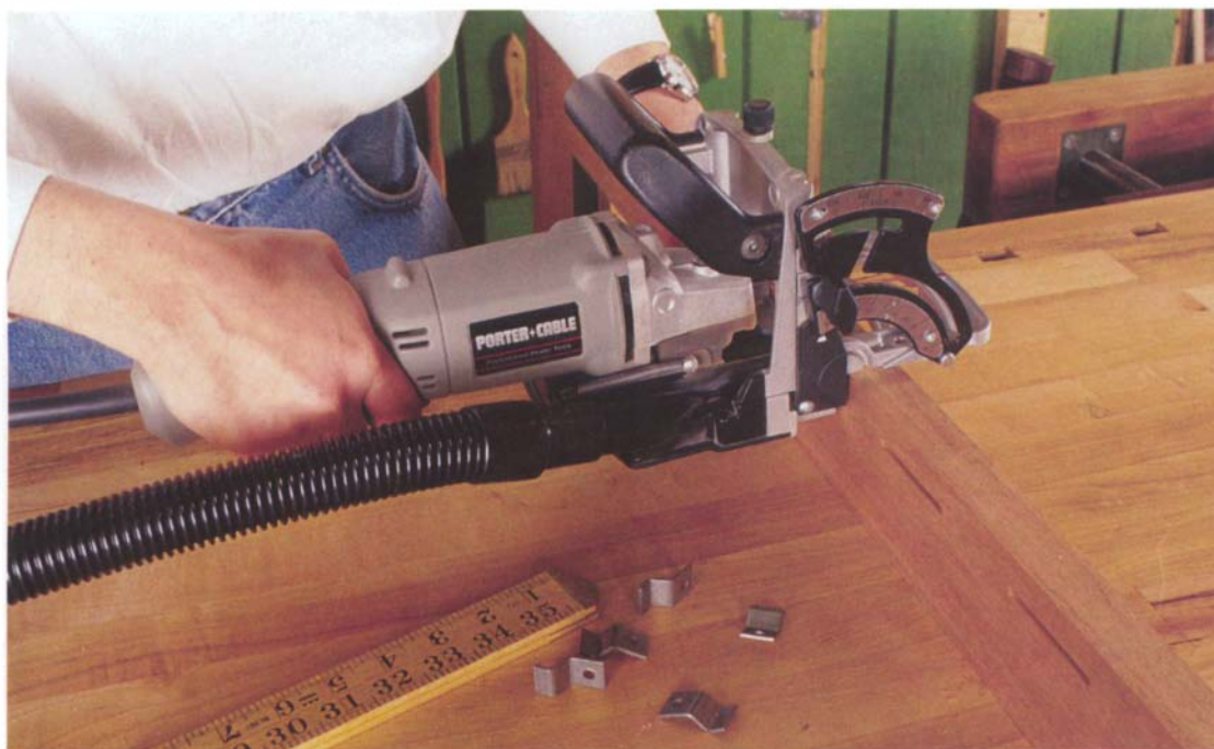
Photo K: A biscuit joiner is a good tool for cutting tabletop fastener slots into aprons.
