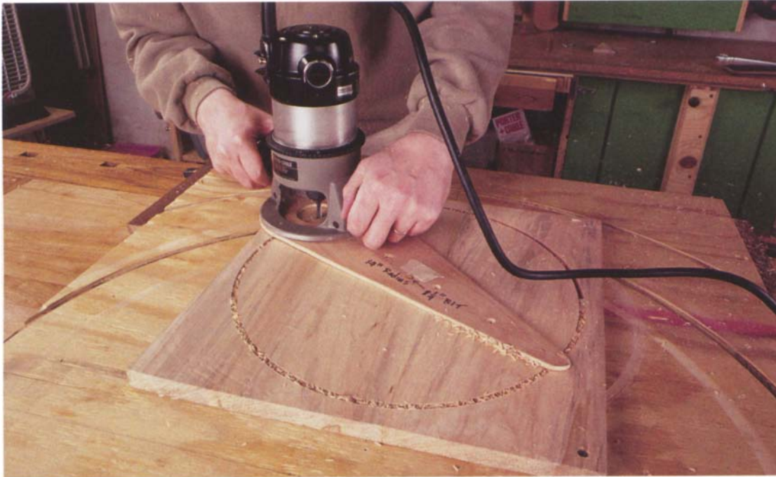
Photo C: Cut out the circular top with a router and trammel.
