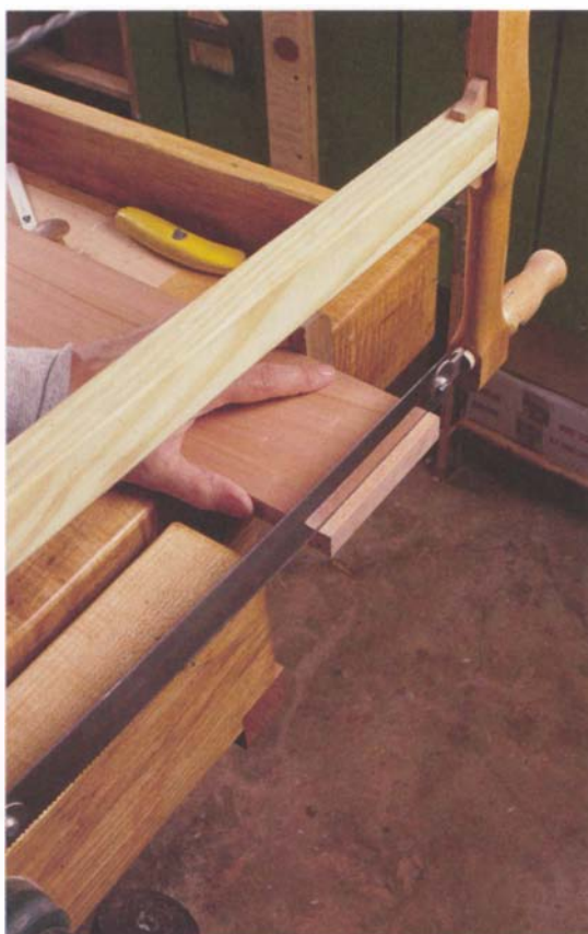
Photo I: Although you could use a backsaw to cut the tenon shoulders, I prefer a bowsaw for its speed and accuracy.
