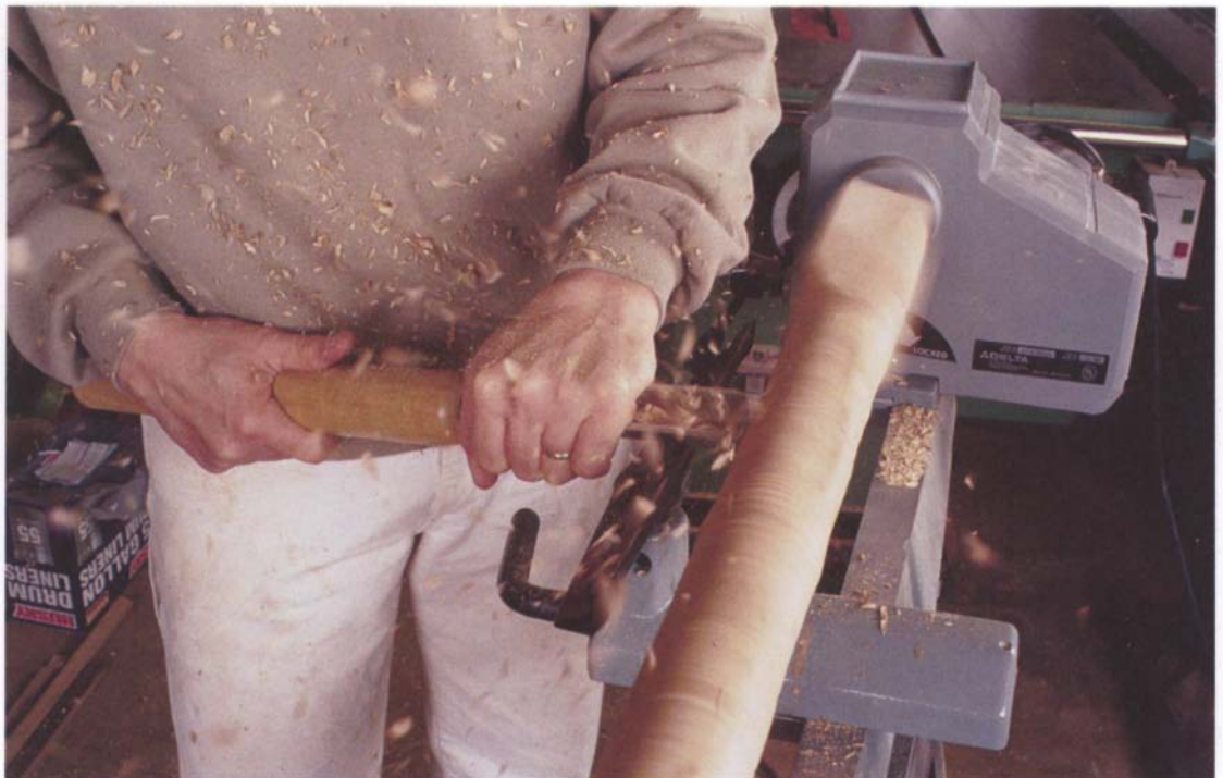
Photo E: Begin shaping the post with a roughing gouge, turning the blank to a 2\frac{1}{6} -in.-diameter cylinder.
