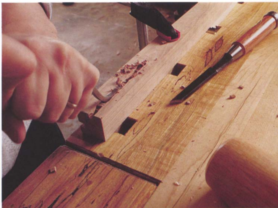
Photo G: Even up the depth of the mortise with a swan-neck chisel.
