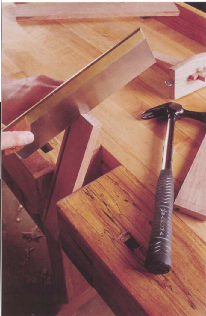
Photo G: Make the initial cuts for the half-blind pins by angling the front-to-rear direction of the saw at 8 to 12 degrees while holding the walls of the saw plumb. Tilt the saw upward to cut between your two marking-gauge lines.
