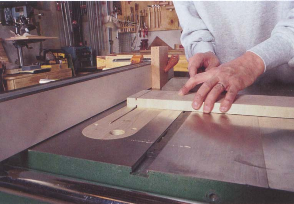
Photo G: Saw the tenon shoulders using the saw's miter gauge and a stop block clamped to the rip fence to register the cut. The stop block prevents kickback that can result from pinching a crosscut piece between the blade and the fence.
