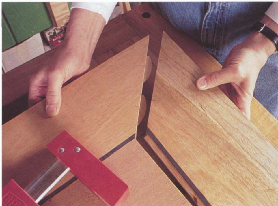
Photo B: Dry-assemble all of the top pieces together before glue-up to make sure they fit tightly.
