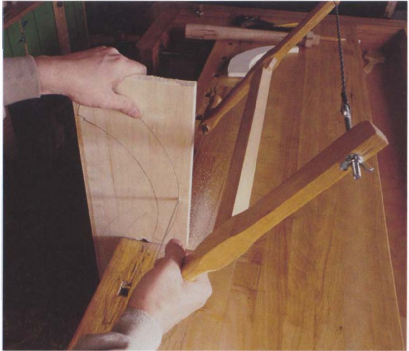
Photo J: After laying out the legs on \frac{3}{8} -in.-thick stock, cut out the shapes using a bandsaw, jigsaw, or scroll bowsaw (shown).
