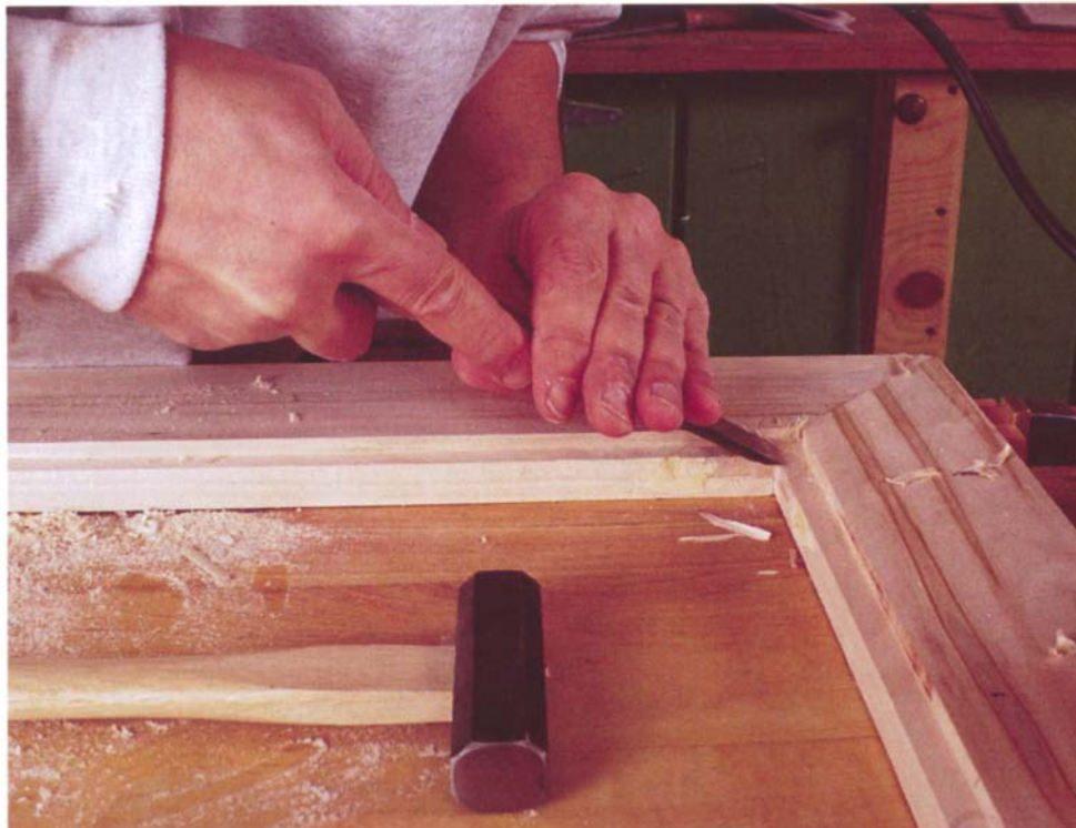
Photo C: Clean up the bottom of the rabbet corner with a chisel.
