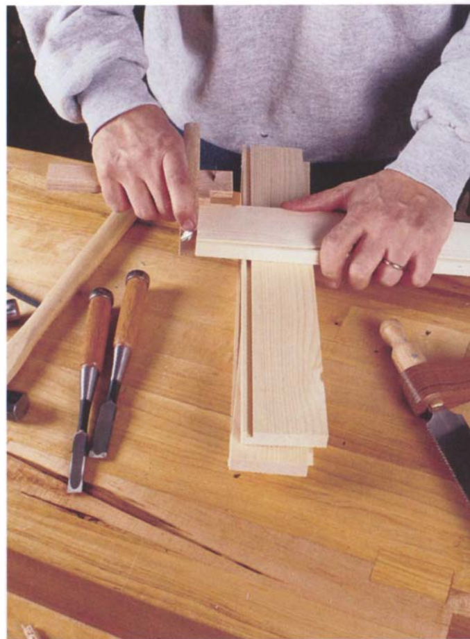
Photo K: Use a marking gauge set to the thickness of the drawer stock to establish the baseline for the pins and tails.
