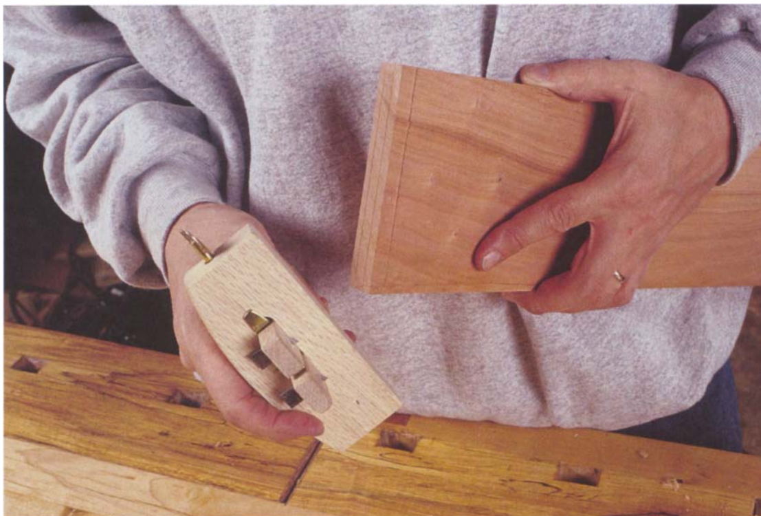
Photo H: Mark out the widths of the apron tenons using a mortising gauge adjusted for a \frac{3}{8} -in. tenon.
