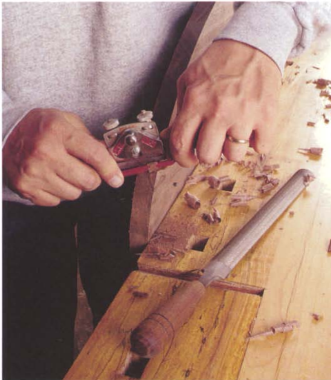
Photo B: Clean up the sawn edges of the top using a spokeshave and file.
