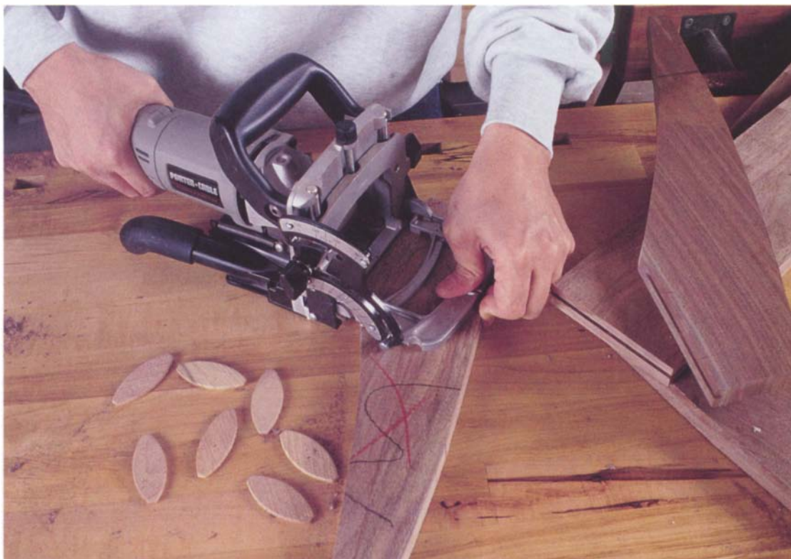
Photo F: Cut two slots for #20 biscuits into the joint face of each leg and into the ends of each rail.
