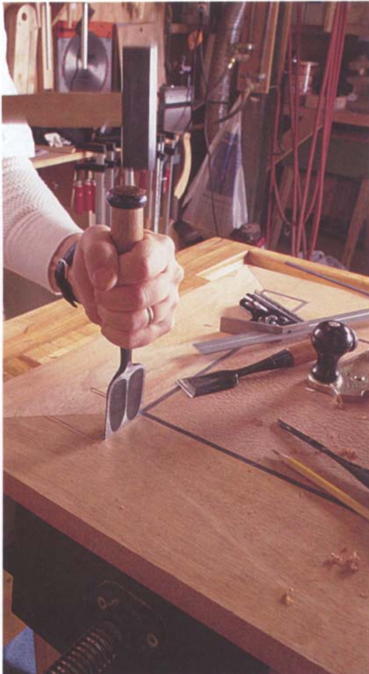
Photo E: To cut the inlay grooves by hand, begin by carefully chopping the walls of the grooves with a sharp chisel set in your knifed lines.
