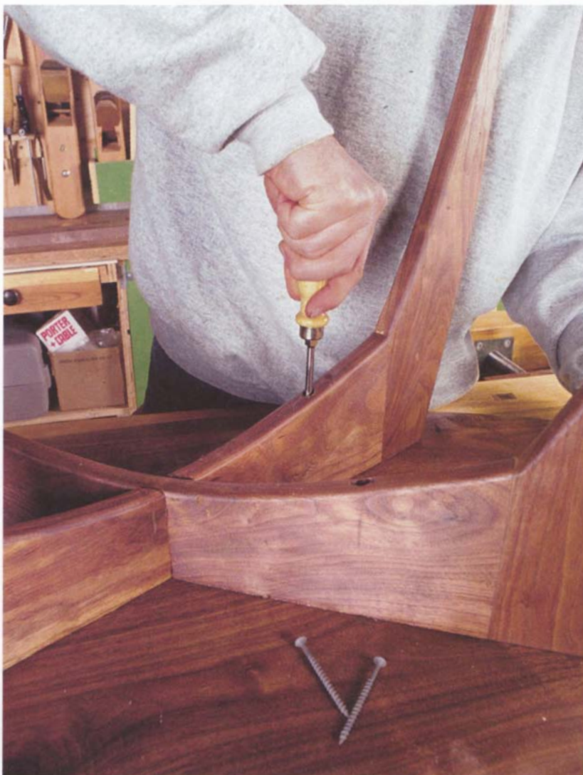
Photo K: To attach the top, drive two 2½-in.-long self-tapping dry-wall screws through the counterbored holes in the rail and into the tabletop.
