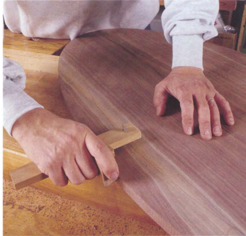
Photo C: Use a marking gauge to define the inside edge of the chamfer on the underside of the tabletop.
