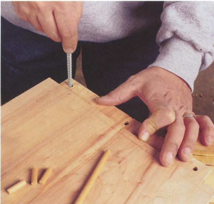
Photo D: To accommodate cross-grain movement of the plank, elongate the outermost holes in the tongues.
