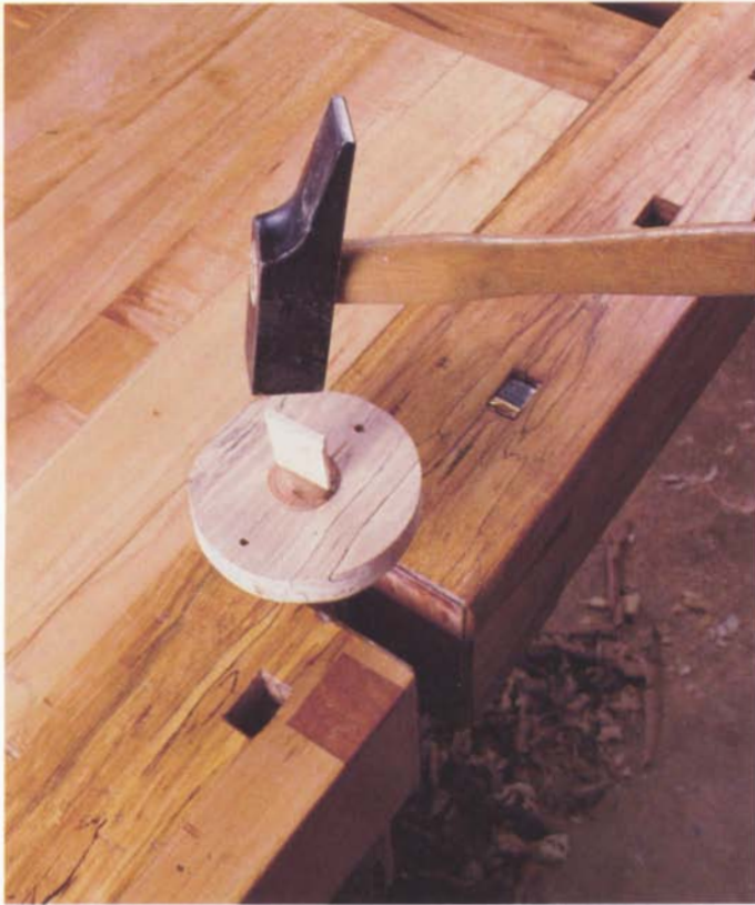
Photo L: Glue the mounting ring to the post tenon, orienting the wedge perpendicular to the grain of the ring. Apply glue to the wedge and kerf, then lightly tap the wedge in place.
