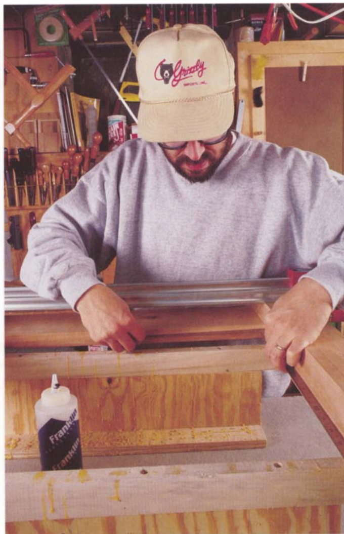
Photo K: Working on a pair of clamping stands, I clamp the short aprons to the legs, then check that the assembly is square.
