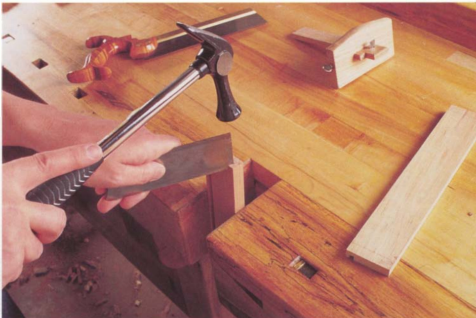
Photo H: Complete the initial pin cuts by inserting an old scraper into the saw kerf and tapping it down to the pin baseline.
