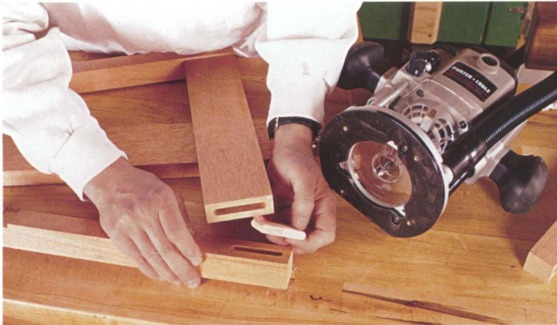
Photo I: After rounding over the edges of the tenon stock and cutting the tenons to length, dry-assemble the leg-to-apron joints. The tenons should fit in the mortise snugly, requiring only a bit of finger pressure to insert them.
