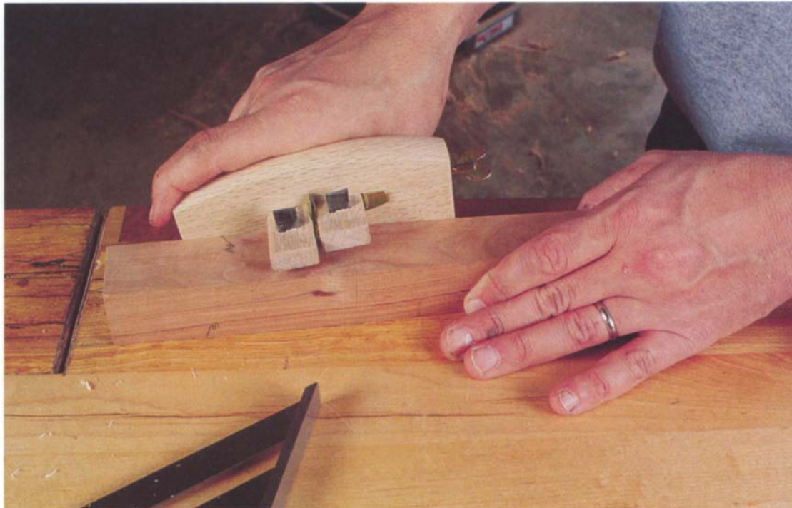
Photo E: Use a mortising gauge to lay out the leg mortises. Remember that the aprons are set back ⅛ in. from the outer faces of the legs.
