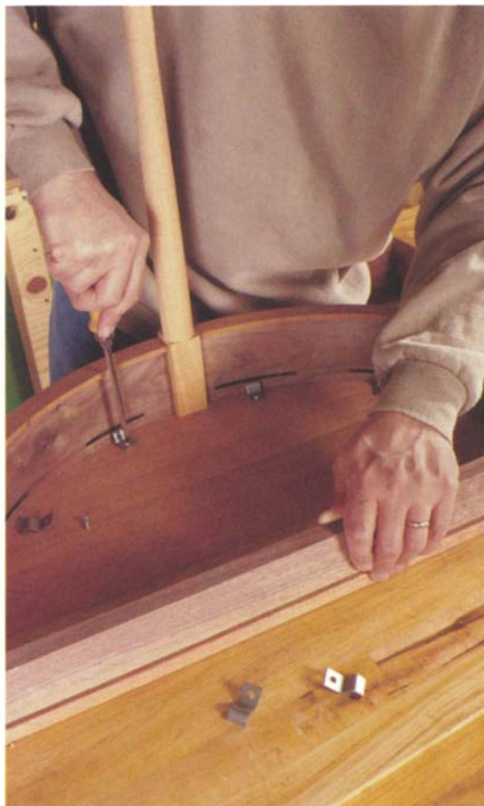
Photo L: Attach the top using tabletop fasteners set into grooves in the curved apron.
