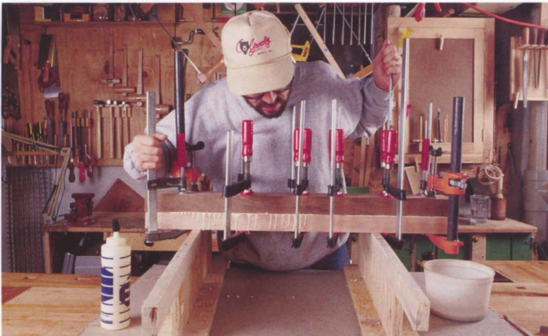
Photo E: Clamp the two leg halves together using a lot of clamps near the edges of the pieces.
