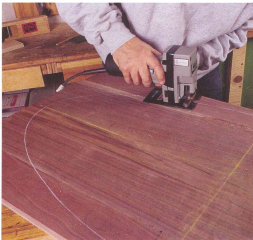
Photo A: Carefully cut the oval out of the blank with a jigsaw. The more smoothly you cut the curves, the less cleanup work you'll have to do.
