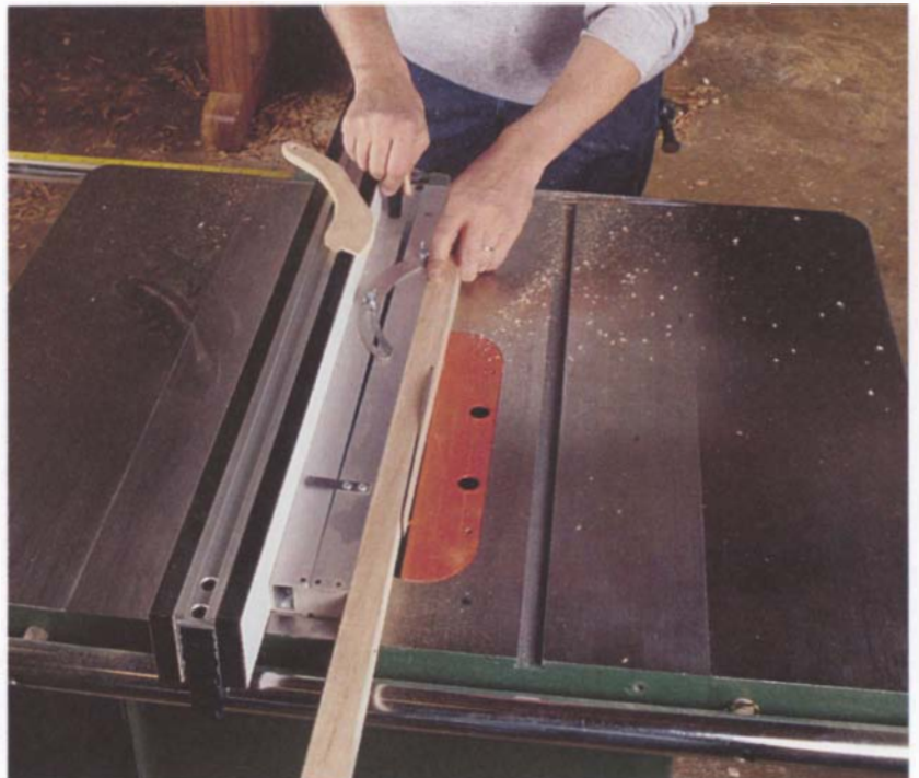
Photo D: Tapering the table legs is easy with a tapering jig. A tab at the operator end of the jig holds the work as you push it forward. As you near the end of the cut, hold the workpiece against the jig with a push stick.
