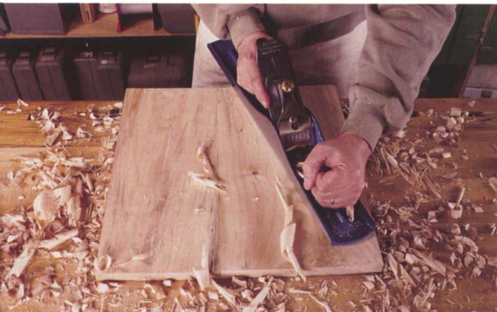
Photo B: After smoothing with a no. 5 jack plane, finish up planing the blank using a jointer plane, moving only in the direction of the grain.
