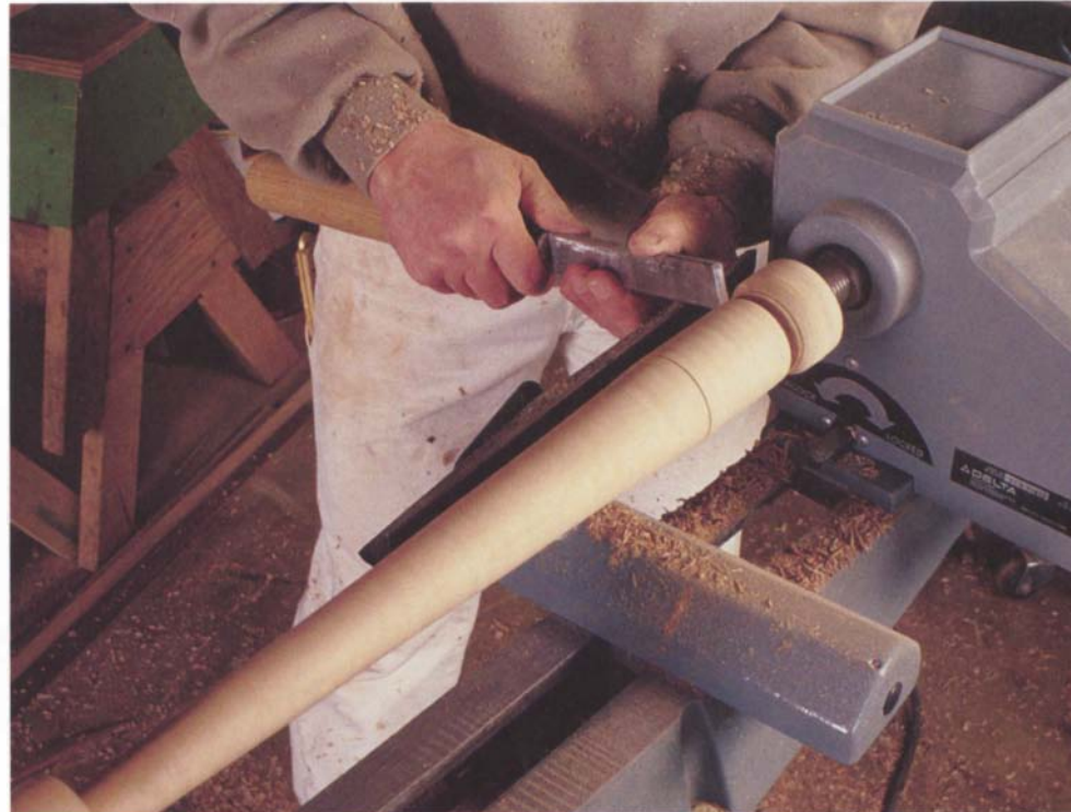
Photo G: Part the post from the blank, then saw off any remaining nubs.
