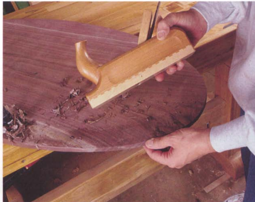
Photo E: Plane a gently sloping chamfer on the underside of the tabletop, staying between your gauge lines.
