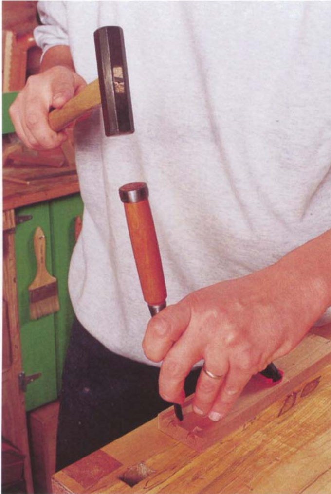
Photo I: Chop out the waste with a sharp chisel.
