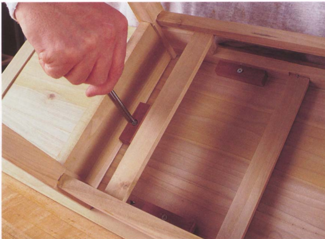
Photo J: Screw the top to the carcass through the screw blocks.
