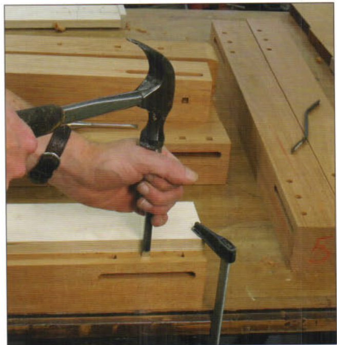
A modified chisel from a hollow chisel mortising machine makes the round holes square. A scrap of plywood clamped to the leg tangent to the holes registers one edge of the plugs and keeps them aligned.
