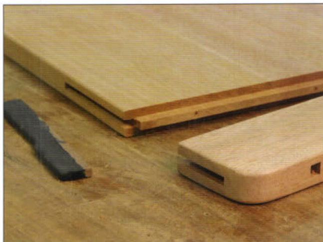
If the breadboard end is thicker than the top, be sure to account for that when milling the grooves for the tongue and splines.
