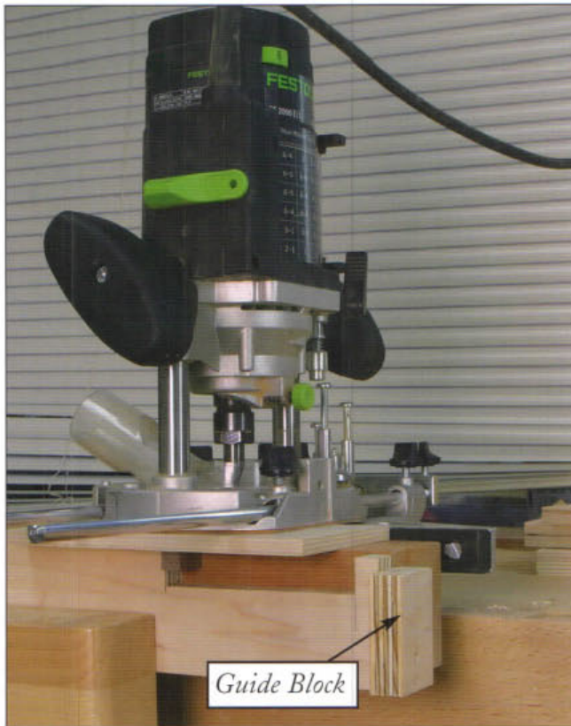
The leg and notched template are placed together in the bench vise. The block on the end of the template registers the template against the end of the leg.
