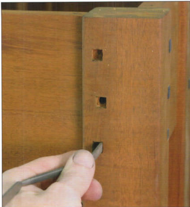
A small flat riffler file cleans up the edges and bottoms of the square holes.
