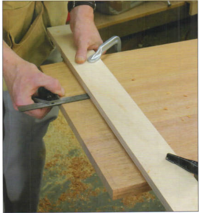
Clamp a straight edge across the end of a top to act as a guide for a router to form the tongue for the breadboard end. A combination square will set the distance quickly and accurately.
