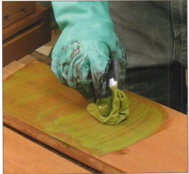
After treating the wood with a potassium dichromate solution, a green stain is applied. The stain is mixed by adding artist's oil colors to a base of Danish oil.
