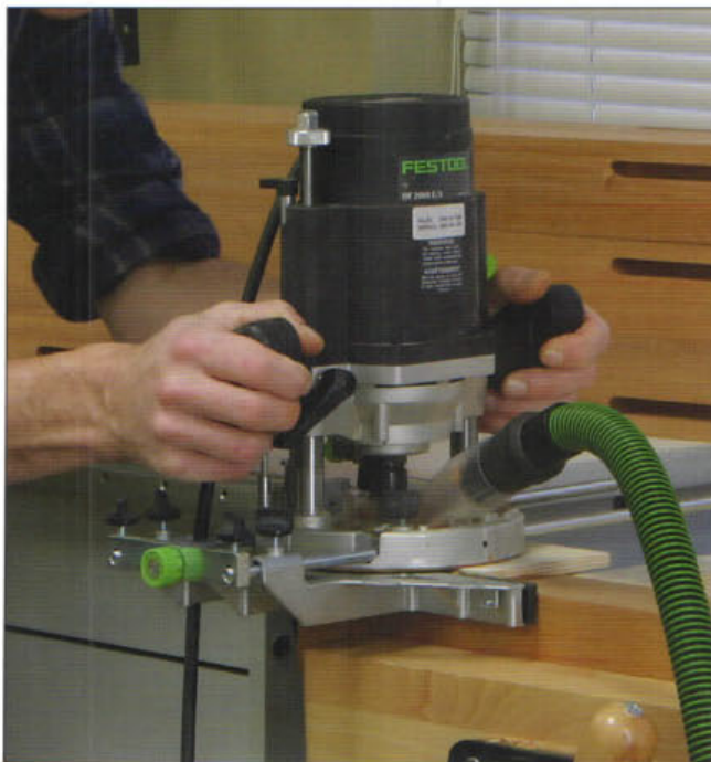
This method allows mortises to be routed without the need for laying out and marking each and every joint.
