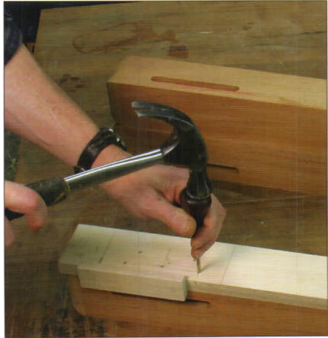
A plywood template is used to mark the centers of square plug locations. After marking, holes are drilled to a consistent depth with a Forstner bit.
