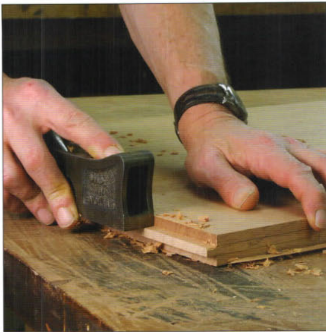
Fine-tune the fit of the tongue, and refine the edge of the shoulder, with a shoulder plane.
