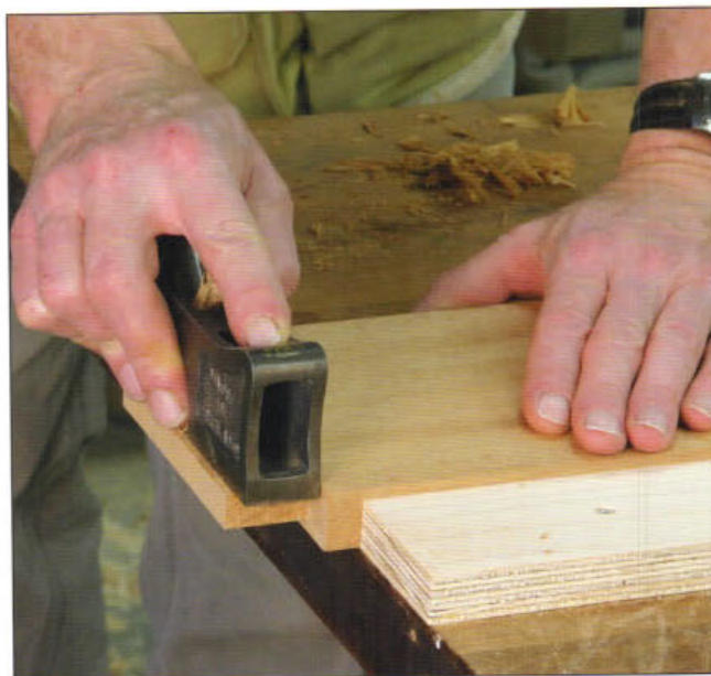
A scrap of wood attached to the top of the bench acts as a stop so that the tenons can be trimmed without clamping them. A shoulder plane or a rasp will remove a small amount of material in a controlled manner.
