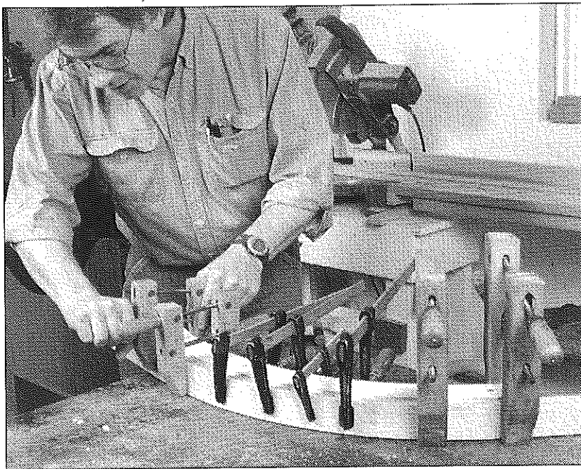
Bending thin laminates around a form.
