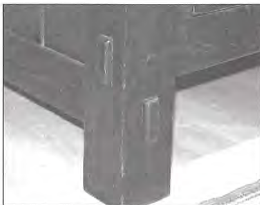
Edges are gently chamfered or rounded in original pieces. Variations in individual pieces indicate that this work was done by hand.
