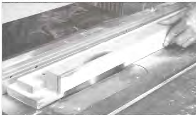
Taper jig consists of a plywood sled with screwed-down blocks to hold the workpiece in place.
