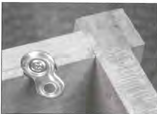
Square the sides of the recess so that the figure 8 fasteners can swivel.
