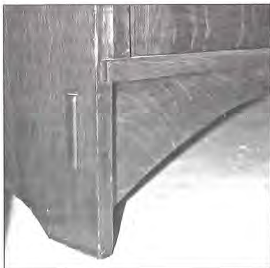
Exposed mortise and tenon joinery is typical in Craftsman furniture.
