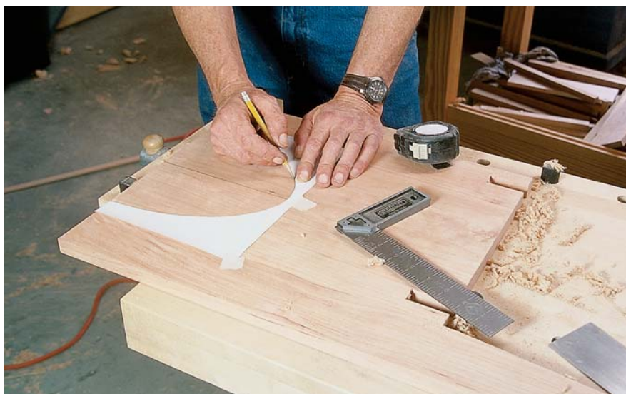
After the joints are cut and the back extension is glued on, position the paper pattern and mark the arched cutout.
