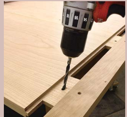
Holes in the outer tenons are elongated to keep pegs from splitting the top during seasonal movement.
