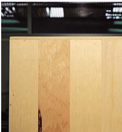
The \frac{1}{4} " spacing shown on the back panels is accomplished by rabbeting a \frac{1}{4} " x \frac{1}{2} " rabbet on opposing long edges.
