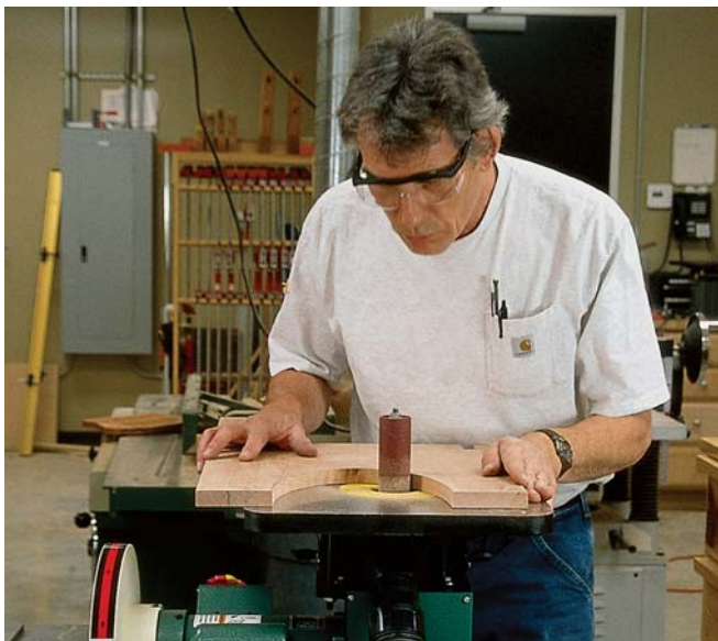
The oscillating spindle sander is ideal for cleaning up the saw marks and sanding to the inside of the pencil line.
