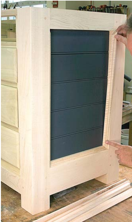
The panels on the base are held in place by the moulding that is installed in picture-frame fashion – the corners are mitered.
