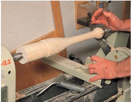
Turning the pedestal is a great way to practice your lathe skills. While there is a pattern to follow, the lines are fluid enough to allow for personalization, slight miscalculations or both.
