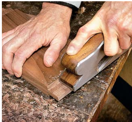
The tenons can be fine-tuned with a shoulder plane or a rabbet plane.
