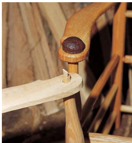
The arm shown with the wedge in place in the front-leg split tenon, waiting for a cookie. A finished version is shown behind.
