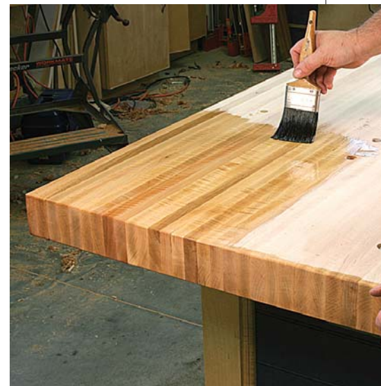
Two coats of an oil/varnish mixture is all the protection necessary for the bench. You don't want too much finish on the top. There's no need to have pieces sliding about.
