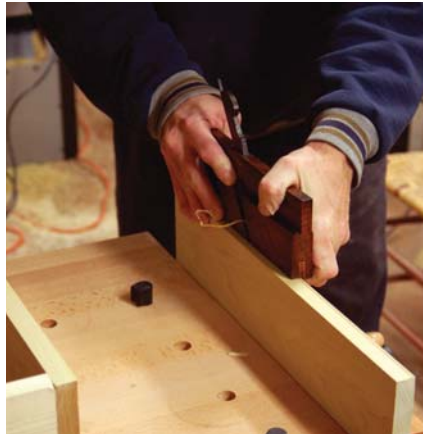
Although the bead on the Shaker original was likely made with a scratch stock (because there is evidence of this tool everywhere at Pleasant Hill), I chose an 1/8" side-bead plane.
