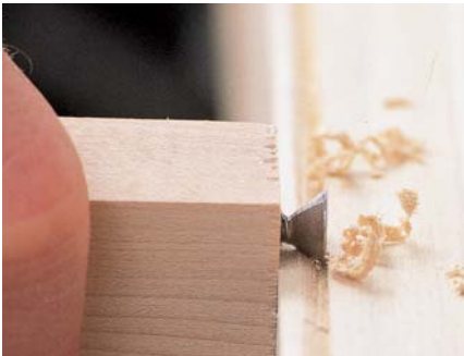
The homemade 10-minute cockbeading tool in use.
