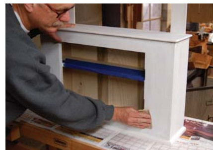
The original cupboard had been stained. I chose to use a primer and paint combination in order to best mimic the look of the aged original finish.
