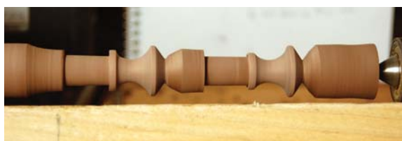
Use a skew to shape the top of the knob and a fingernail gouge to cut the cove. The tenon can be cut with a paring chisel laid flat on the rest with the bevel down.
