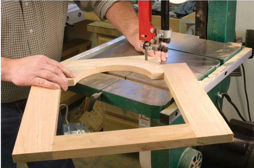
Fit the hood door. Once the outer arch is cut, the door is fit to the hood. Fit the door in position then fine-tune the fit to create an even reveal around the door.
