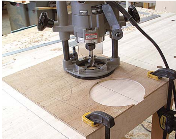
Drilling holes for bench accessories is a task that can kill a drill, but with a plunge router and upcut router bit, the job is short and sweet. Align the centers and rout.
