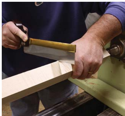
A simple saw cut at your layout line determines the shoulder and helps to keep it intact while turning.
