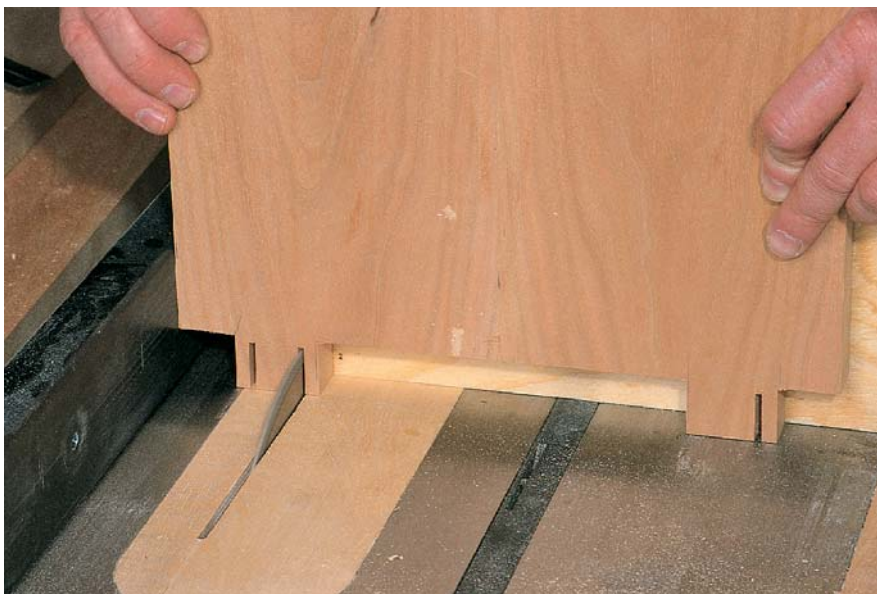
Cutting Tenons. Cut the tenons to the actual width on the table saw. Set the blade to 1" high, defining the length of the tenons. After marking the depth with a gauge, cut the waste out from between the tenons. Set the saw to \frac{7}{8} " high for cutting the slots that accept the wedges used to hold the table together. See the diagram for the actual size of the outer parts of the tenon. Use a backing board on your miter gauge to hold the boards upright
