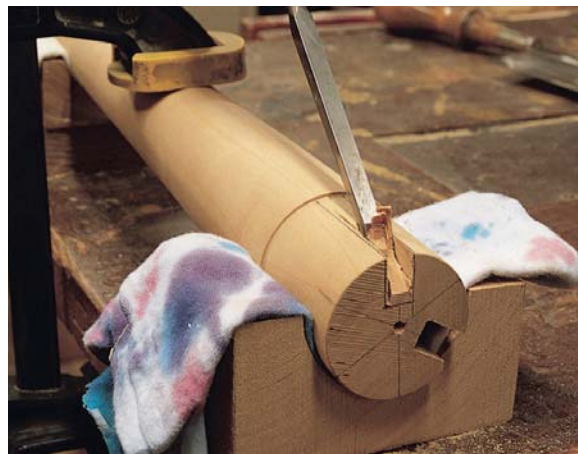
Begin chopping out the waste with a mortise chisel.
