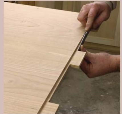
The long tenons of your breadboard end hold pieces to the top, but it's the ¼" tenon that runs the width of the top that keeps things flat and level.
