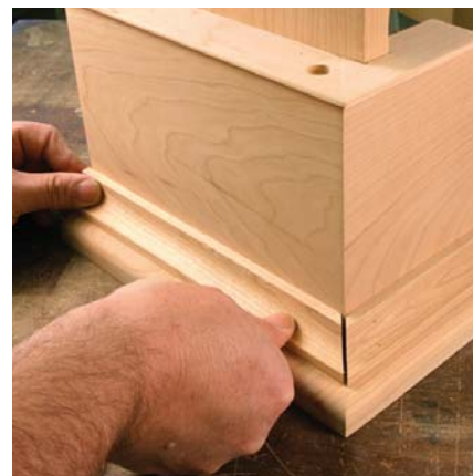
This moulding is created at the router table with a ½" cove bit. The bit is slightly raised with each pass, creating the irregular profile.
