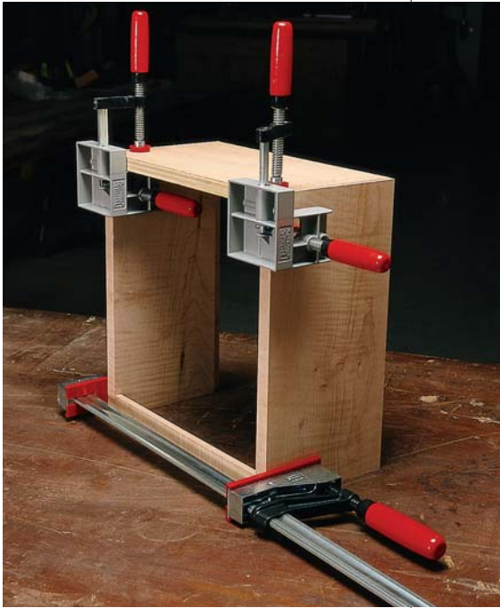
These 90° clamps made gluing up the top case a lot easier. Getting things square was a real snap.
