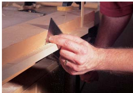
Clamp a straightedge to the back line of the stool, gently press the saw against it and rip the back edge (left). Use the ripping teeth on the back of the Ryoba.
