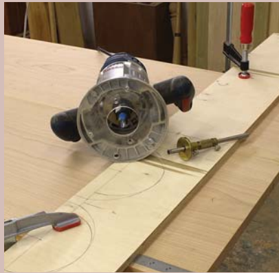
A plywood straightedge guides my router in the first step to forming a tenon for the breadboard ends on the countertop. A 1 ½"-long tenon is the result.
