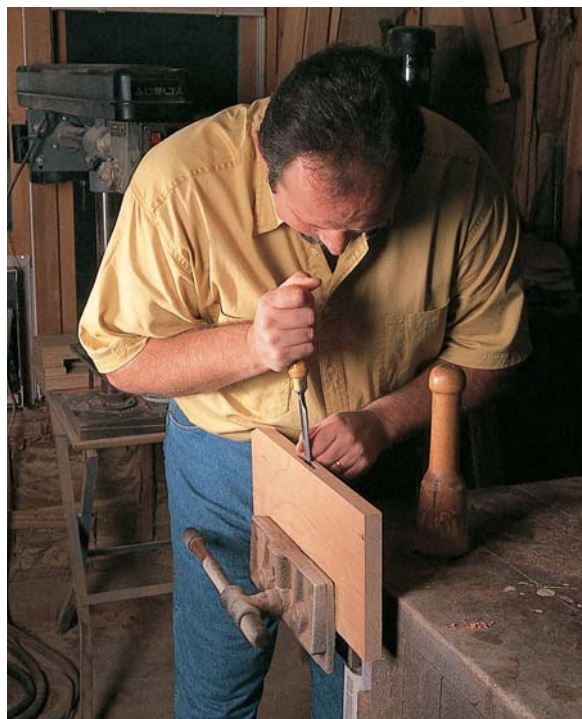
After drilling out the mortises in the feet using my drill press, I cleaned up the mortise and squared the corners with a chisel. I'm glad they shot this picture because I don't use hand tools too often.
