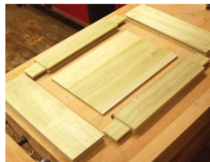
Before you glue up the door, lay out the parts and make certain that they will all come together during glue-up.
