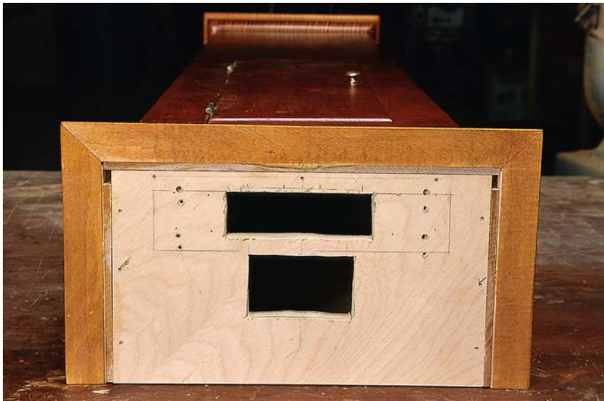
Here you can see the cutouts to accommodate the swinging pendulum and the hanging chains from the works.
