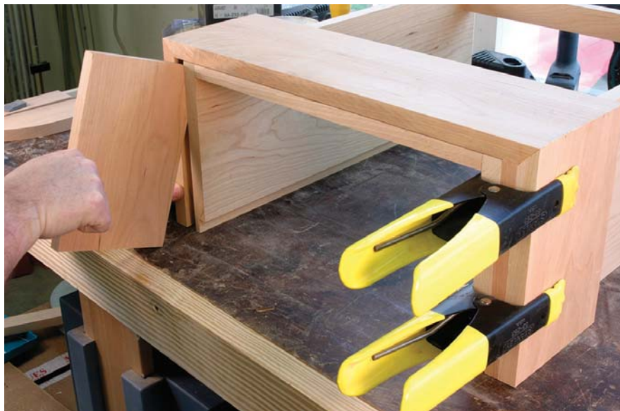
Taking the time to check the fit of the gallery assures a proper fit. After the gallery is assembled the spacers can be manipulated to specific thickness.
