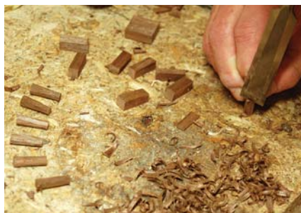
Riven pegs are not only historically accurate, they are also stronger than sawn pegs because they eliminate the possibility of grain run-out.
