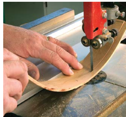
Trim the bead to width at the band saw, but the majority of the work of matching to the flat bead is completed with chisels. Carefully angle the ends of the bead to fit those of the matching corner pieces.
