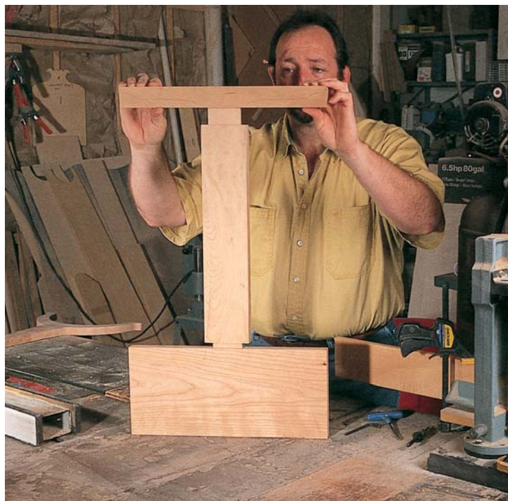
With the mortise-and-tenon joints complete, I transferred the shape of the legs from the template to the pieces. Band saw the shape, then sand the edges smooth. You might note that the grain orientation on the feet isn't really the best, as it makes a weak support. But when making a reproduction....
