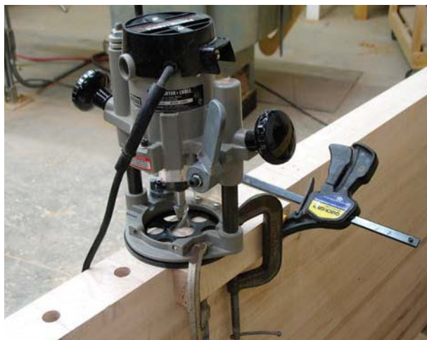
A second rigging is needed to drill the holes in the top's front edge. These holes are for accessories that hold wide panels in place.
