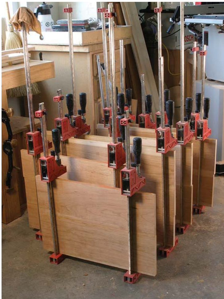
A sea of panels. I wanted to glue up all the panels at the same time – but I ran out of clamps and space. Above are the six door panels and two lower side panels.
