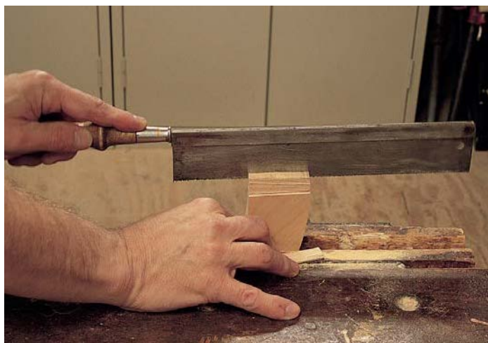
Mark the shoulders of each tenon and then, with a backsaw, cut each shoulder to depth. Then rough in the tenon cheeks.
