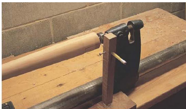
The lines being drawn with my marking gauge divide the circumference of the pedestal base into three equal sections. Each of these lines will become the center of a leg-tenon mortise.
