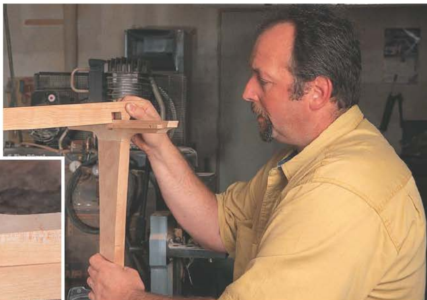
The legs and stretcher are held together with an edge-lap joint. The legs are notched through the mortise-and-tenon joint (left), and a mating notch is cut in the stretcher (above).
