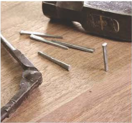
I laid out the nails using dividers (shown on the left). Then I drilled 3/32" pilot holes and drove in the 6d nails and set them with a homemade nail set.
