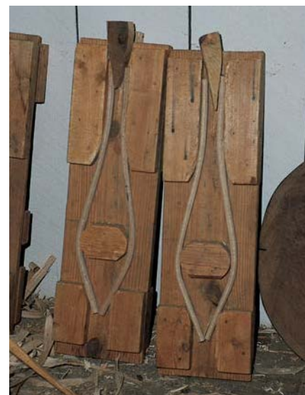
The jigs I use are fairly simple 2x material with blocks added to space and shape the pieces. Two sets of back rails are shown. The jigs for the back legs are even simpler.
