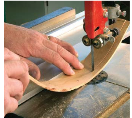
Trim the bead to width at the band saw, but the majority of the work of matching to the flat bead is completed with chisels. Carefully angle the ends of the bead to fit those of the matching corner pieces.
