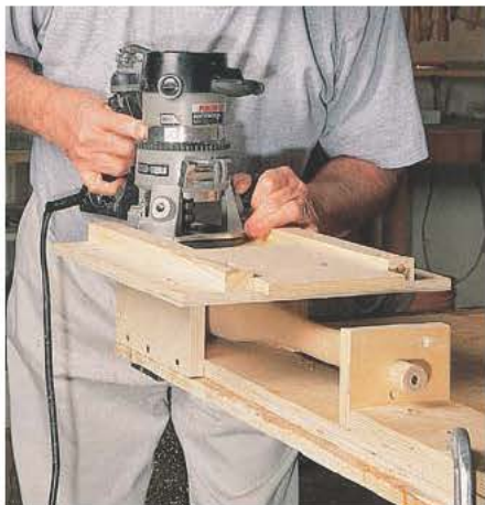
The dovetailing jig makes it fairly simple to place the leg, run the groove, then rotate the leg to the next position. Note the screw in the diagram and photo that's used to hold the pedestal in the appropriate position.
