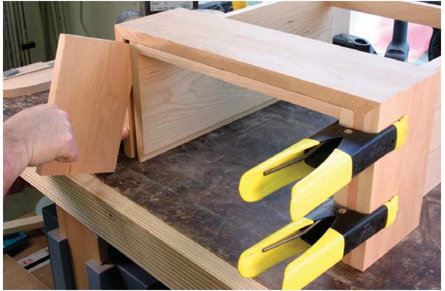
Taking the time to check the fit of the gallery assures a proper fit. After the gallery is assembled the spacers can be manipulated to specific thickness.
