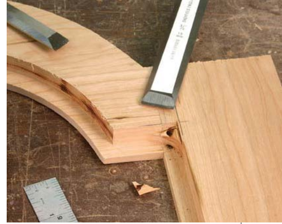
Prep the door for glass. The inside corners are left rounded by the rabbeting bit and need to be squared with chisels. Cut the end grain using the force provided from a mallet while cutting the side grain with only hand pressure. Too much force can crack the face of the door.
