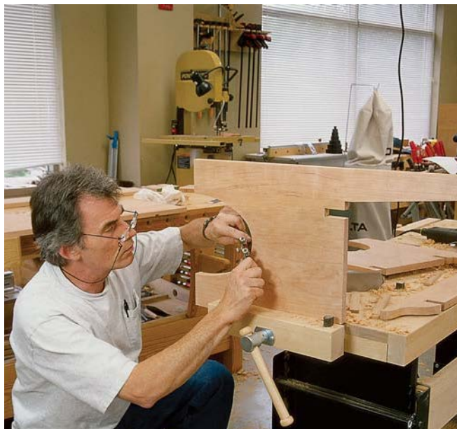
A spokeshave eases the edges the block plane couldn't reach.
