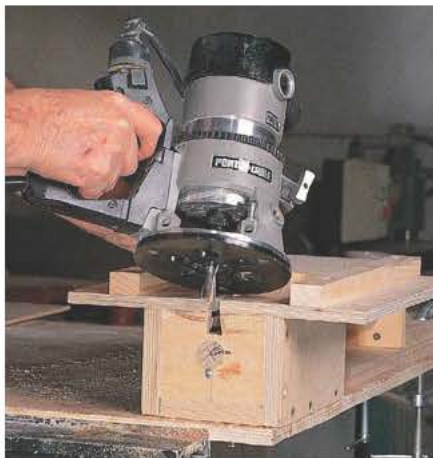
The dovetailing jig makes it fairly simple to place the leg, run the groove, then rotate the leg to the next position. Note the screw in the diagram and photo that's used to hold the pedestal in the appropriate position.
