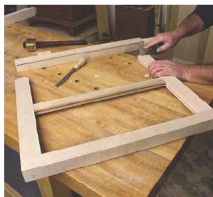
Dry assembly is the best time to discover that your tenons are too tight – not after glue is spread and things become messy.
