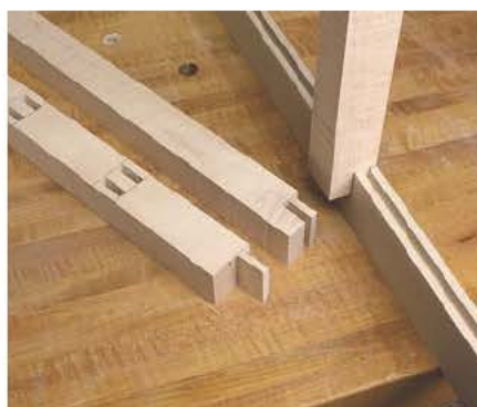
As the sole runner support, these dividers need strength. A screw through the back and a tenon in the rail gives the vertical dividers double the holding power.
