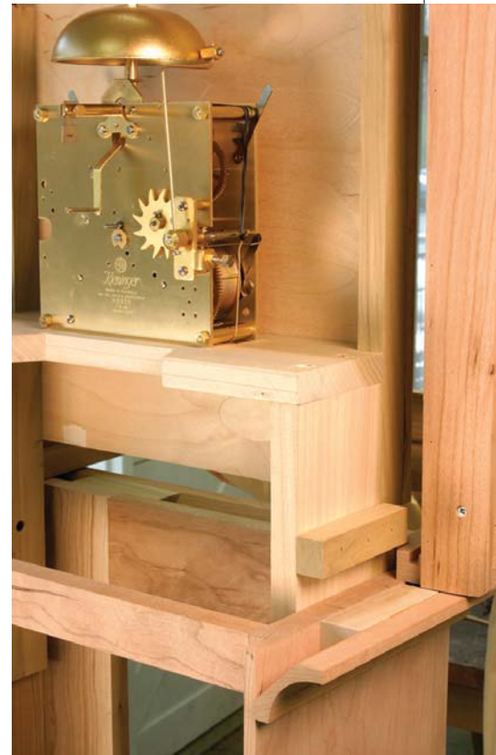
Positioning the movement. The seat board holds the movement in the correct orientation to the dial allows the weights to hang as needed. The cutout in the seat board is for the pendulum and the blocks attached to the sides keep the hood from tipping forward.
