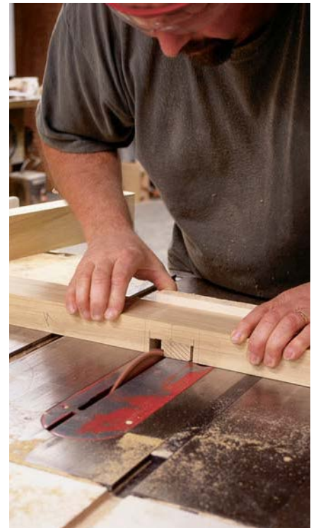
Nibbling away the mortise locations on the leg halves can be accomplished with a flat-tooth rip blade or a dado stack.
