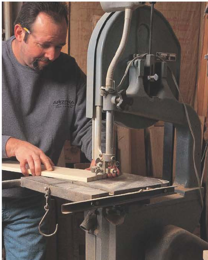
The drawers are assembled in traditional Shaker fashion using half-blind dovetails on the front—but that doesn't mean you can't cheat on what tools you use. After marking and cutting the pins on the fronts, the band saw makes quick work of what would have been a lot of hand-cutting to create the tails.
