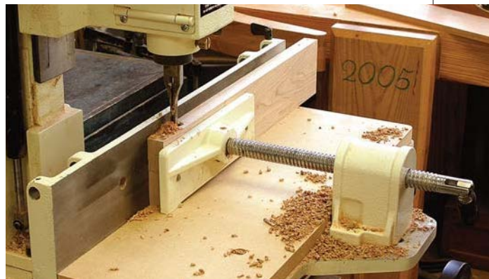
Many mortises. The majority of joints in this project are mortise and tenon. Take the time to set the hollow-chisel mortiser to cut dead-on centered mortises, \frac{1}{4} " deep – it will save you a lot of frustration and time later.
