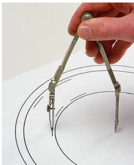
It's simple work to ink the lines for the paper face. After you make the three circles, use a compass to ink the top and bottom of the Roman numerals (right). Then ink the straight lines to fill in the numerals. It's not calligraphy, so you don't have to worry about curving lines far right).
