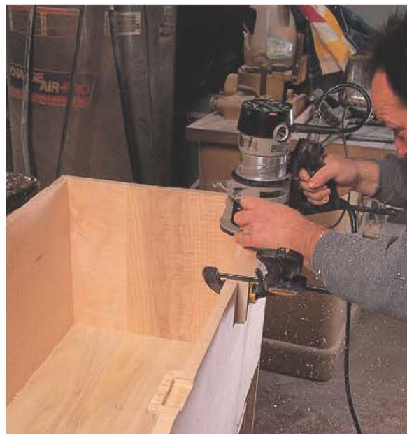
With the hinge blocks glued in place against the cabinet back, mark the hinge shape on the top of the block and the back. Next rout out the hinge mortise to the full depth of both hinge leaves.
