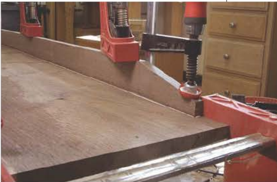
Some creative clamping ensures a tight joint. The clamp on the far right ensures that the apron will be flush to the edge of the seat at the ends. The F-style clamp keeps the tapered apron against the seat. Thank goodness for its swiveling clamping pad.
