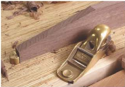
It only takes a few strokes to clean up the sawn edge with a plane. Any sharp plane will do – planing downhill is always easy work.
