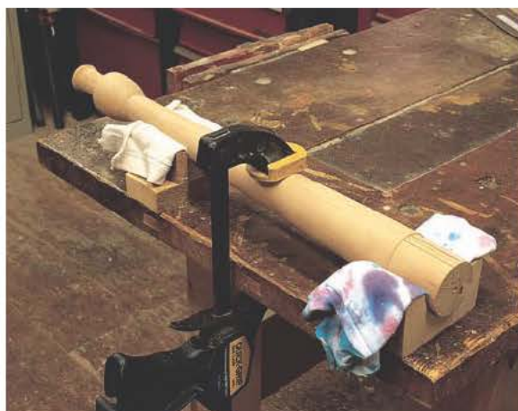
Fix the pedestal on your bench with a pair of U-blocks and a clamp.
