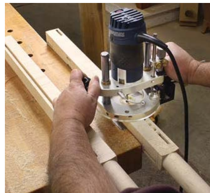
Instead of drop cuts at a table saw, it's best to use a plunge router and fence to make panel grooves.
