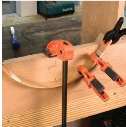
The offcut from the gallery front is an excellent caul for clamping the laminated bead into the profile. Small spring clamps close any gaps between the pieces.
