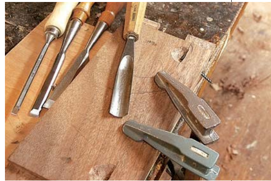
Paring chisels will cut the flat in each screw pocket. The rounded excavation can be made with a gouge.
