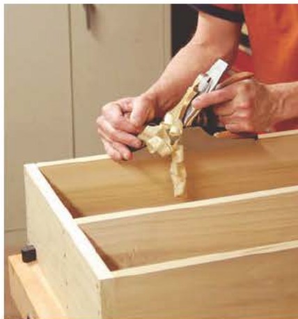
Use a plane to level the edges of the cupboard's case before you attach the face frame.
