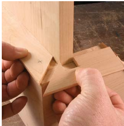
Locate and trim the notch with a handsaw then cut 45° miters at the end. The holes for the columns are centered in the flat bead and held flush with the front edge of the hood side.
