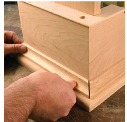
This moulding is created at the router table with a ½" cove bit. The bit is slightly raised with each pass, creating the irregular profile.
