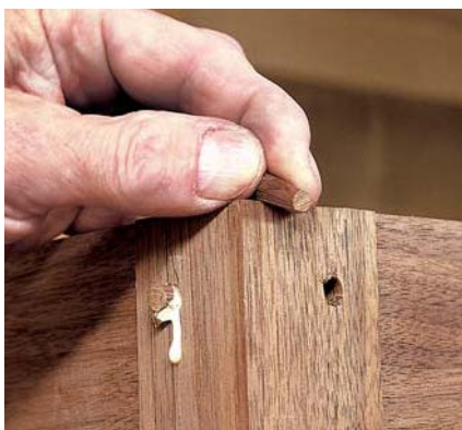
Split out the pegs. Then shave them to size with a paring chisel.
