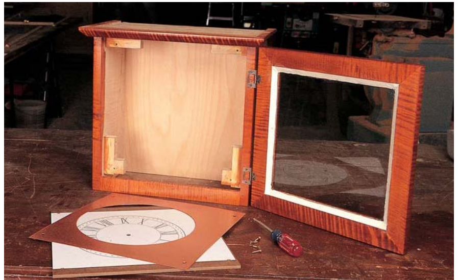
The bonnet, glazing compound, face, copper surround and cleats for attachment.
