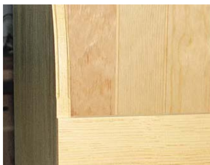
By using a portion of a Roman ogee bit, a delicate detail is added to the radiused edges of the sides. A cove bit with a guide bearing will also work.
