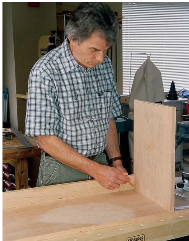
With the ends placed in the dados in the bottom of the seat, you can mark the location of the lap-joint cuts in the seat rail without measuring.
