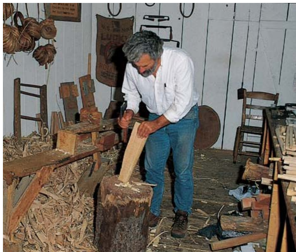
Most woodworkers don't list a hatchet as part of their tools, but when I'm chopping out the shape for the top slat it's my best friend.
