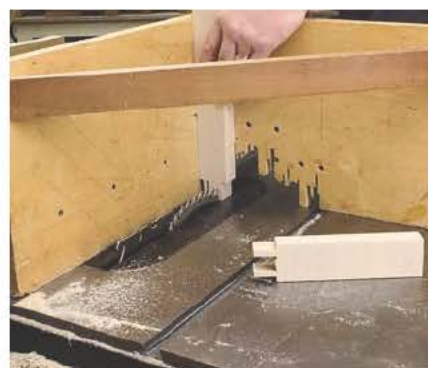
It's invaluable to test joinery setups using a scrap milled when your parts are milled. The twin tenons on the drawer blades can be fussy.
