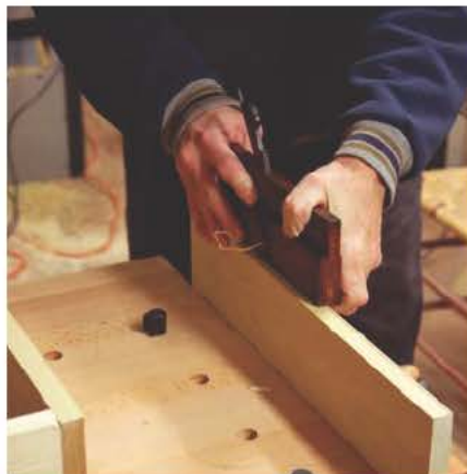
Although the bead on the Shaker original was likely made with a scratch stock (because there is evidence of this tool everywhere at Pleasant Hill), I chose an \frac{1}{8} " side-bead plane.
