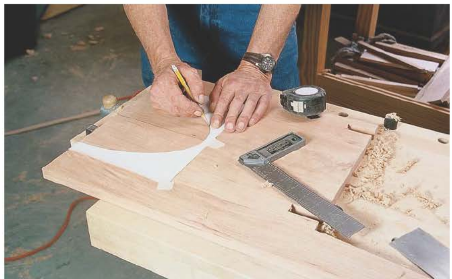
After the joints are cut and the back extension is glued on, position the paper pattern and mark the arched cutout.
