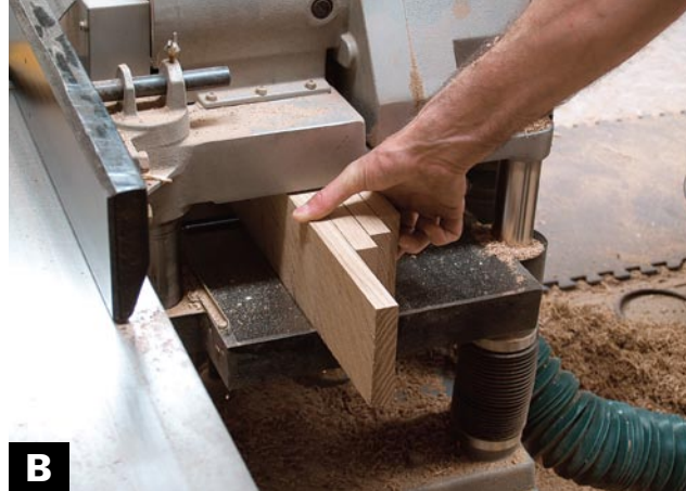
GANG-PLANE THE JOINTED BOARDS to a common width. Hold the boards together as they are pulled into the planer, and then grasp them tightly together as they emerge on the other side.
