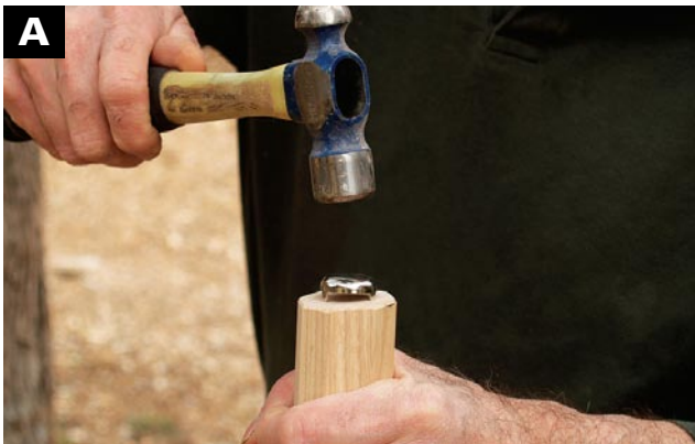
CENTER A GLIDE ON THE BOTTOM of each leg and tap it into place with a hammer or mallet.
