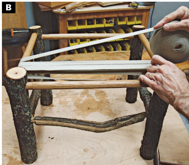
WRAP THE TAPE AROUND AND AROUND the side stretchers, maintaining a uniform tension as you go. For this first part, rather than cutting the tape in 3-yd. or 4-yd. lengths, I leave it in the roll to avoid having to join shorter pieces.
