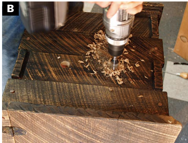
DRILL THROUGH THE SIDES FOR THE ROPE handles to fit. Drill only partway from the outside. When the tip of the drill bit starts to enter the inside, finish the hole by drilling from the inside. This will prevent tearout.
