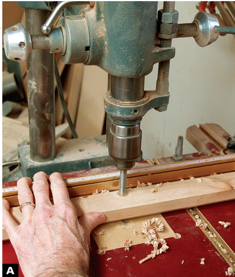
USE A DRILL PRESS AND FENCE to position the mortises accurately.
