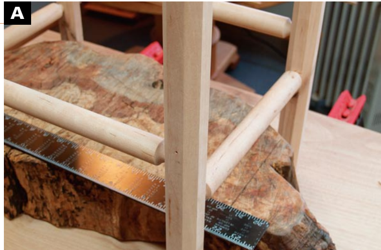
PLACE THE FRAME OVER THE STUMP to transfer the locations of the holes in the left and right stretchers so that the stump can be drilled for the dowels to fit.
