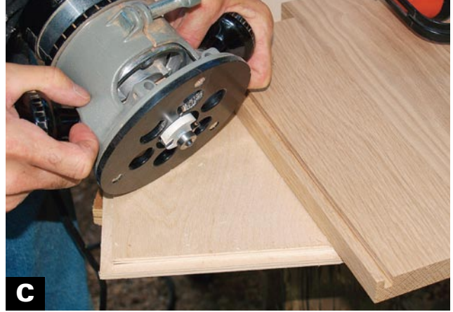
USE A \frac{3}{8} -IN. RABBETING BIT TO CUT the bottom panel edge. Adjust the depth of cut until the tongue will fit the groove in the sides of the chest.
