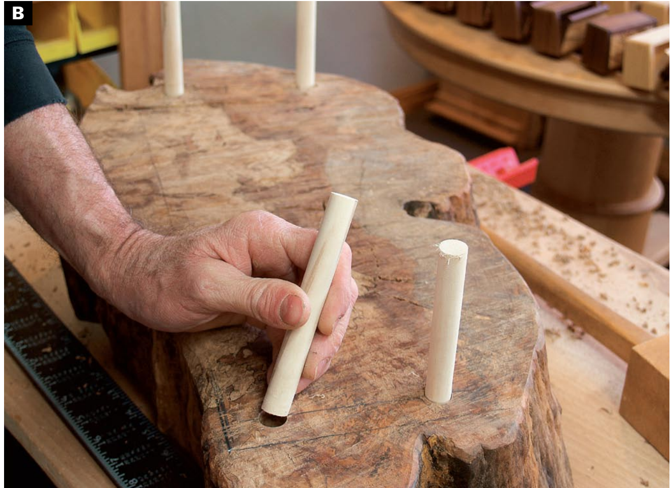
PLACE THE FRAME OVER THE STUMP to transfer the locations of the holes in the left and right stretchers so that the stump can be drilled for the dowels to fit.
