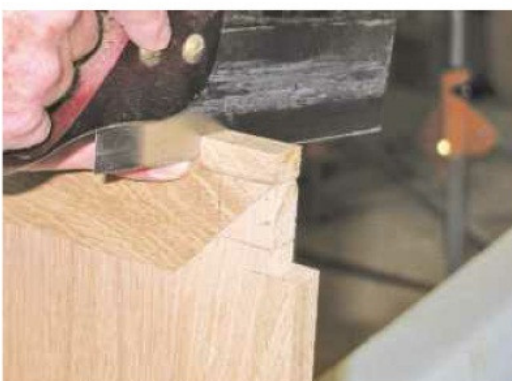
11 Use the template to mark out the shelf corner profiles and cut them by hand. Work with care
