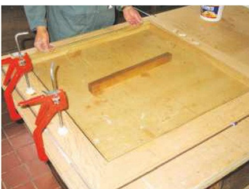
14 Mitre the corners, dry-assemble the frame and check that the glass fits in its rebate
