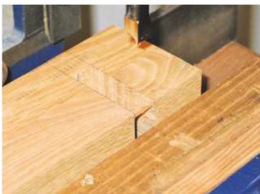
4 Use the mortiser to cut the slots for the shelf in the same way while the legs are still square
