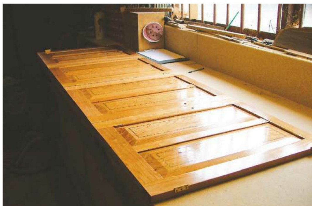
21 The resulting high-gloss finish needed de-nibbing and waxing to soften the glassy look
