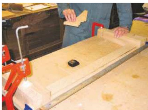
10 Dry-assemble one end of the table and cut a template from scrap wood for the shelf corner
