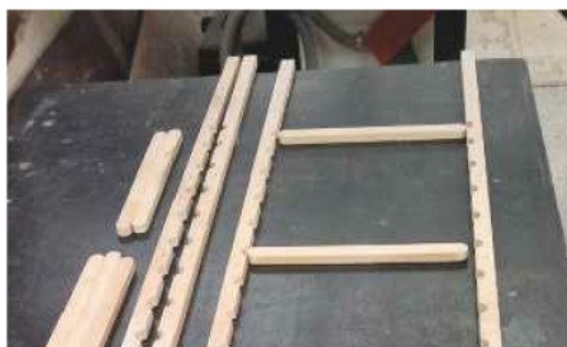
31 The finished set consists of four standards and ten cleats, ready for fitting into the carcass
