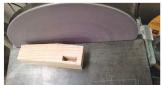
19 Remove the bandsaw marks from the tapers using a disc sander
