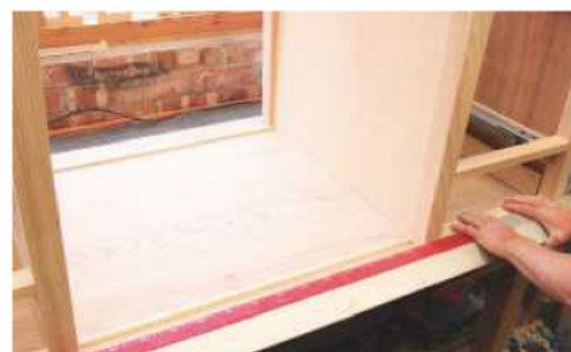
45 Place the desktop face down and carefully align the two pedestals on it
