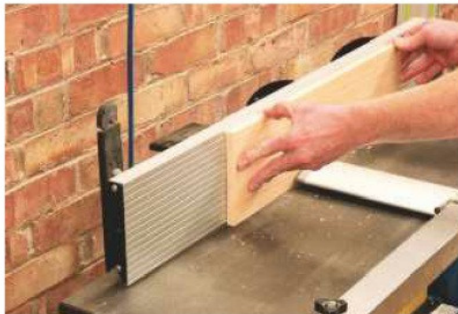
21 Make up the drawer box panels to the sizes in the cutting list
