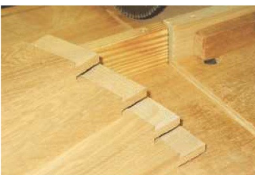
7 Cut the rail tenons using a pull-over crosscut saw or on the bandsaw
