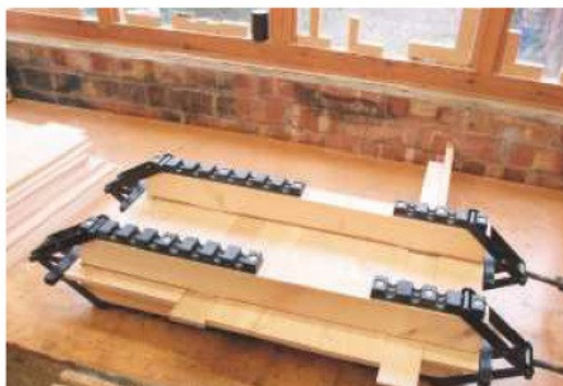
22 Assemble the larger panels by rub-jointing and cramping narrow boards
