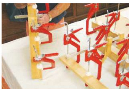
6 Each two-part leg assembly is glued, cramped up and checked for square
