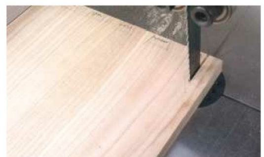
6 Make a cut-out in each front corner of the top and base panels to accept the face frame
