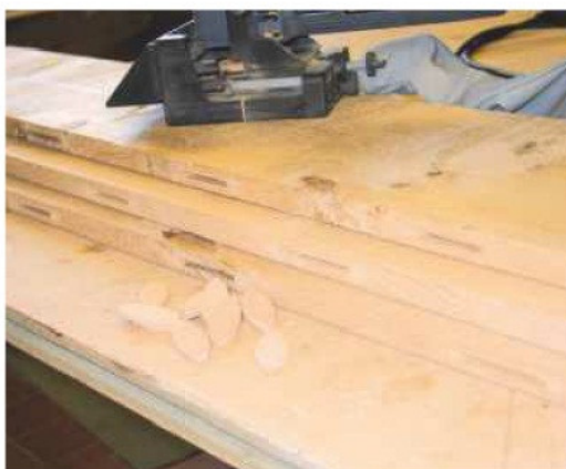
18 The planked top is jointed up from a number of pieces using biscuits
