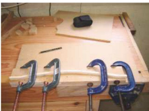
6 Make a former for the curved seat slats and assemble each one from four ash strips
