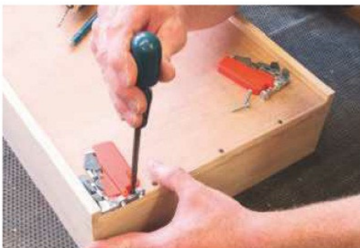
32 Screw the runner locking clips to the front edge of each drawer base
