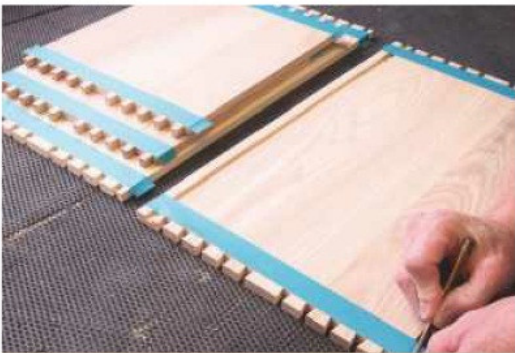
27 Low-tack masking tape allows easier clean-up of excess glue from the internal corners after assembly
