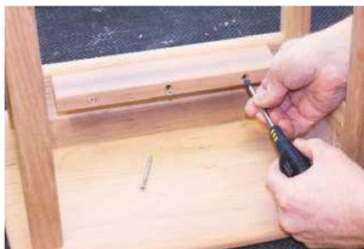
17 Prepare the spacer blocks and screw them to the rear rails of the top two tables
