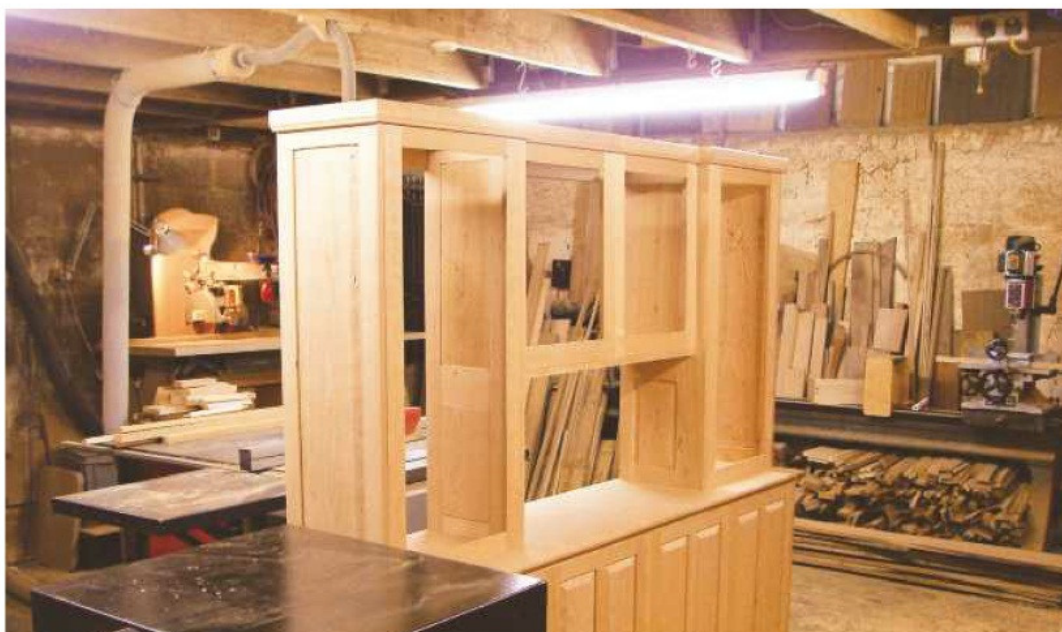
17 The upper and lower parts of the dresser can now be united and the top and bottom doors fitted
