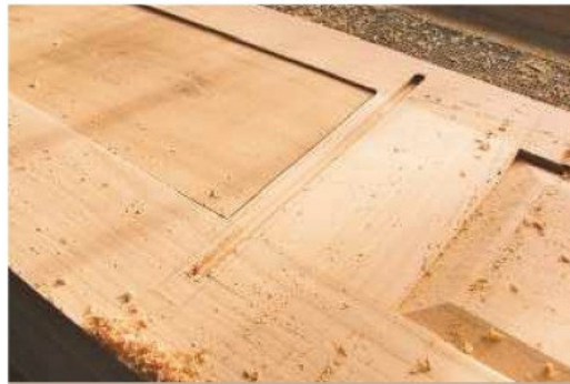
3 Stopped housings cut across the centre rails of the inner panels will receive the shelf ends
