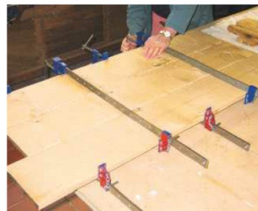
19 Rub the joints and cramp the top up from both sides to keep it flat
