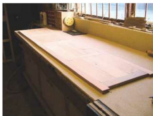
9 Make up the base panel and infill between the rails with tongued-and-grooved boards
