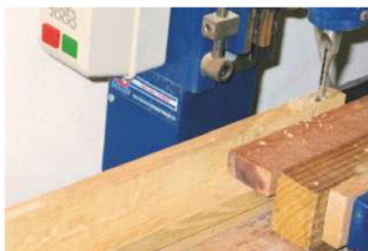
9 Position each leg on the mortiser so that the slots are cut in the same place
