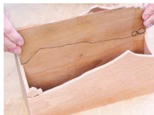
18 Cut the divider so it slides between the grooves. Saw the outline and sand it smooth
