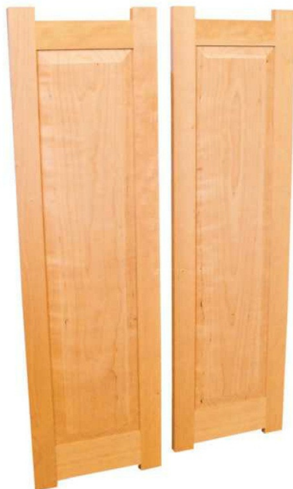
1 The end panels for the upper carcass
