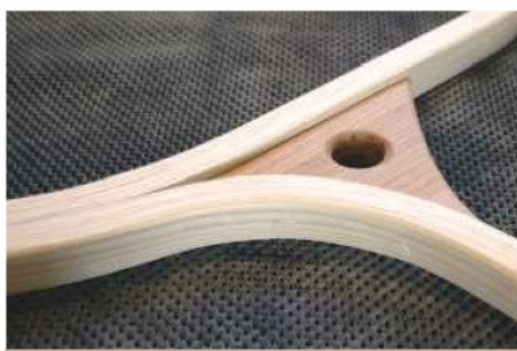
23 Fix the shaped and decorated brackets in place and cover any visible screw heads with ash plugs
