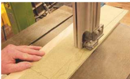
5 Cut the template shape on the bandsaw, working close to the pencil mark
