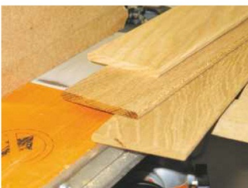
17 Machine both edges of an offcut to make the beading, then cut it to width
