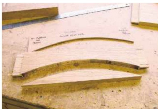
18 To speed up the repeat cutting, I made a rod for each chair rail pattern
