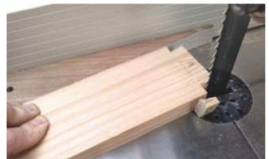
5 Cut the rail dovetails on the bandsaw against a 1:5 wedge held against the fence
