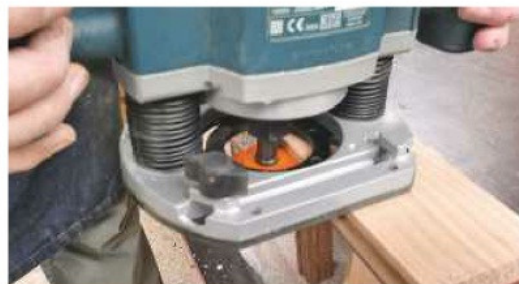
22 Rout a 6mm groove in the inside edges of all the back frame parts
