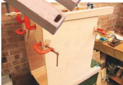
16 Assemble two rear legs and a back panel, then add in the two side panels
