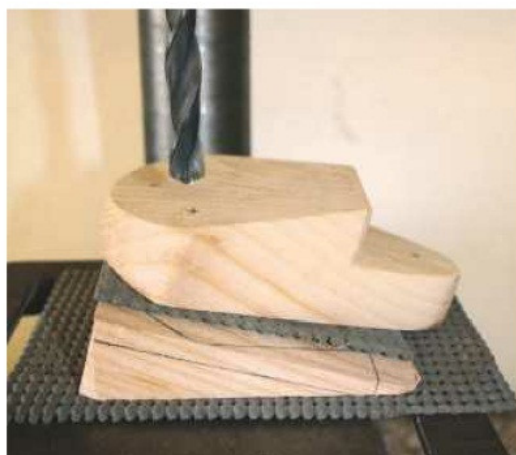
7 Drill the counterbores in the sockets first, then tackle the screw holes
