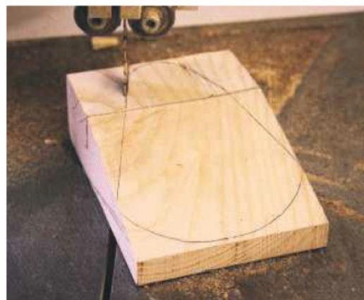
6 Cut the socket shape on the bandsaw, then cut the step by hand
