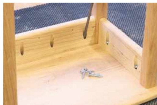
16 Align each frame on its tabletop and drive in the pocket hole screws to attach it
