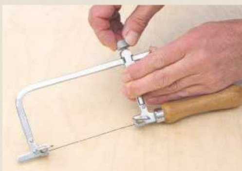
1 A piercing saw can be used for intricate shapes, though its blade cannot be rotated. This is secured with two thumbscrews. Slackening off the knurled thumb wheel on the frame releases tension and enables you to replace the blade
