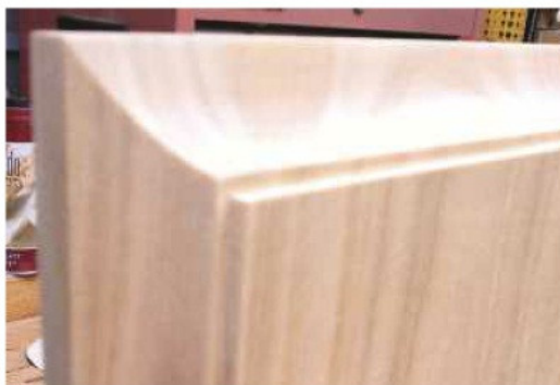
27 You can add a small rebate just below the cove to create a shadow line
