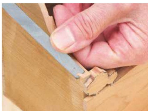
16 Use a sharp chisel to contour upper edges if they meet at slightly different heights
