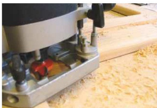
18 Round over the internal edges of the open frames with a bearing-guided cutter
