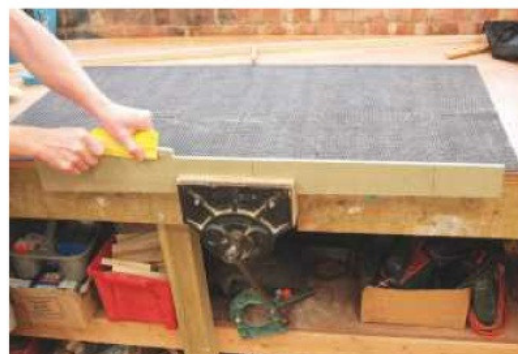
6 Sand the edge of the template by hand until it's smooth to the touch
