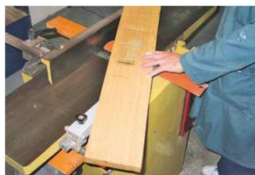
3 Any 'misses' that occur during surfacing can be removed during the thicknessing stage
