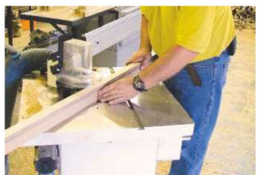
6 Most of the excess timber was removed in a single continuous movement
