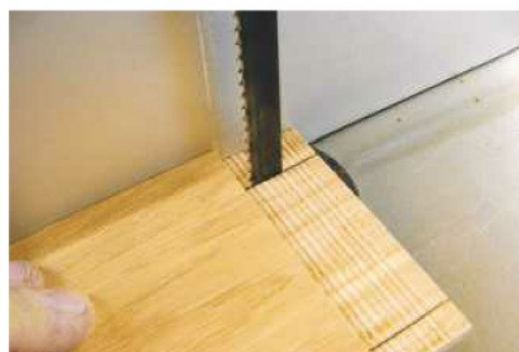
16 ...before cutting them down in width as required on the bandsaw
