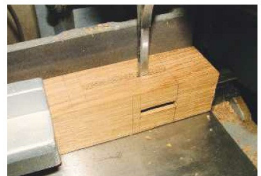
13 Cutting the mortises on the front legs was much more straightforward
