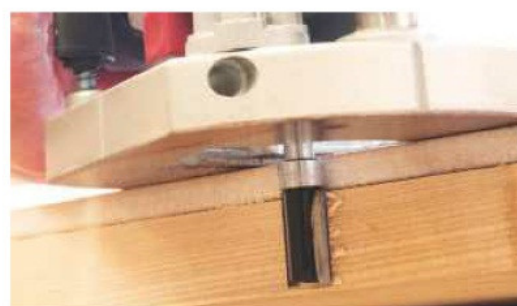
44 Reattach the template and trim the desktop precisely to size with a straight router cutter
