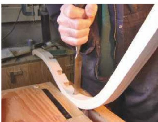
9 Then cut each socket accurately to size with a sharp chisel and a mallet
