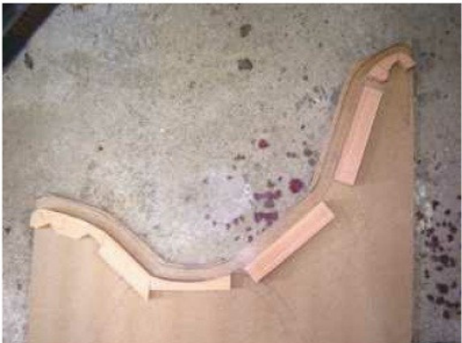
1 Draw out the frame profile on an MDF sheet and attach the former blocks for the seat frame
