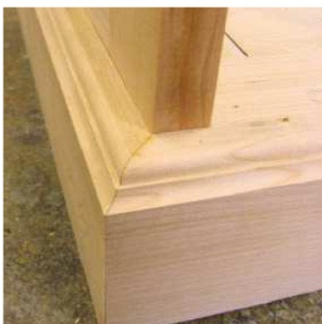
25 Glue and pin the corner mitres to make sure they can't open up over time
