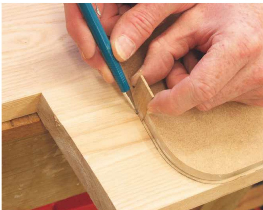
42 Draw around the template with a slim spacer to mark up the desktop
