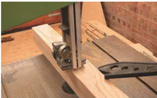
10 To save router time and cutter wear, rough-cut each leg to shape first
