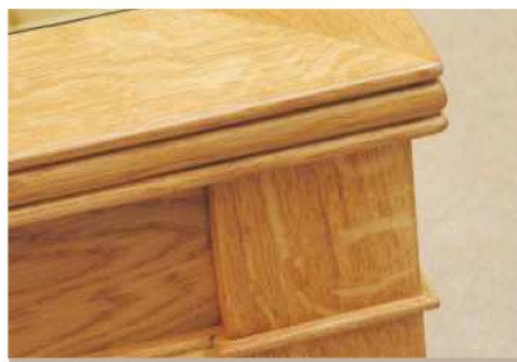
19 Clean up all the edges, apply sealer and wax, and drop the glass into place
