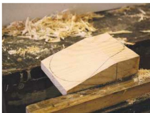
5 Use the template to mark out the curved shape of each socket
