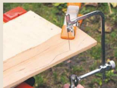
2 Fit a new blade so teeth are pointing down towards the handle. This keeps it under tension when sawing
