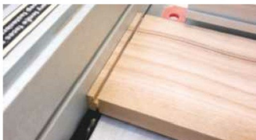
23 Cut stub tenons on the rails and muntins to fit into the grooves
