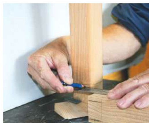
17 Use a pencil, block and straightedge to scribe each splayed leg, then cut it to length
