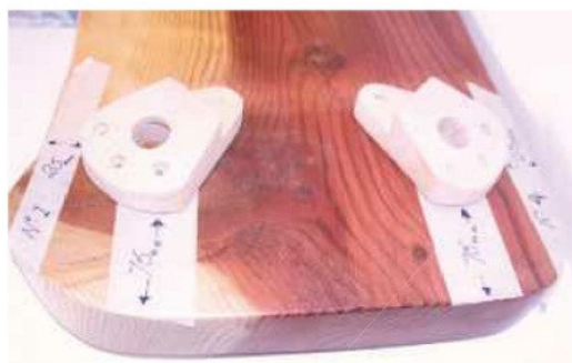
12 Position the sockets at the narrow end and take some measurements
