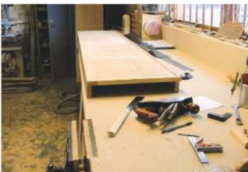
22 Attach two long and two short cleats to the underside of the base panel
