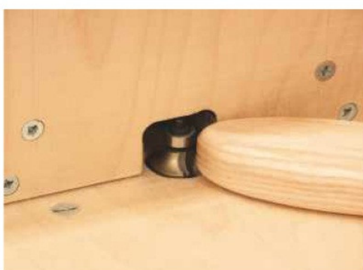
37 Round over both edges of the four handles on the router table
