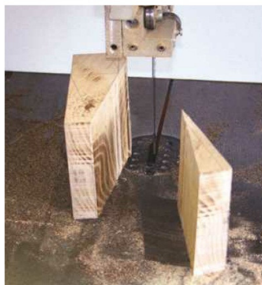
4 Mark out each socket and cut off the wedge on the bandsaw
