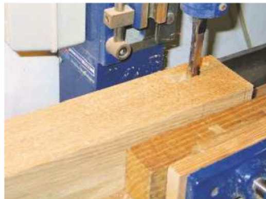
3 Using a bench mortiser is the quickest way of chopping out all the leg mortises
