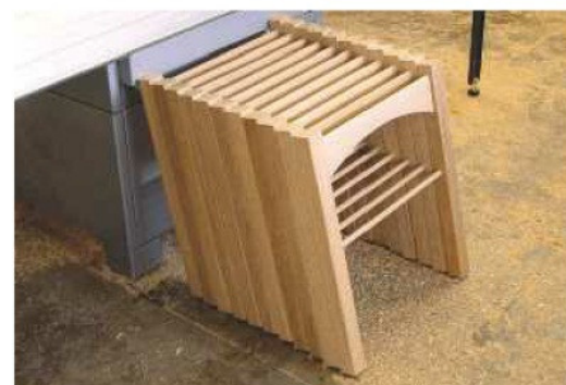
21 The first stage of the assembly was to make up all the front frames
