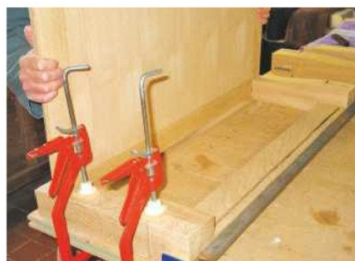
12 Test the fit of the shelf corners in the leg slots, and ease them if they're too tight for easy assembly
