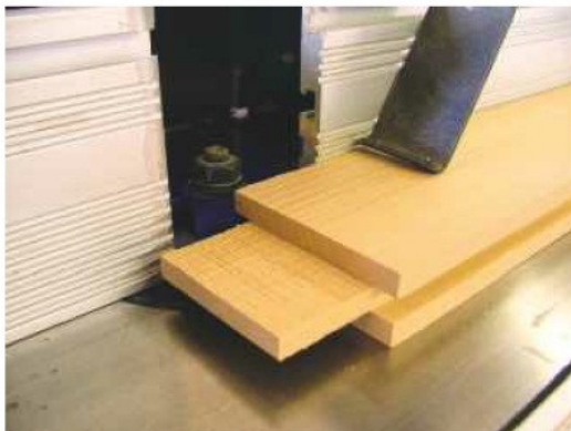
4 Cut grooves for the panels into the stiles and rails using a slotting cutter
