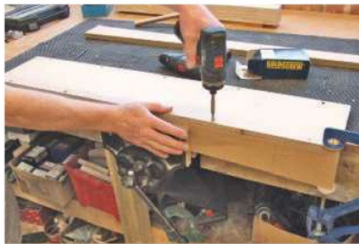
8 Screw the jig sides to the base. Note that the template is 50mm longer than the sides
