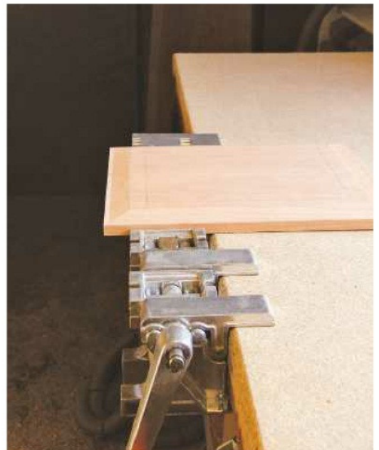
6 ...as the jaws grip their edges but don't impede access to the panel surface
