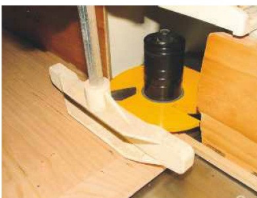
10 I fielded the panels on my spindle moulder, taking a succession of thin cuts
