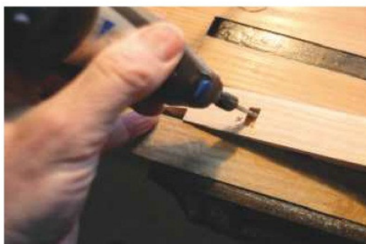
17 I resorted to using a Dremel multitool to cut the front seat frame mortises
