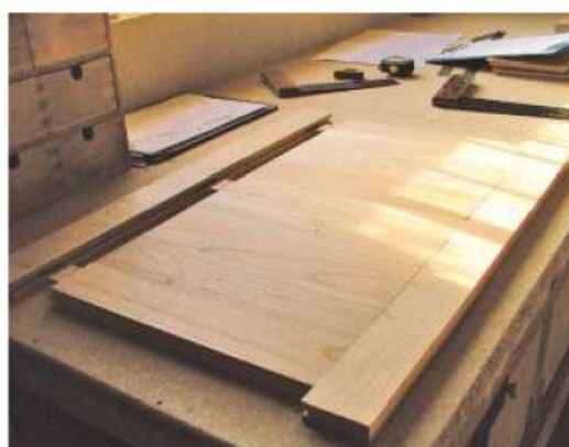
14 Make up the central divider with two stiles, three rails and tongued-and-grooved board infills
