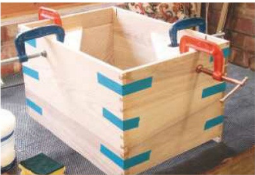
28 Tape and right-angled corner webs help to hold the assembly square
