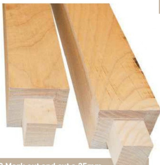
9 Mark out and cut a 25mm square stub on the end of each leg
