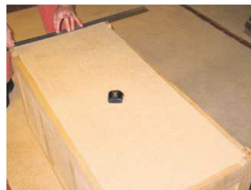
16 Mark the dimensions of the base panel from underneath and cut it to size
