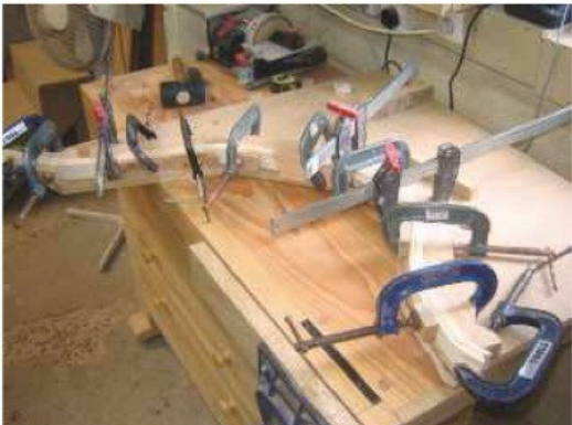
2 Make up each seat frame by gluing and cramping six ash strips to the former
