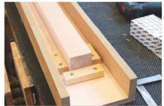
9 Screw small wooden blocks to the base of the jig to locate the leg ready for routing
