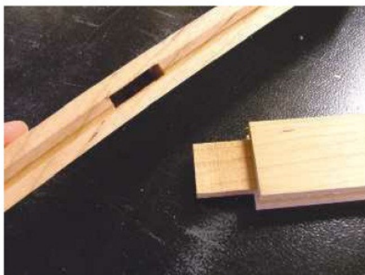
7 The slimmer components forming the door muntins don't need haunched tenons
