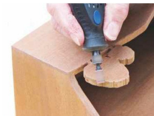
17 Soften the sawn outlines using a multi-tool fitted with a fine-grit sanding drum
