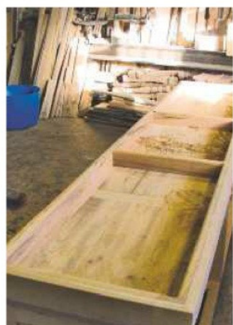
24 Turn the carcass over so you can attach the mitred plinth mouldings to the cleats
