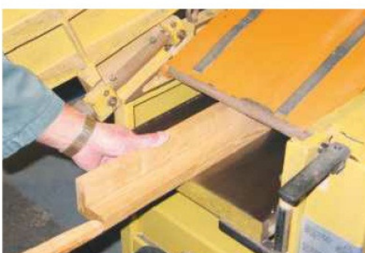
7 Plane the oversize legs to their finished size and then cut them to length
