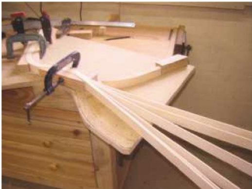
4 Reposition the former blocks and make up the two leg frames in the same way
