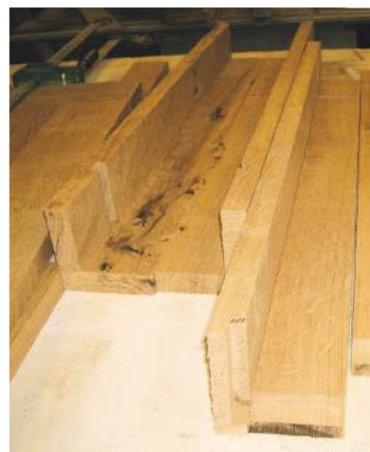
5 The legs were glued up using biscuit joints to reinforce the long edge joints
