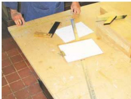
1 Drawing a rod – a full-size top view of the table – on a large board offcut is a useful technique to adopt
