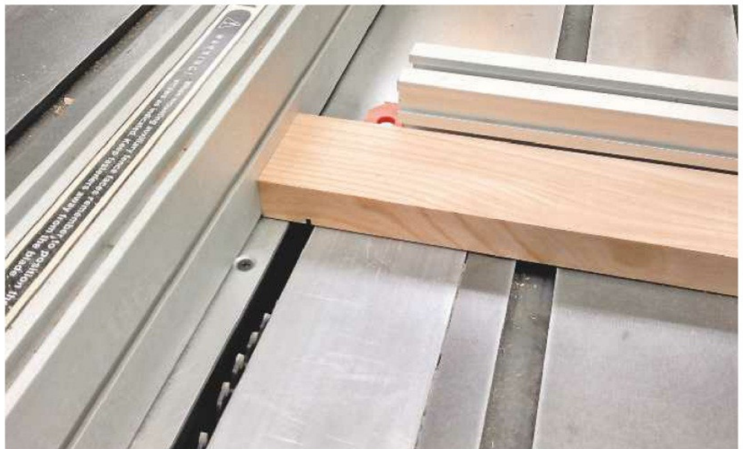
16 Cut the tenon shoulders on the table saw; note that they're offset
