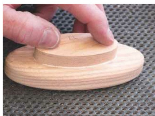
38 Glue a spacer to each handle, taking care to centre it accurately
