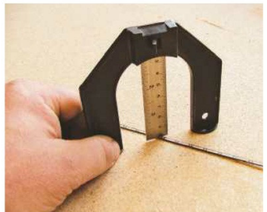
7 I use my Trend depth gauge to measure the thickness of the inlay...
