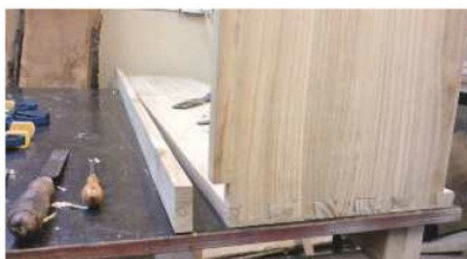
11 The uprights that will form the face frame fit into the notches cut in step 6
