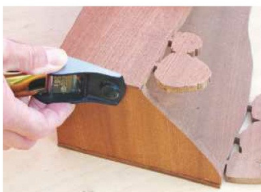
14 When the glue has dried, carefully trim the excess end grain on the corner joints
