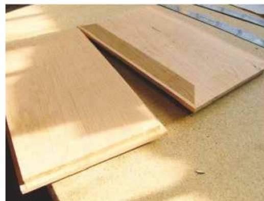
11 Form a rebate on the back of each panel to create a tongue all round
