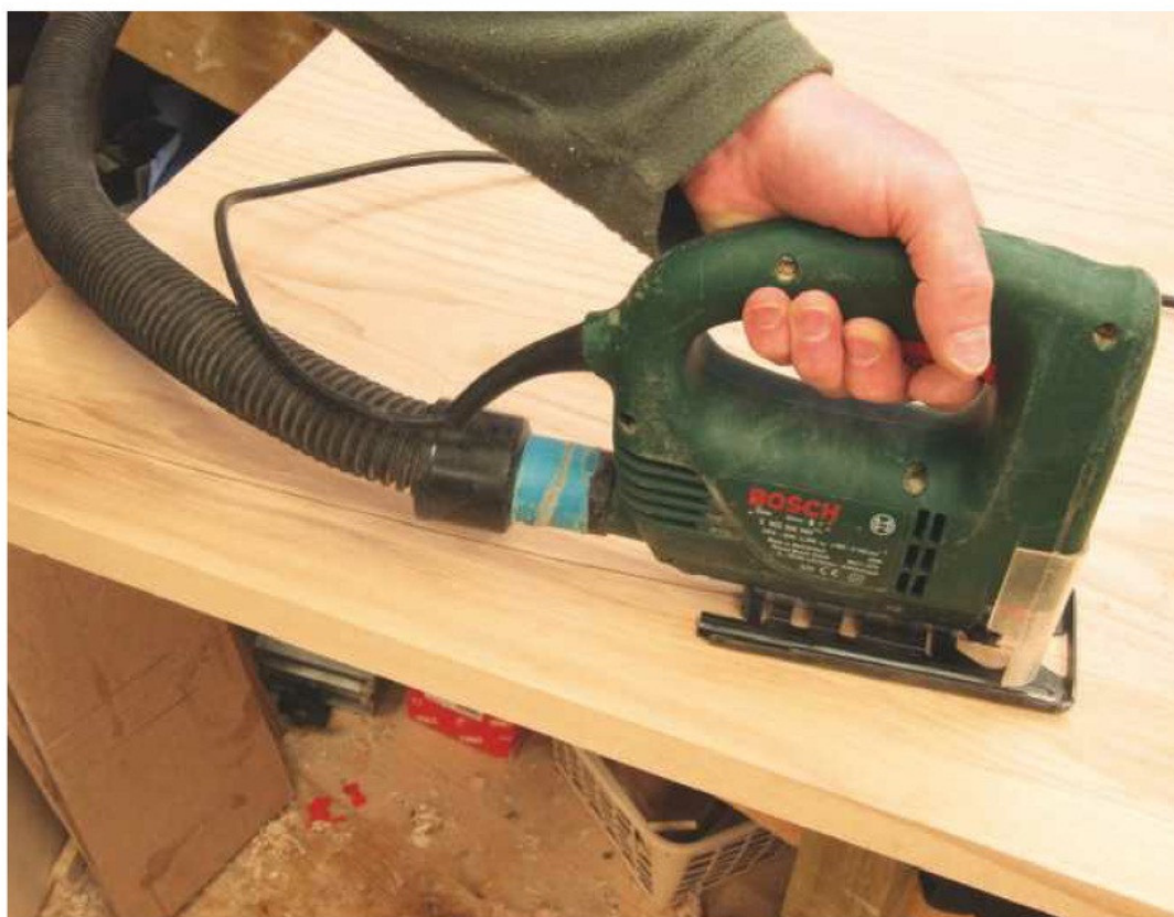
43 Cut the desktop roughly to shape, following the oversize marked line
