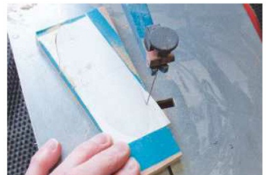
35 Cut an MDF template for the oval handle shape using the scroll saw
