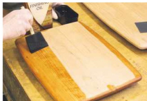
19 Apply finishing oil with a foam brush, sanding down lightly between coats. Then wax it
