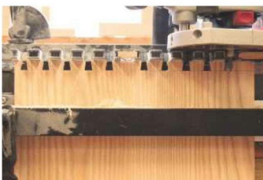
24 Cut the side panel tails first, followed by the end panel pins
