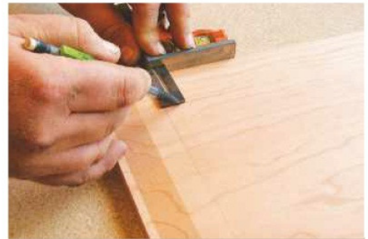
4 Mark the position of the inlay on the various raised panels with a fine pencil line
