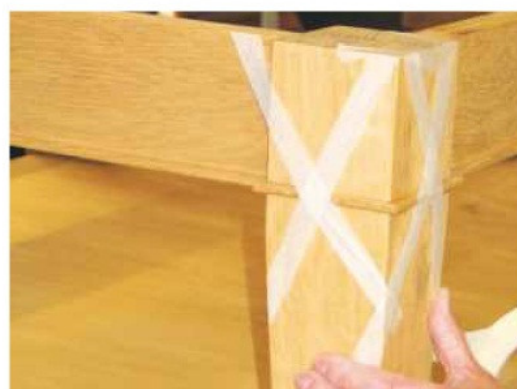
18 Glue the leg beads into their grooves and secure them with tape
