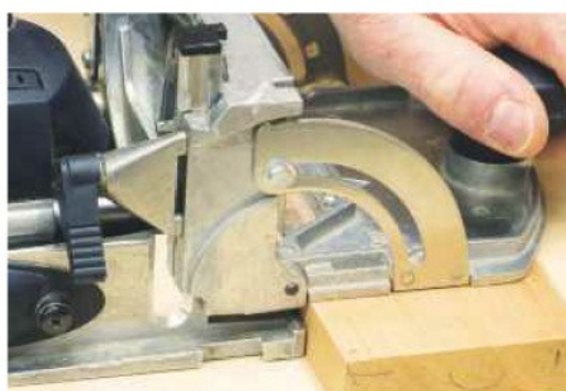
10 Fit biscuits in the board edges to help align the joints during the glue-up
