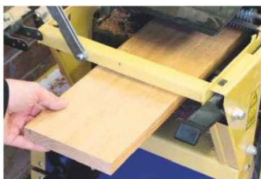
9 Thickness to 20mm the cherry boards that will make up the three tabletops
