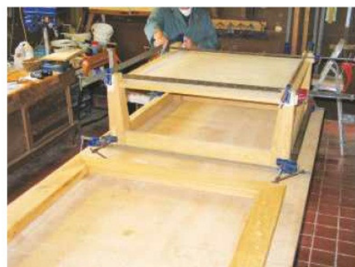
15 Assemble the sub-frame upside down. The table's top frame is shown in the foreground
