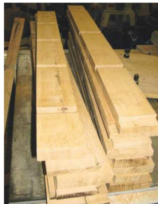
4 The modular design means you can save time by machining batches of parts like these shelf housings in the legs
