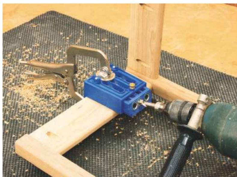
8 I decided to attach the tops with pocket hole screws, and drilled holes in the top rails
