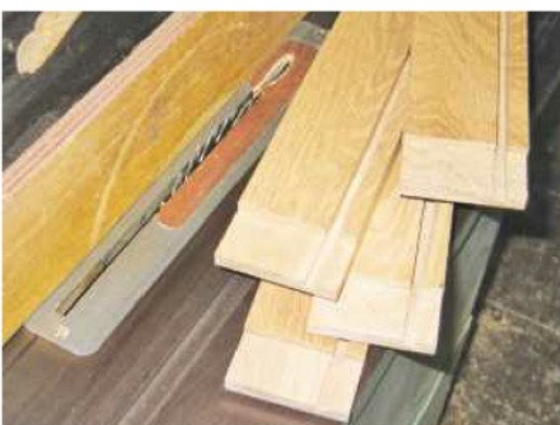
8 Machine a groove on the inner face of each rail to receive the top buttons
