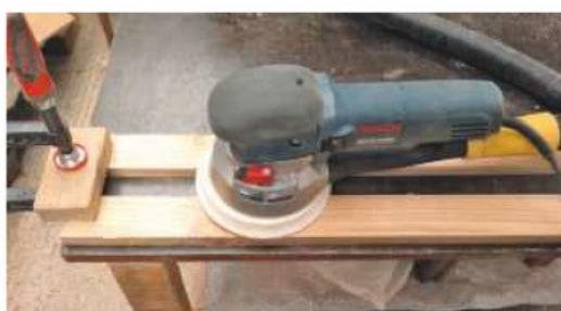
12 To avoid rounding over their edges, sand them while cramped together as shown
