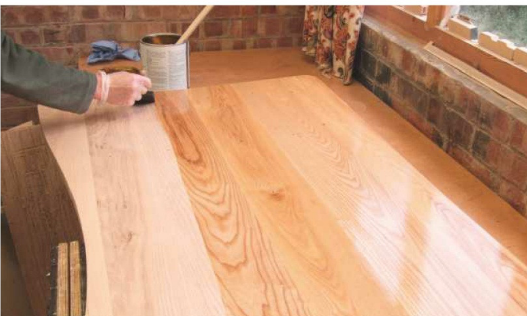
48 Apply hardwax oil and then liquid wax to the various components
