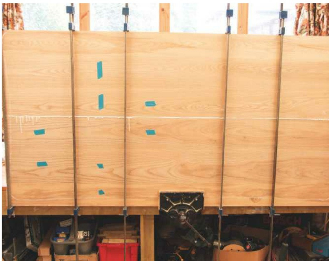
39 Glue up and cramp the boards you've selected to form the desktop
