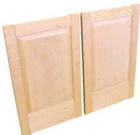
12 Dry-assemble the two end panels and check their overall dimensions
