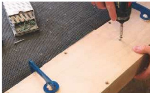
11 Cramp the rough-cut leg in the jig and secure it with two screws
