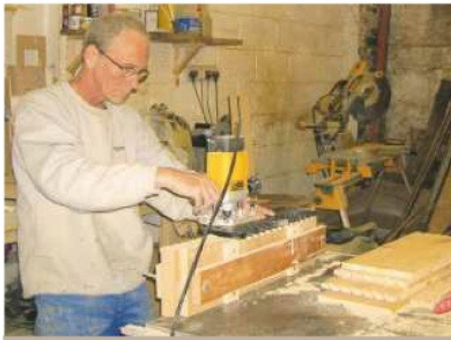
11 The drawer box was made by thickening some of the remaindered oak to \frac{1}{2} in and the sides and front were joined with dovetails cut on a jig
