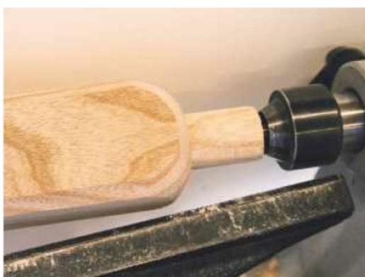
10 Turn the stub to a spigot and create a rounded chamfer on the leg as shown
