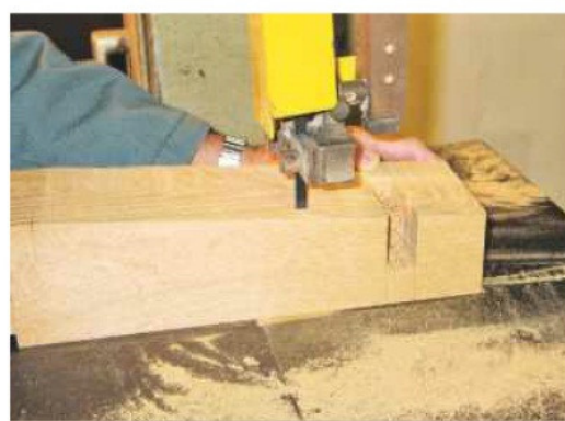
6 Cut the leg taper roughly to shape on the bandsaw, working just outside the marked line
