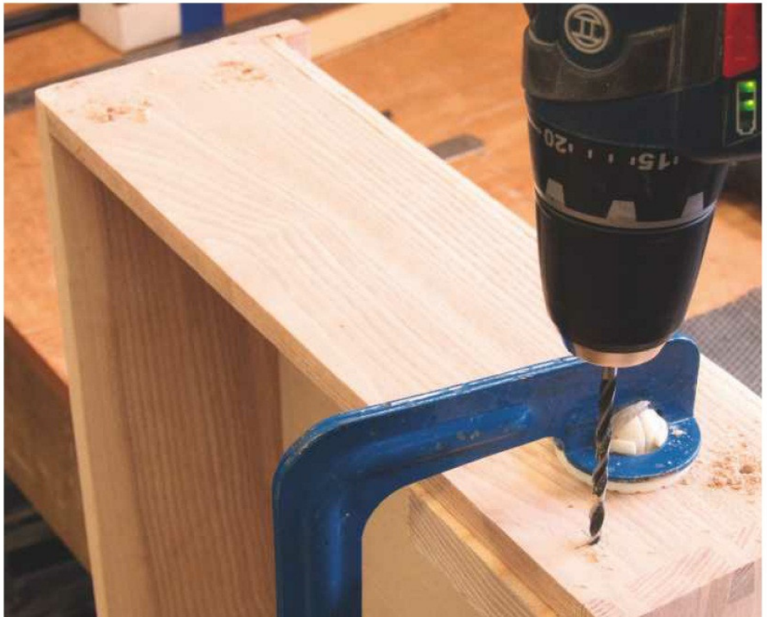
33 Drill four screw clearance holes in the front end of each drawer box
