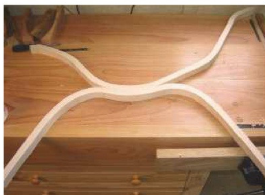
5 Release the completed leg frames from the former and test their fit against the seat frames
