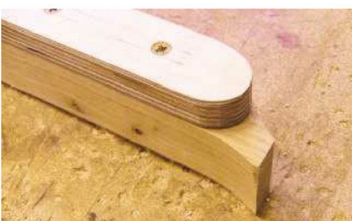
7 To avoid breakout, the top end of each leg was cut by hand and then sanded to shape
