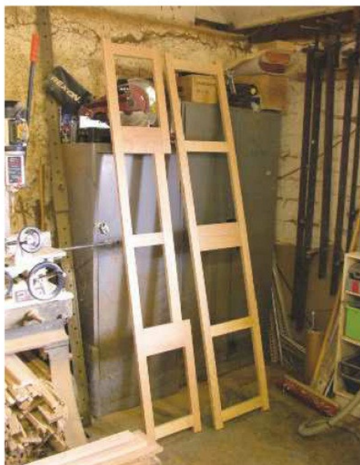
8 Make up the top frame. The one for the upper cabinet is also shown here
