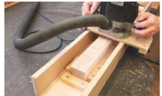
12 Shape each leg by making a series of shallow cuts with the router
