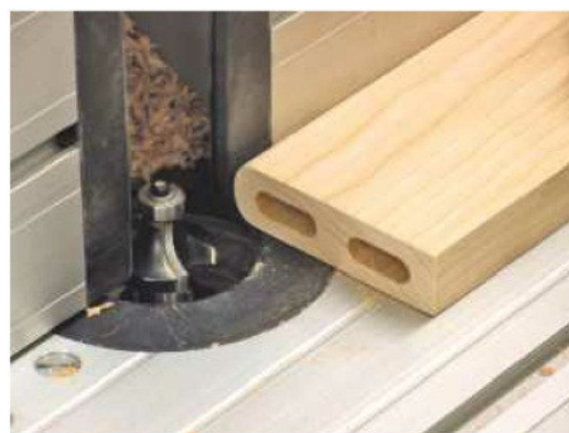
5 Use the same cutter to soften the exposed edges on the upper and lower rails
