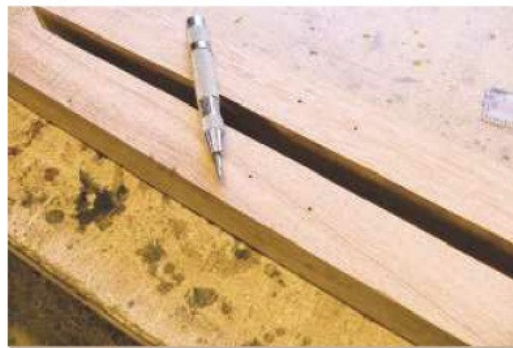
10 I marked and centre-punched the positions of all the holes for the lower side rail dowels
