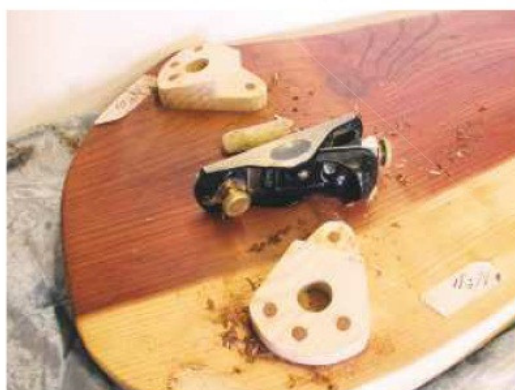
14 Conceal the screw heads by gluing contrasting wooden plugs into all the counterbores
