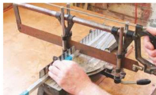
47 Cut the aluminium hanger rails to length with a fine-toothed saw and file their ends smooth
