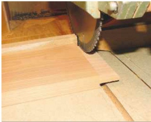
2 Create the tenons by making a series of parallel cuts on the radial arm saw
