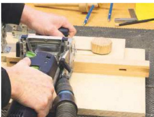
3 Cut the mortises in the legs. I'm planning to use loose tenons (Dominos) here
