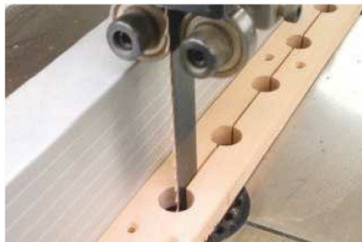
29 Drill 25mm holes down the centre line and saw the standard in half
