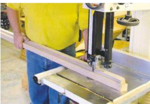
3 After screwing the rod to each blank, I removed the excess timber on the bandsaw
