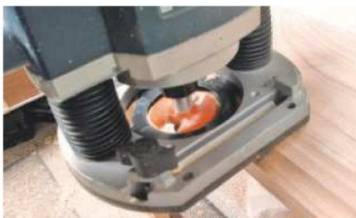
26 Cut the top panel to size and rout a cove moulding on its edges
