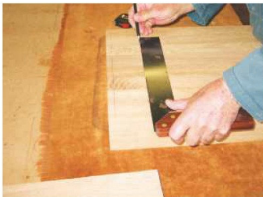
2 Mark out the leg mortise holes on all four components in one go for complete accuracy
