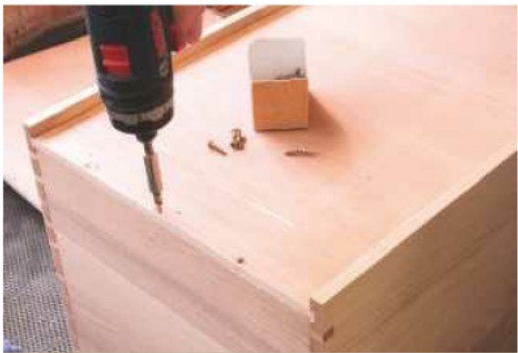
29 Glue each drawer base in place and screw the front and rear edges
