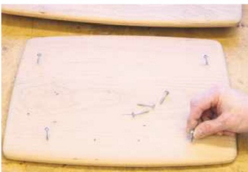
18 Remove the top for finishing and fit four screws as shown to act as temporary supports
