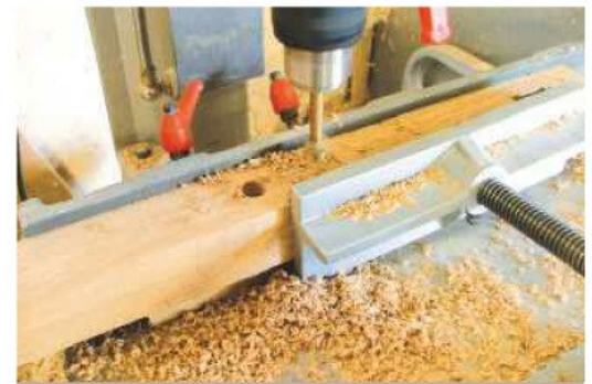
11 The holes were drilled precisely in line using a Jacobs chuck in my bench mortiser
