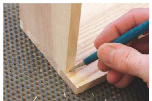
26 Dry-assemble each box to test its fit, then mark the base position
