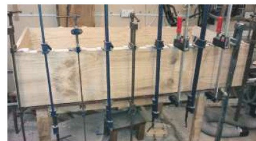
14 Use biscuits for alignment as you glue and cramp the face frame on
