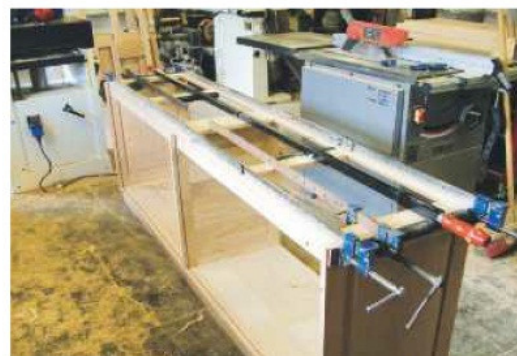
23 Assemble the base panel, the top frame, the end panels and the central divider
