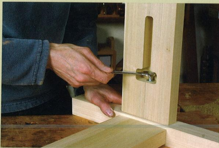
HIDDEN BOLT. Use a jig to rout a T-shaped slot inside the side rails (above). Then insert the bolt and tighten it into the nut embedded in the head or foot rail (left).
