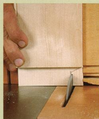
TRIM TENONS TO SIZE AND SHAPE. A matching template made to the negative shape of the one used to check mortises shows where to cut the angled haunch on the tenons. The first cut is made with a stop block on the miter gauge.
