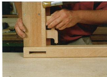
BRACKET ALIGNMENT IS TRICKY. The author locates a dowel hole on his table by sliding the bracket along a guide board clamped to the apron and marking with a dowel center.
