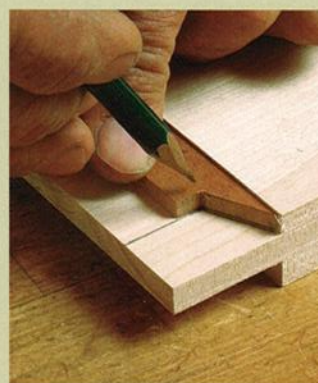
TRIM TENONS TO SIZE AND SHAPE. A matching template made to the negative shape of the one used to check mortises shows where to cut the angled haunch on the tenons. The first cut is made with a stop block on the miter gauge.
