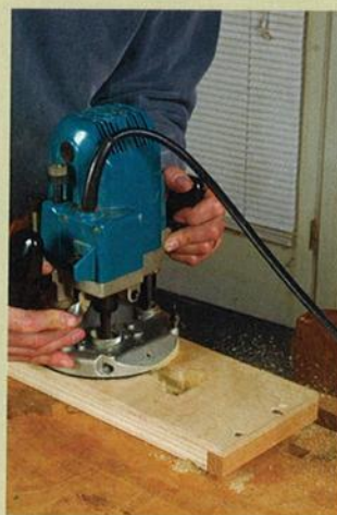
HIDDEN BOLT. Use a jig to rout a T-shaped slot inside the side rails (above). Then insert the bolt and tighten it into the nut embedded in the head or foot rail (left).
