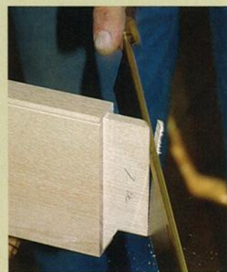
THIS HANDWORK IS FAST AND ACCURATE ENOUGH. A dovetail saw makes quick work of trimming the angled haunch and mitering the ends of the tenons.
