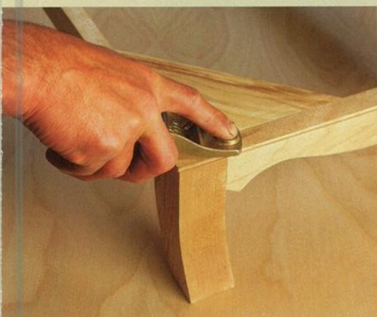
BACK FOOT MEETS THE FRAME. Saber feet are often linked with rails to create a strong frame that's screwed to the bottom of the chest. The foot is trimmed flush to the frame with a block plane.
