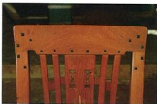
EBONY SUBSTITUTE. To substitute for ebony, the author used Ebon-X (chemically altered walnut) for black details.
