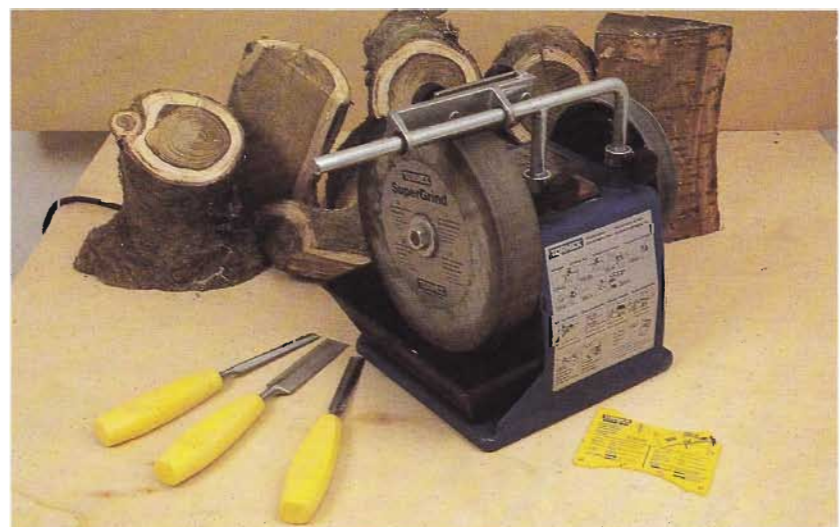
FIG 1.13 The Tormek sharpening system.
