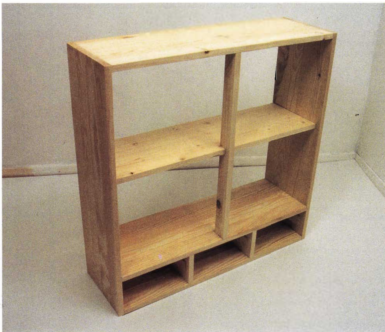
FIG 8.5 The carcass before the back is fitted.
