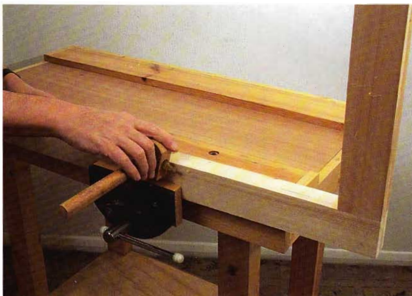
FIG 14.5 Marking the position of the inner frame with a marking gauge.
