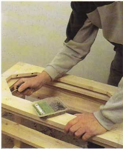
FIG 9.9 Fitting the corner braces.
