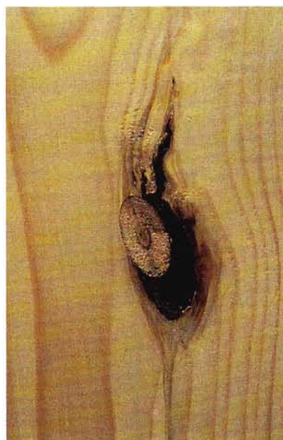
FIG 2.2 Undesirable: a dead knot, partially removed from its hole.
