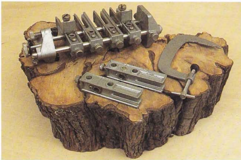
FIG 1.11 The Record dowelling jig.
