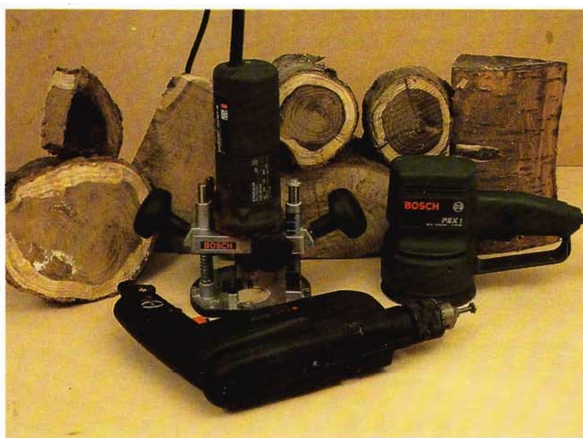
FIG 1.1 A \frac{3}{8} in (10mm) portable drill, random orbital sander, and \frac{1}{4} in (6mm) router.
