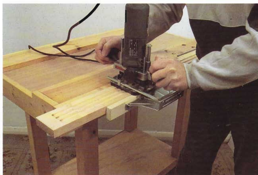
FIG 10.3 Cutting the flutes with a router.
