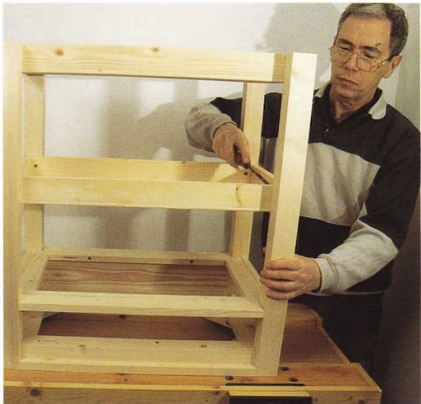
FIG 9.11 Fitting one of the slatted shelves.
