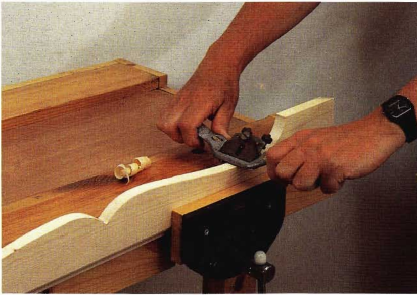
FIG 12.11 Smooth the decorative curves after they have been sawn to shape.
