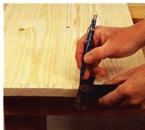
FIG 13.4 Marking the slope of the tails with a sliding bevel.
