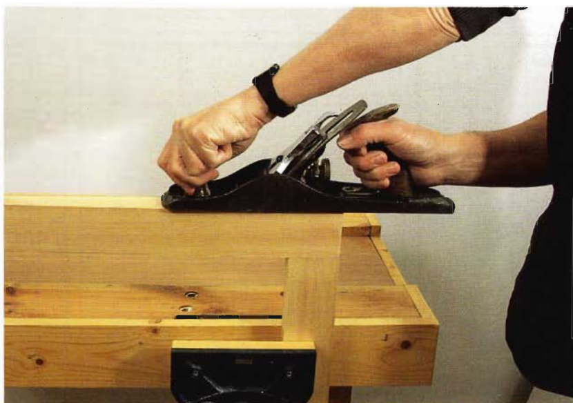
FIG 14.4 Cleaning up a corner bridle joint.
