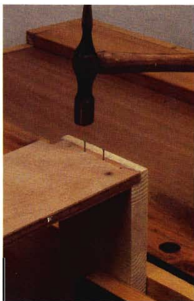
FIG 8.7 Pinning the sides of the drawer to the front.
