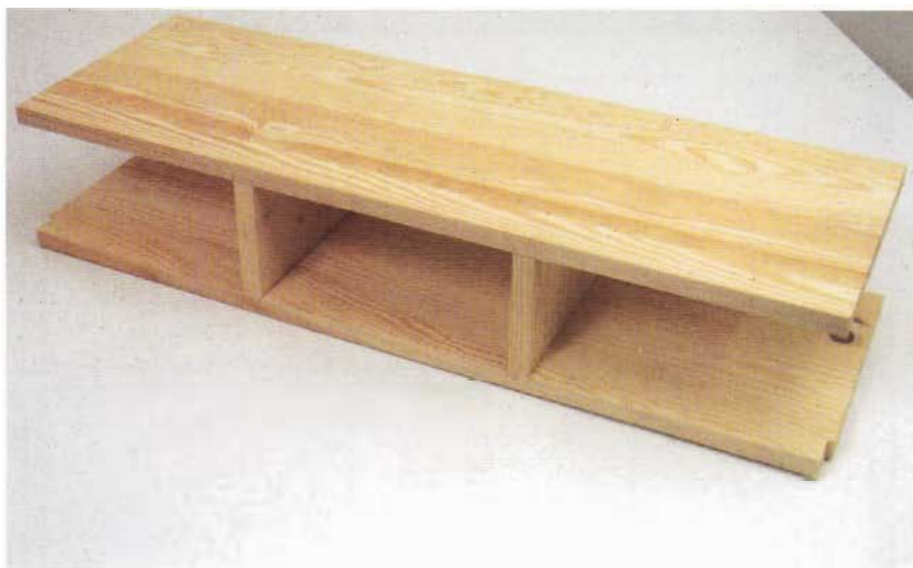
FIG 8.4 The assembly that houses the drawers.
