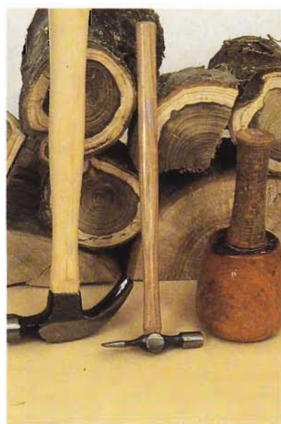
FIG 1.10 A medium-weight claw hammer, pin hammer and mallet.
