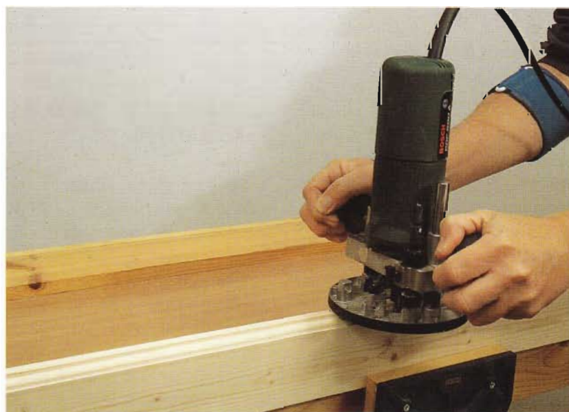
FIG 13.8 Cutting the decorative moulding on the plinth.
