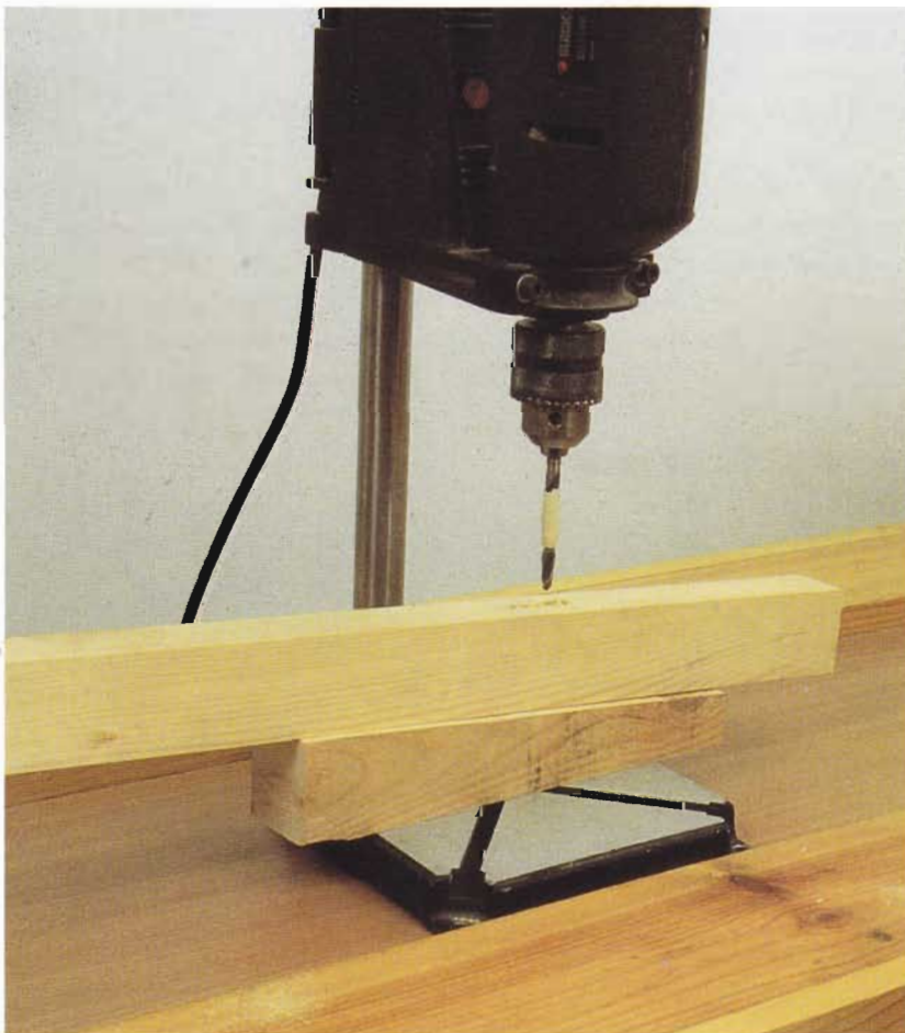
FIG 6.8 Drilling a sloping hole with a jig.
