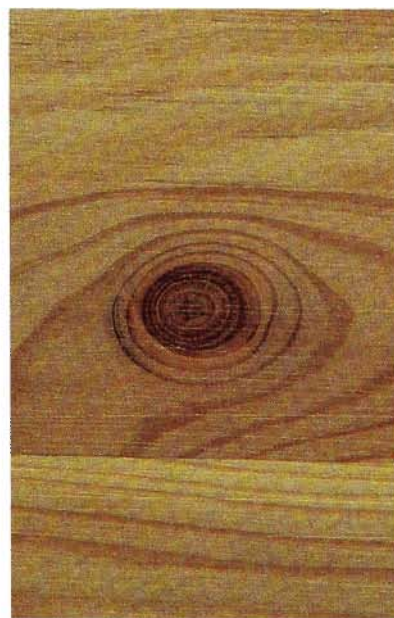
FIG 2.3 Desirable: a light-coloured, uncracked knot.
