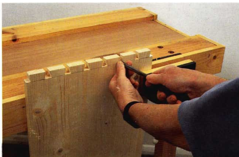
FIG 13.4 Marking the slope of the tails with a sliding bevel.
