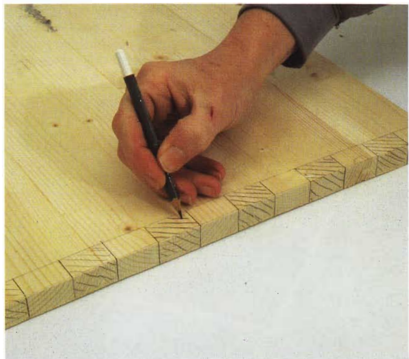
FIG 16.3 Marking the areas of waste wood to be cut away.
