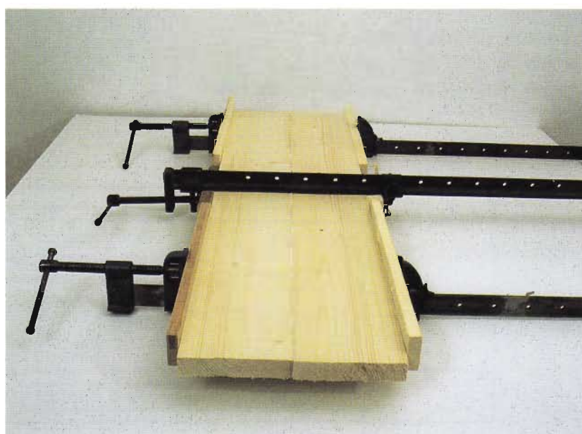
FIG 7.17 The centre section of the top, clamped together.
