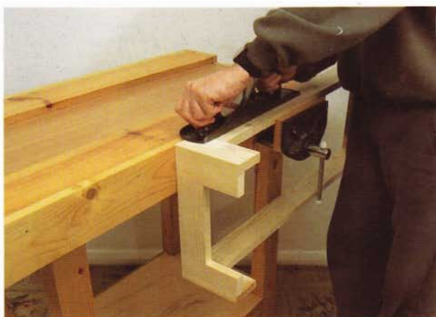
FIG 17.4 Cleaning up the outside of the outer frame.
