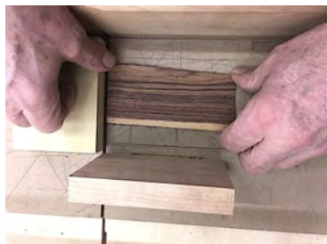
5. Squared-off veneer pushed up to the rabbet in block # 2 before cutting off.
