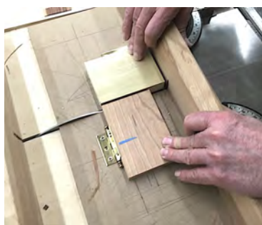
6. Cut off crossbanding section: both hinged blocks are down to support the veneer. Note: both blocks are zero-clearance. They were each cut by the blade after they were screwed in place.
