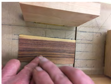
2. Position the veneer so grain lines are parallel to guide lines.
