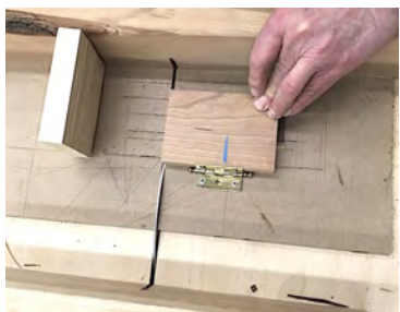
3. Square one end, holding down veneer with hinged block.
