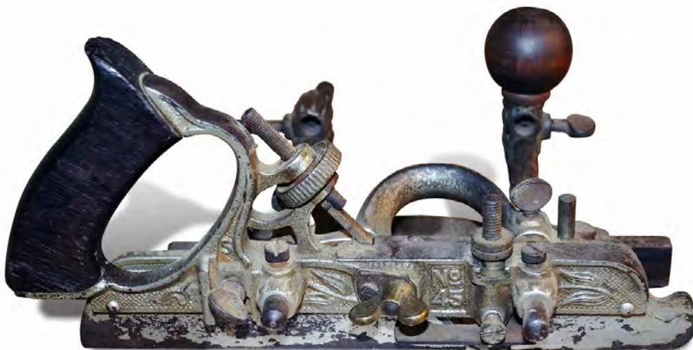
Figure 3. Stanley #45 set up to cut a bead
