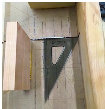
1. Guidelines on sled—perpendicular to the blade.
