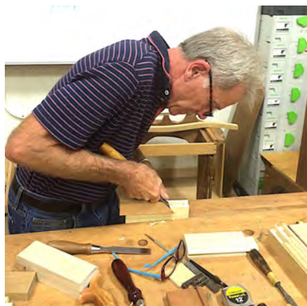
Steve demonstrates the cope-and-stick joinery method.
