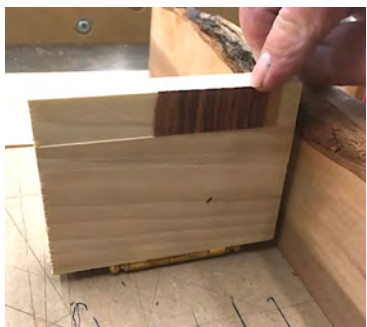
4. Second hinged block has a shallow rabbet (less than the thickness of the veneer), which determines the length of each piece when cut.
