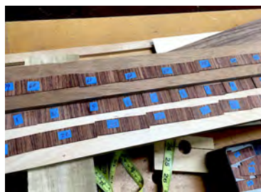
8. Numbered and jointed sections (all 90 of them!) ready to install.
