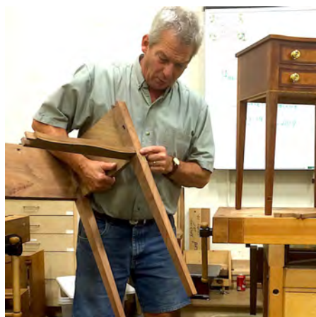
Jeff shows where dovetails and mortise and tenon are used on construction of this serpentine table.
