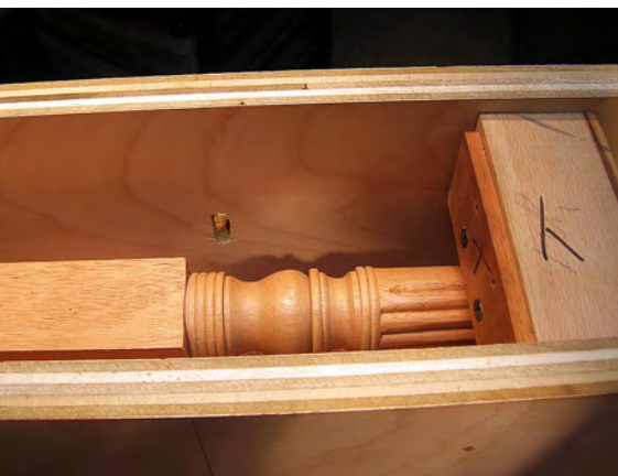
Leg in reeding box with cutter block
