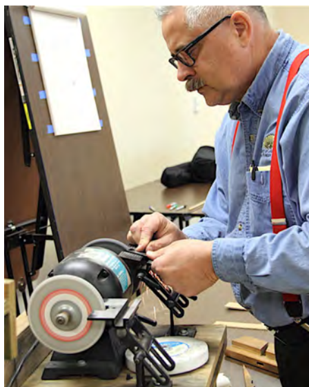
Tod Herrli demonstrating grinding a molding plane iron
