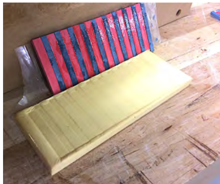
The glue-up showing the foam pad used to accommodate the differing thicknesses
