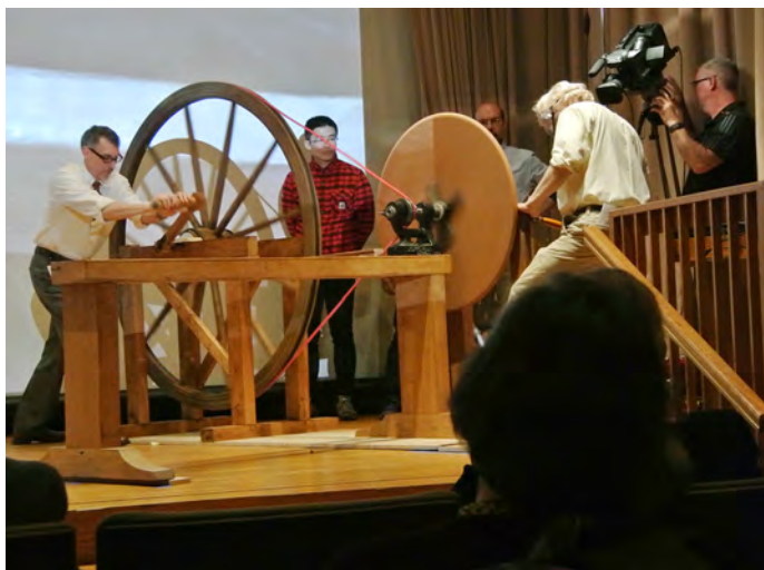
Joshua Lane powering the Winterthur lathe while Greg Landrey turns the table top. (Photo courtesy of Dale Ausherman)
