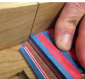
...then cut in miter box to correct dimensions
