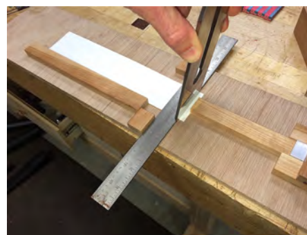
Jig to cut interspersed white vertical pieces
