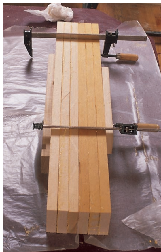
STEP 9 | Spread the clamping pressure evenly by using several clamps. Gluing two legs at once saves time and clamps. Be sure not to glue the two legs to each other.
