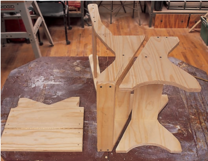
STEP 11 | Assemble the chair using glue and screws.
