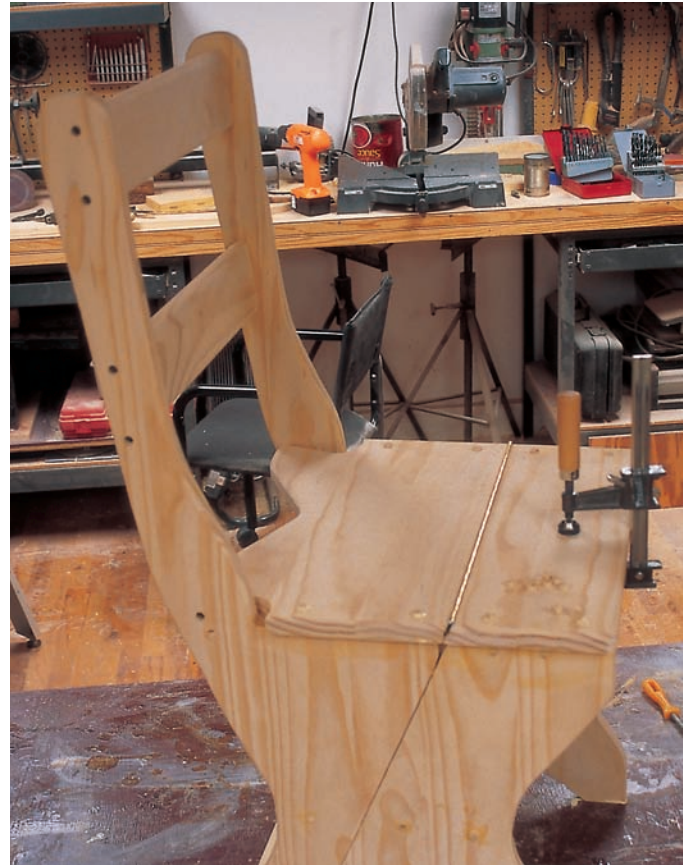
STEP 12 | After cutting the seat to shape, separate the front and back parts. Then attach the continuous hinge to the parts. The bevels on the hinged edges of the seat should match the angle of the front and back parts of the chair sides. Finally, attach the seat to the chair, using glue and screws. Plug all the screws holes on the chair and sand them flush.
