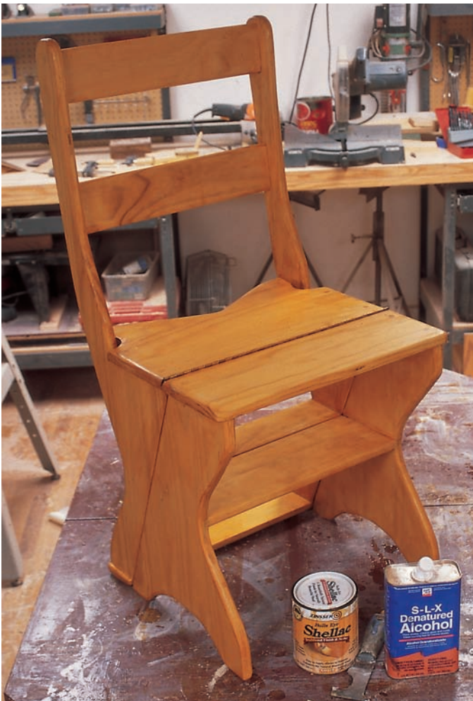
STEP 13 | Finish the chair how you like. I used three coats of shellac.
