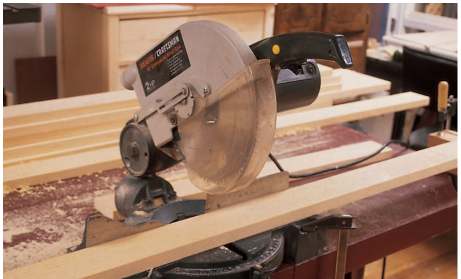
STEP 6 | Cut the leg lumber to length.
