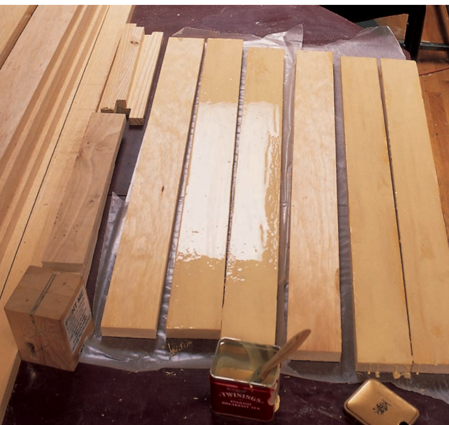
STEP 8 | Spread the glue evenly on the leg stock. Don't use too much glue, as it will ooze out, the parts will slide around, and you'll need to increase the clamping pressure to force the excess glue out of the joint.
