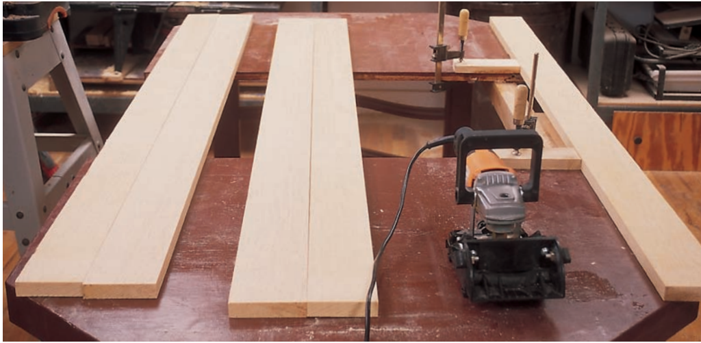
STEP 4 | Use biscuits and glue to strengthen the top.
