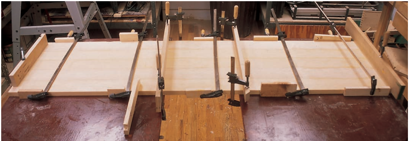
STEP 5 | Glue up the top. Clamping the top to the work surface will help hold the top flat.
