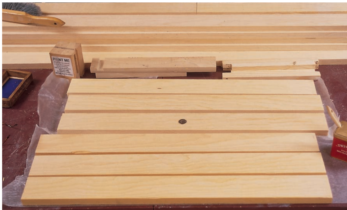
STEP 7 | Three pieces of leg lumber are glued together to make a leg blank.
