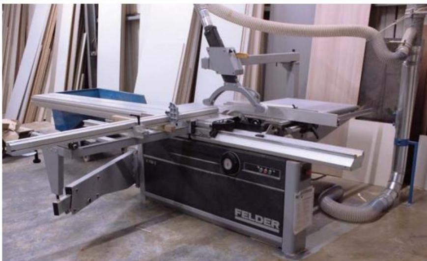
The K700S sliding table saw installed at Kings Oak
