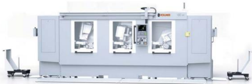
The VOLLMER CC355 production system machines carbide-tipped saws in a single working cycle using three machining stations
