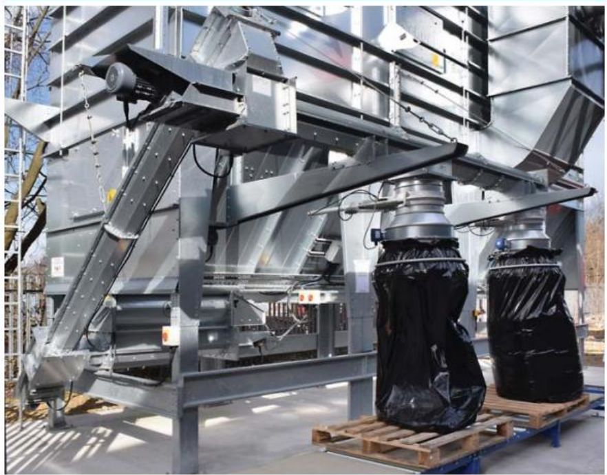
Waste is discharged pressure-free, via a rotary valve, and then transferred to collection bags by a series of 3 screw conveyors.
