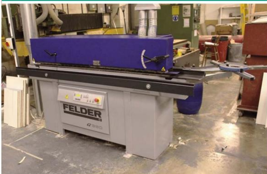
The G360 Edgebander installed at Kings Oak
