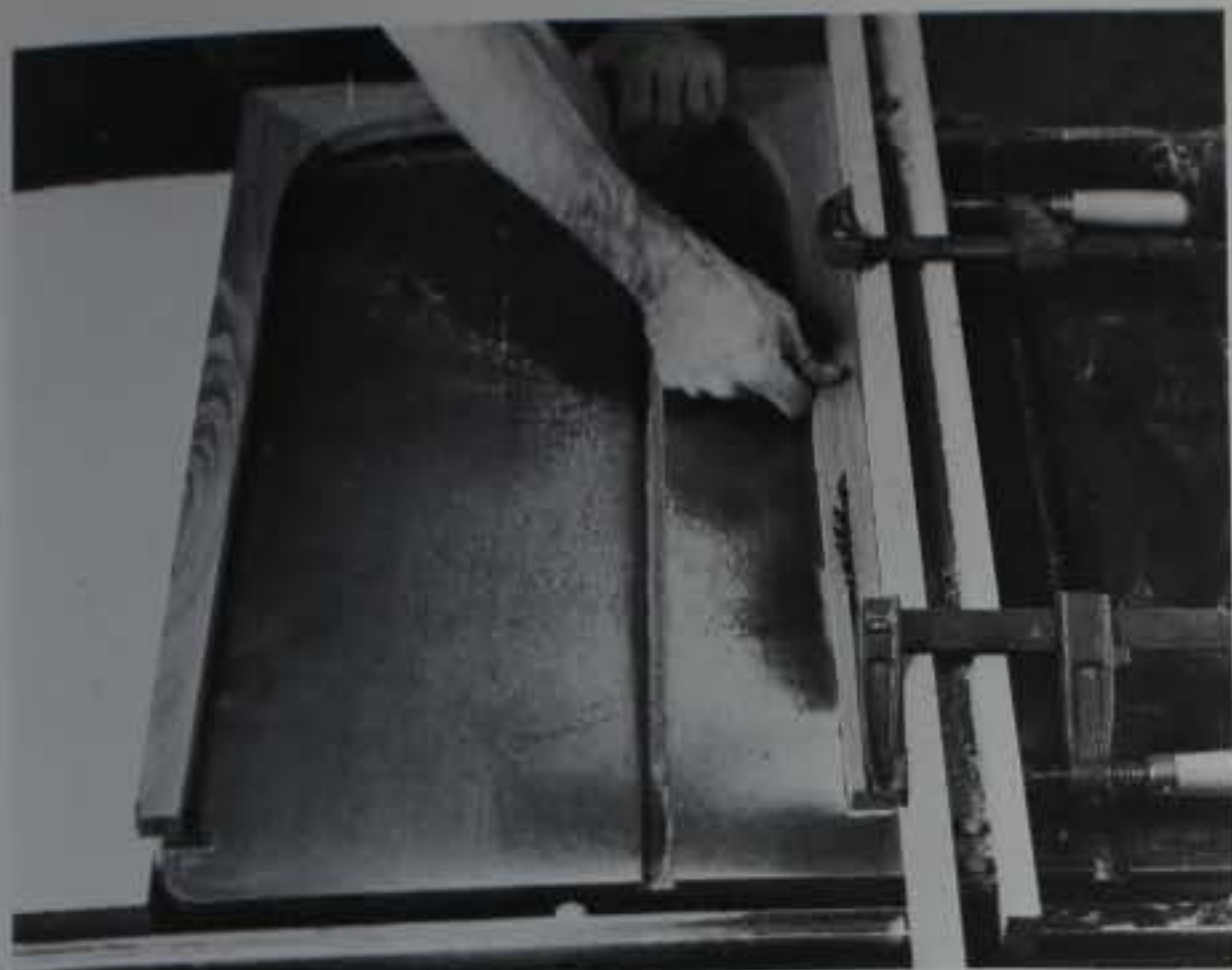
E. Wooden auxiliary fence guides bevel cut on legs. A push stick is used for the last several inches of the cut, and care is taken to keep stock from being burned or gouged by the blade.
