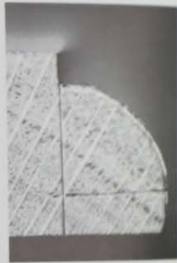
A series of passes with the rabbet plane wastes the bulk of the waste. The open side of this plane allows the iron to cut right to the shoulder of the fillet. At right is an end view of the roughed curve.
