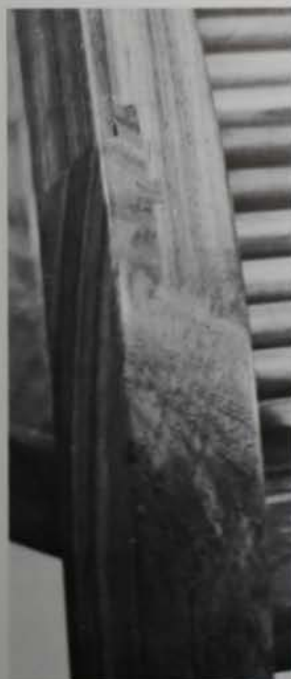
Chinese keyed splice shown in photo and drawings joins leg to desk.
