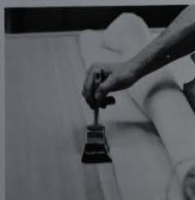
Glue is brushed on a tambour section. Then a veneer hammer, working from center to edges, smooths out the canvas.
