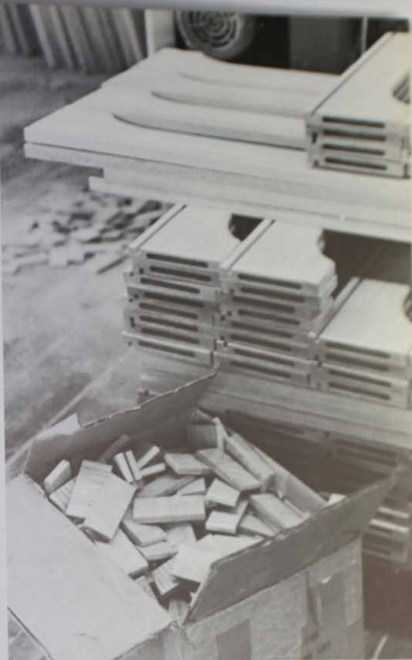
If production work is to proceed apace, like parts should be stacked together to be machined as units of work. These table aprons, which have been shaped, mortised and grooved, await assembly. The box contains the floating tenons that will join aprons to legs.
