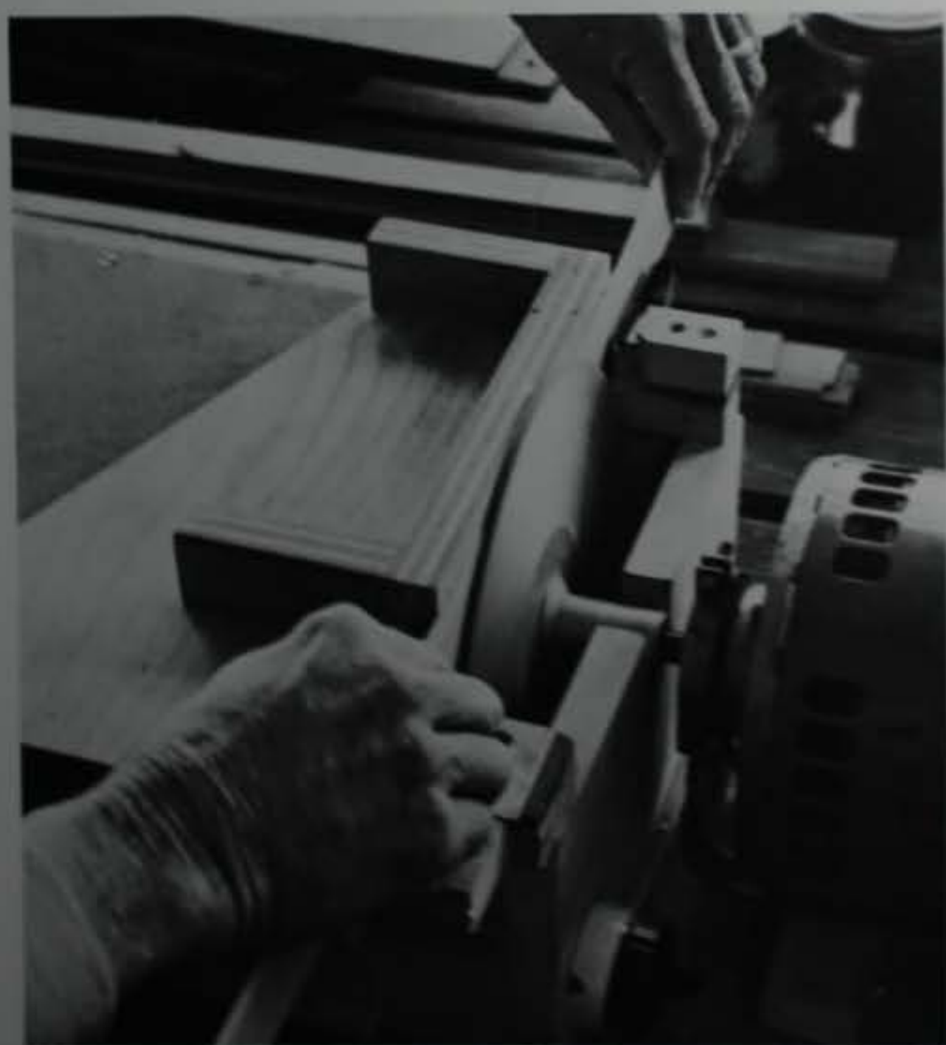
A better method for thicknessing stock employs a tapered sanding disc mounted on a direct-drive mandrel opposite an adjustable fence. This device will give accurate results, thicknessing 1½-in. wide planks to tolerances of 0.003 in. edge to edge.
