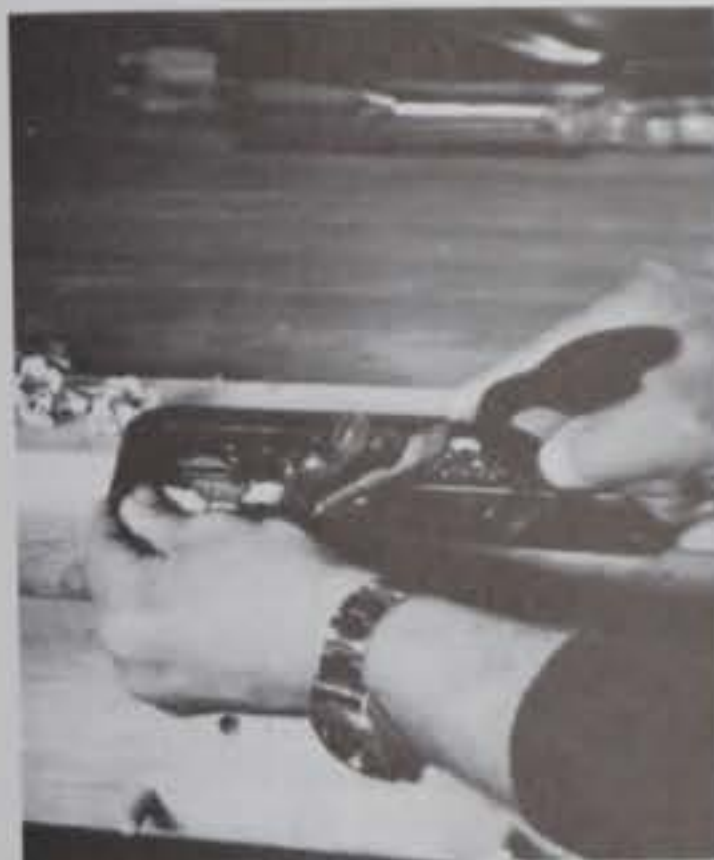
A series of passes with the rabbet plane wastes the bulk of the waste. The open side of this plane allows the iron to cut right to the shoulder of the fillet. At right is an end view of the roughed curve.
