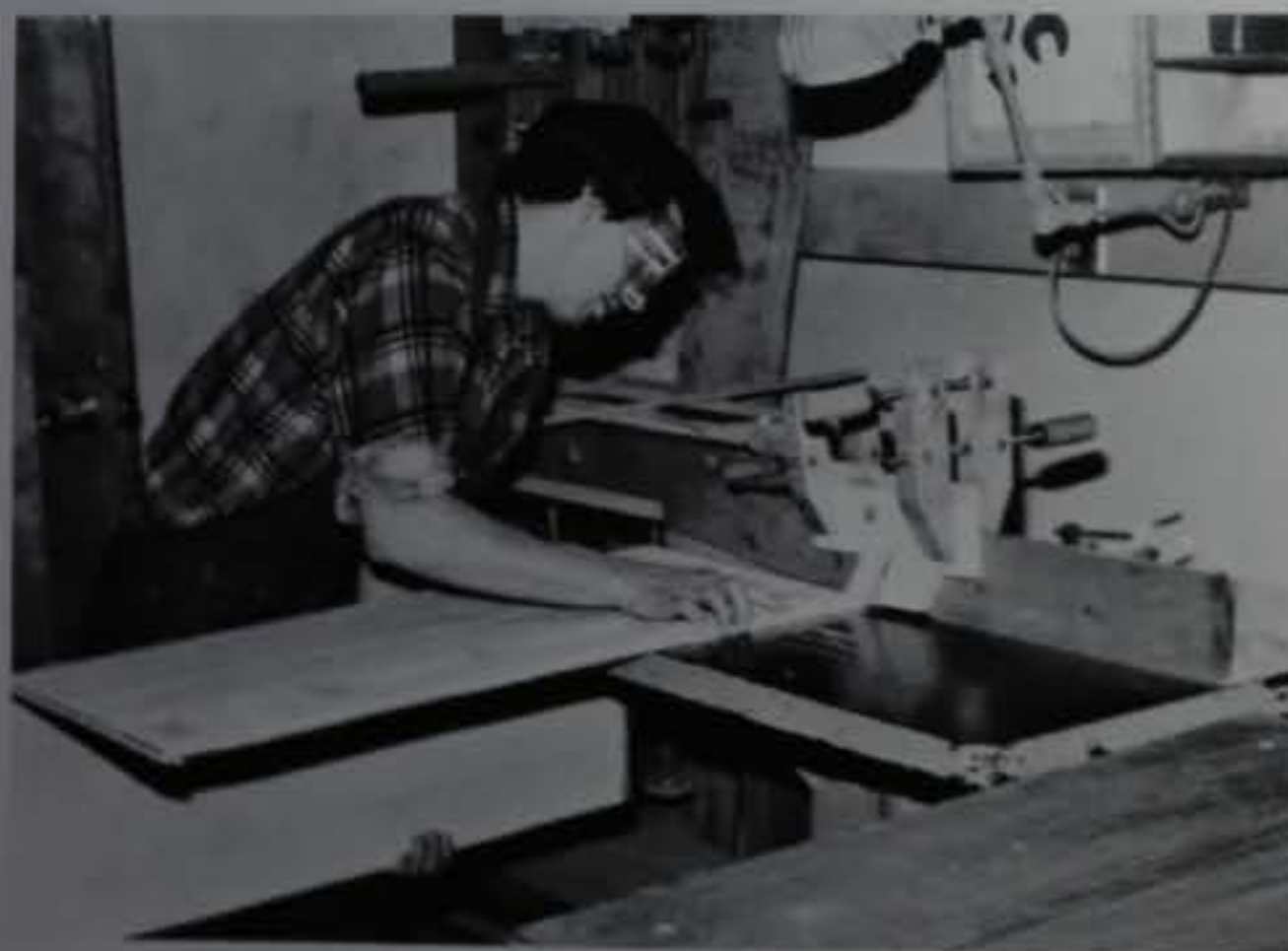
After tambour is glued up, tongue shoulders are sawn (left), then waste is routed from front and back (above). Canvas flap is for attaching handles.
