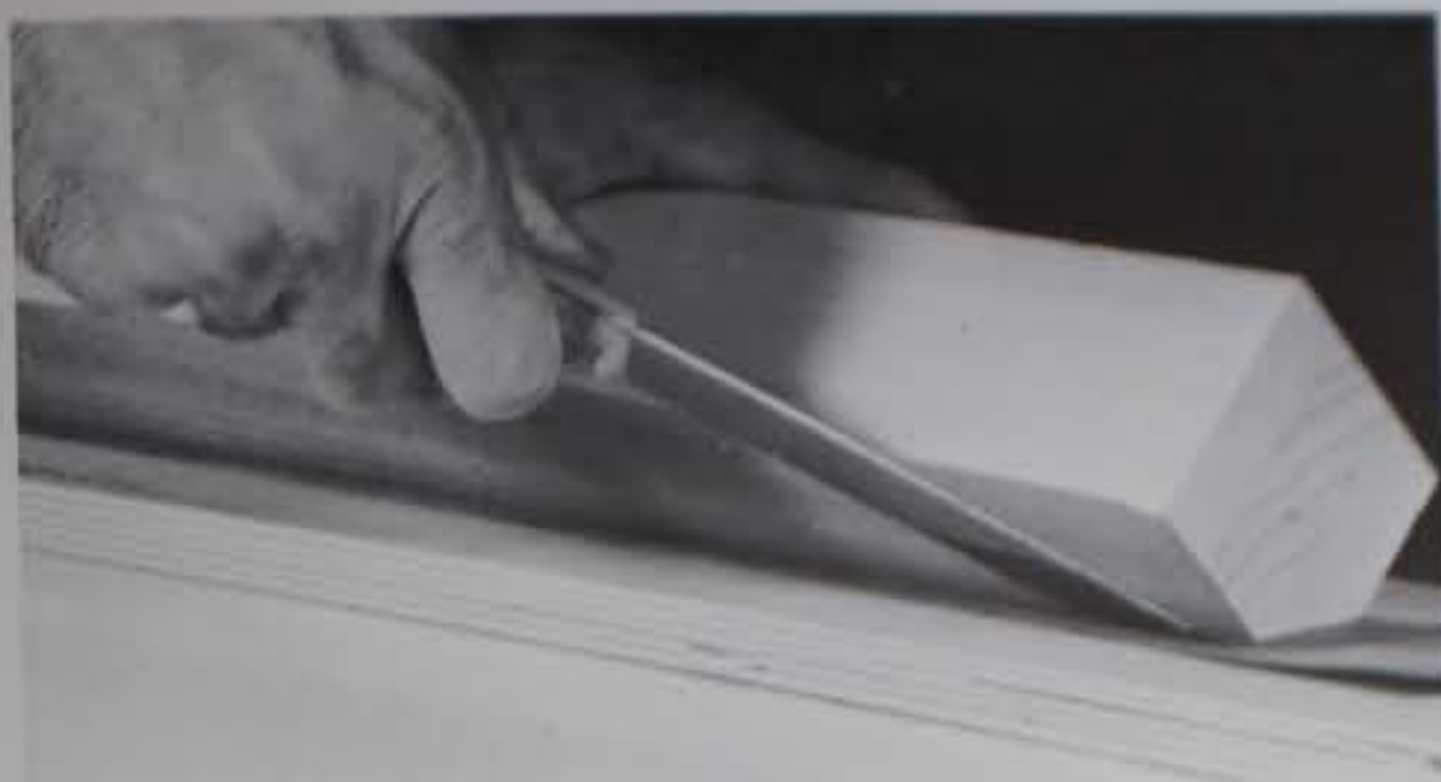
When the glue has set, use a serrated veneer knife, or a veneer saw, to trim the excess veneer and plane flush.
