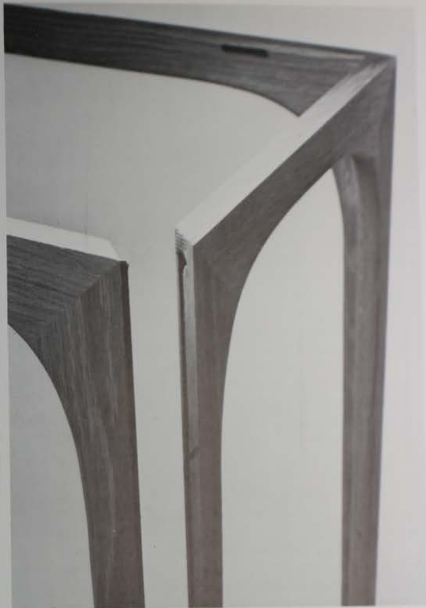
G. The legs should fit together easily, and the mating surfaces should have no gaps for an ideal interface. When the glue is applied, the joints are assembled by hand, pressed together and secured with clamps and tape at frequent intervals along their length.
