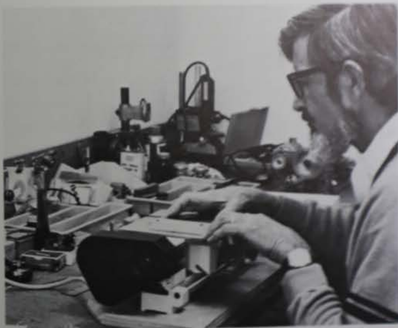
For producing crisp and precise mortises, grooves and tenons, Dorsett uses a machinist's slotting saw mounted on a mandrel and driven by a horizontal miller. Fence and table register the stock.
