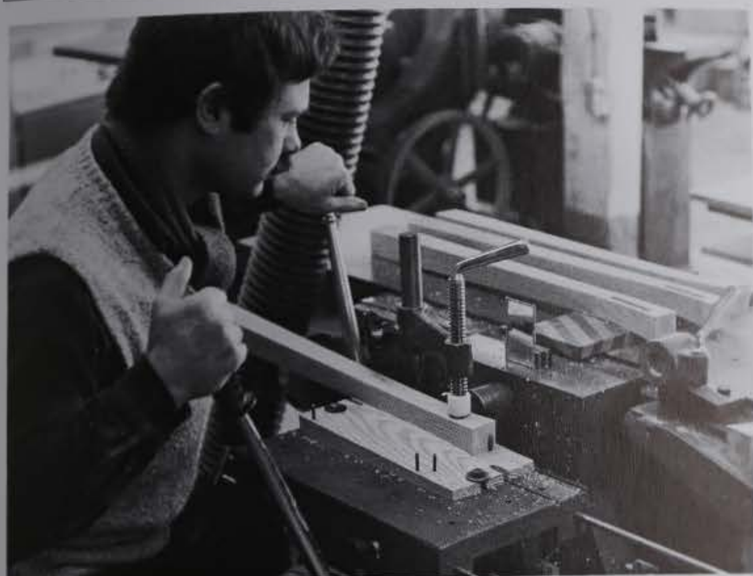
To mill angled mortises in 200 legs, Tracy bolted a 4° ramp to his Steton Combinata. A mirror taped to the machine lets him view the action.
