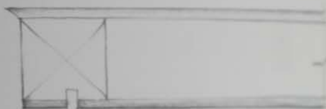
B• SPLINED AT RIGHT ANGLES.
