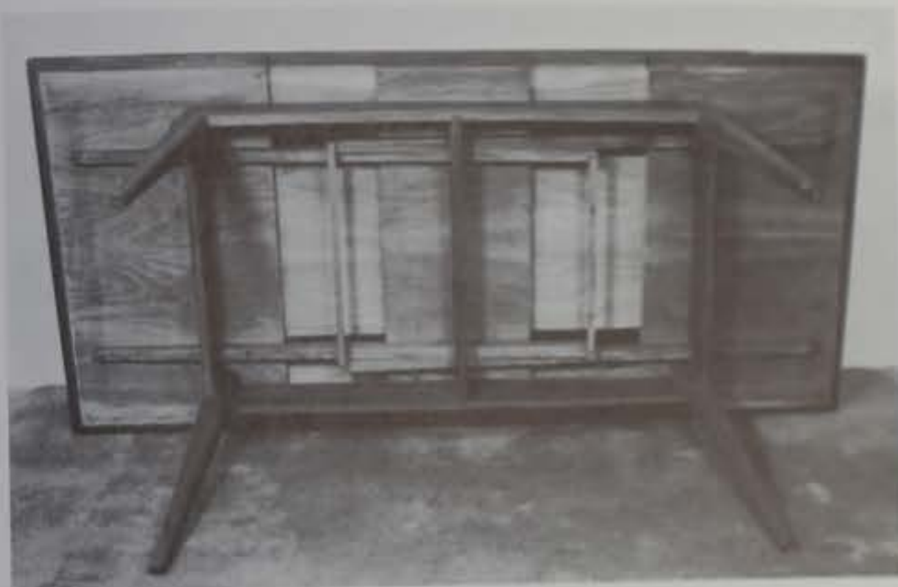
Partly open view from below shows system of slides, stops.
