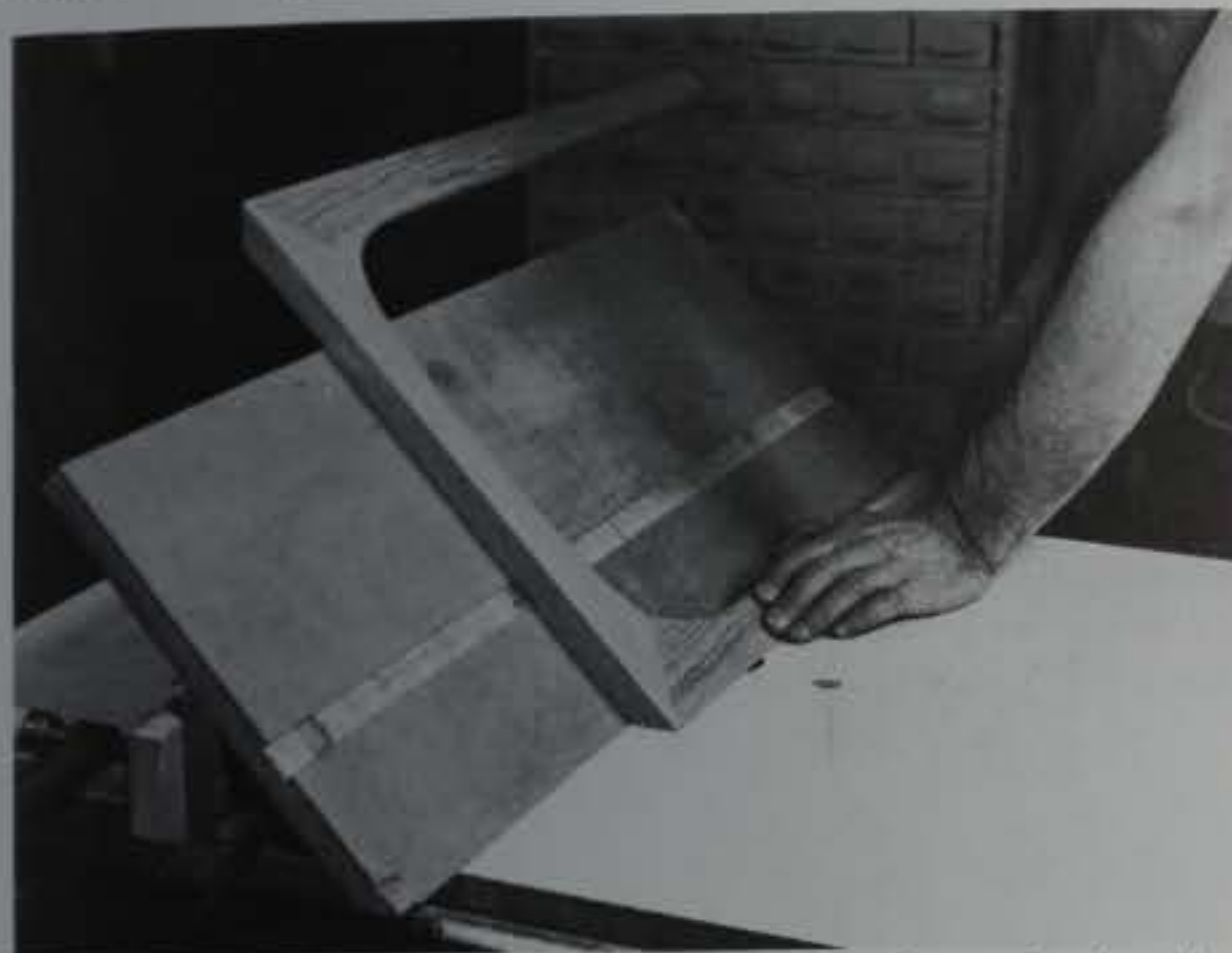
F. A wide fence on router table is used to guide stock when slotting the miter down the length of the legs. The extra-large fence gives needed support to the leg-and-apron assembly and ensures accuracy in cutting.
