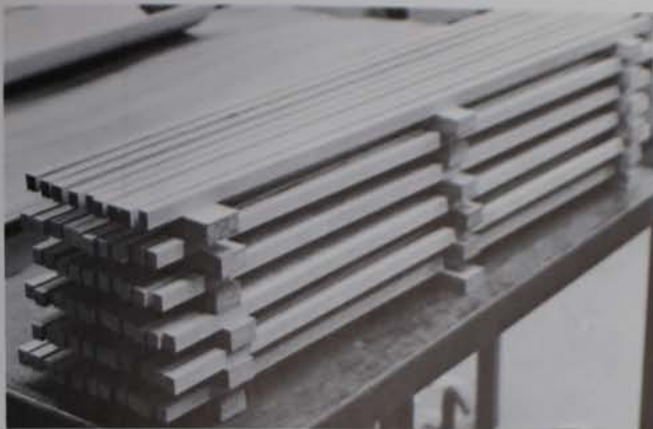
Stickered tambours dry unrestrained; warped ones will be discarded.
