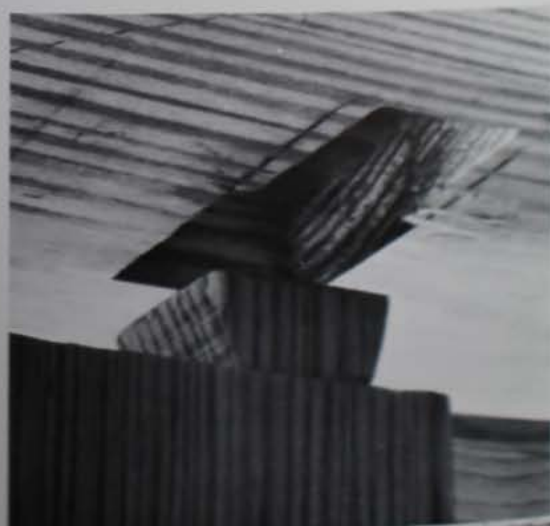
Close attention to joinery, proportion and grain orientation can make the difference between success and failure in the simple design of the table at left. Removable top is secured by dovetail pins, above, which are engaged in housings.
