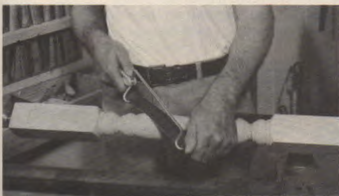
Fig. 31-7. A—Make a contour block to sand mouldings, trim, and other curved surfaces. B—Strips of abrasive used by hand or in a bow sander work well with turned pieces. (Glit, Inc.)
