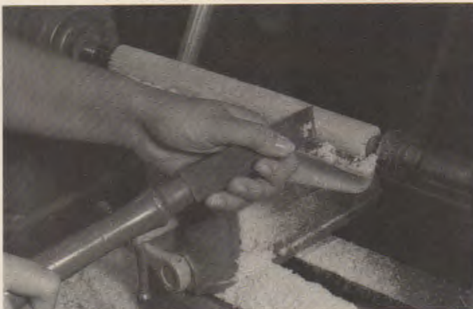
Fig. 27-1. Between-center turning for making spindle products. The guard was removed to show the operation.
