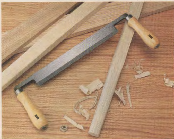
Fig. 26-61. A draw knife shapes table legs quickly. (American Machine and Tool Co.)
