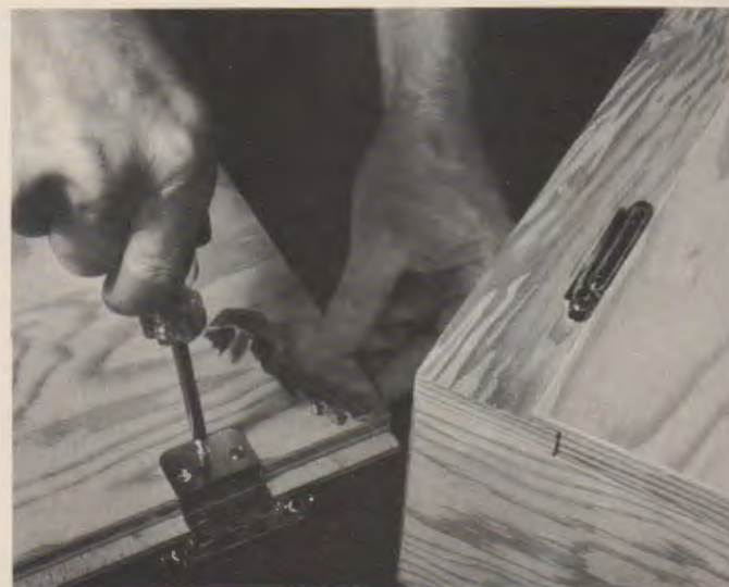
Fig. 17-18. One leaf of semiconcealed formed hinges is decorative and installed on the cabinet surface. This one is used with a lip edge door. (American Plywood Assoc.)
