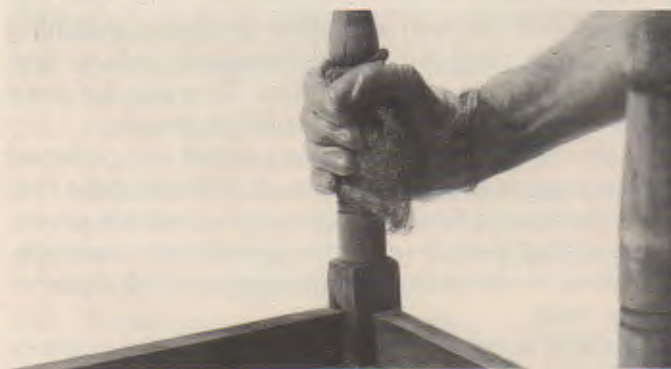
Fig. 48-28. After washing the surfaces, rub with steel wool. (Benjamin Moore)
