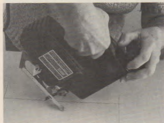
Fig. 22-30. Plunge cutting with a saber saw. The tip of the blade must not "bounce" on the material.
