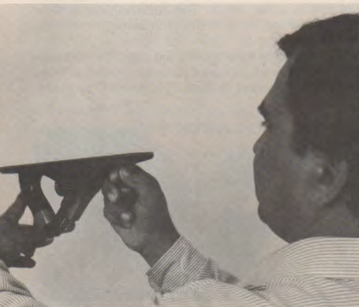
Fig. 24-5. Sight down the sole to check whether the plane iron extends equally through the mouth.
