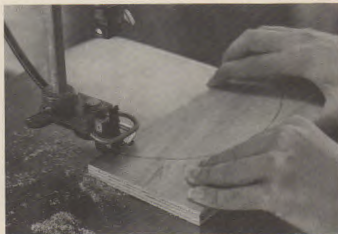
Fig. 21-53. A saber saw blade can be installed in the bottom chuck of most scroll saws.
