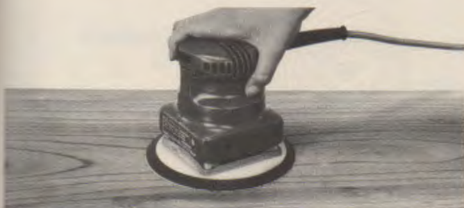
Fig. 31-26. Abrasive disks are used on some orbital and in-line finishing sanders. (Makita U.S.A., Inc.)
