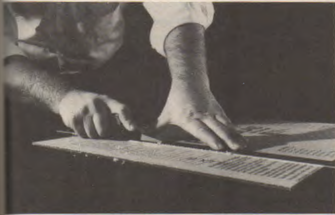
Fig. 15-24. Steps in fracturing plastic. Left. Score with a plastic cutter. Fracture by bending over a dowel rod. (Rohm and Haas)
