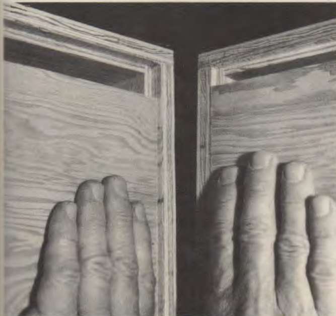
Fig. 29-13. Rabbet joints are often used to hide the edge and grain of a back panel. (American Plywood Association.)
