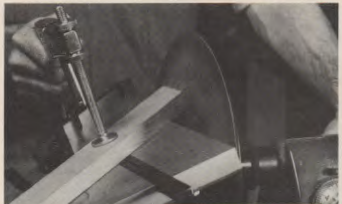
Fig. 31-12. Locate table adjustment controls and rotation of the disk before using the disk sander. (Powermatic Houdaille)
