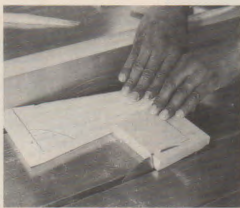
Fig. 40-33. A—Four-sided plinth assembled with compound miter joints. B—Sawing pass one with the five degree taper guide and with the blade at 44.75 degrees. C—Sawing pass two using the 10 degree taper guide. The guard was removed to show the operation.
