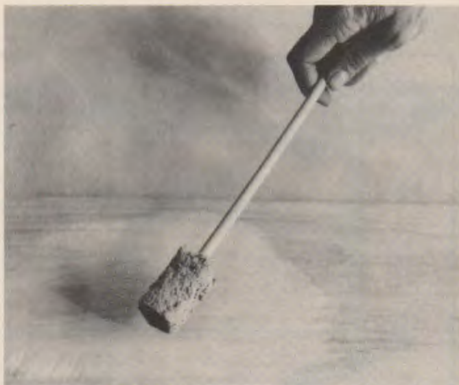
Fig. 45-10. One method to apply bleach is with a sponge attached to a length of dowel.
