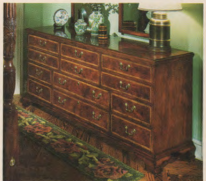
Fig. 40-2. An ogee bracket foot is shaped. (Thomasville)
