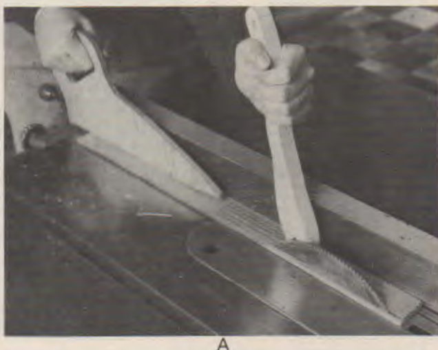
Fig. 21-55. A—Set hollow ground blades high. The guard has been removed to show the operation. B—Resin buildup (dark material) results from sawing only on the rim of a hollow ground blade.
