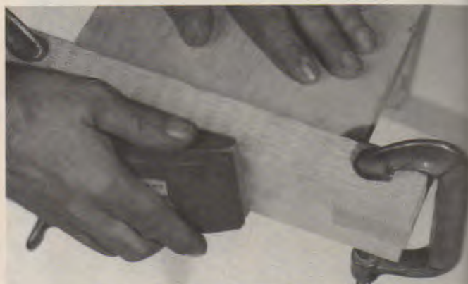
Fig. 31-6. Use C clamps to secure scrap wood when sanding end grain. (Norton Co.)
