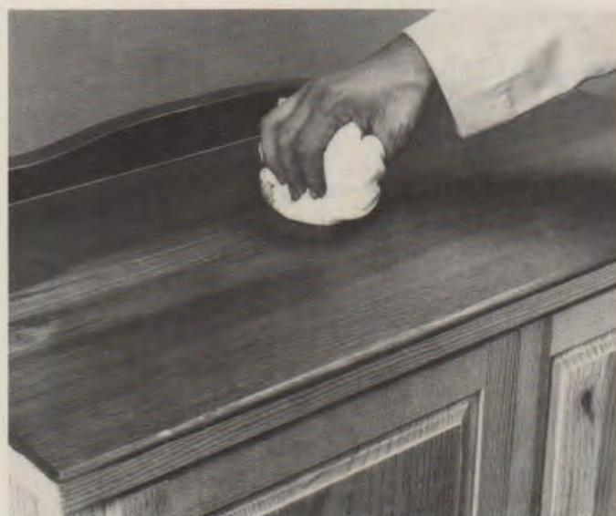
Fig. 47-12. The last step in filling is to wipe lightly along the grain to remove any leftover filler and smooth out streaks. (Carver-Tripp)
