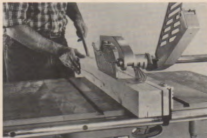
Fig. 21-20. A one-pass resawing operation. This split guard has one side raised. (Delta)
