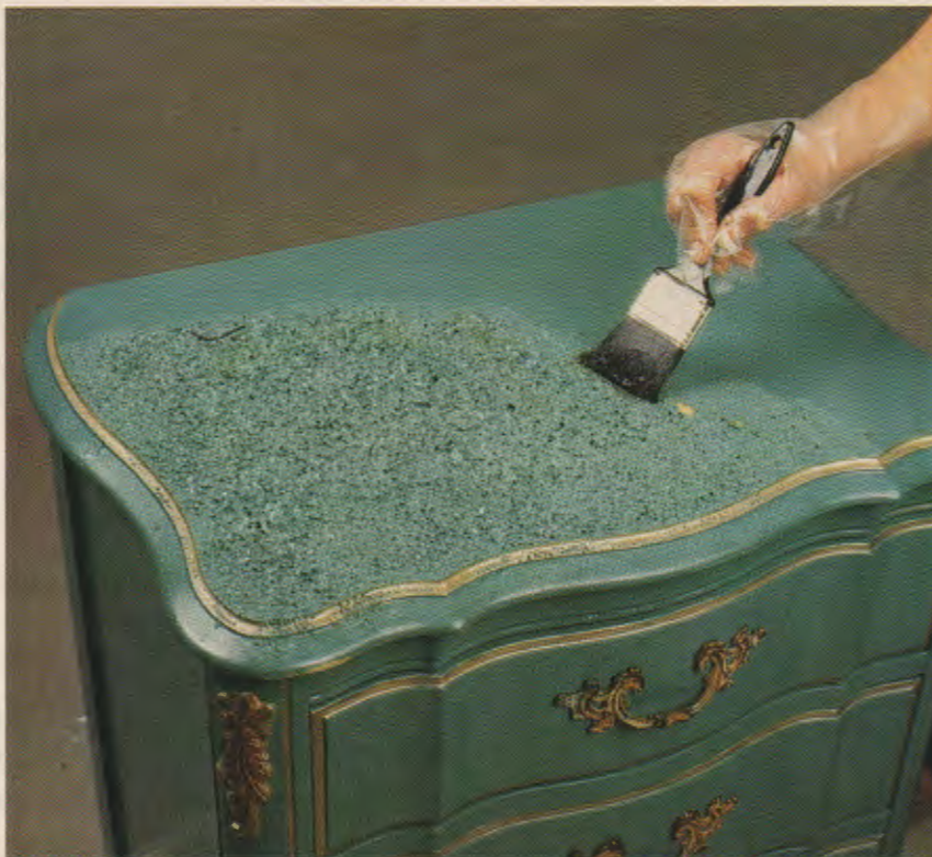
Fig. 44-9. Applying paint remover softens the finish. (Klean-Strip)
