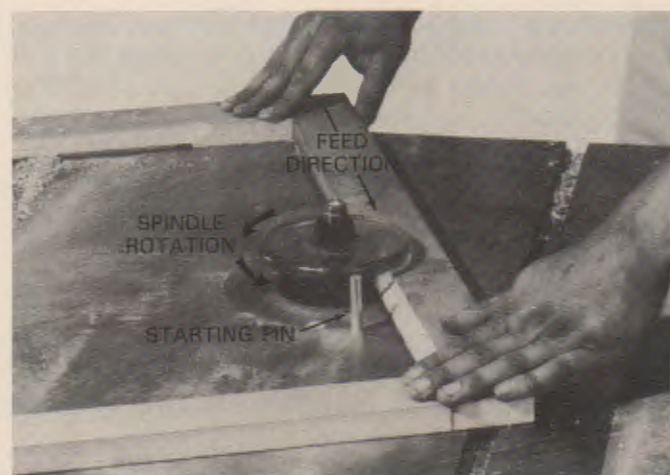
Fig. 26-5. With a collar and starting pin, neither a fence nor miter gauge is needed. (Delta)
