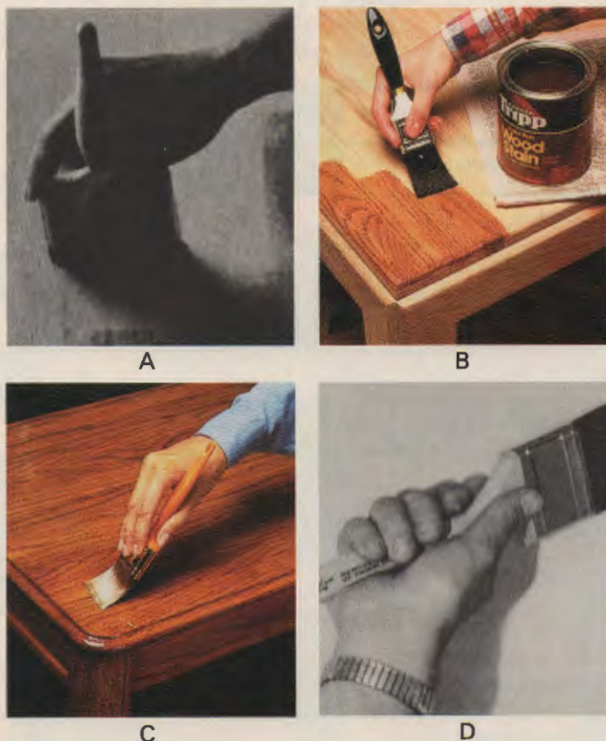
Fig. 46-3. Brushing on a finish. A—Touch the brush to the surface at a 15 degree angle. B—Overlap 50 percent when spreading filler. C—Overlap 25 percent when applying topcoating. (Carver-Tripp) D—Brushing vertical surfaces.
