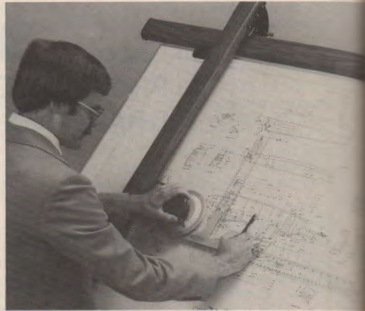
Fig. 9-3. Drafting machines combine the functions of a T-square, triangle, and scale. (Vemco)
