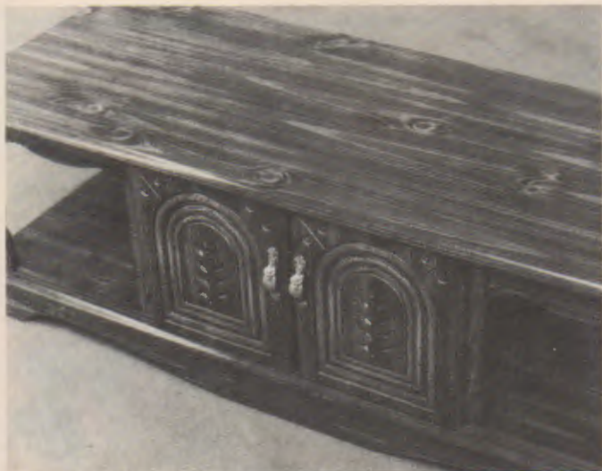
Fig. 47-16. Shading is much like antiquing, except that the grain shows through.
