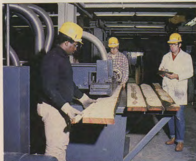
Fig. 11-7. Flitches are ripped manually to maximize width. (Forest Products Laboratory)
