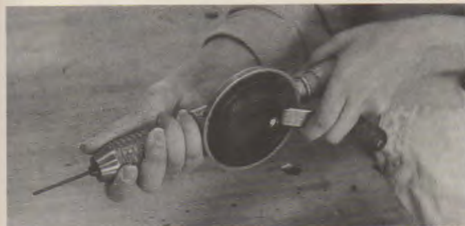
Fig. 25-32. For both a brace and hand drill, install the bit and tighten the chuck by hand.
