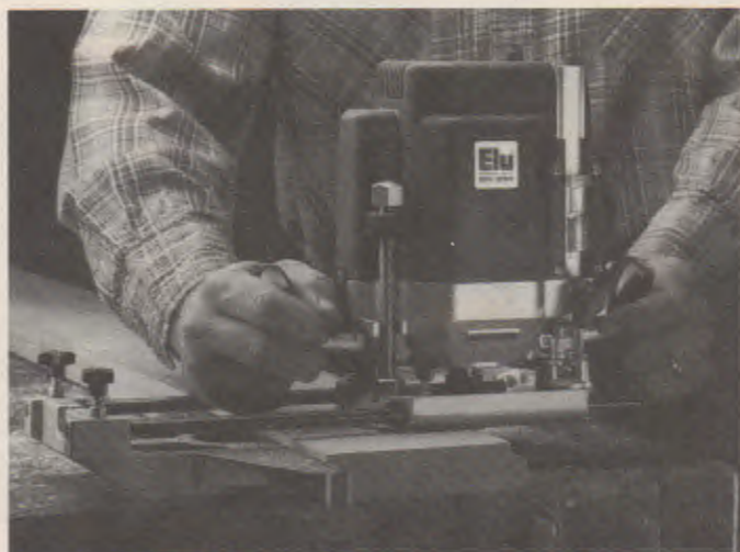
Fig. 26-44. Shaping an edge using a router fence to guide the bit. (Black & Decker)
