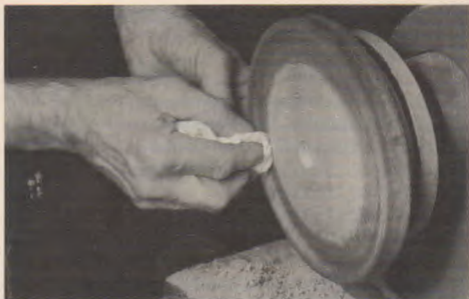
Fig. 48-8. French polish applied on a turned part. Guard removed to show operation.
