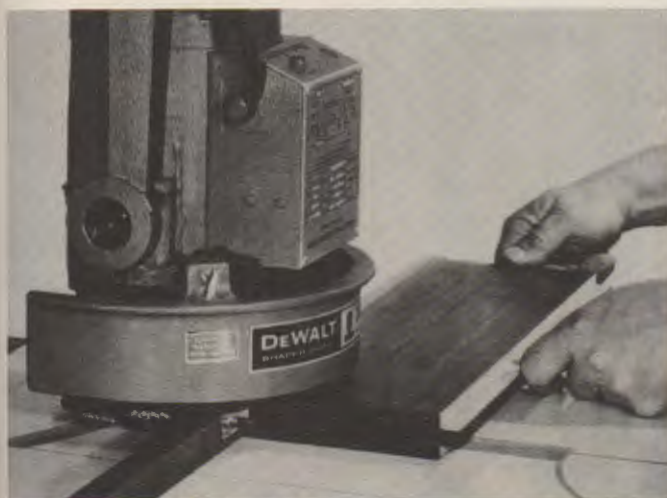
Fig. 29-27. Cutting the groove with a radial arm saw and dado blade. (DeWalt)
