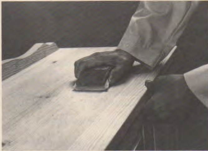
Fig. 45-2. Correct minor scratches with abrasives. (Carver-Tripp)
