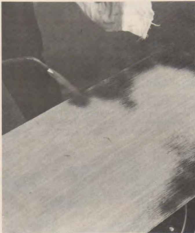
Fig. 45-16. Scorching the surface with a propane torch. Notice the water-soaked rag ready in case the wood catches fire.
