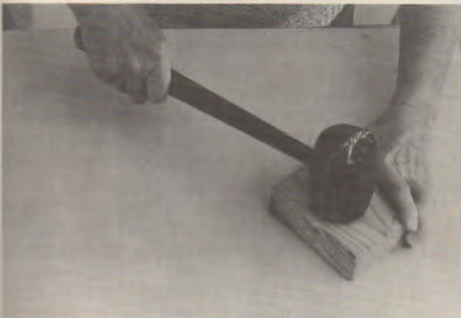
Fig. 36-11. A—With a rolling pin, roll outward from the center to remove air bubbles. B—You can apply more pressure to the ends with a J-roller. C—Rap the surface with a wood block and hammer. (Franklin International)
