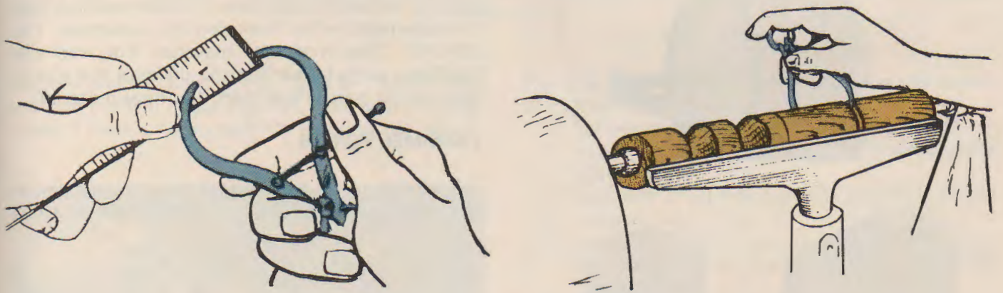
Fig. 20-20. Set and use the outside caliper to check diameter measurements. (The L.S. Starrett Co.)
