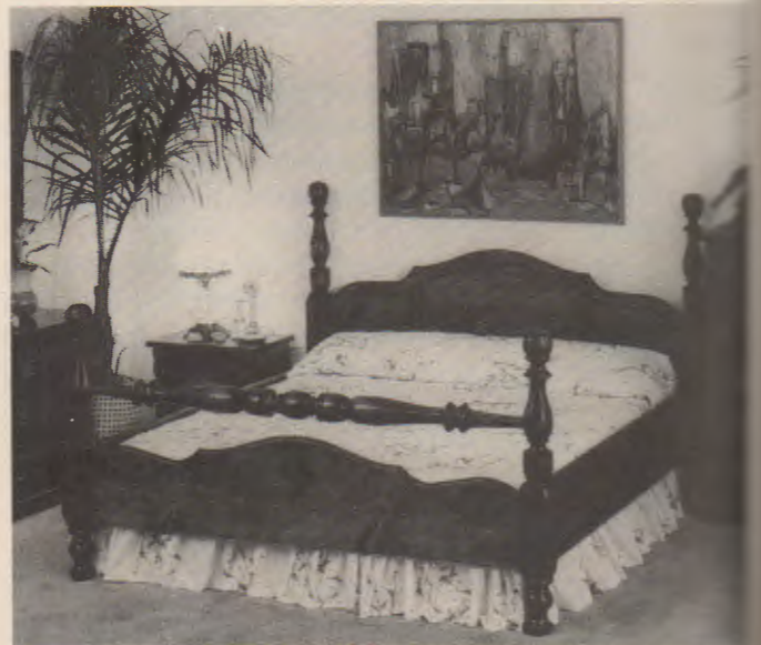
Fig. 27-2. These bedposts were turned between centers (Trendwest)
