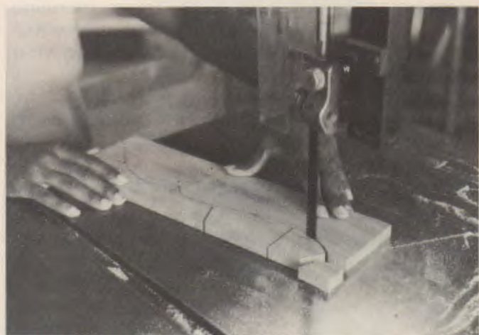
Fig. 21-40. Guide the workpiece with both hands when sawing curves. Blade guide and guard raised for photo.
