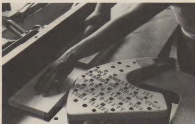
Fig. 23-6. Hold the board firmly against the table when face jointing. (Delta International Machinery Corp.)
