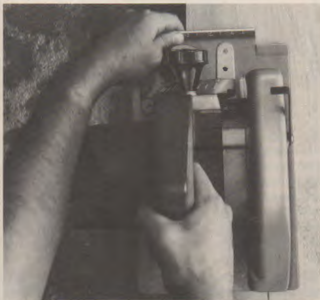
Fig. 22-20. Three methods of guiding a circular saw. A—Using a saw guide. B—Clamping a straightedge. (Makita). C—Guiding with your fingers and the measurement marks on the saw. (Milwaukee Electric Tool Corp.)
