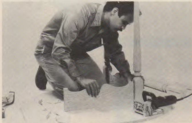
Fig. 40-11. Assembling the legs and apron pieces using plate joinery. A—Mark slot locations on the legs. B—Mark slot locations on the apron pieces. C—Cut the apron slots. D—Align the apron and leg to cut the leg slots. E—Put glue and a plate (biscuit) in both slots on one leg. F—Assemble the legs and apron on a flat surface. (Steiner-Lamello)
