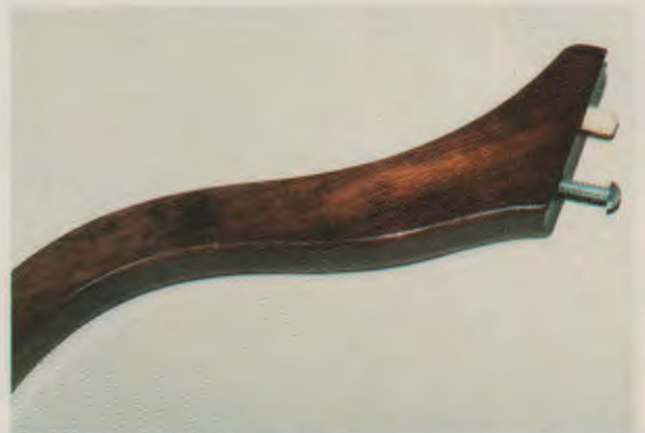
Fig. 40-17. Place an insert nut and dowel in the leg. The screw travels through the pedestal and threads into the insert nut.
