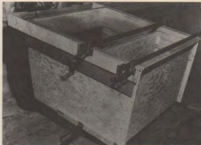
Fig. 33-20. The same number of clamps have been placed on each side of this case assembly. Doing so balances clamp pressure. (Franklin International)
