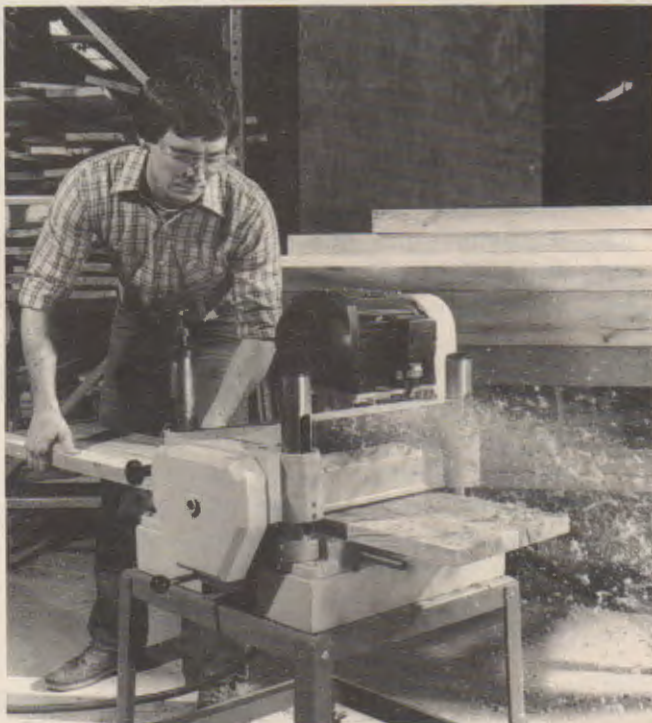
Fig. 23-1. Surface lumber square on jointers and planers. (Delta)
