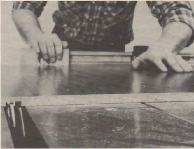
Fig. 29-9. Chippers between the blades make this dado a one-pass operation. Guard removed to show operation. (Delta)
