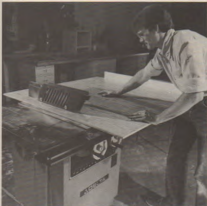
Fig. 21-13. Ripping plywood. (Delta)
