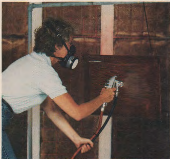
Fig. 6-14. Spraying is an efficient method of applying finishing materials. (DeVILBISS)
