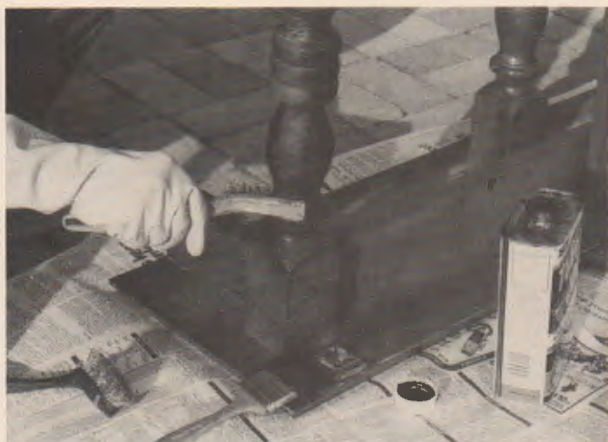
Fig. 48-27. After the remover has been absorbed, take off peeled coatings with a putty knife or wire brush. (Carver-Tripp)
