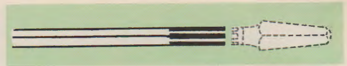
Fig. 25-4. Auger bit shanks have a tang fit in a brace. The tang can be sawed off so the bit can be used in power drills. (Irwin)
