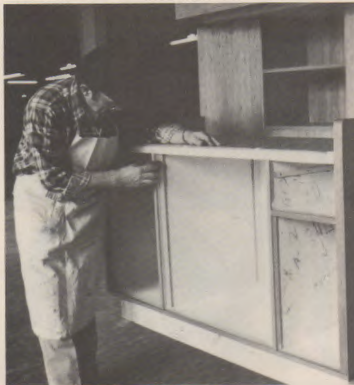
Fig. 45-1. Inspect surfaces and remove defects before applying finish. (Columbus Showcase)
