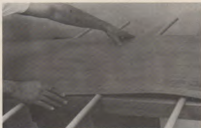
Fig. 35-10. Using dowels to separate veneer from the core. (Franklin International)
