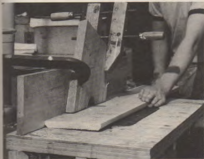
Fig. 26-13. Featherboard hold down jig. (Delta)
