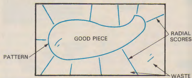
Fig. 15-8. For irregular curves, place the glass over the pattern. Score along the pattern, then make radial scores to remove waste around the workpiece.
