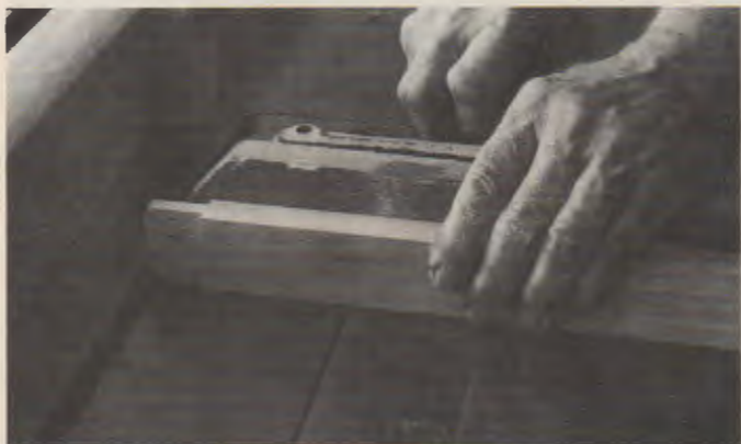
Fig. 29-43. Sawing tenons by making a series of crosscut passes.
