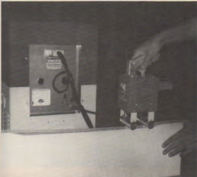
Fig. 32-21. The electrodes on RF gluing guns are shaped according to the joint you are bonding. (Workrite)
