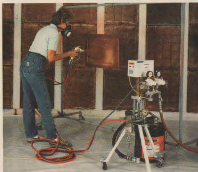
Fig. 52-22. Prefinishing doors. (Devilbiss)
