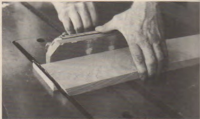
Fig. 21-18. When beveling, feed stock so the excess falls off below the blade. Guards have been removed to show the operation. A—Ripping. B—Crosscutting.
