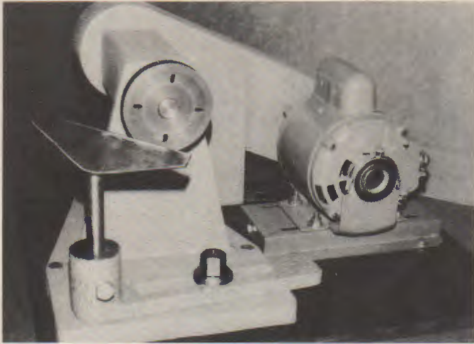
Fig. 27-5. The bowl lathe is for faceplate turning only. (Brodhead-Garrett)
