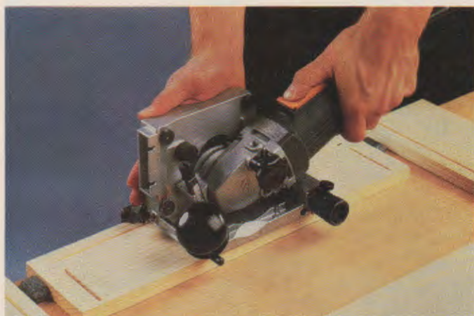
Fig. 29-59. Using plate joinery to assemble a drawer. Recognize the joining plates, or biscuits. Also notice the semicircular slot made in the wood by the plate joining machine. (Black & Decker)
