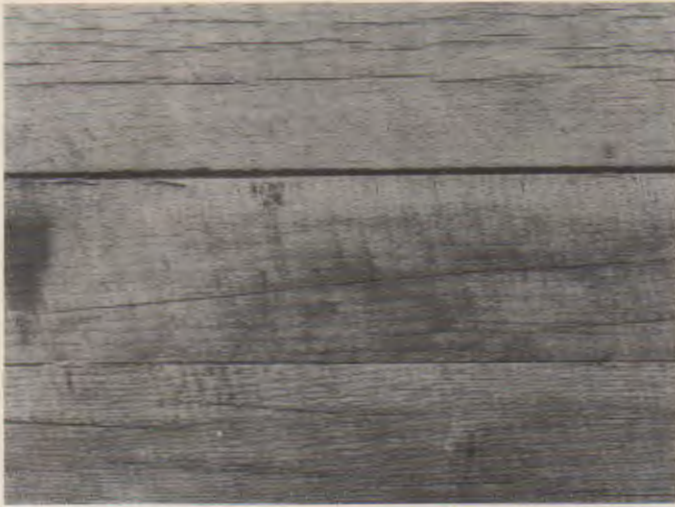
Fig. 11-17. Honeycomb is caused by separation of wood rays. Top. It is seen as voids in the end of cut lumber. (Forest Products Laboratory) Bottom. Honeycomb as depressions in surfaced lumber. (Western Wood Products Association)
