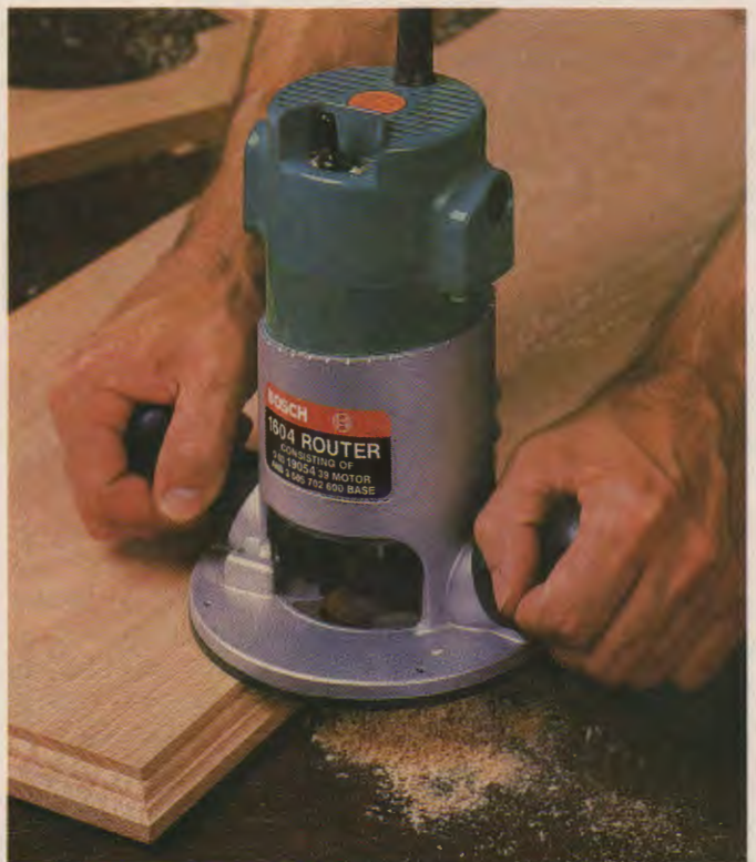
Fig. 6-11. Edge designs are created with a portable router and bit. (Robert Bosch Power Tool Corp.)
