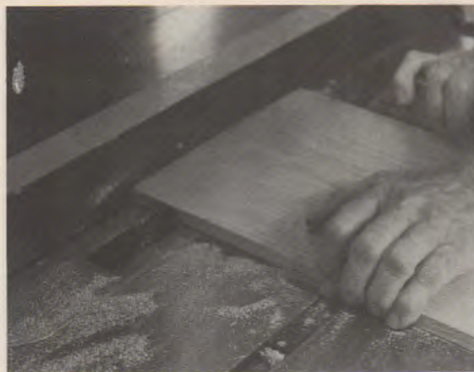
Fig. 21-9. Both the rip fence and miter gauge are used for cuts not completely through the material. A dado cut is shown. The guard has been removed to show the operation.
