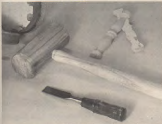
Fig. 27-35. Split turning. A—Glue two pieces of stock together, separated by sized paper. B—Turn the desired shape, then split the parts with a mallet and chisel.
