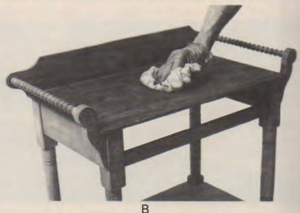
Fig. 47-6. Applying oil stains. A—Apply the stain with a small pad or brush. B—Wipe off the excess after the stain has had a chance to soak in. (Benjamin Moore)
