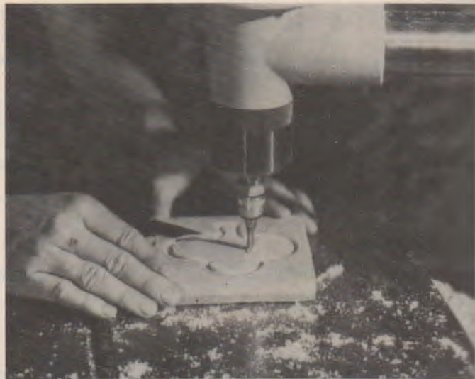
Fig. 26-25. Freehand routing. The guard has been removed to show the operation. (Delta)
