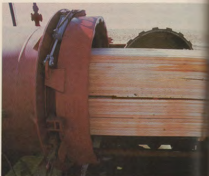
Fig. 11-28. Wood preservatives are applied in a high pressure container. (Georgia-Pacific Corp.)
