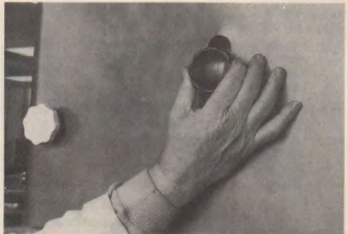
Fig. 21-38. Tracking adjustment is found on the back of the machine behind the upper wheel.
