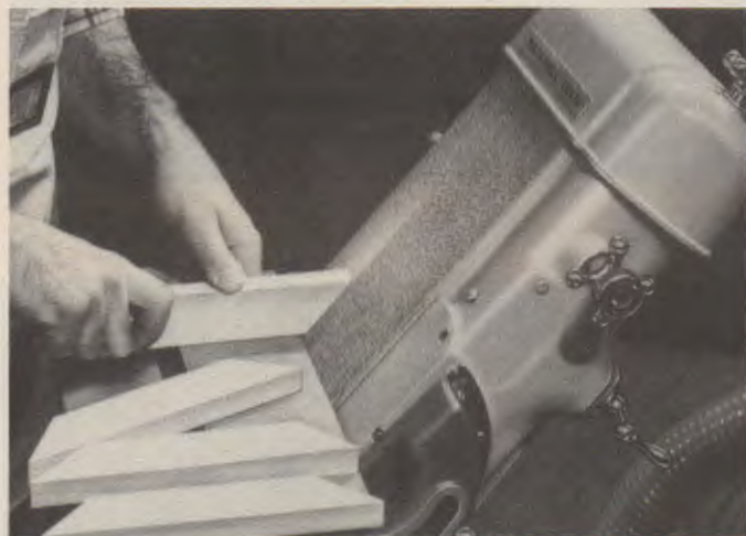
Fig. 31-7. A—Make a contour block to sand mouldings, trim, and other curved surfaces. B—Strips of abrasive used by hand or in a bow sander work well with turned pieces. (Glit, Inc.)
