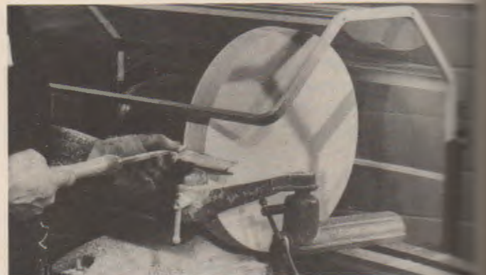
Fig. 27-3. Faceplate turning. (Delta)
