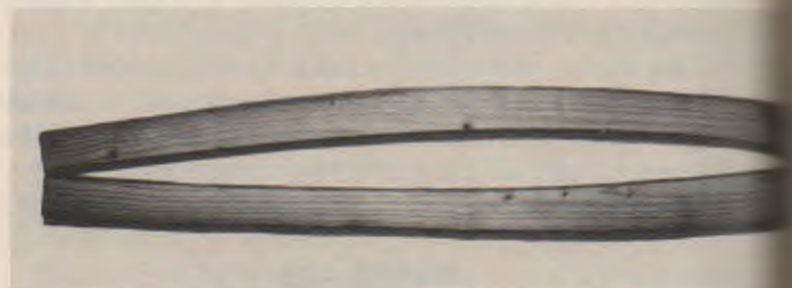
Fig. 10-12. The distortion of reaction wood during cutting can be dramatic. (Forest Products Laboratory)
