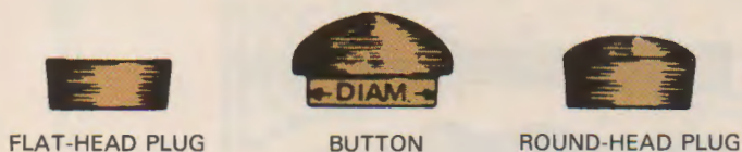
Fig. 11-36. Plugs and buttons cover counterbored holes.
