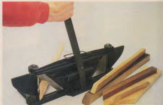
Fig. 28-27. The miter trimmer shears perfect miters on moulding. (The Fine Tool Shops)
