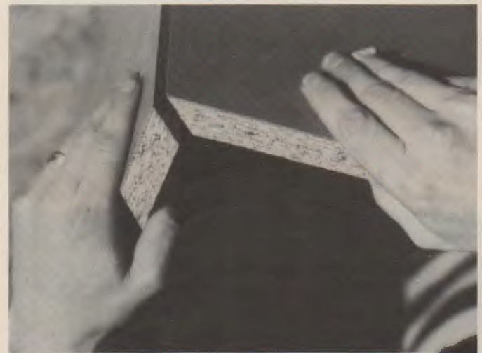
Fig. 14-17. Laminates are typically bonded to a particleboard core. The particleboard supplies strength. The laminate provides the desired appearance. (Columbus Showcase)
