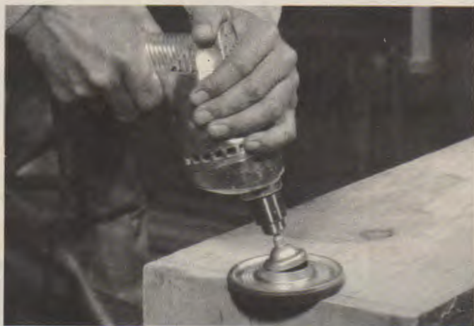
Fig. 31-27. Use disk sanders when the surface will be hidden. (Norton Co.)
