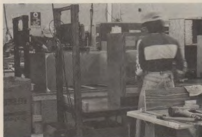
Fig. 52-23. Finishing touches are made to the case before prefinished doors are installed. The case sides are covered with laminate. (Formitex)
