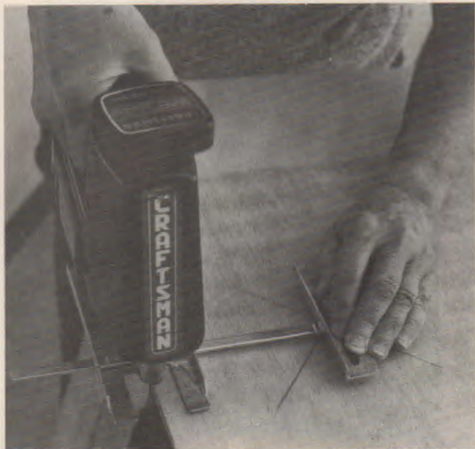
Fig. 22-29. Saw accurate circles with a guide and pivot accessory.
