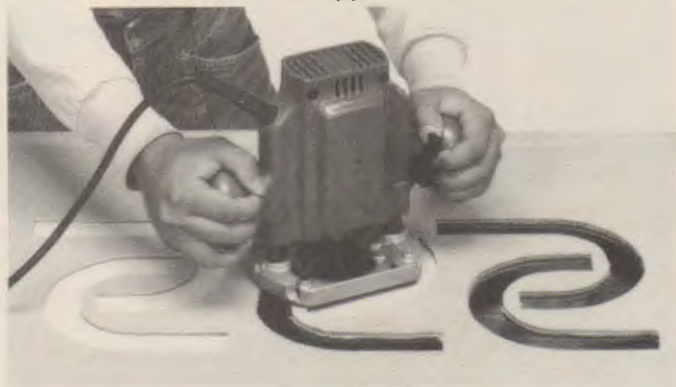
Fig. 26-50. Routing with a template guide. A—The template is placed over the workpiece. The plunge router shown here plunges the bit into the workpiece to start the cut. (Makita) B—The template guide then rides along the template. (Bosch)
