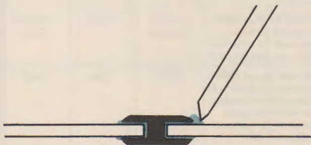
Fig. 15-20. Press grout between came and glass pieces.
