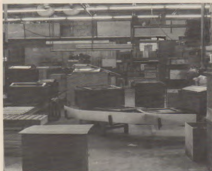
Fig. 52-20. Spraying completed products. A—The finish is applied in a ventilated spray booth. B—Dried cabinets roll out ready for packaging. (Riviera Cabinets)
