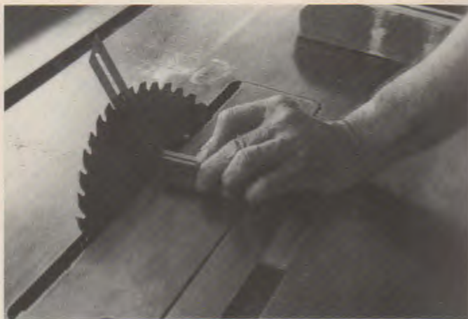
Fig. 21-17. Set blade tilt with a T-bevel. First set the T-bevel angle with a protractor. Remove the guard for this set up.
