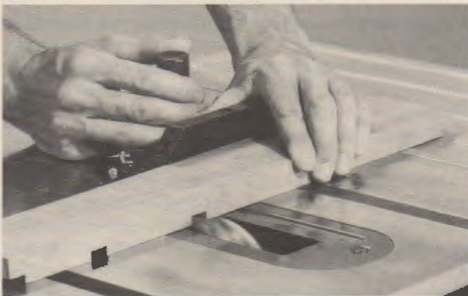
Fig. 29-9. Chippers between the blades make this dado a one-pass operation. Guard removed to show operation. (Delta)
