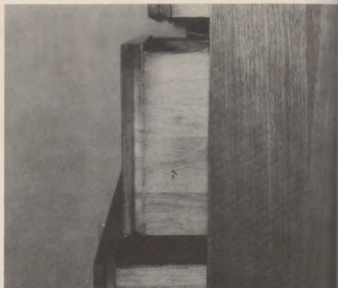
Fig. 42-9. Lip-edge dovetail. The drawer front end and side are not flush.
