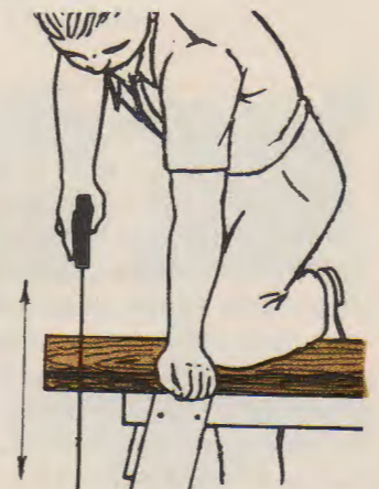
Fig. 22-12. A—Start a cut using your thumb as a guide. B—Then proceed with long strokes. (Porter)
