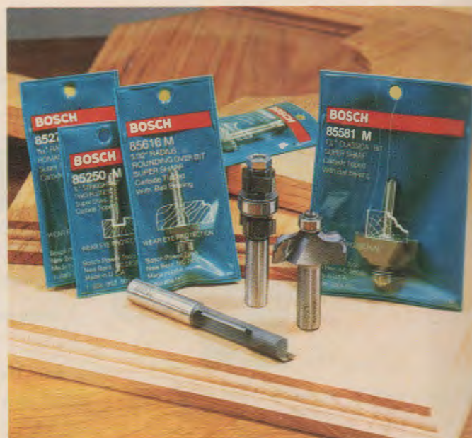
Fig. 26-20. Router bits. Notice that some are assembled, while others are one piece. (Bosch)
