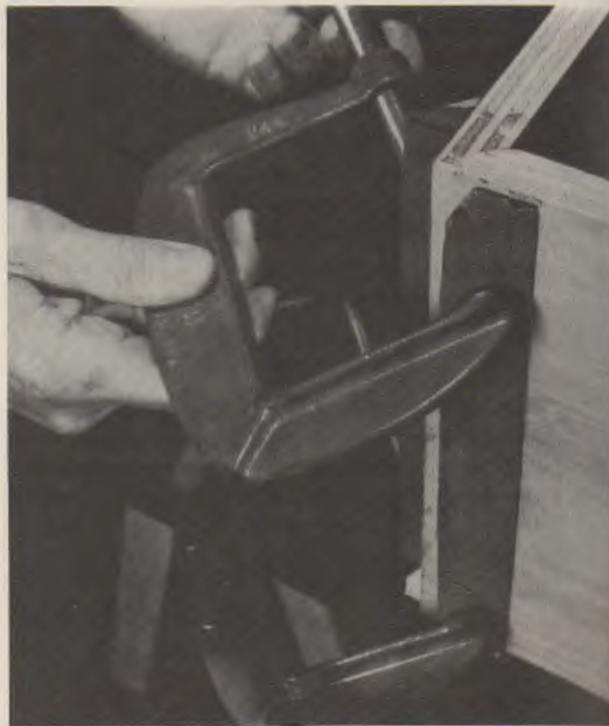
Fig. 33-6. C clamps can secure mitered corners. (Franklin International)
