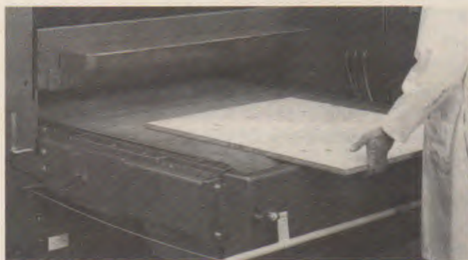
Fig. 31-19. Widebelt sanders typically smooth only one surface at a time. (Timesavers, Inc.)
