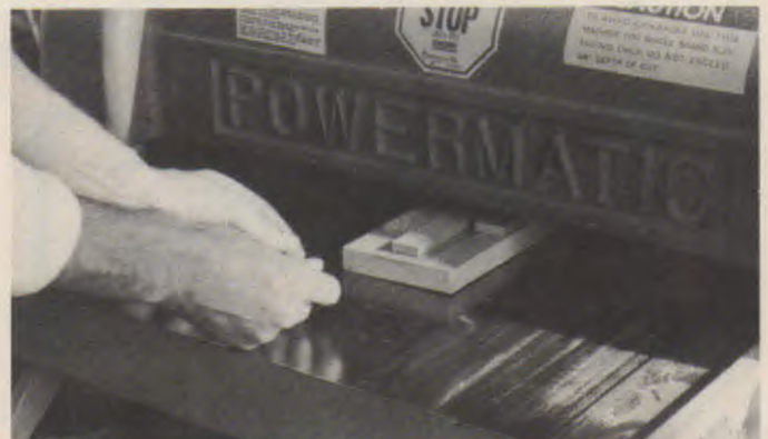
Fig. 23-15. Surfacing thin material requires a backing board.
