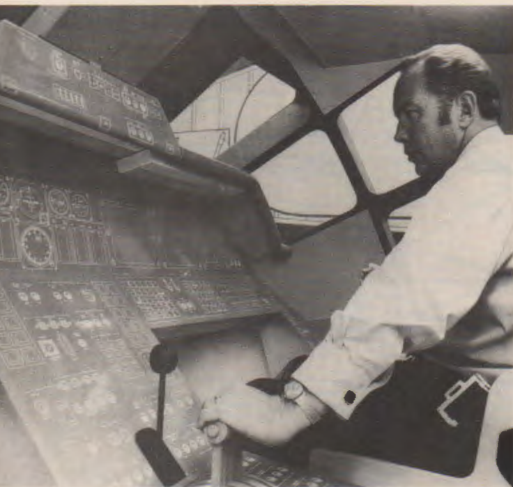
Fig. 8-10. Hard mock-ups have movable parts to test for human comfort. Here, a research pilot checks line of sight to instrument panel and reach to controls.
