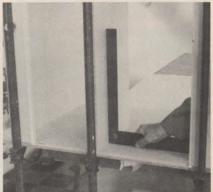
Fig. 49-43. A—Assemble the cabinet with glue and bar clamps. B—Check the squareness.
