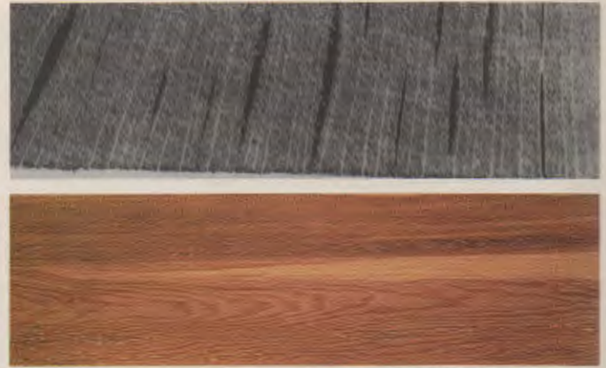
Fig. 11-17. Honeycomb is caused by separation of wood rays. Top. It is seen as voids in the end of cut lumber. (Forest Products Laboratory) Bottom. Honeycomb as depressions in surfaced lumber. (Western Wood Products Association)
