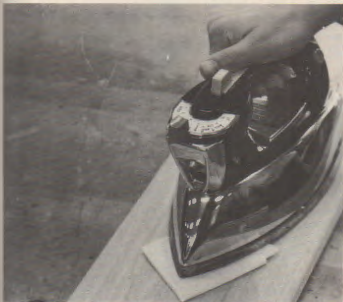
Fig. 31-2. Raise dents with water or a wet pad and an iron before abrading. (Glit, Inc.)
