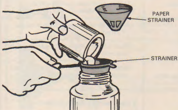
Fig. 46-14. Strain out debris before filling the finish cup. (DeVilbiss)
