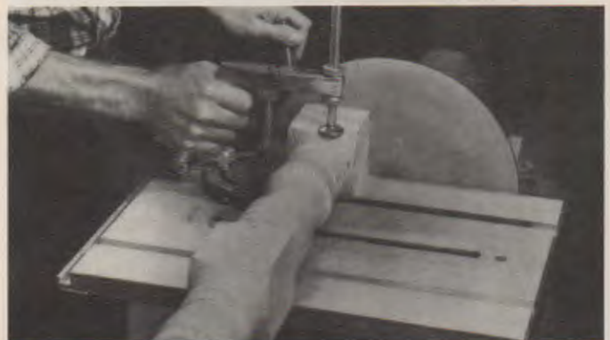
Fig. 31-13. By using a miter gauge or tilting the table, many different workpieces can be abraded. (Shopsmith, Delta International Machinery Corp.)
