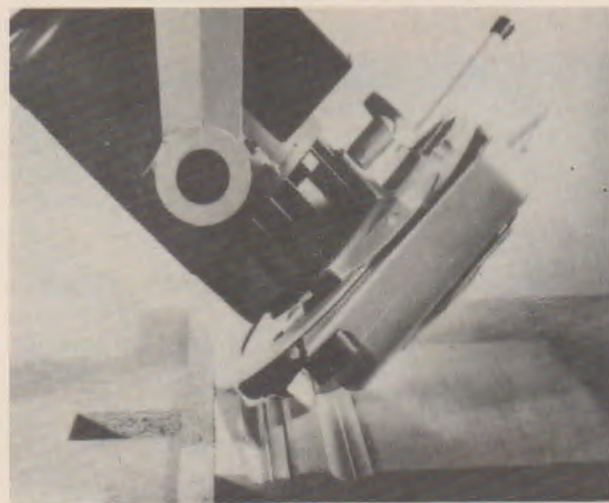
Fig. 26-36. A—A cutterhead guard is necessary when the cutterhead is set in the horizontal shaping position. B—Shaping at an angle. (DeWalt)
