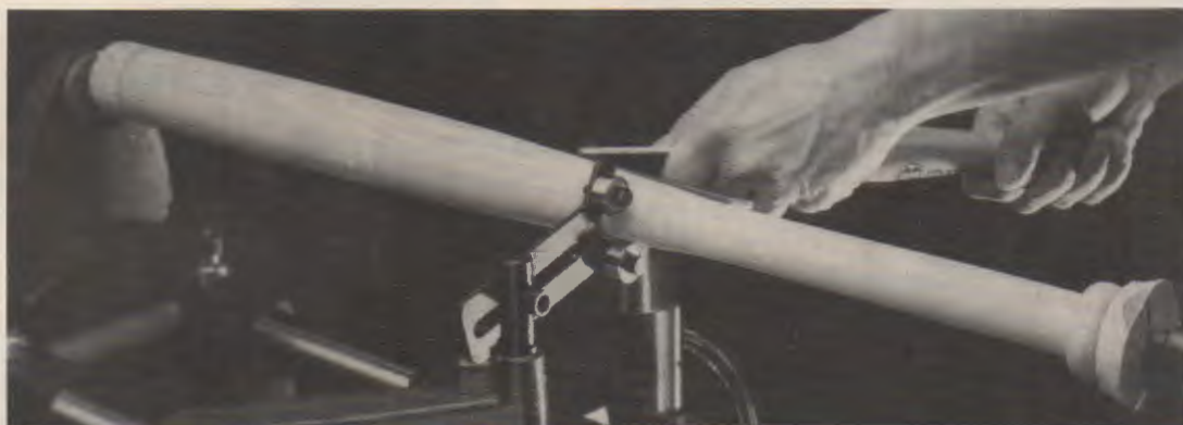
Fig. 27-27. A steadyrest increases stability and reduces chatter. The guard was removed to show the operation. (Shopsmith)
