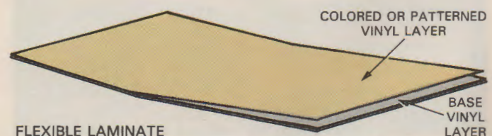
Fig. 14-18. Flexible laminates are composed of layers of vinyl or other flexible plastics.
