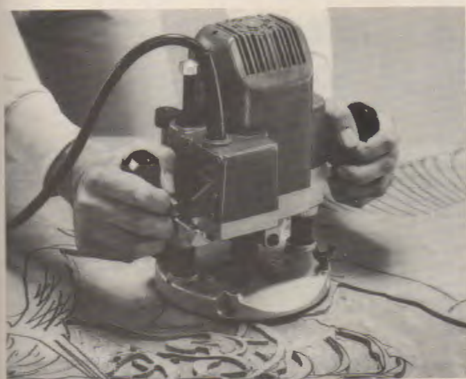
Fig. 26-47. Work on carving may begin with routing out excess material. (Makita)
