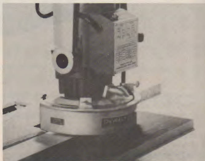
Fig. 23-18. The radial arm saw can be converted to a surfacer with a cutter and guard. The arbor is placed down. (DeWalt)
