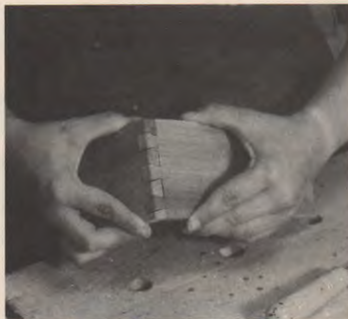
Fig. 29-50. Dovetails are an intricate, but attractive joint.
