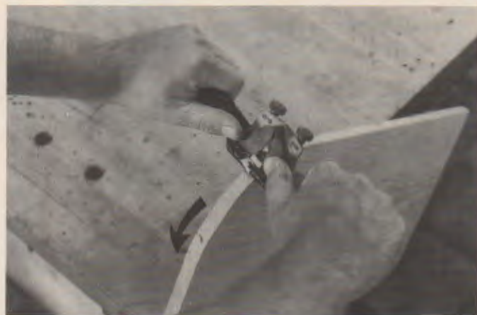
Fig. 26-55. Push or pull the spokeshave around contours with the blade leaning away from the direction of cut.
