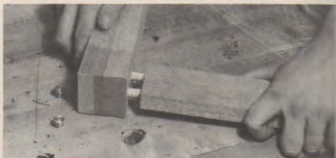
Fig. 29-58. A—Dowel centers. B—Drilling holes in apron end for dowel joint to leg. C—Place dowel centers in the apron to mark hole locations. D—Keep the parts square while pressing the apron to the leg. E—Drill dowel holes in the leg at locations marked by the centers. F—Assembling the leg and apron.
