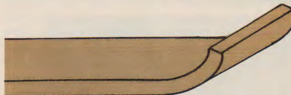
Fig. 34-17. Partial curved laminations. A—Kerfing. B—Inserting veneer in the kerfs. C—Gluing and clamping the lamination. D—Finished product.
