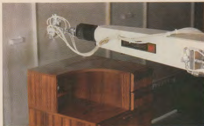
Fig. 52-21. Spraying with a robot. (Devilbiss)
