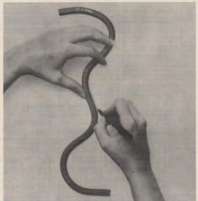
Fig. 9-10. Top. A French curve can be used to draw any irregular curve. Bottom. A flexible curve will bend to trace long curves. (Hearlily & Co.)
