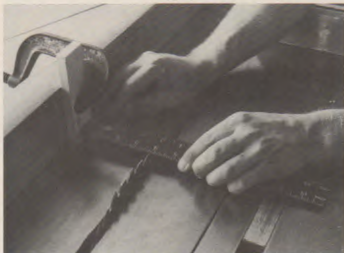
Fig. 21-16. A—Stop block clamped to the rip fence determines the length of parts cut to duplicate lengths. B—Set the blade-to-stop block distance with the block clamped to the fence near the blade. Guards are removed to show these procedures.
