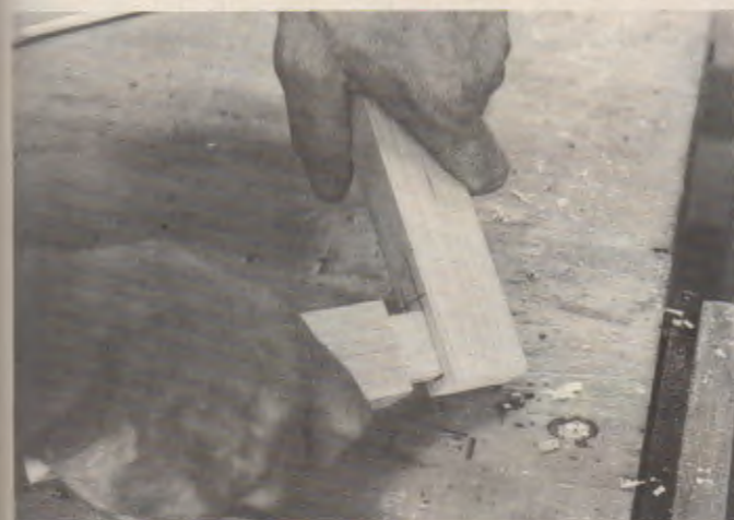
Fig. 29-45. Hand mortising. A—After drilling several holes, chisel out the mortise. B—After making shoulder and cheek cuts with a backsaw or dovetail saw, chisel the tenon square. C—Assembling the joint.
