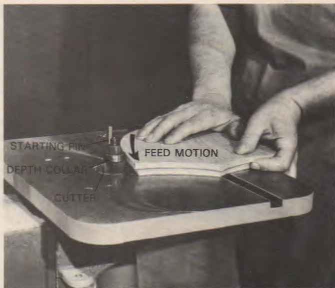
Fig. 26-15. A collar and starting pin are installed for shaping irregular surfaces. The guard has been removed to show the operation. (Delta)
