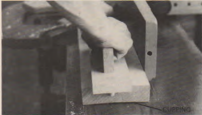
Fig. 23-7. The concave side of a cupped face should be placed down.
