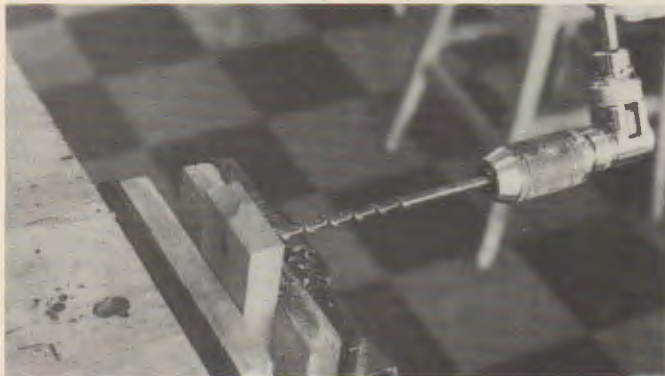
Fig. 25-37. Two attachments for determining depth. A—Depth gauge. (Stanley) B—Drill stop. (General Hardware)
