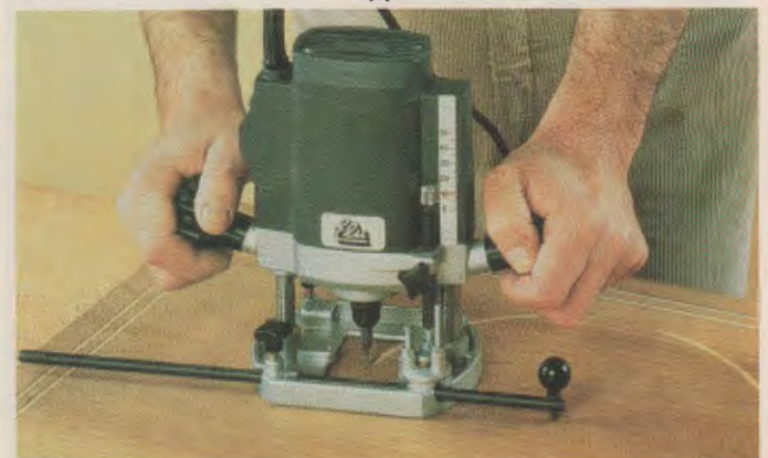
Fig. 26-43. Router guides provided by the manufacturer. A—Fence. (Makita) B—Circle guide. (Black & Decker)
