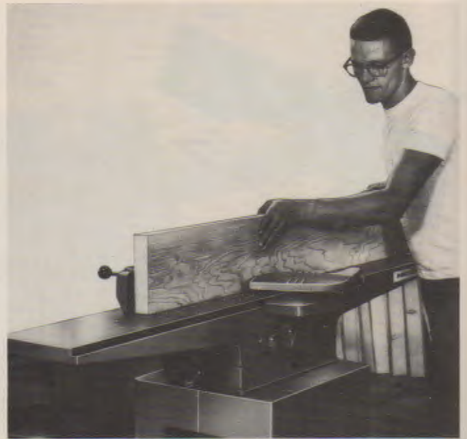
Fig. 23-8. Edge-jointing. Your left hand holds the workpiece against the fence. Your right hand does the feeding. (Delta)
