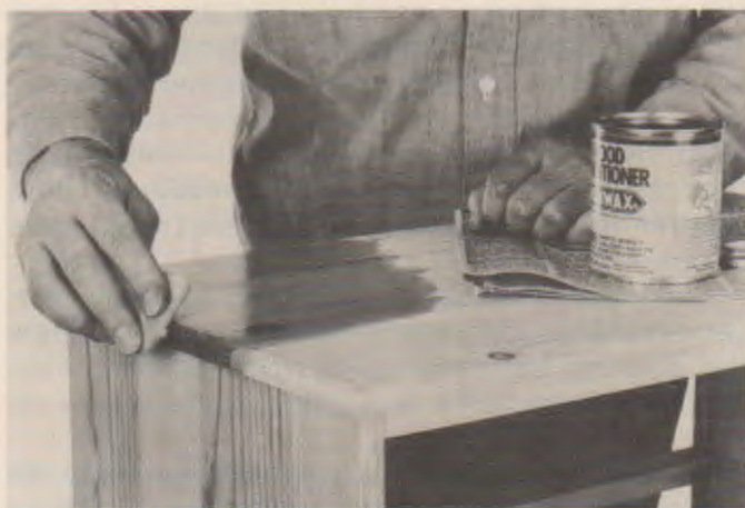
Fig. 47-3. "Wood conditioner" is just one name given to washcoating products. (Minwax)
