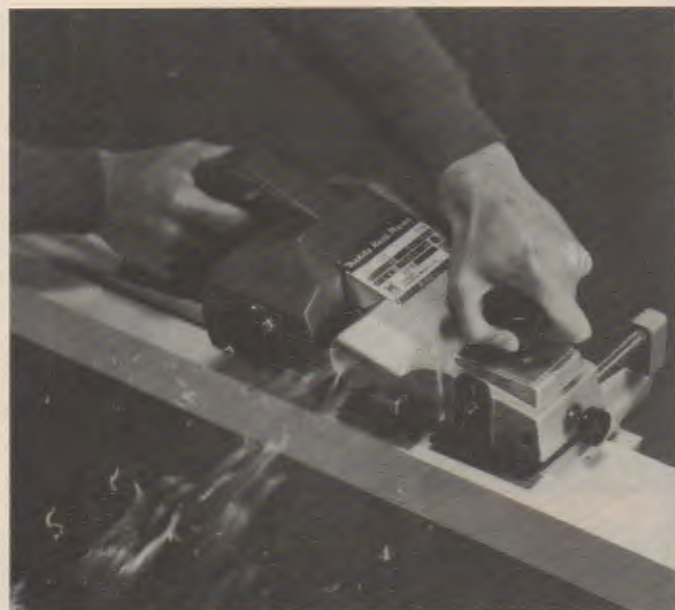
Fig. 6-8. A portable power planer works well for narrow faces and edges. (Makita U.S.A., Inc.)
