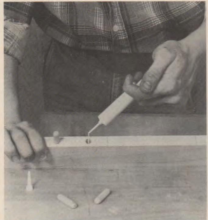
Fig. 32-17. A—Apply adhesive with a stick. (Franklin International) B—In holes, use a glue syringe. (Shopsmith, Inc.)
