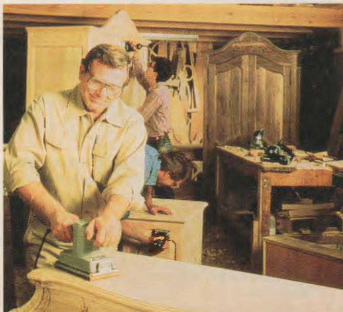
Fig. 31-1. This assembled product is abraded with an in-line sander before applying finish. (Porter-Cable Corp.)
