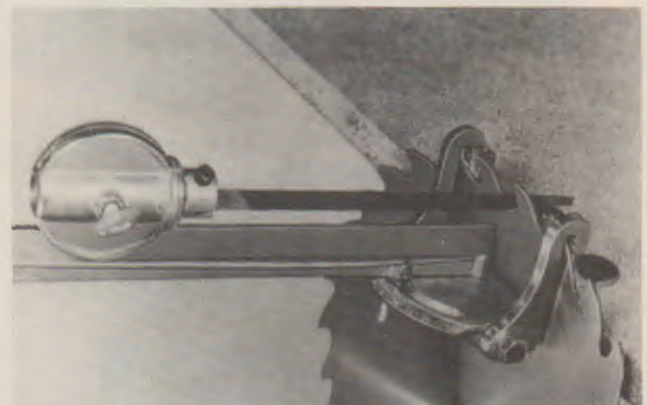
Fig. 21-64. This saw filer is adjustable for various tooth angles. (Brookstone)
