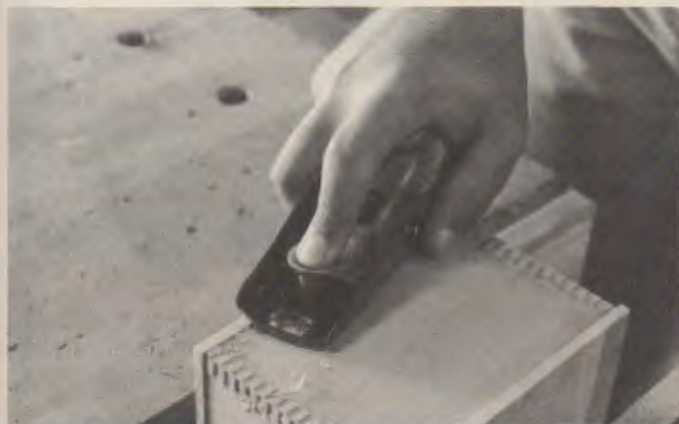
Fig. 24-8. Hold a block plane in the palm of your hand.
