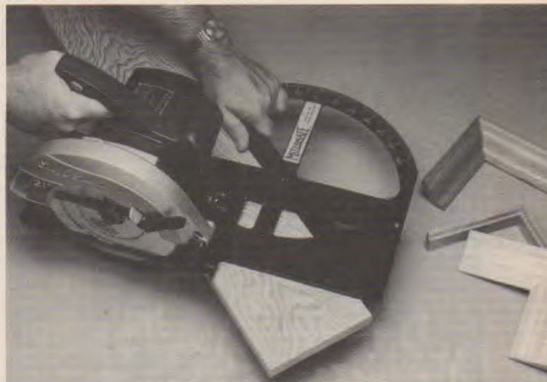
Fig. 22-22. This circular saw accessory allows you to cut angles. (Matrix Enterprises)
