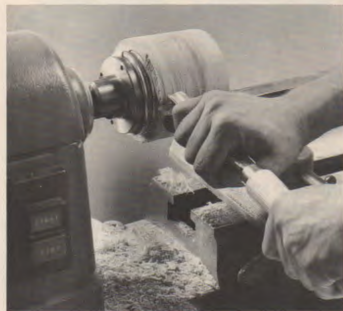
Fig. 27-43. A gouge quickly turns the edge to diameter. The guard was removed to show the operation. (Delta)
