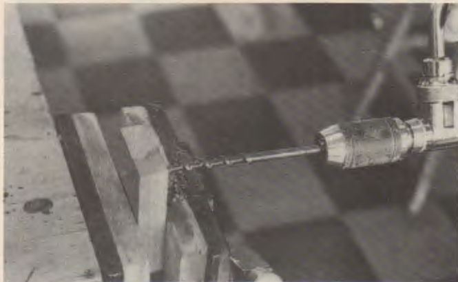
Fig. 25-35. Back up your workpiece when drilling a through hole. Failure to do so may tear the wood.
