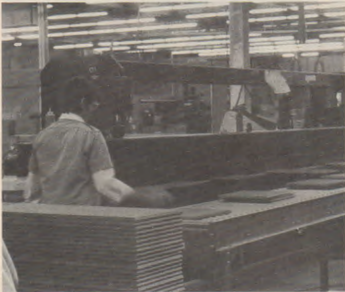
Fig. 52-15. Edge banding particleboard panels with plastic laminate. (Riviera Cabinets)
