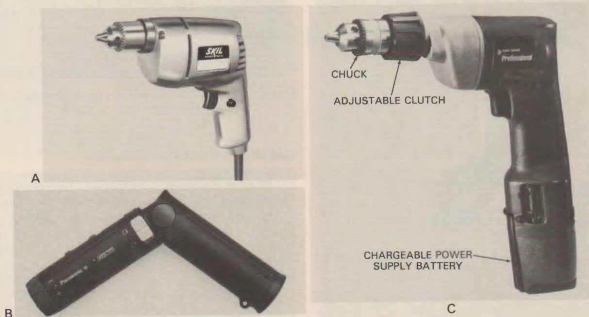
Fig. 25-28. A—Portable power drill. (Skil) B—Cordless drill and power screwdriver. It can bend to 90° angles. (Panasonic) C—This battery operated drill has an adjustable, five position clutch for matching drill torque to workpiece. This prevents it from stripping screws when using a screw bit. (Black & Decker)
