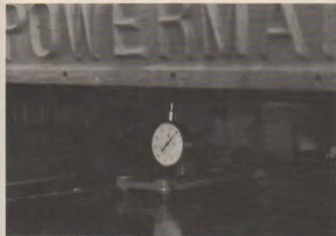
Fig. 23-33. Table and all roller adjustments are made using a dial indicator on a flat base.
