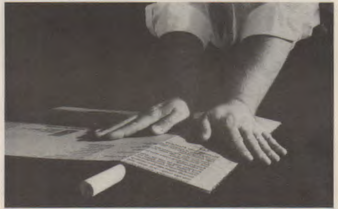
Fig. 15-24. Steps in fracturing plastic. Left. Score with a plastic cutter. Fracture by bending over a dowel rod. (Rohm and Haas)
