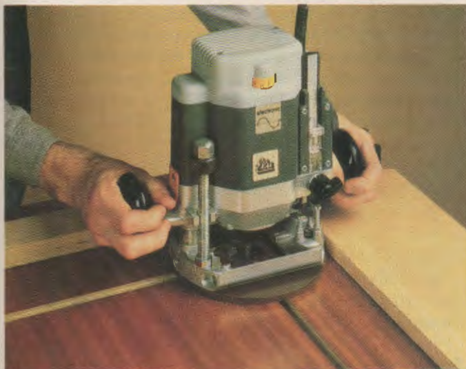
Fig. 26-41. The router base rides along the straight edge for grooving this door panel. (Black & Decker)
