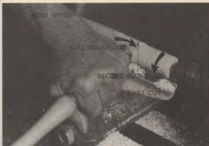
Fig. 27-24. Rough-turn 3 to 4 in. sections to bring the stock to a constant diameter. The guard was removed to show the operation.
