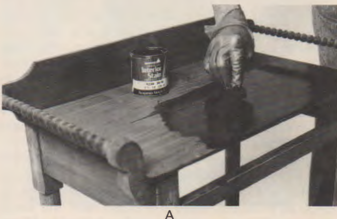
Fig. 47-6. Applying oil stains. A—Apply the stain with a small pad or brush. B—Wipe off the excess after the stain has had a chance to soak in. (Benjamin Moore)
