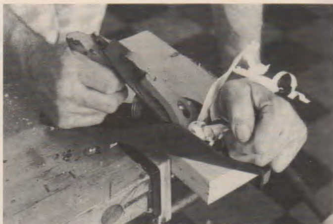
Fig. 24-6. Turn the plane at an angle for easier cutting. The shavings should be thin.
