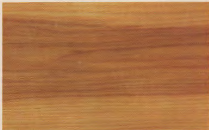
Fig. 12-18. Hickory is strong and elastic. It is valued for bent laminations, such as skis. (Fine Hardwood Veneer Assoc.)
