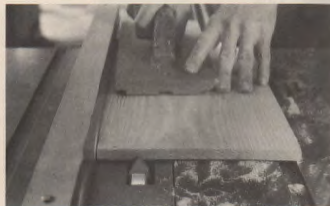
Fig. 26-34. Shaping a face on the table saw.
