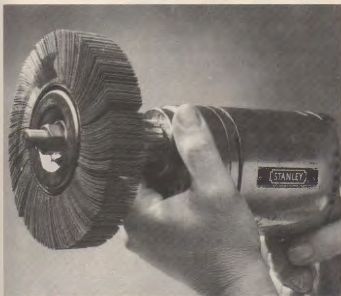
Fig. 30-16. Flap wheels mounted on a drill will smooth in tight corners and around contours. (Norton)
