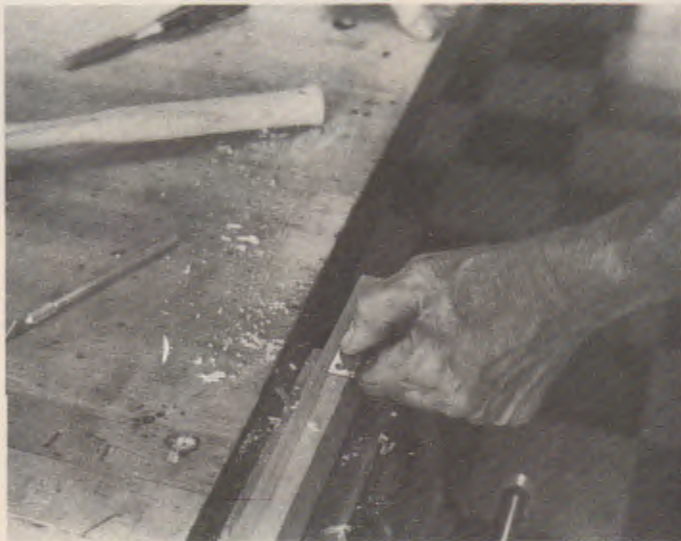
Fig. 41-7. Fastening a butt hinge. A—Cut around the hinge leaf with a knife. B—Cut on the line with a chisel. C—Chisel out the pocket. D—Check the hinge fit. E—Drill the pilot holes and install the hinge.
