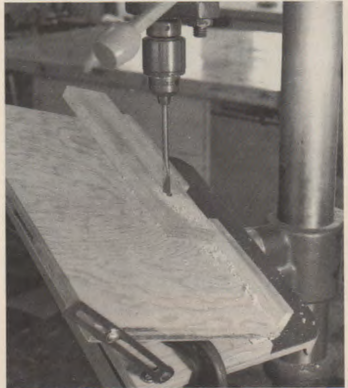
Fig. 25-45. Both the jig and table are tilted for compound angles.
