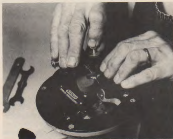
Fig. 26-64. This grinding jig allows you to sharpen router bits. (Stanley)
