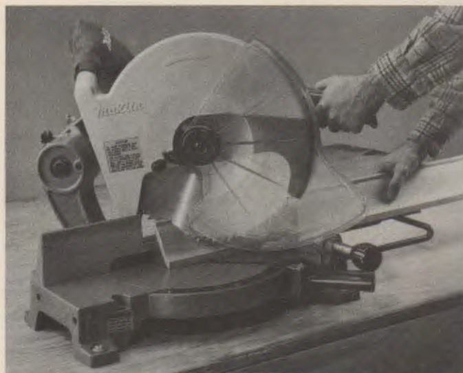
Fig. 22-24. Power miter box set to cut moulding. (Makita)
