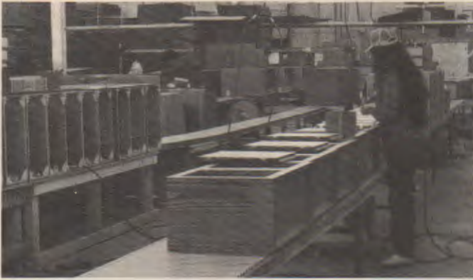
Fig. 52-24. The prefinished doors and catches are installed last on laminate covered cabinets. (Formitex)
