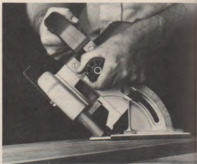
Fig. 22-19. It is difficult to align with a marked line when beveling. (Milwaukee Electric Tool Corp.)
