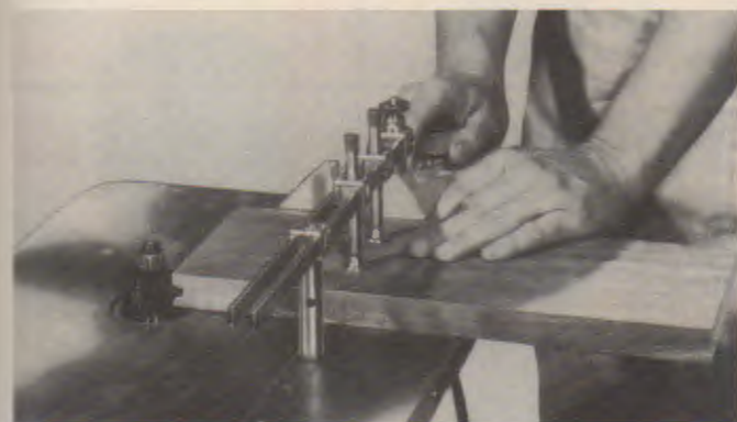
Fig. 26-4. Narrow workpieces are held in a miter gauge. The guard has been removed to show the operation. (Delta)
