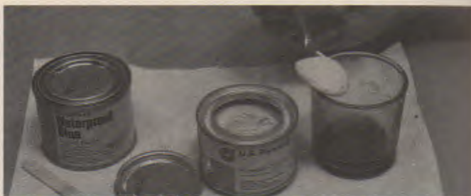
Fig. 32-7. Measure proportions of resin and catalyst in two part adhesives accurately. (Franklin International)
