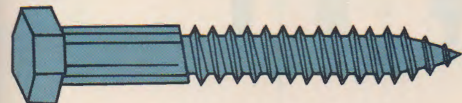
Fig. 16-36. Lag screws may be up to 6 in. long. Use them where strength is essential.
