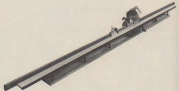
Fig. 28-2. Longer stock can be cut on the radial arm saw with table attachments. (Biesemeyer)
