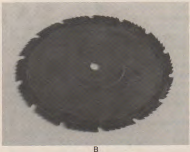
Fig. 21-55. A—Set hollow ground blades high. The guard has been removed to show the operation. B—Resin buildup (dark material) results from sawing only on the rim of a hollow ground blade.
