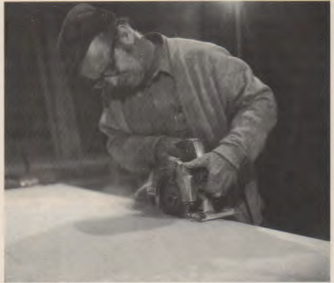
Fig. 15-34. Plastic tops are cut and shaped with conventional woodworking tools. Use carbide tipped saw blades and router bits. (DuPont)
