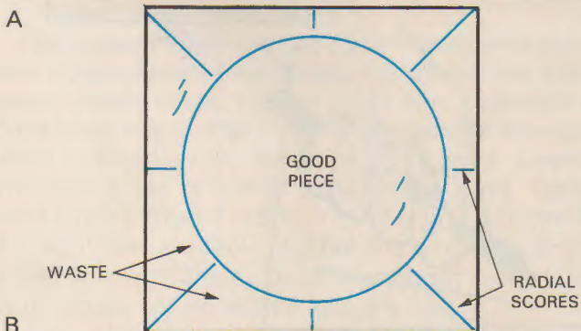
Fig. 15-7. Cutting circles. A—The swivel knob has a rubber bottom which keeps the cutter from moving while you score the glass. (Brookstone Co.) B—Radial scores help separate the waste material, making it easier to remove the glass circle.
