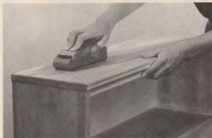
Fig. 31-5. Sanding along the wood grain makes abrasive scratch marks less visible. (Norton Co.)
