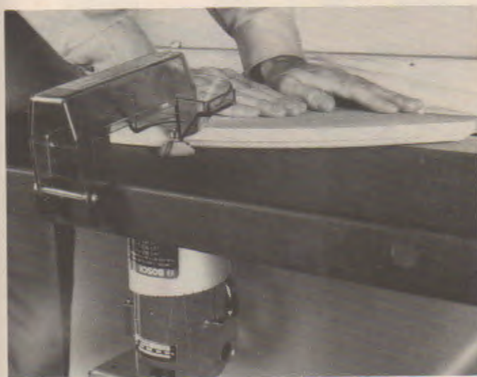
Fig. 26-52. A—Mounting a router under a commercial router table. B—The router is then used like a shaper. (Bosch)
