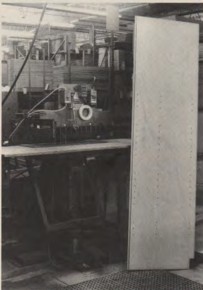
Fig. 52-7. Multiple spindle drill press creates rows of holes for 32 mm cabinet construction. (Riviera Cabinets)
