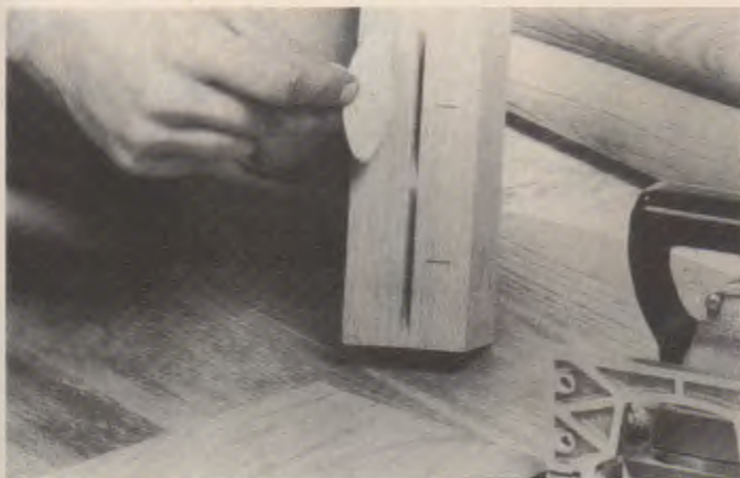
Fig. 40-11. Assembling the legs and apron pieces using plate joinery. A—Mark slot locations on the legs. B—Mark slot locations on the apron pieces. C—Cut the apron slots. D—Align the apron and leg to cut the leg slots. E—Put glue and a plate (biscuit) in both slots on one leg. F—Assemble the legs and apron on a flat surface. (Steiner-Lamello)
