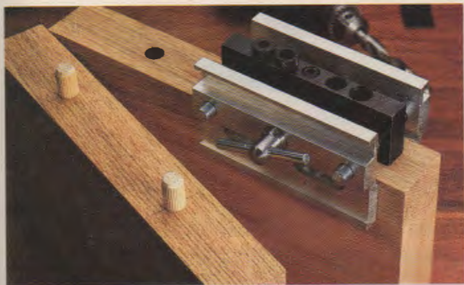
Fig. 28-13. Doweling jig centers the drill bit on the edge of material. (The Fine Tool Shops)
