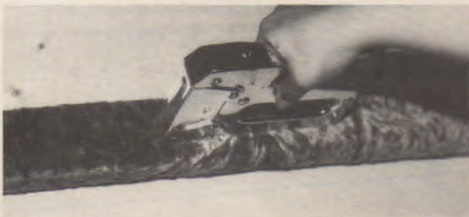
Fig. 16-14. Most staple guns use a spring-action handle for ease of operation.
