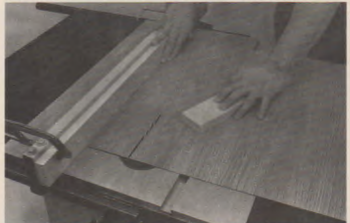
Fig. 36-3. Laminate can be cut with a number of tools. The saw teeth must enter the decorative side of the laminate on the cutting stroke. Guard was removed to show operation. (Franklin International)
