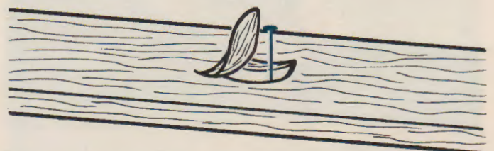
Fig. 16-12. Nails can be concealed under peeled-up shaving of wood. (National Retail Hardware Assoc.)
