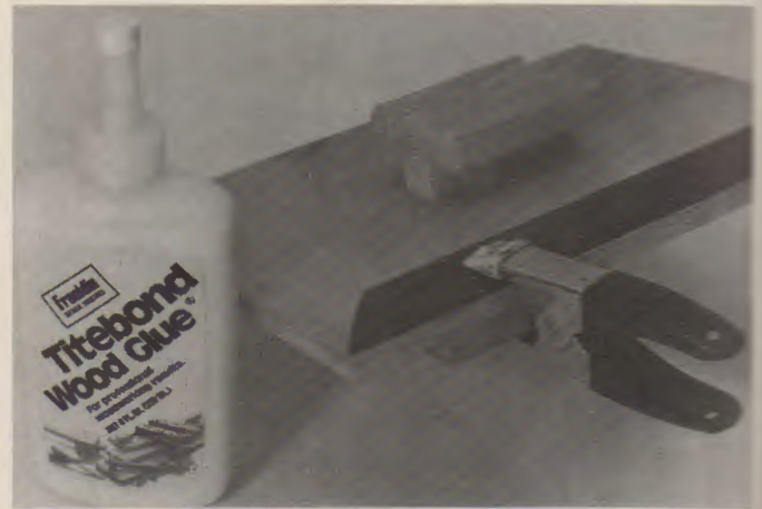
Fig. 33-1. Spring clamps work much like clothespins. (Franklin International)
