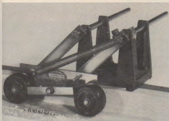
Fig. 28-4. Ripping guides keep material against the table and fence, and prevent kickback. The guard was removed to show the operation. (Fisher Hill Products)
