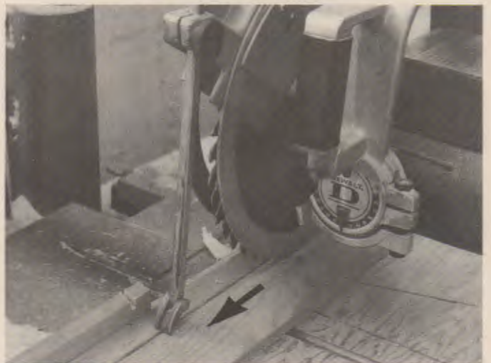
Fig. 21-27. Top. A stop positions stock for sawing multiple parts to length. (Black & Decker) Bottom. Make minor changes by turning the adjusting screw.
