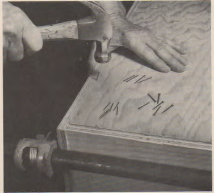
Fig. 16-3. While the glued cabinet assembly is still clamped, the 1/4 in. plywood cabinet back is attached with brads. The back keeps the assembly square. (American Plywood Assoc.)
