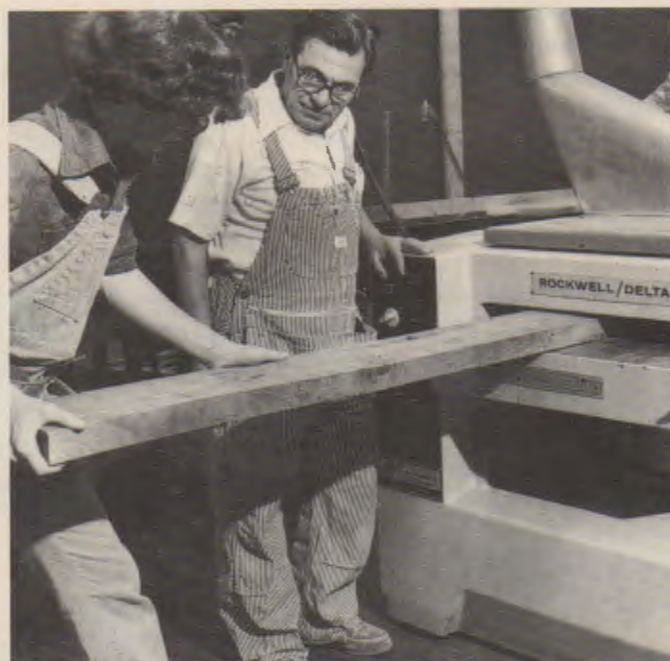
Fig. 23-12. Planers surface material to thickness after jointing the first face. (Delta)
