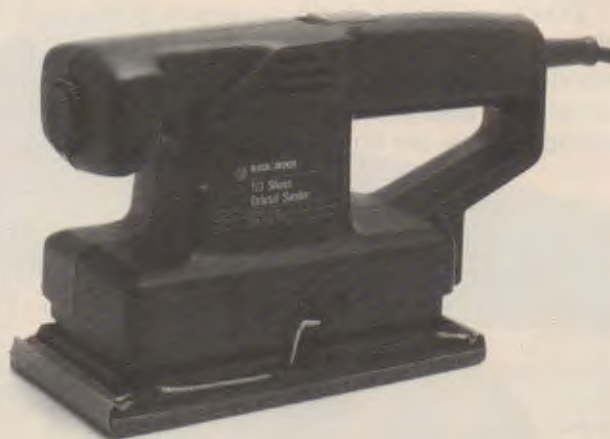
Fig. 30-11. Sheet abrasive is commonly used with portable orbital sanders. (Black and Decker)
