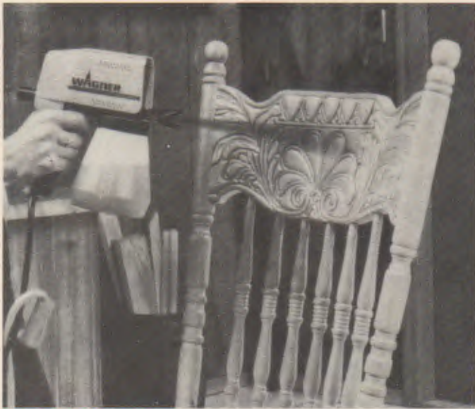
Fig. 46-27. Hold airless spray guns about 12 in. from the surface. (Wagner)
