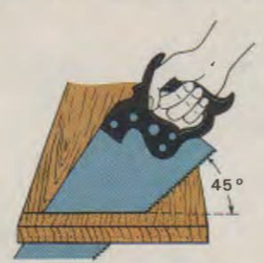
Fig. 22-11. Ripping should be done at a 60^\circ angle, while crosscutting is at a 45^\circ angle. (Porter)
