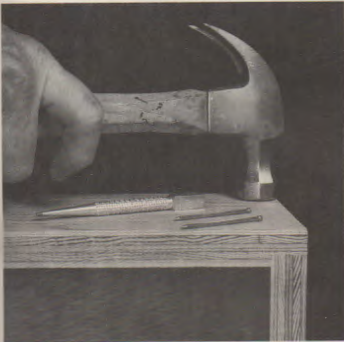
Fig. 16-3. While the glued cabinet assembly is still clamped, the 1/4 in. plywood cabinet back is attached with brads. The back keeps the assembly square. (American Plywood Assoc.)
