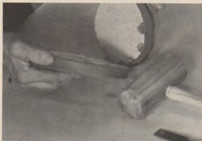
Fig. 27-41. Top. Screws enter the backup board but not the workpiece. Bottom. The backup board is separated from the workpiece with a mallet and chisel.
