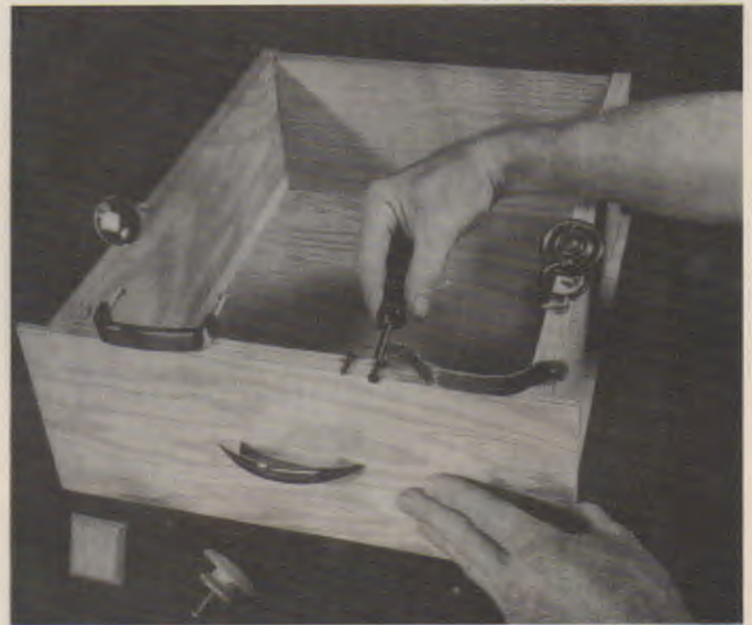
Fig. 17-5. Surface mount pulls and knobs are attached from the inside of the drawer. (American Plywood Assoc.)
