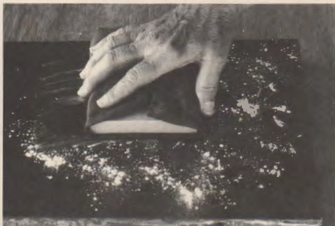
Fig. 48-19. Rubbing the surface with pumice stone creates sheen.
