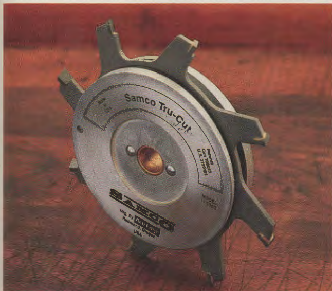
Fig. 29-8. Dado cutters. A—Adjustable dado cutter. (The Fine Tool Shops) B—Dado blades and chippers. (Delta)
