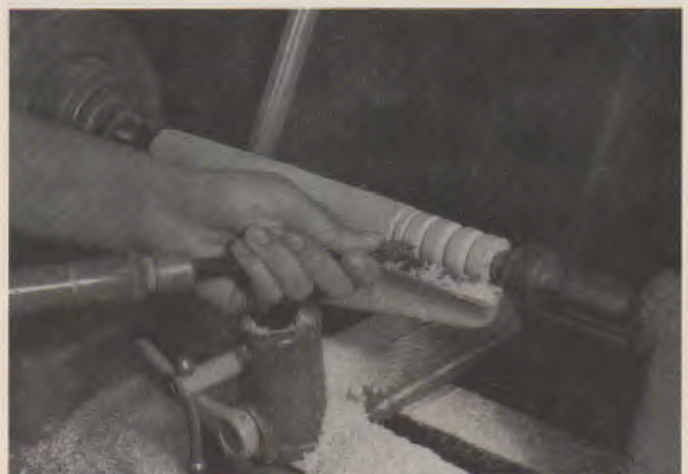
Fig. 27-12. Scraping V-grooves with the spear-point tool. The guard was removed to show the operation.
