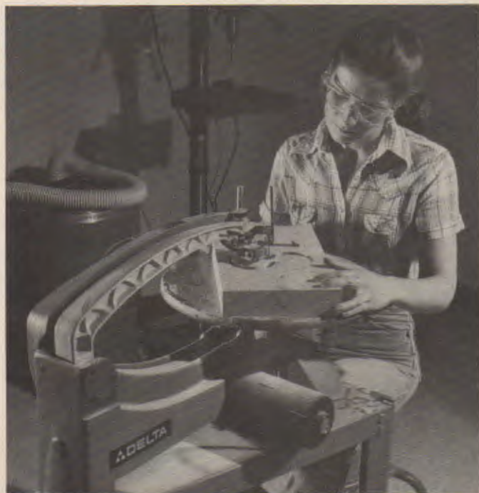
Fig. 21-52. Completing an interior cut. (Delta)
