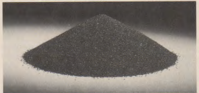
Fig. 30-2. Abrasive grains are the essential ingredient for making solid and coated abrasives. (Norton)
