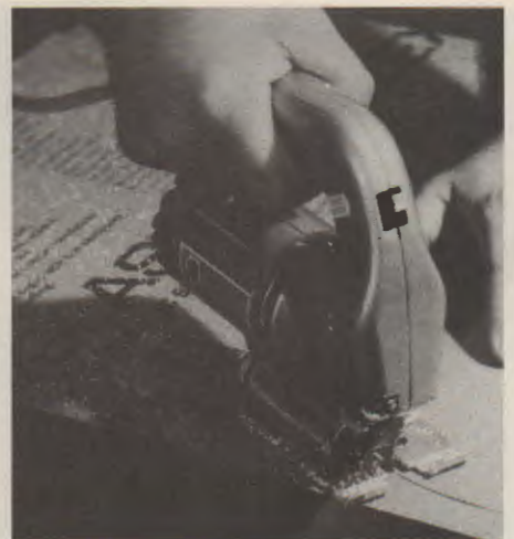
Fig. 15-25. Sawing plastic. Left. Circular sawing with a hollow ground blade for plastics. (The guard has been removed to show operation). Middle. Sawing straight lines with a saber saw using a clamped straightedge. Right. Saber sawing curves along a layout line. (Rohm and Haas)
