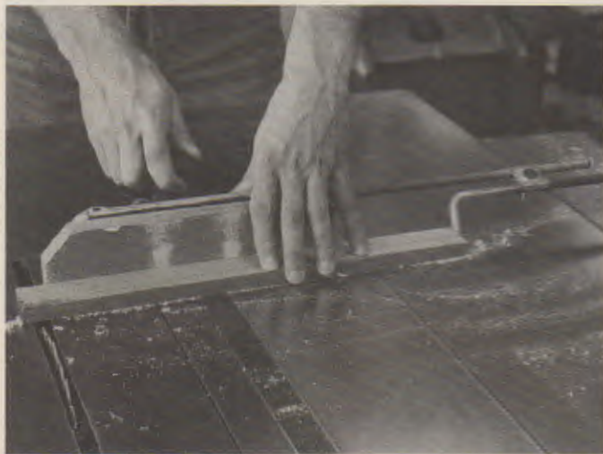
Fig. 21-15. Use a stop rod for cutting duplicate parts to length. The guard was taken off to show the operation.
