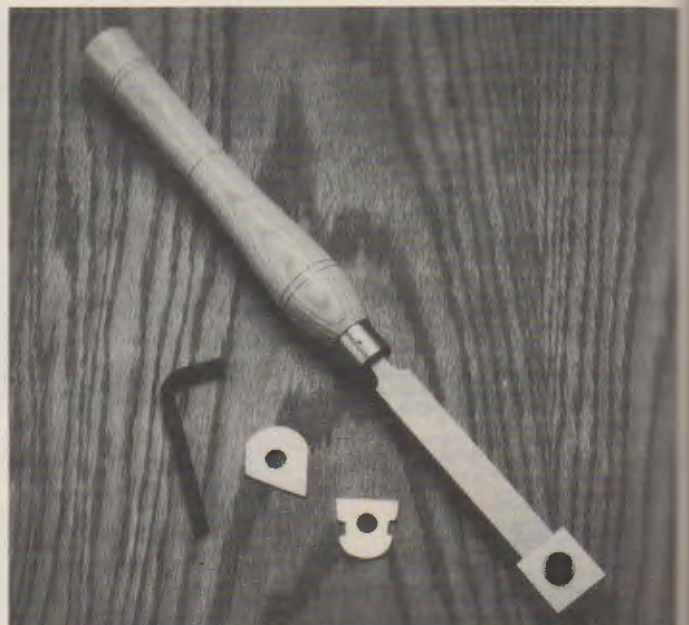
Fig. 27-14. Interchangeable cutters allow you to create additional contours. (Shopsmith)
