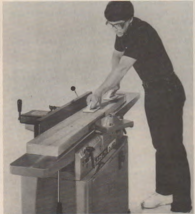
Fig. 23-1. Surface lumber square on jointers and planers. (Delta)
