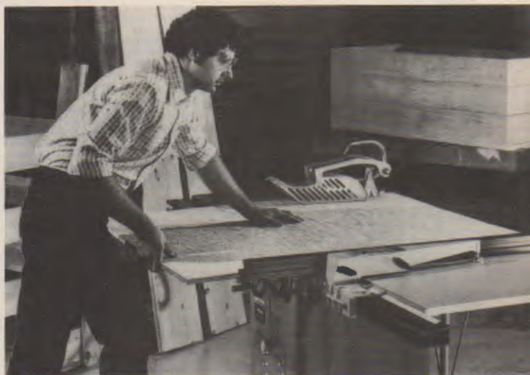
Fig. 1-8. Reducing sheets of plywood to component sizes with a table saw. (Delta)
