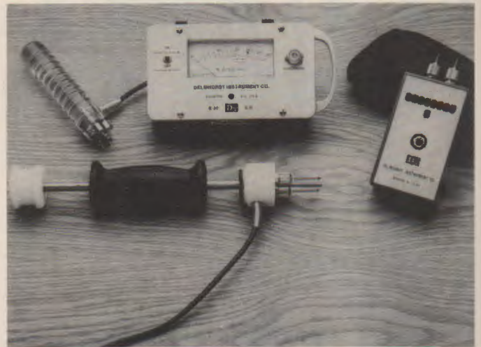
Fig. 10-9. Moisture content of wood can be determined by a moisture meter. Insert probes in the wood to obtain a reading. (Woodcraft)
