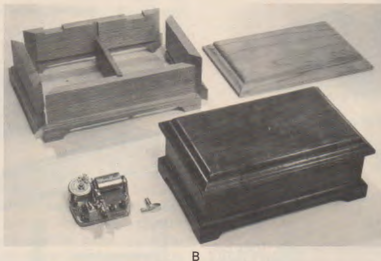
Fig. 38-5. A—Several alternative joints can be used on case goods. B—The corners of this jewelry case are mitered and the bottom is dadoed. (Craft Products)
