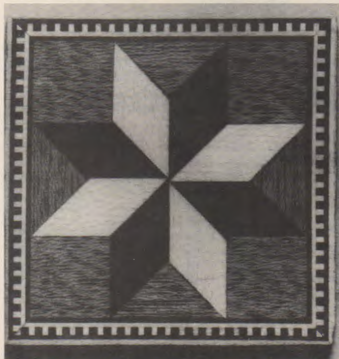
Fig. 35-14. The center shapes of this design show intarsia. The outer design consists of inlaid bandings. (The Woodworker's Store)
