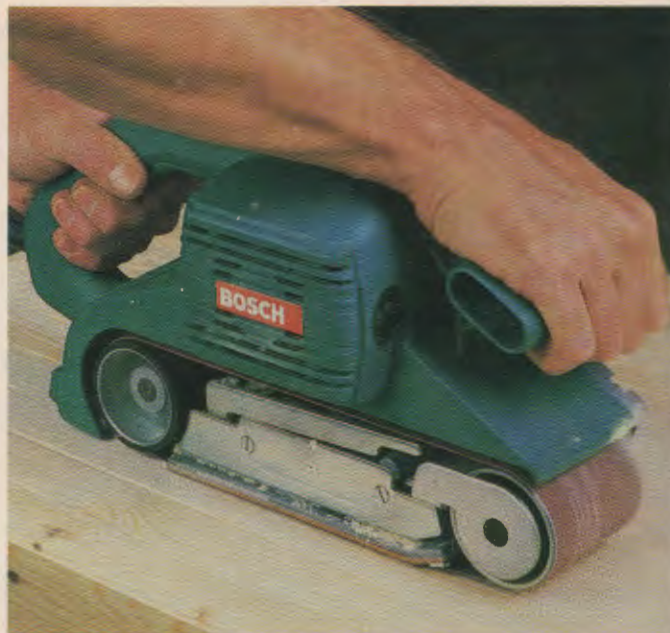
Fig. 6-12. Smoothing a surface with a portable belt sander. (Robert Bosch Power Tool Corp.)
