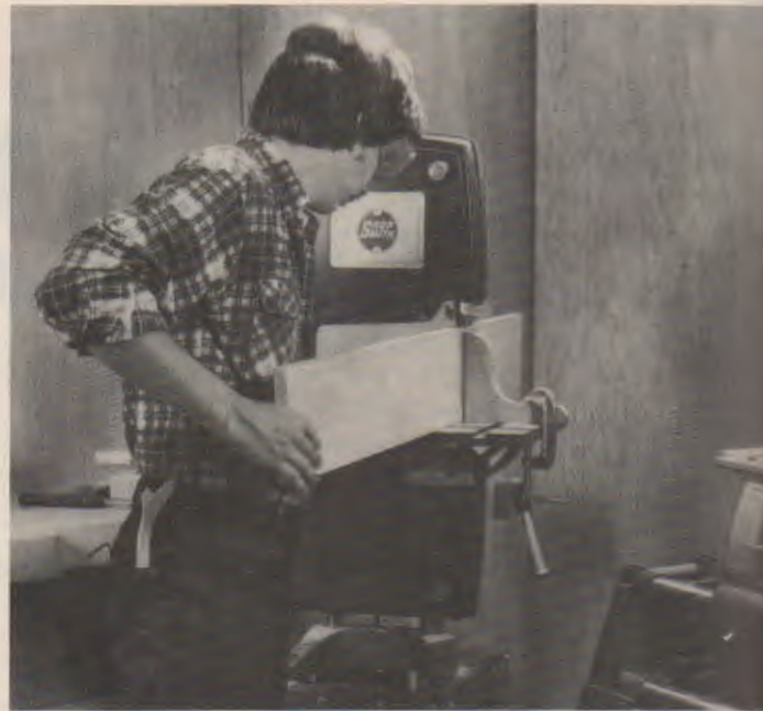
Fig. 18-2. This person has thoroughly planned the sawing operation. He has made a jig for stability and has a push stick. Safety glass and the proper stance further reduce the chance of injury. (Shopsmith, Inc.)
