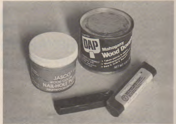
Fig. 45-4. Common repair materials include wood putty, wood dough, stick shellac, and wax stick putty.
