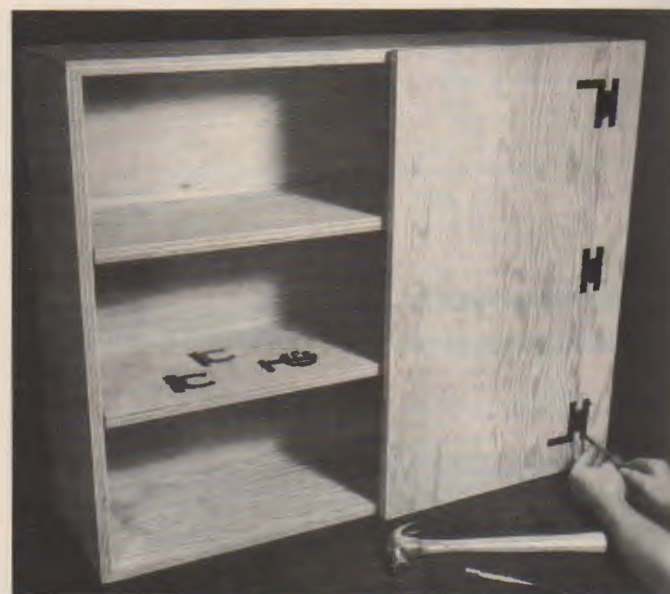
Fig. 17-19. "H" and "HL" surface hinges are used on flush and some lip front cabinets. (American Plywood Assoc.)
