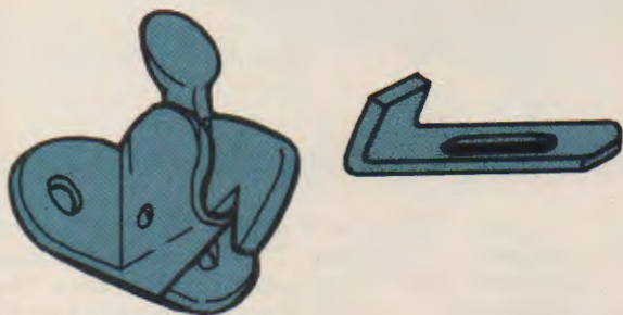
Fig. 17-33. An elbow catch hooks onto a bent strike. (The Woodworker's Store)
