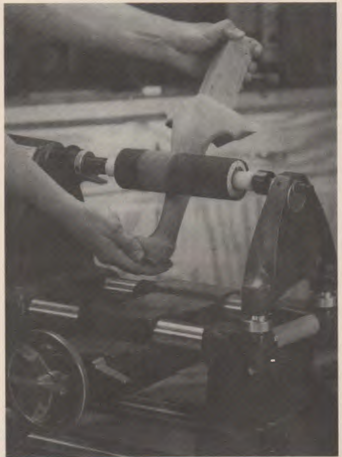
Fig. 40-25. A—Marking stock using the pattern. B—Cut the first profile shape. C—Tape the waste back to the leg. D—The leg after cutting the second profile and removing the waste. E—Smoothing the final leg shape. (Shopsmith)
