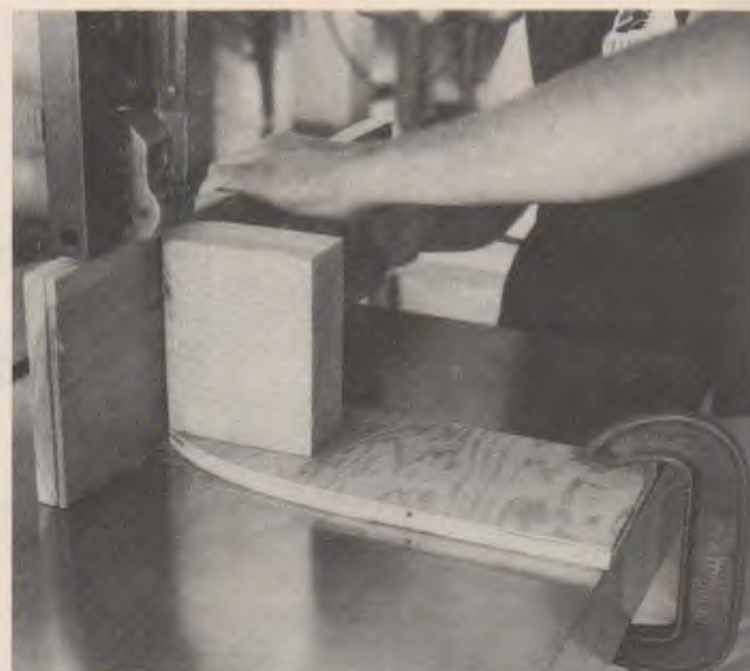
Fig. 21-47. Resawing on the band saw is a one-pass operation. Hold material firmly against a rounded auxiliary fence.
