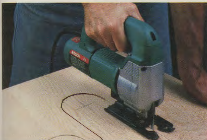
Fig. 22-1. Portable power tools, such as this saber saw, are often an excellent alternative to stationary power tools. (Robert Bosch Power Tool Corp.)
