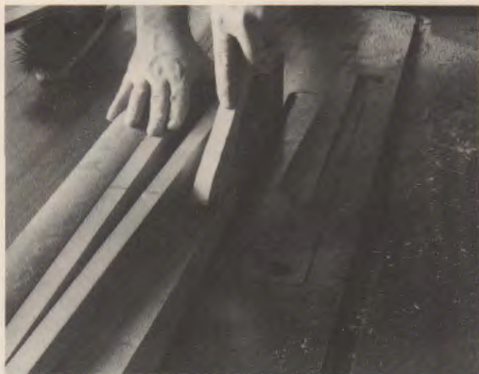
Fig. 40-18. Make a taper jig to cut tapered legs. The guard was removed to show the operation.
