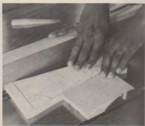
Fig. 40-33. A—Four-sided plinth assembled with compound miter joints. B—Sawing pass one with the five degree taper guide and with the blade at 44.75 degrees. C—Sawing pass two using the 10 degree taper guide. The guard was removed to show the operation.
