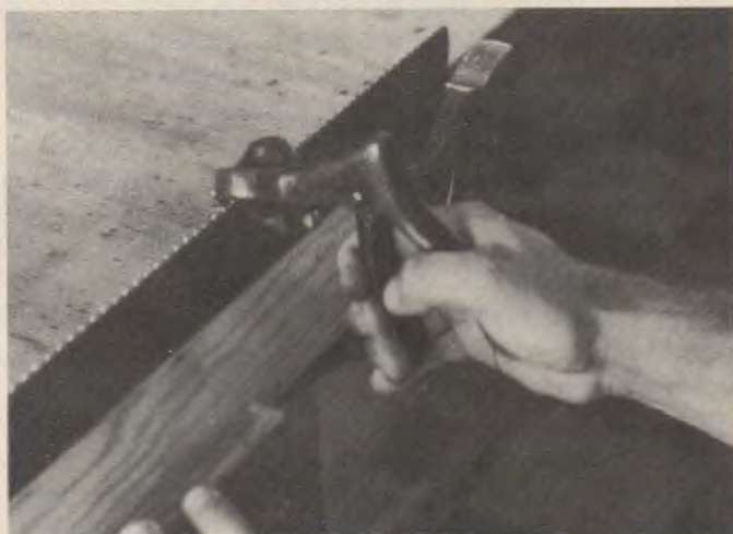
Fig. 22-33. A—Adjust the TPI on the setter. (Stanley) B—Place the saw set over the teeth and squeeze the handle.
