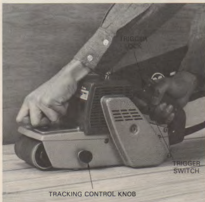
Fig. 31-23. Move the belt sander in short overlapping strokes. Check the tracking for proper adjustment before and while using the tool. (Makita U.S.A., Inc.)
