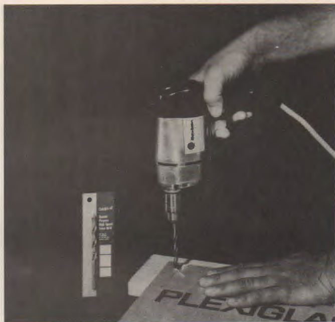
Fig. 15-26. Mark centerlines for drilling on protective paper cover. Place a board under the plastic while drilling. (Rohm and Haas)
