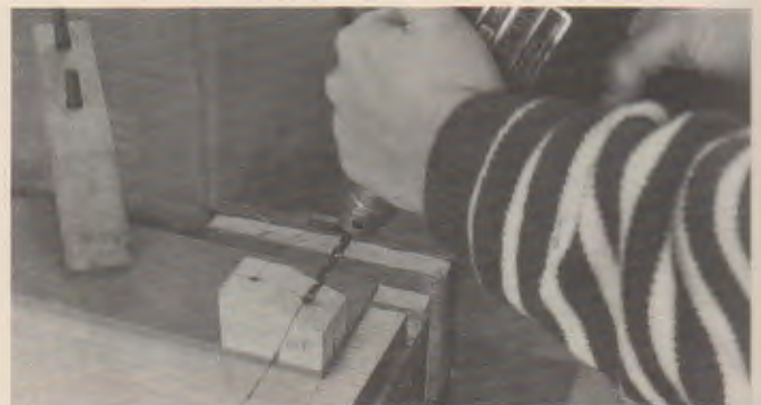
Fig. 25-38. Angled holes can be accurately drilled with a jig.
