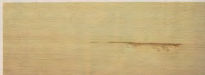
Fig. 11-12. Bark pockets are formed when bark cells are enclosed during growth. (Western Wood Products Assoc.)
