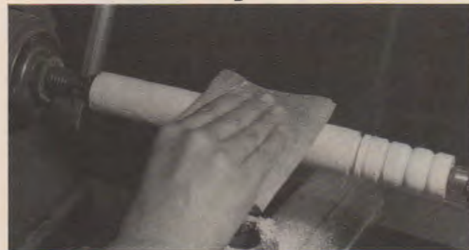
Fig. 27-48. A—Apply abrasive paper under the rotating workpiece to remove tool marks. The guard was removed to show the operation. B—Abrasive cord for sanding detail. (Woodworker's Supply) C—Remove circular scratches by sanding the workpiece along the grain. Do not have the lathe on for this operation.
