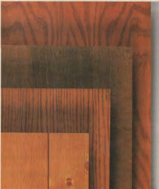
Fig. 13-14. Hardwood plywood is fabricated with hardwood face veneers for use where appearance is important. (Georgia-Pacific Corp.)
