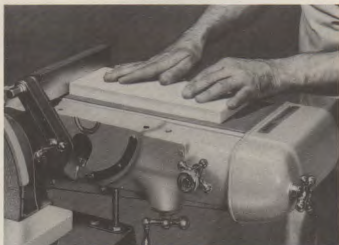
Fig. 31-9. Tilt the belt sander table for convenience. A—Smoothing miter cuts. B—Smoothing surfaces. The table keeps your work positioned on the abrasive. (Delta International Machinery Corp.)
