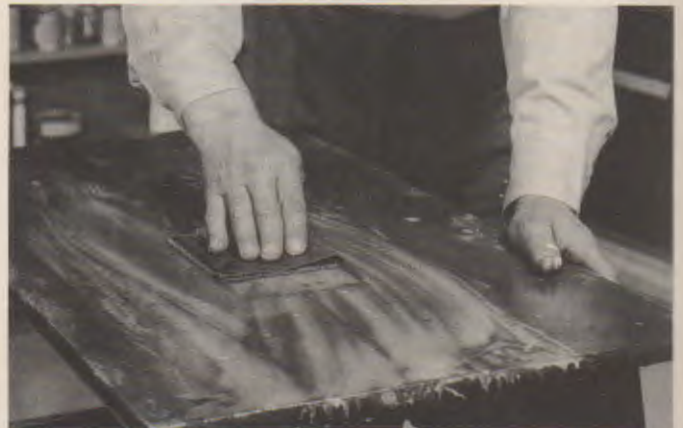
Fig. 48-18. After the final film of built-up lacquer or enamel topcoating, smooth the surface with 400 grit wet-or-dry silicon carbide abrasive and water. (Norton)
