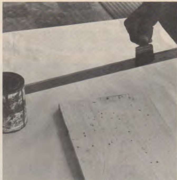
Fig. 45-14. Simulated distressing caused by tapping a brush dipped in enamel against a scrap board, splattering finish onto the surface.
