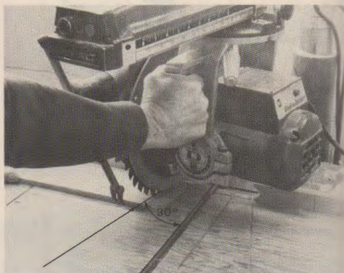
Fig. 21-26. Crosscutting at 30° with a radial arm saw.
