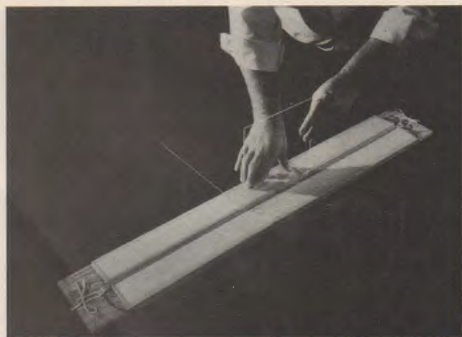
Fig. 15-27. This electric strip heater provides the correct amount of temperature for thermoforming acrylic plastic. (Rohm and Haas)
