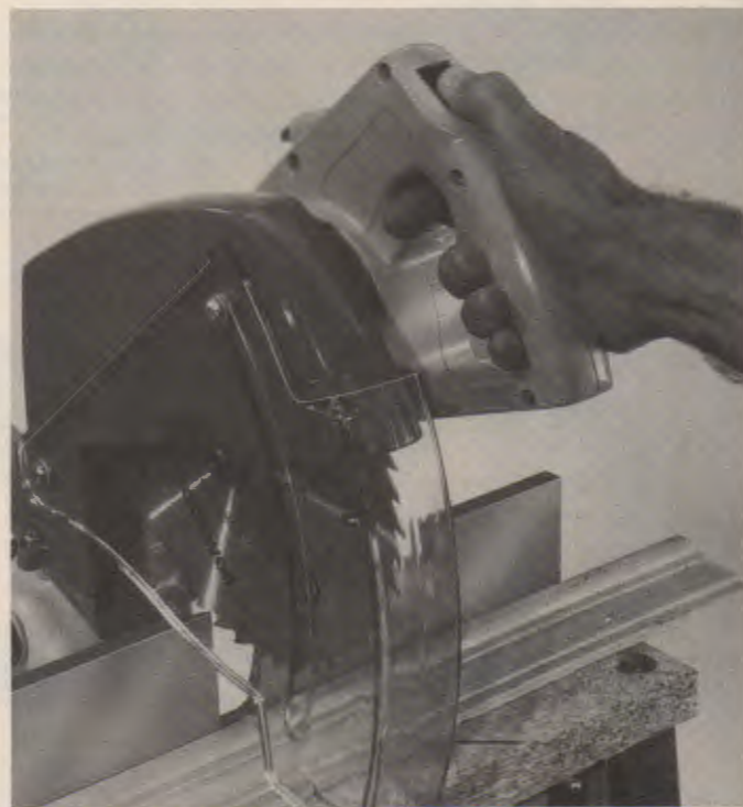
Fig. 6-4. Point-of-operation guards protect you from areas where the cutter contacts the workpiece. (Rockwell International)
