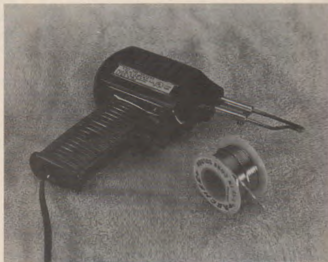
Fig. 15-18. A soldering gun or iron melts the solder to bond the lead came.
