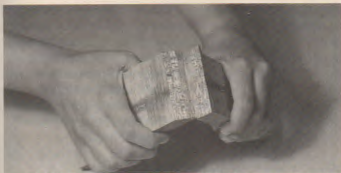
Fig. 32-3. Shear test on wood glue bonds show that glue can be stronger than the wood itself.
