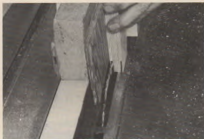
Fig. 29-40. Making shoulder cuts.
