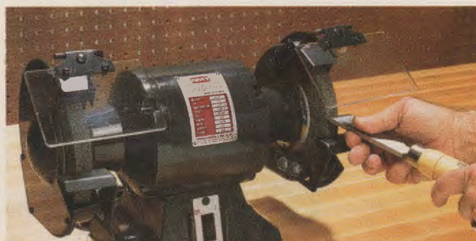
Fig. 30-18. Grinding wheels are solid bonded abrasive wheels. (American Machine and Tool Co.)
