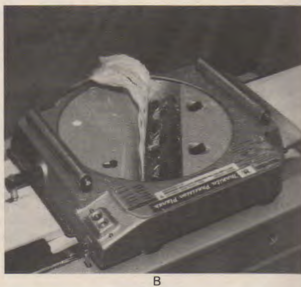
Fig. 23-17. A—Stationary cutterhead planer. B—Material is removed in long continuous chips. (Makita)
