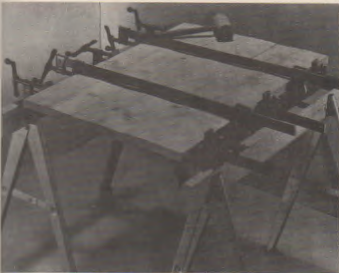
Fig. 33-24. Alternate bar clamps on top and bottom of assembly. Use a mallet to position boards which slip out of place. (Franklin International)
