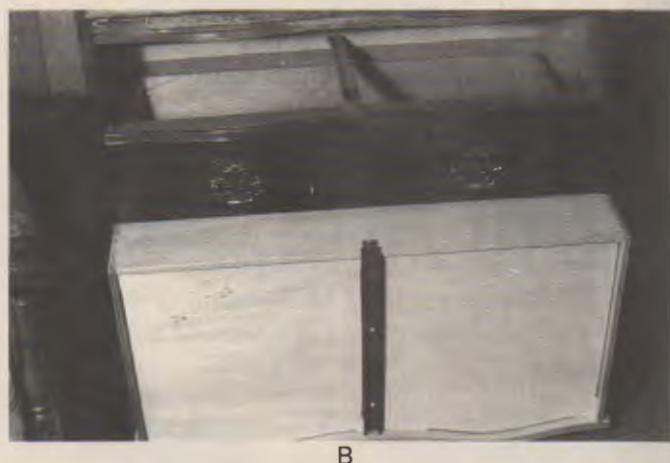
Fig. 42-20. Web frame construction provides drawer support.
