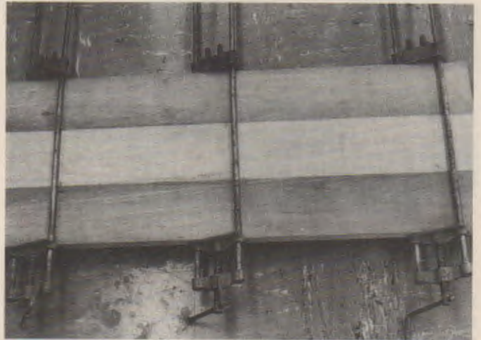
Fig. 33-26. Double bar clamps align the boards while clamping.
