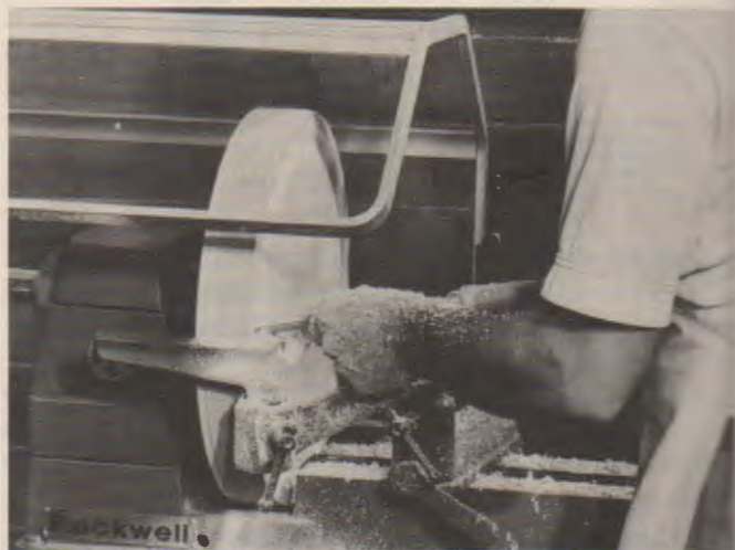
Fig. 27-45. Both the face and edge can be turned without having to reposition a right angle tool rest. (Delta)
