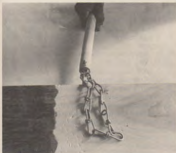
Fig. 45-13. Actual surface distressing with a length of chain. Notice the distressed effect once stain is added.
