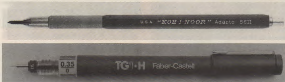
Fig. 9-5. Leadholders. Top. Thick leads must be sharpened. (Hearlily & Co.) Bottom. Thin leads maintain a fine line. (Utley)
