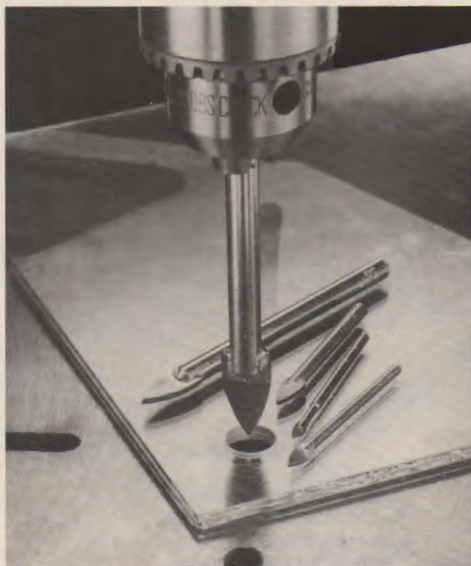
Fig. 15-13. A glass drill has a spearlike point. It drills by scraping the glass rather than cutting it. (Brookstone Co.)
