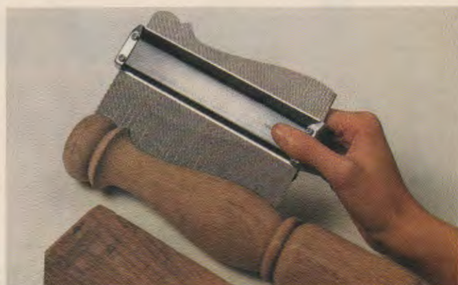
Fig. 20-26. The template former conforms to the shape of the piece to be copied. (The Fine Tool Shops)
