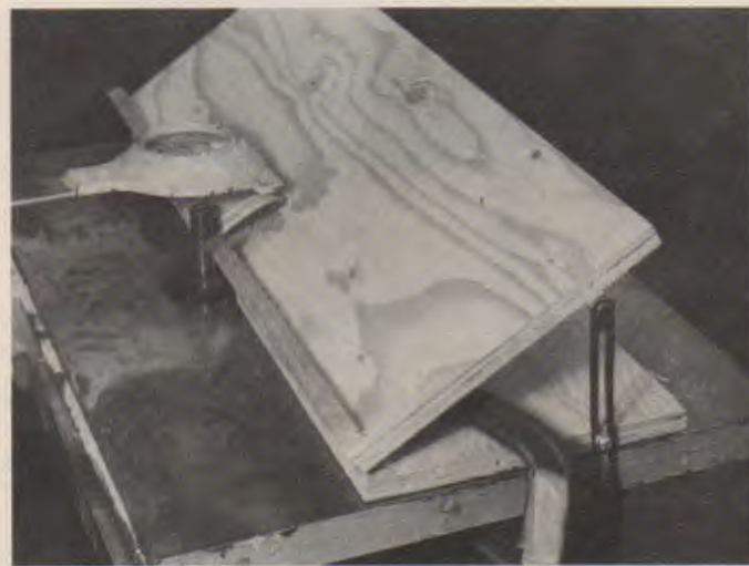
Fig. 26-17. Guiding the workpiece with a template.
