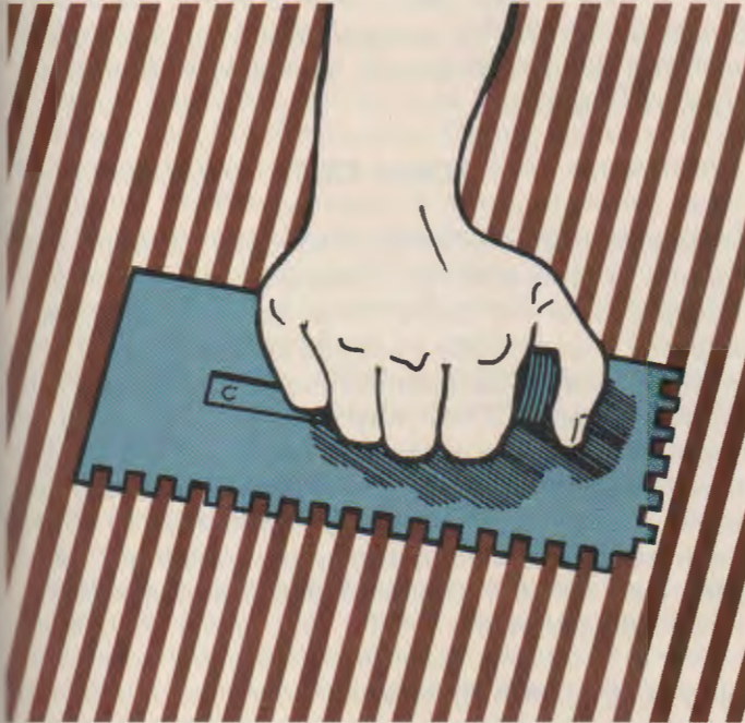
Fig. 15-37. A notched trowel spreads mastic evenly.
