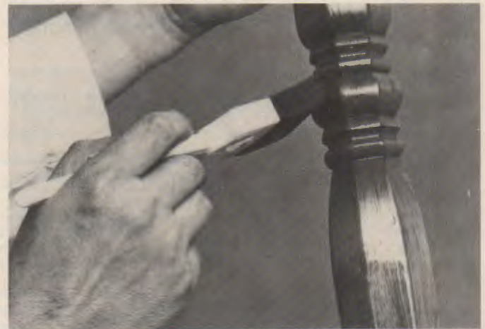
Fig. 46-30. Wiping on a finish. A—Cloth pad. B—Using an ear swab. (Minwax) C—Foam brush. (Carver-Tripp)
