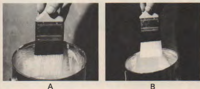
Fig. 46-2. A—Dip brush bristles only halfway into the finish. B—Tap, do not rub, the brush on the container.
