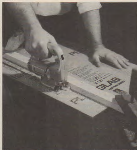
Fig. 15-25. Sawing plastic. Left. Circular sawing with a hollow ground blade for plastics. (The guard has been removed to show operation). Middle. Sawing straight lines with a saber saw using a clamped straightedge. Right. Saber sawing curves along a layout line. (Rohm and Haas)
