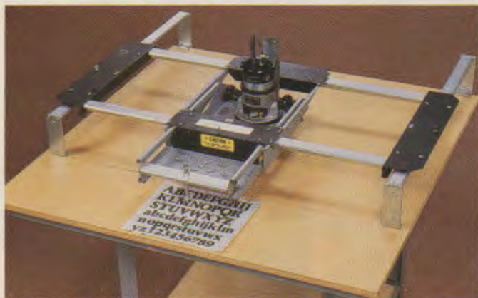
Fig. 28-10. Frame guide to rout letters. (Woodworker's Supply of New Mexico)
