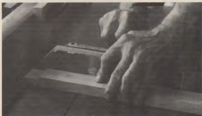
Fig. 29-44. Miter tenons if they meet in the component. (Delta)
