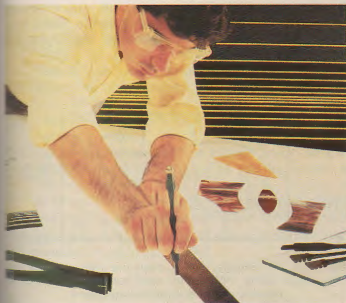
Fig. 15-4. Glass is scored with a glass cutter. A straightedge serves as a guide for scoring straight lines. (The Fletcher-Terry Co.)
