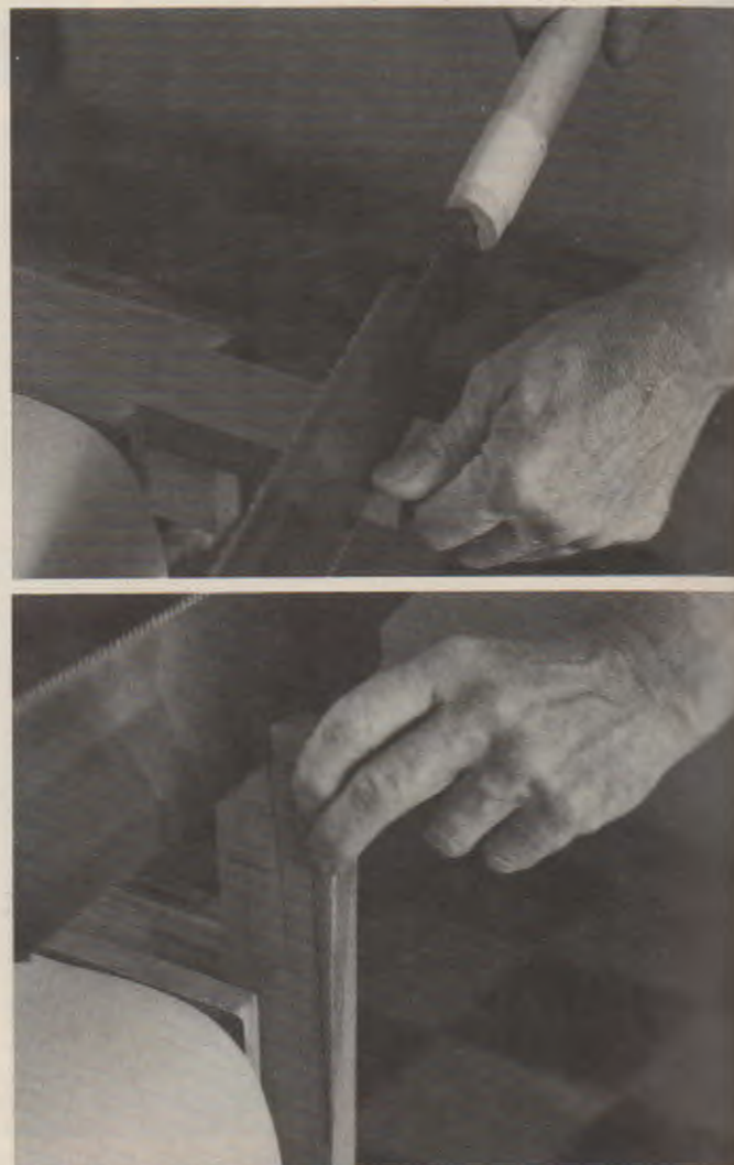
Fig. 22-5. The pull-stroke combination saw can be used for both crosscutting and ripping.
