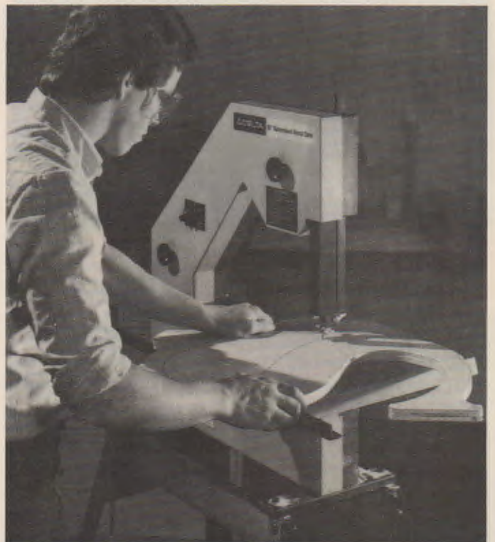
Fig. 21-39. With large, curved workpieces, first cut away as much waste as possible to prevent it from hitting the machine frame. (Delta)
