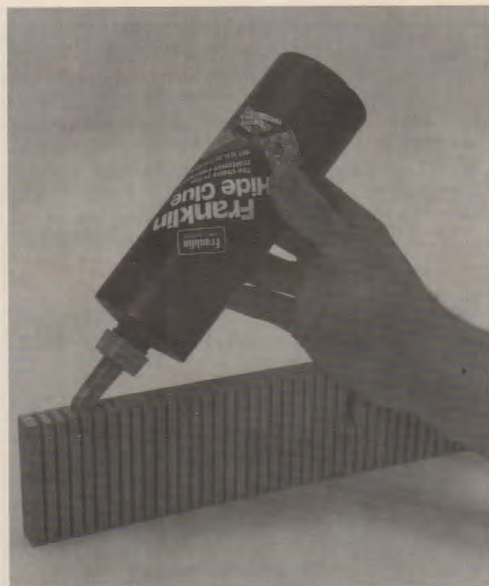
Fig. 32-5. Liquid hide glue being applied directly from the plastic container. (Franklin International)
