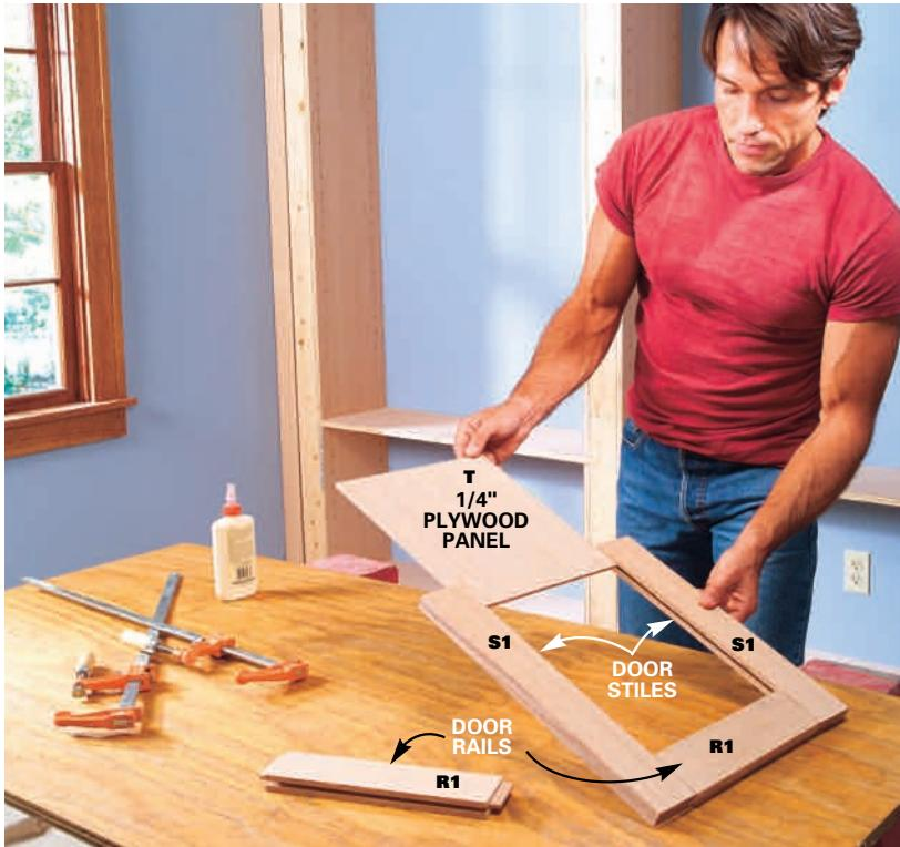
**13 ASSEMBLE** the doors as shown. First, glue the tenons of the top rail into the grooves of the stiles, then slip the plywood panel in place. No need to glue the plywood; just let it float in the grooves. The plywood should be 1/8 in. narrower and shorter than the distance from groove to groove to ensure a foolproof assembly. Clamp the doors, making sure they lie flat. Clamps can pull the frames and warp them if you're not careful.
