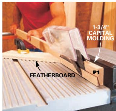
**9 SET** your saw to 20 degrees and taper the upper capital molding and the top shelf face molding (Fig. A). Make the front shelf molding in the same manner, only cut it from 1-1/2 in. strips.
