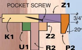
**21** FASTEN the front top extensions with your pocket hole jig. Nail a 3/4-in. x 3/4-in. strip to the top of the face frame and glue the extension to this for added support.
