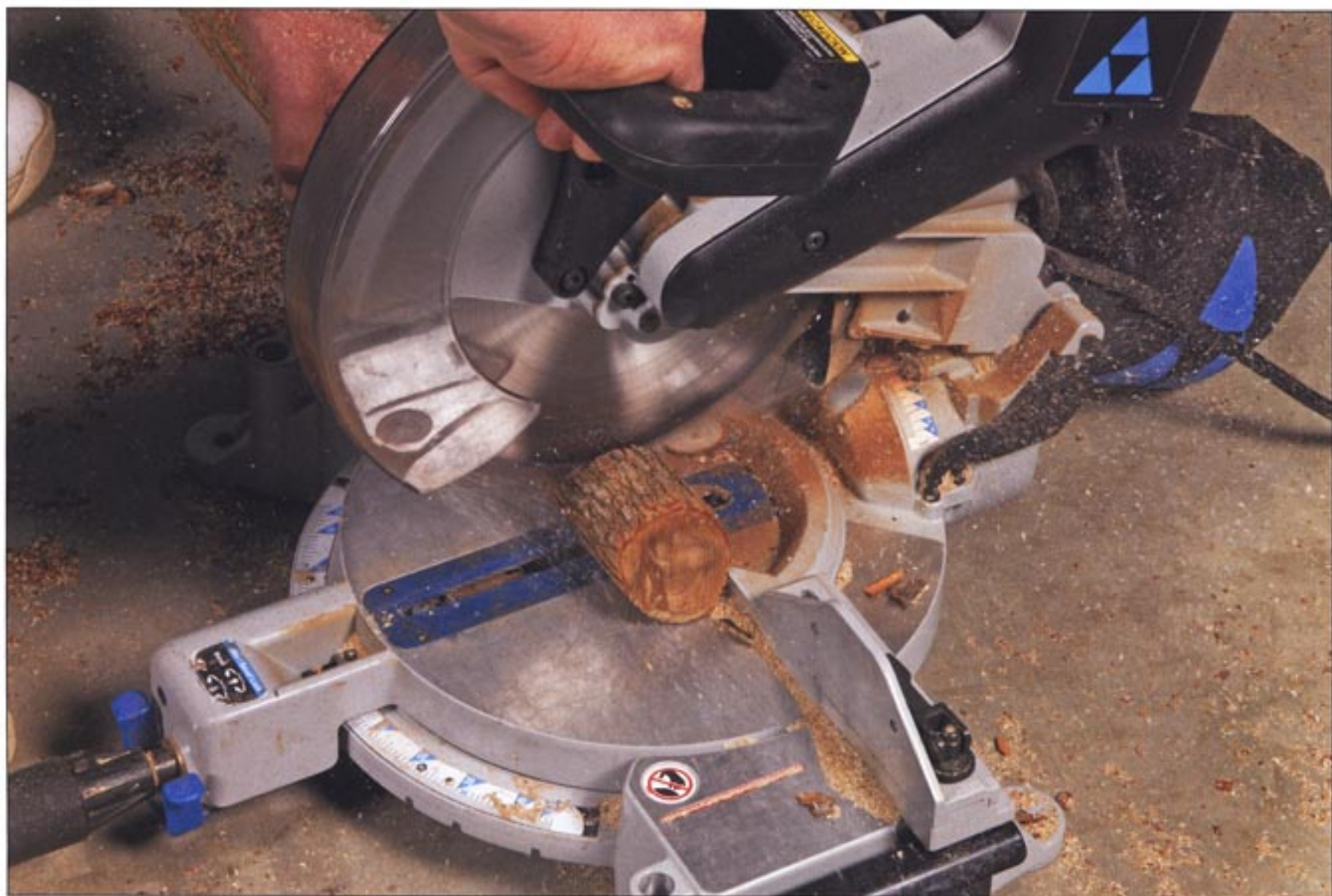
Cut to size with a chop saw.
