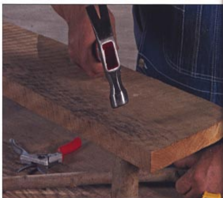
Check to make sure the shelf is positioned right and nail the shelf into the other leg.
