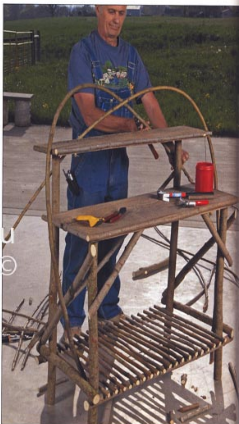
On the other end of the table, do the same thing. Thread the thick end of a long piece of willow inside the side brace and behind the front leg. Bend it over as a mirror image of the first piece of willow trim. Nail into place wherever it hits the wood frame.
