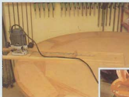
LEFT Router trammel for cutting true circle on top
