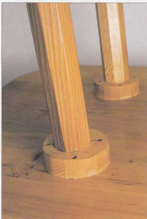
Underside of table, showing leg collars
