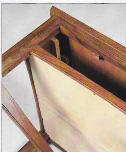
Top fixing and drawer runner
