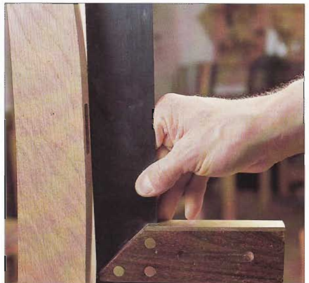
ABOVE: Create a flat on the curved back leg for the tenon shoulders
