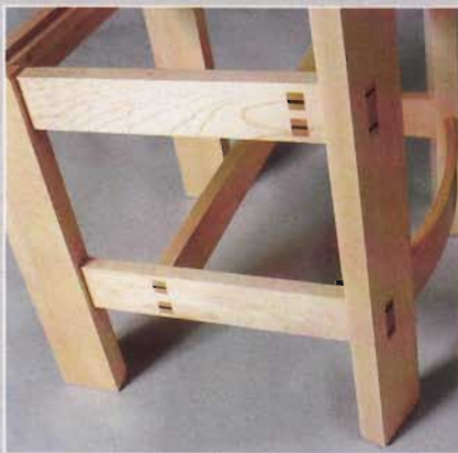
Detail showing the through-wedged tenons and laminated back rail
