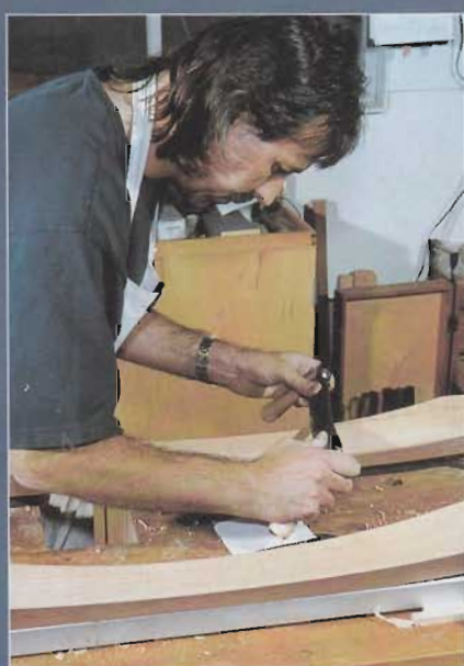
A draw knife is used for chamfer on inside of legs
