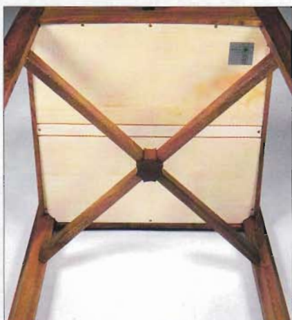
Underside, showing split dust panel in order to achieve an easy fit
