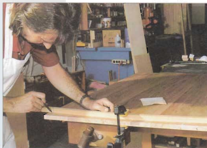
Marking out curve of top
