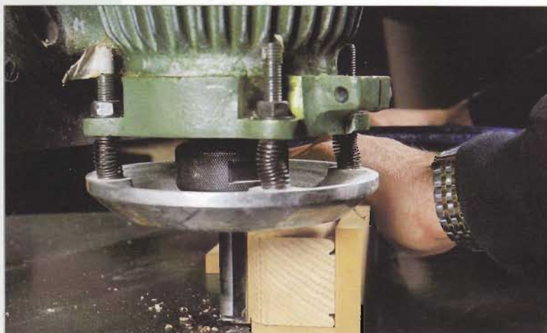
Jig and template in use for shaping the round tops of the legs
