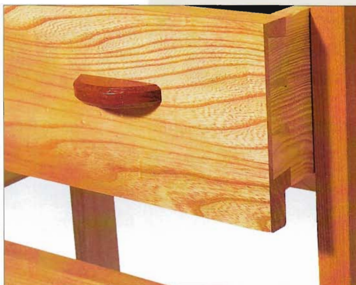
Top drawer detail showing overhang that covers the drawer rail
