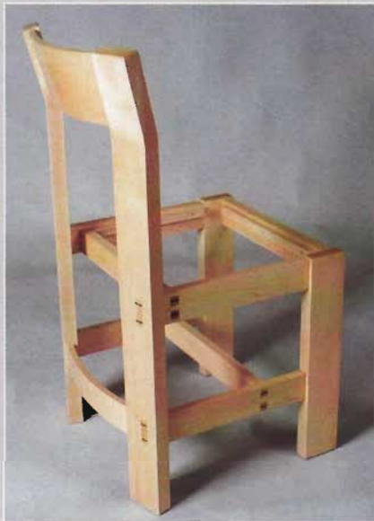
Seat removed showing rails for support
