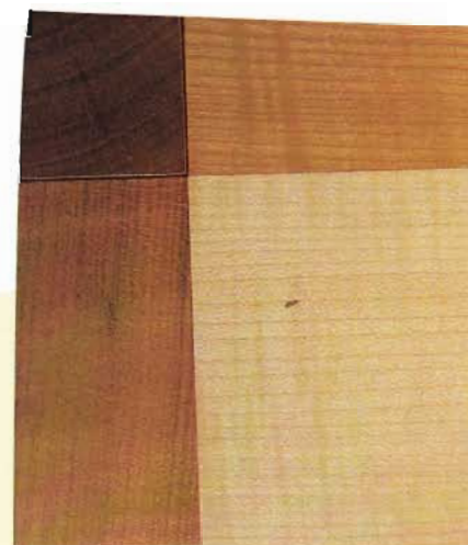
The drop-in top is a fine piece of book-matched ripple sycamore veneers
