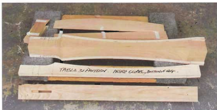
Leg template and shaping jig
