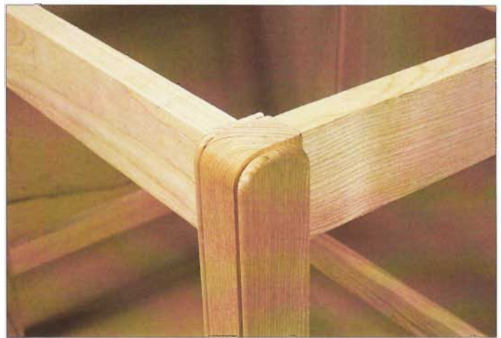
The finished bead on the front legs...
