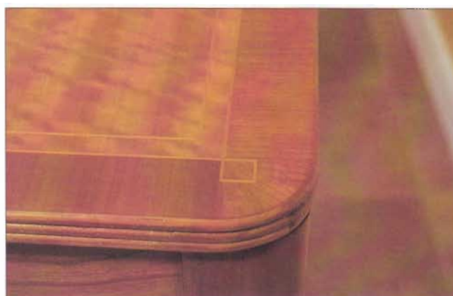
Cross banding, stringing lines and top edge reeding
