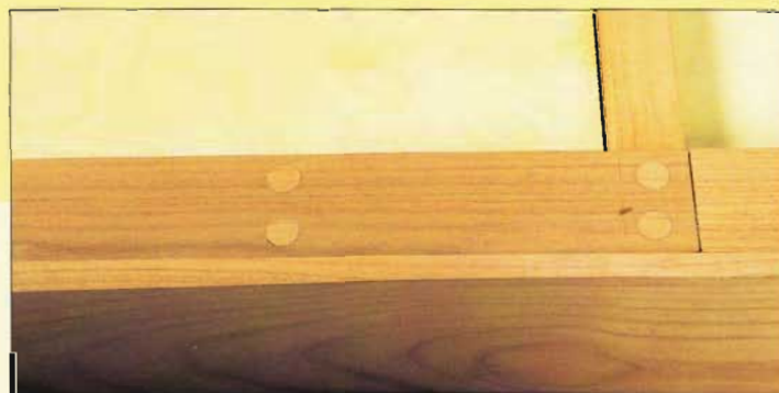
Under-frame is screwed and plugged into side rail rebates
