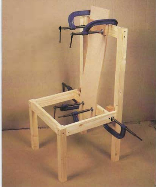
Full size mock-ups are a pre-requisite when chair making
