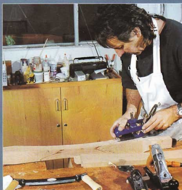
Cleaning up shape with compass plane
