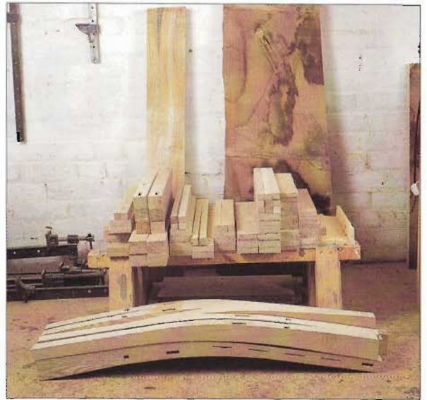
ABOVE: Morticed components stacked in handed pairs – very important!
