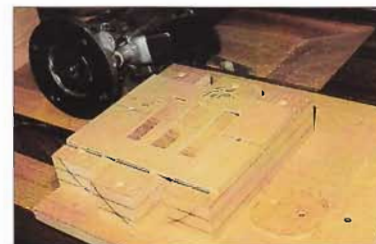
TOP RIGHT: Components of top and legs with tenon and mitred secret dovetails
