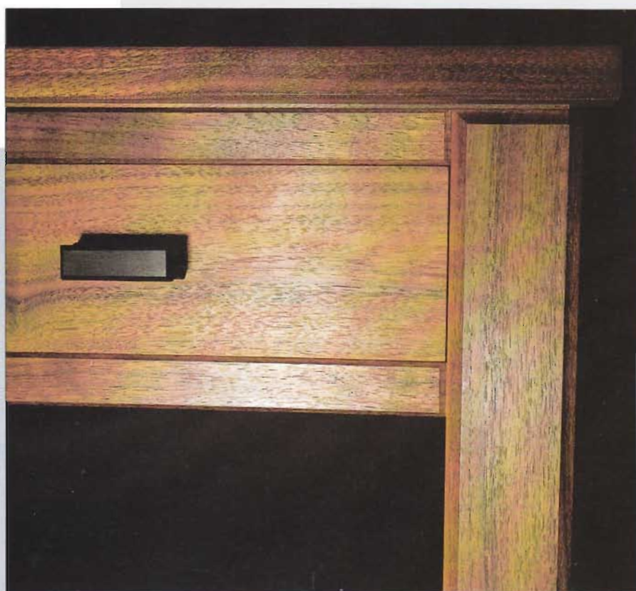
The chamfer detail is designed to catch the light and create interest
