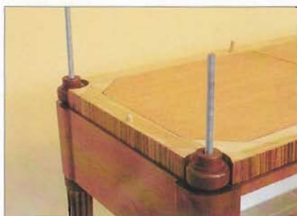
Above: Leg rods and spacers Below: Zebrano cross-banded sub-frame in place
