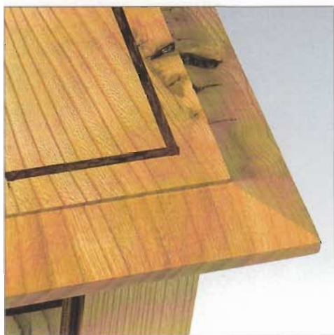
A small element of inlay is introduced into the top
