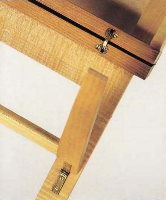
Fine soss hinges in the folding drawer front and the hinged stay
