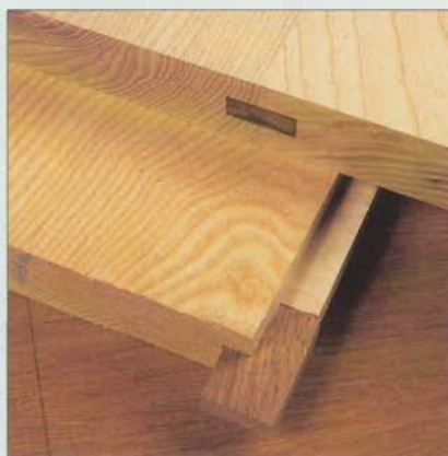
Top construction, plywood tongue and plug
