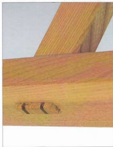
Stretcher rail detail
