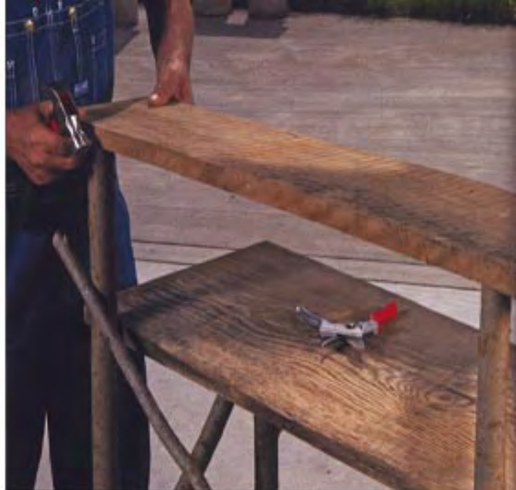
Lay it on top of the back legs so that it is parallel to the front edge of the large tabletop, centered from side to side, and doesn't extend back further than the outermost braces in back.
