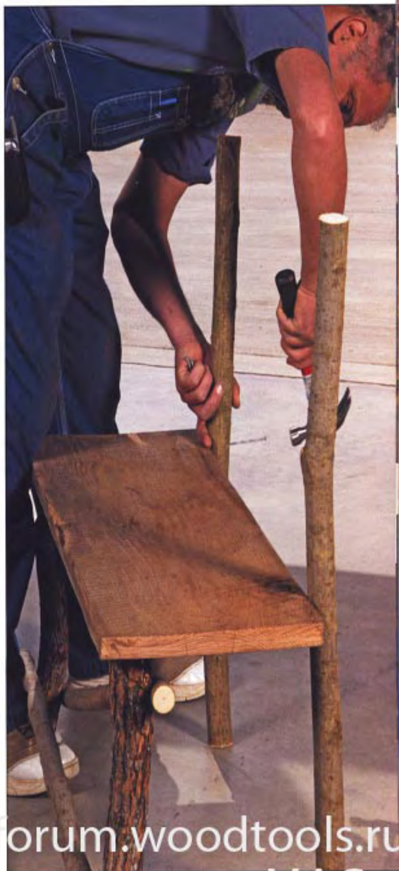
Attach the remaining 36" stick as the fourth leg.
