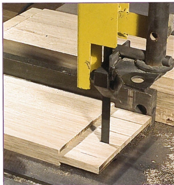
• The haunches on the tenons are cut out on the bandsaw
