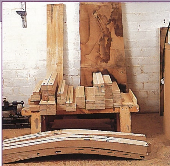
• Mortised components stacked in handed pairs – very important!
