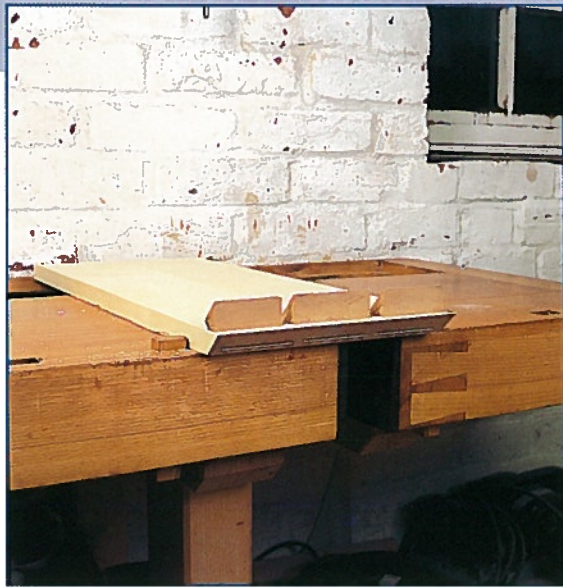
• Blocks are glued on to assist with the sometimes tricky operation of assembly
