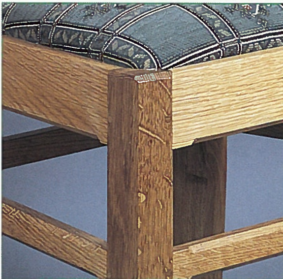
• Stopped chamfer detail on the top rails
