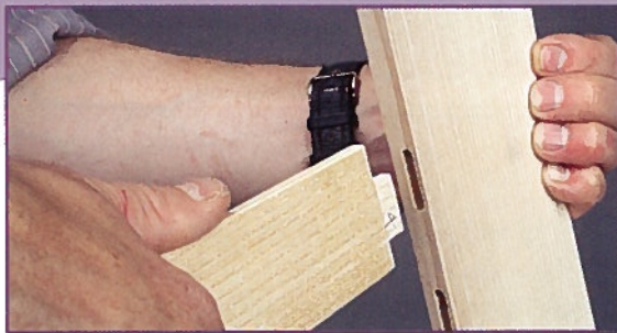
• The splats are tenoned into the crest rail
