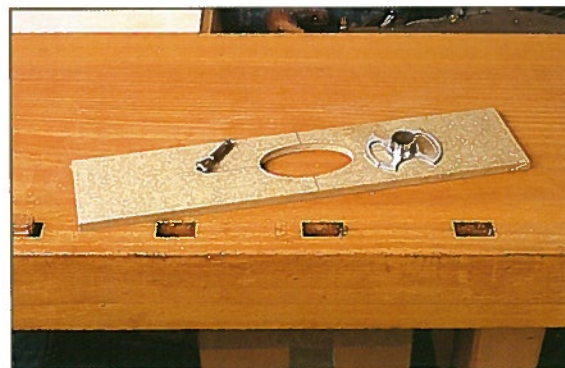
• Template and guide bush for cutting the handle
