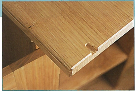
• Undersides of the adjustable shelves are notched for positive location
