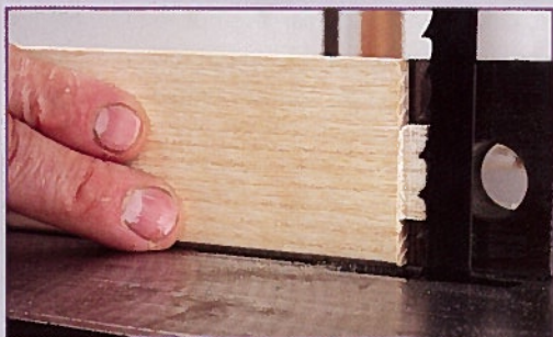
• Tenons cheeks were cut on the bandsaw
