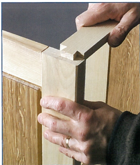
• Everything is locked together by the two dovetailed top rails
