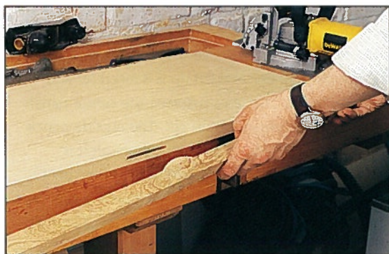
• Substantial solid lippings were biscuit jointed to all the carcass edges
