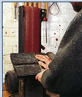
• A sander, accurately set up can make the task of cutting a lot of mitres less frustrating and time-consuming
