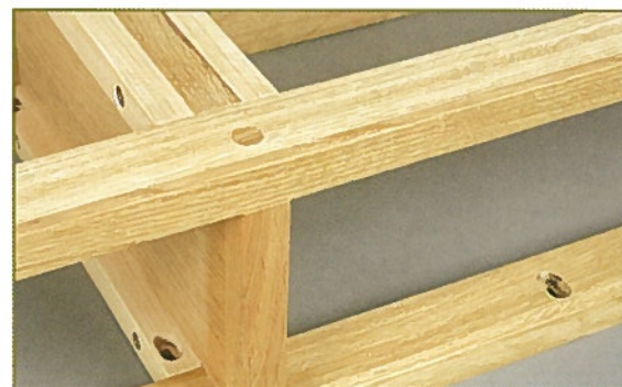
• Looking from the base showing the slotted holes in the kickers, to allow the top to expand and contract
