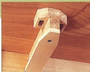
• Slotted block on end of guide rails aids expansion and acts as stops
