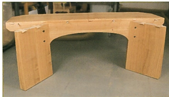
• The central stretcher beam is an integral part of the top
