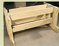
• I chose to do a dry-fit to check that it would actually go together
