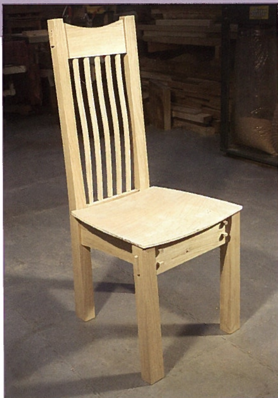
• A finished seat blank on a dry assembled chair
