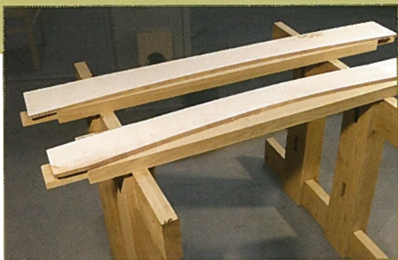
• Templates are used to mark out the shape of the curved rails and as guides on the spindle moulder
