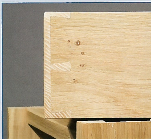
• Lapped dovetails are used for the drawer fronts
