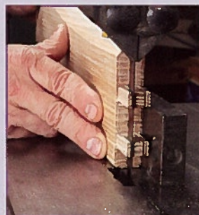
• The wedge slots were also cut on the bandsaw
