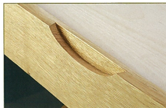
• The drawer pulls are routed out of the fronts
