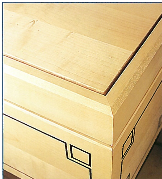
• Corner detail – the chamfer on the lid and the bottom carcass allow light to play
