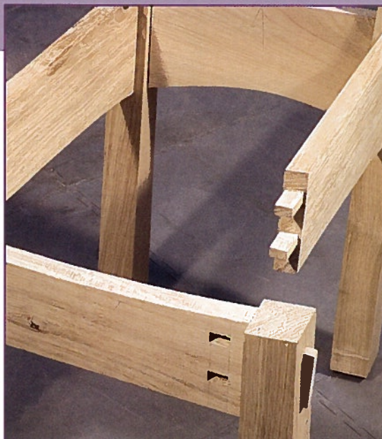
• Tenons through the front rail, as opposed to going into the leg, makes for very strong construction
