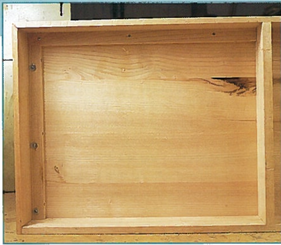
• The substantial plinth is biscuit jointed together, and support battens are screwed to the inside edge. Note the washers on slotted holes to allow for movement
