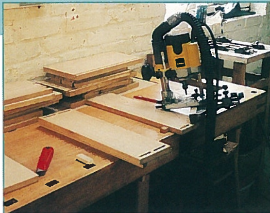
• Use a router to take out some of the waste
