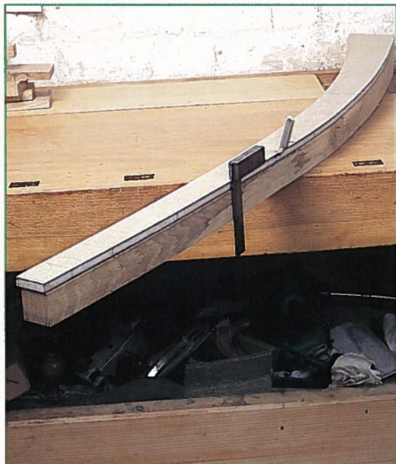
• MDF templates are used to mark out legs and then bandsawn to rough shape
