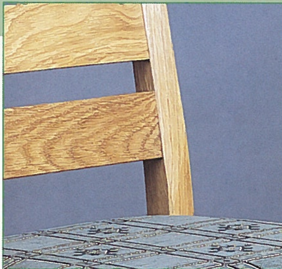
• The back legs are bevelled to meet the slats
