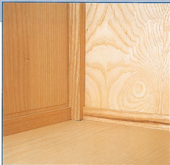
• The ply bottom is grooved in
