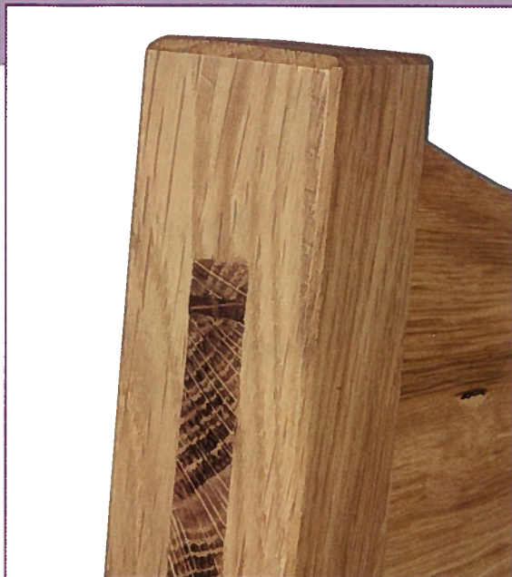
• All the tenons are through-wedged with contrasting brown oak
