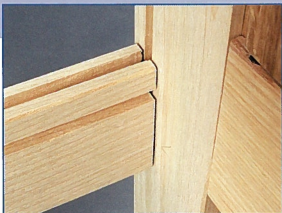
• The back is grooved into the back rail and vertical side rails
