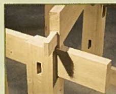
• I tapered the tenons to make sure there were no problems when gluing up
