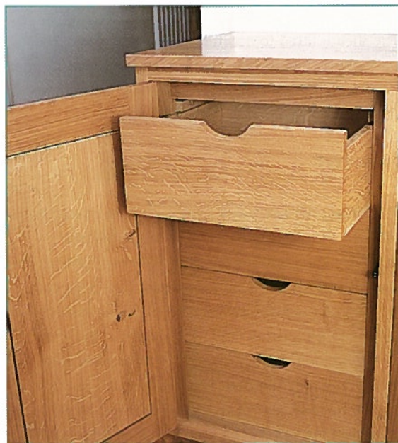
• Runners allow deeper drawer fronts and give clean visual lines, as there are no dividers
