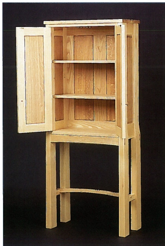
• The interior with framed panels in the back
