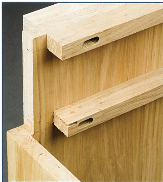
• The runners are slotted to allow for expansion
