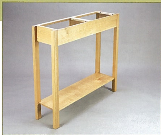
• The back rail is double-tenoned into the legs, with a haunch in the middle
