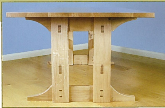
• Through-wedged tenons lock everything together
