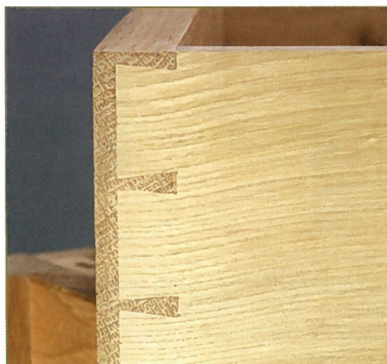
• The solid drawer fronts are lap dovetailed in the traditional manner
