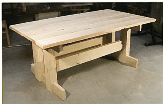
• Dry assembly of all the main components before shaping
