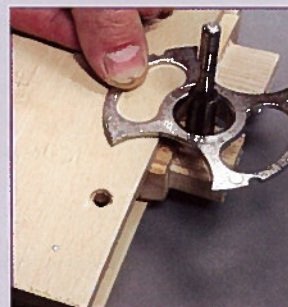
• Cutting the curved tenon shoulders on the rear of the side rails
