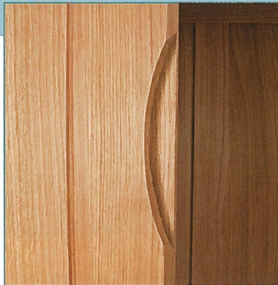
• The recessed handles are undercut with a dovetail cutter
