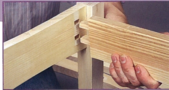
• Front rail joints before glue-up
