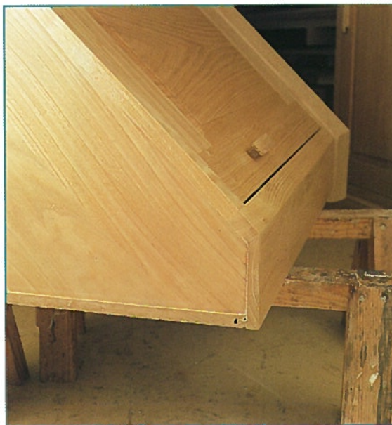
• The bottom panel is held in using biscuits
