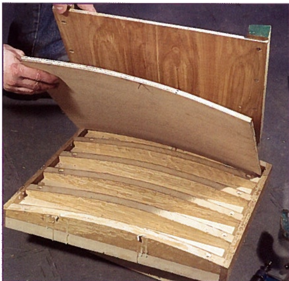
• The seat mould – the seat is made from two sheets of \frac{3}{8} in (4mm) ply
