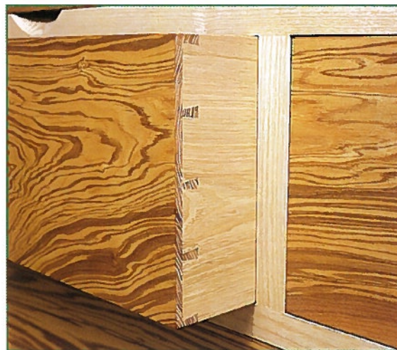
• Olive ash in drawer fronts contrasts with white oak drawer sides, revealing lap dovetails
