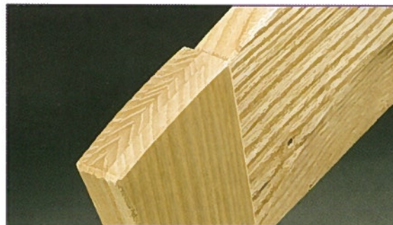
• End-grain of leg laminations
