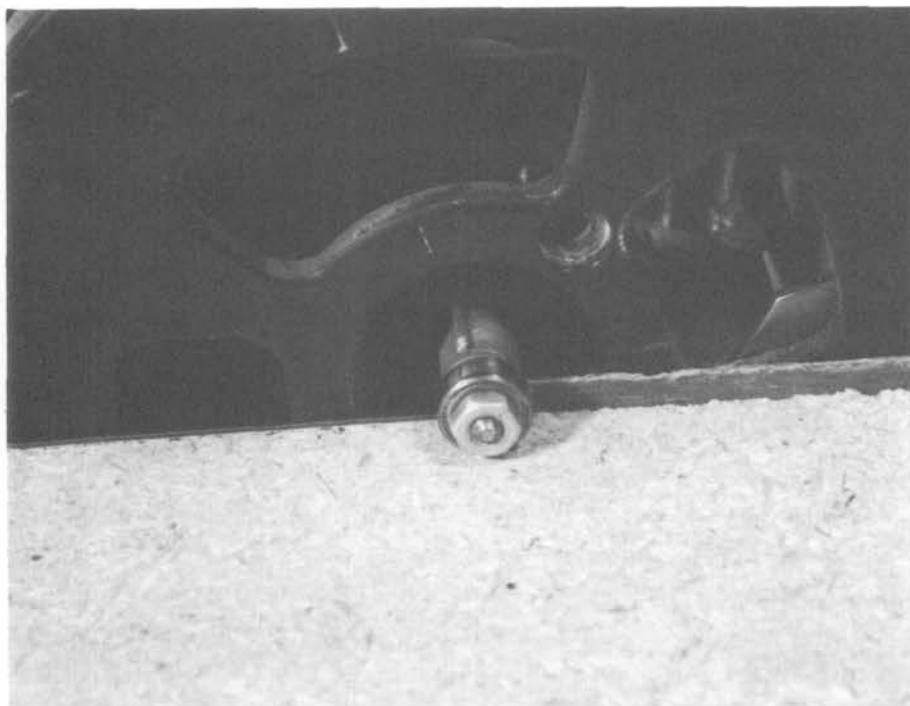
Illus. 24. A router equipped with a laminate-trimming bit is one of the most efficient ways of trimming the overhanging edges of the plastic laminate. The bit has a pilot that rides against the side of the board to guide it. The pilot will follow curved surfaces as well as flat ones. It will also follow irregularities in the surface of the board, so you should fill them in or sand them out before you apply the laminate.
