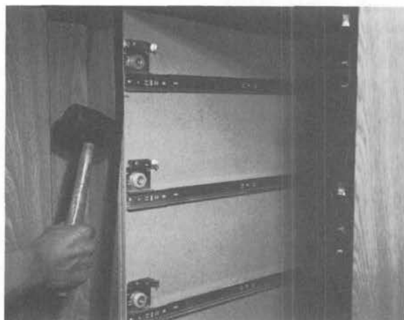
Illus. 234 (left). Use a rubber mallet to tap the T moulding into the kerf. Illus. 235 (right). This specialized hinge makes the simplified construction of these cabinets possible. It pushes the door away from the side of the cabinet as it opens, providing clearance for the full overlay design of the doors. Its adjustment capabilities make it easy to line up the doors after installation. A special 35-mm drill bit is recommended for making the recess in the door.
