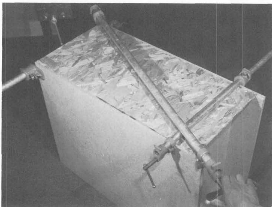
Illus. 122. Bar clamps are very useful for assembling cabinets. The clamp running diagonally between the corners pulls the cabinet into square.
