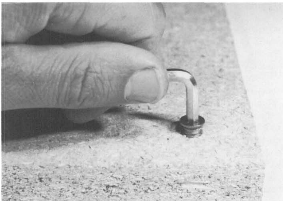
Illus. 126. A threaded insert has coarse wood screw threads around its outside diameter, providing greater holding capacity in particle board. In the middle of the insert, there is a smaller hole threaded for a machine screw. This insert has a hexagonal hole part of the way that accepts an Allen wrench; other types have a slot that accepts a standard screwdriver.
