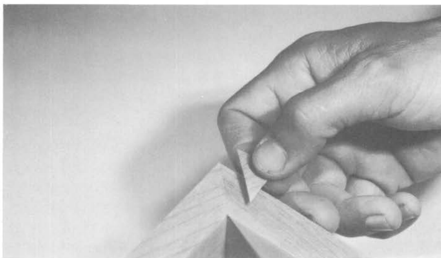
Illus. 20. When you apply and trim the second piece of tape with the square and knife, you'll get a perfect-fitting mitre joint.
