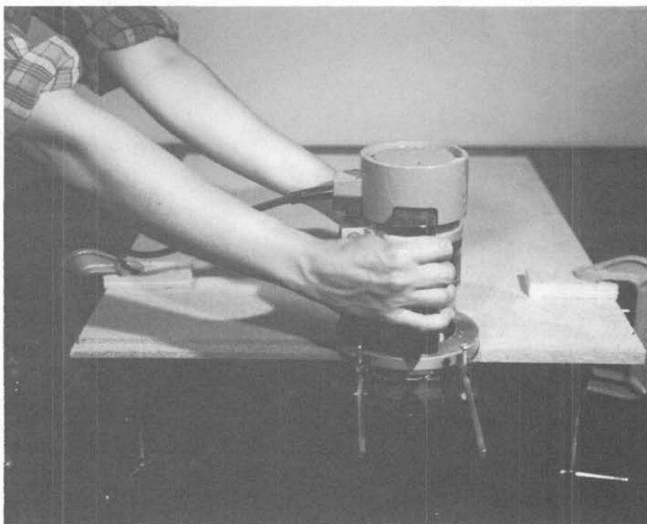
Illus. 226. Use a fence attached to the router for guiding the rabbet cuts.
