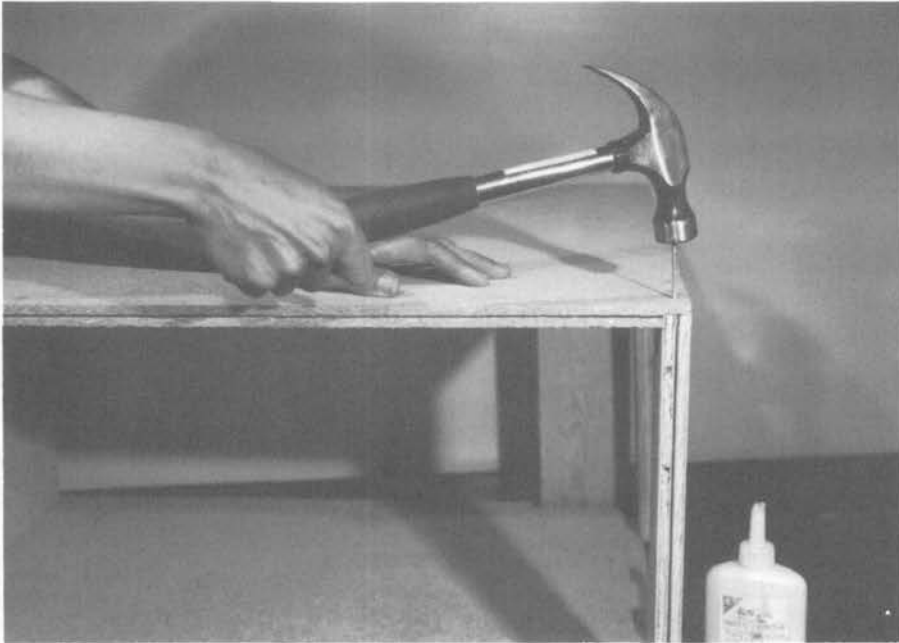
Illus. 229. Assemble the parts using glue and nails. Assembly will be easier if you position the parts so that you are always nailing against a firm surface.
