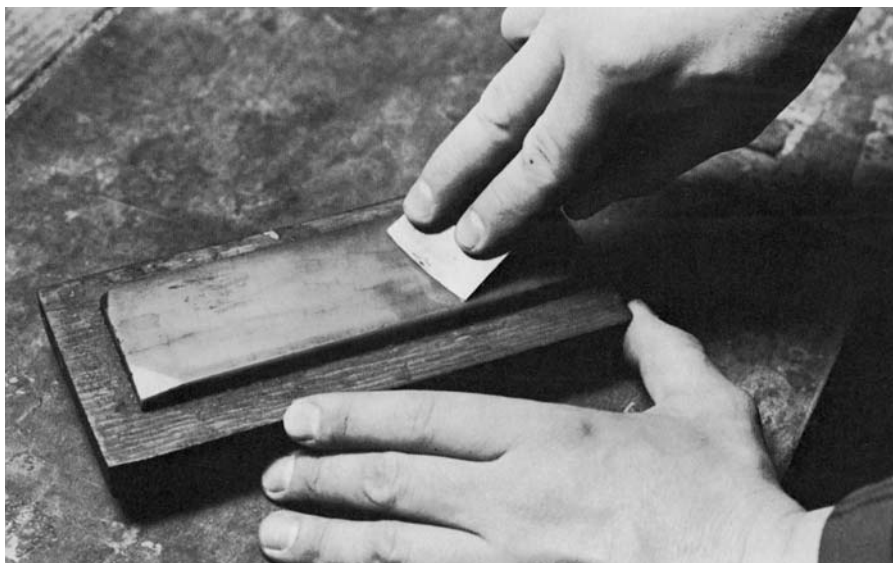
HONE THE ENTIRE LENGTH OF the radiused cutting edge of a fore plane.
