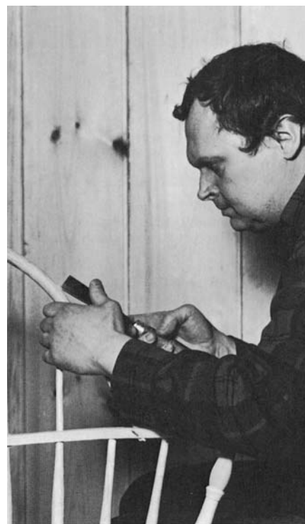
REST THE ARM ON THE bench top to wedge the ends of the bow. Shave the spindle ends flush with the bow.
