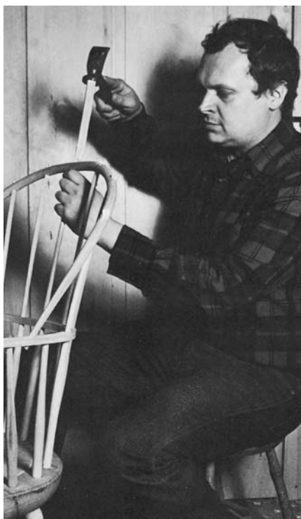
REST THE ARM ON THE bench top to wedge the ends of the bow. Shave the spindle ends flush with the bow.
