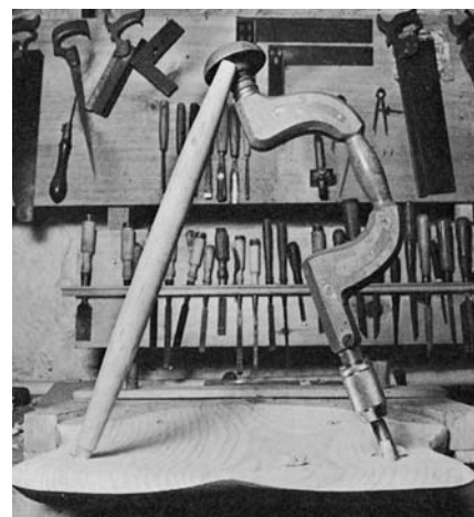
GAUGE THE SPY OF THE front leg against a bevel square. You can estimate the shallow rake of the leg (left). Use a dummy leg to find the rake and splay angles of the second front-leg socket (above).
