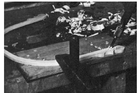
POSITION THE ARM ON THE stumps and mark one socket on a hand. Bore the first socket carefully; check the angles against bevel squares if necessary.
