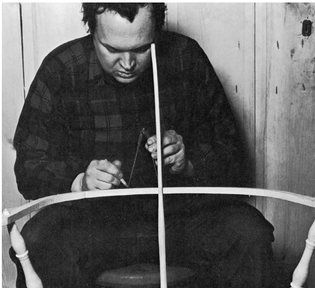
CHECK THE SOCKET LOCATIONS ON the arm against the spindles. Small adjustments to align a spindle and a socket will not be noticeable.
