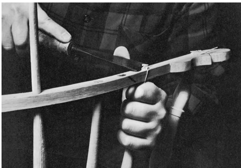
SHAVE THE TENONS AND WEDGES flush with the arm, then scrape and sand the surfaces.
