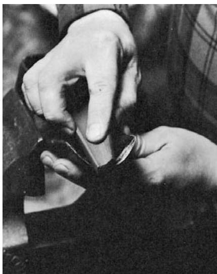
SHARPEN A GUTTER ADZE BY honing the cutting edge with an India gouge slip and buffing inside and out.
