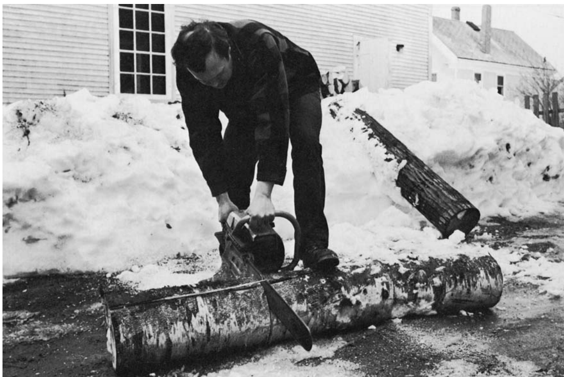
FOR MAKING CHAIR LEGS, FIRST cut the log into billets about 20" long.
