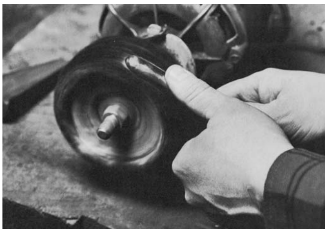
WORK THE NOSE OF A spoon bit to a perfect radius on an India gouge slip. Buff the shaped spoon bit inside and out to finish the cutting edge.
