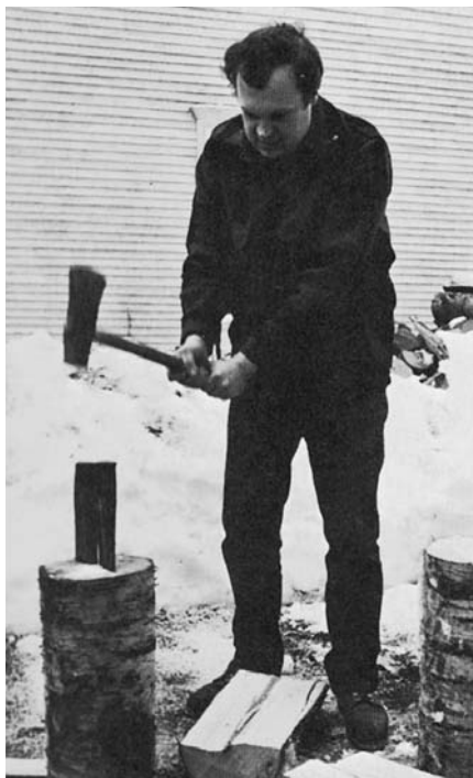
HALVE THE BILLETS. SET ONE or two wedges in the center, and drive them to open the billet. Sometimes, a solid blow will spilt a billet cleanly.
