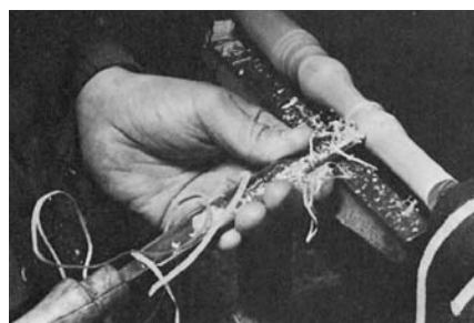
THE STUMP IS A MINIATURE leg , and the same techniques are used to turn it. The tapered tenon on the lower end of the armpost is the same size as the tenon for the legs. The tenon at its upper end fits into a 7/16" tapered socket.
