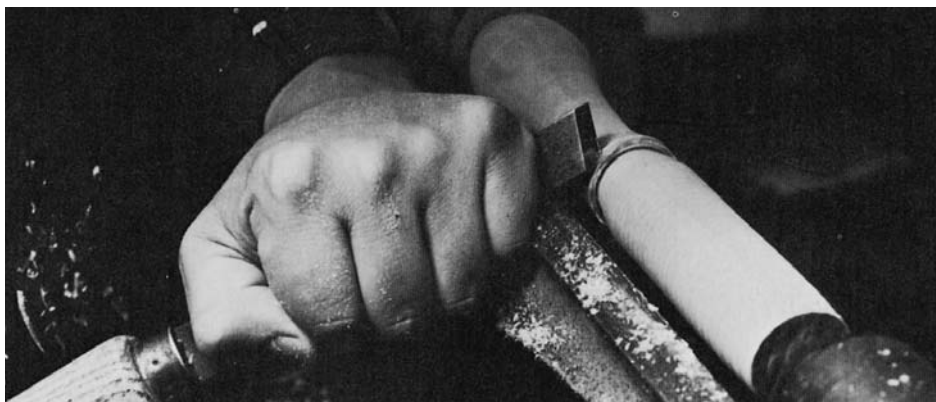
USE A SMALL GOUGE TO cut the cove that ends the major vase. Make the cove's stop with a small skew; use your free hand to control vibration. Shape the bottom of the vase and its wafer with a skew.
