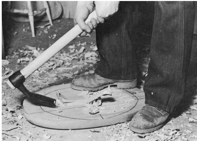
ROUGH OUT THE TOP SURFACE with a gutter adze, working into the middle. Sever a chip with each swing – don't pry it up.
