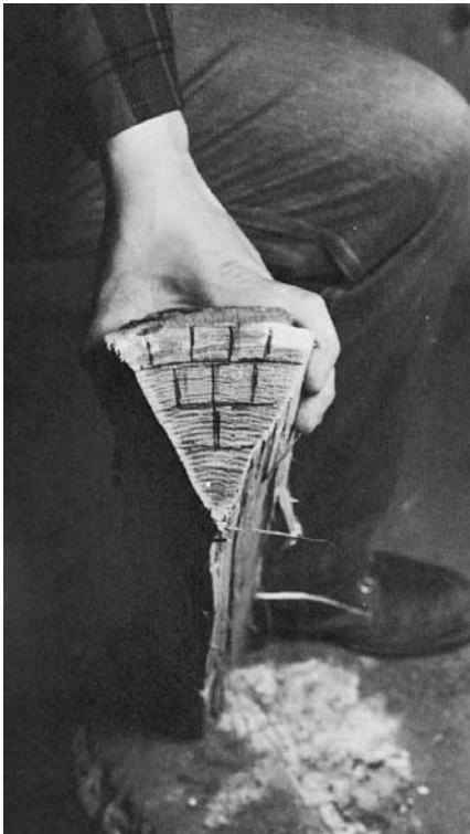
SPLIT 1" SQUARE SPINDLE BLANKS with a hatchet and wooden maul. Be sure to plan the riving sequence so you are always splitting pieces of equal mass.
