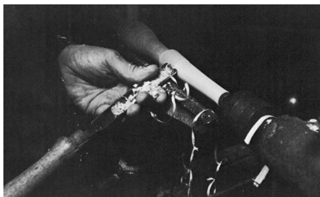
SHAPE THE BOBBIN WITH A large gouge. Clean up the surface with a planing cut. Cut a cove at the beginning of each arrow with a small gouge. Turn the arrows with a large gouge; make the tapers slightly concave.
