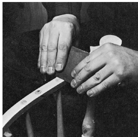
SHAVE THE TENONS AND WEDGES flush with the arm, then scrape and sand the surfaces.
