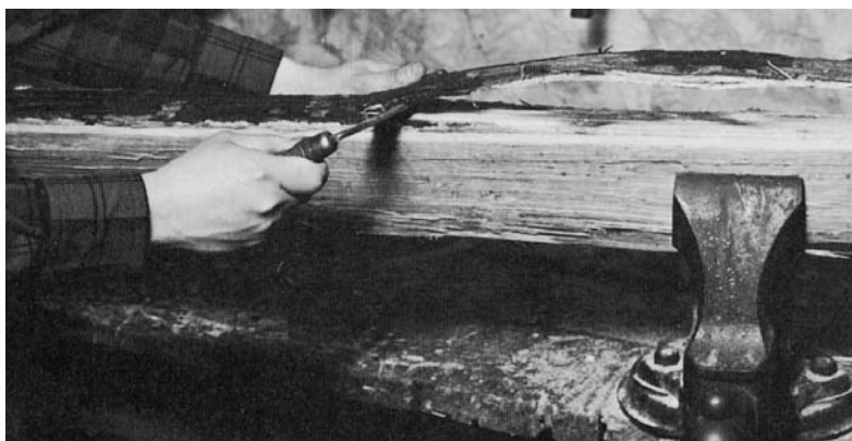
AFTER RIVING, STRIP THE BARK off the red oak billets with a drawknife.
