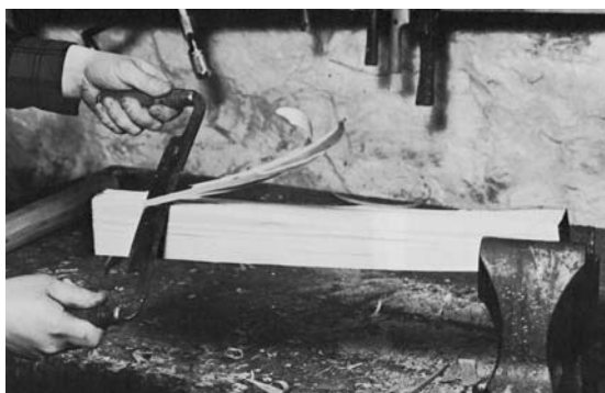
PREPARE THE TURNING BLANK FOR the lathe by removing the high spots with a draw knife.
