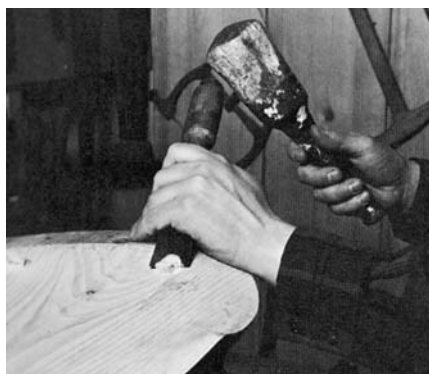
A WIDE, SHALLOW CARVING GOUGE (#3 sweep 35mm) works well to trim the tenon ends flush with the surface of the seat.
