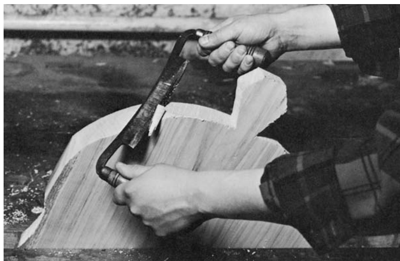
TO ROUGH OUT THE QUARTER round back edge of the shield seat, make three cuts with the drawknife. The three are shown in the drawing and show how little wood needs to be removed with spokeshaves.
