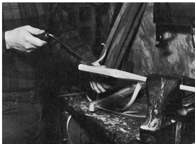
ROUGH OUT THE LONG, THIN end of the spindle with a drawknife. Work the last 6" or so of the bottom end with a drawknife. Turn the spindle again and thin the shaft above the swelling.
