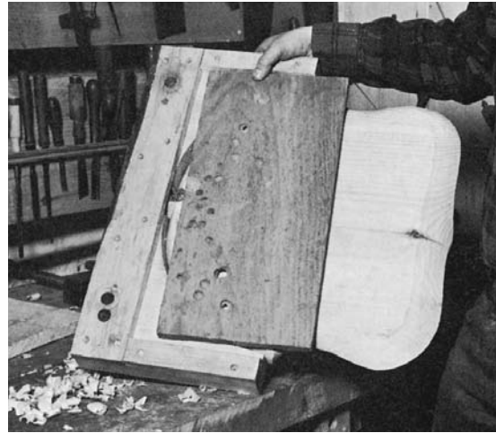
PLACE A BACKING BOARD BENEATH the seat, so that you do not bore into the bench top.
