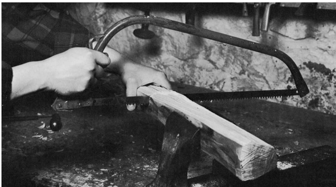
CUT THE LEG BLANKS TO length . A Swedish brush saw works well for this.
