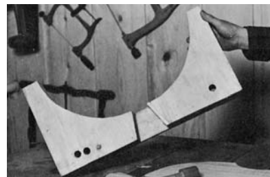
A SIMPLE WOODEN FRAME WILL hold the seat on the bench while shaping. Two threaded wooden screws fit through the back of the frame into the bench top. Bore and tap a series of holes in the bench top so that the frame can be positioned for several different jobs.
