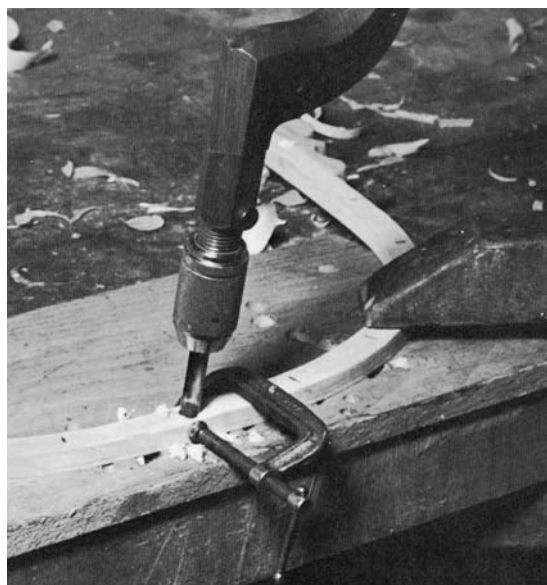
BORE THE CENTER SPINDLE SOCKET in the arm .
