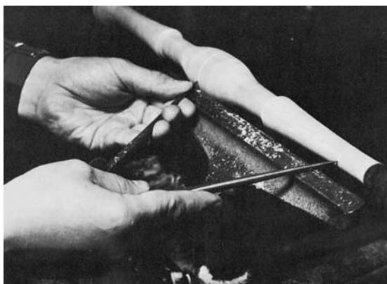
SCRIBE THE TENON SHOULDERS AND turn the tenon.
