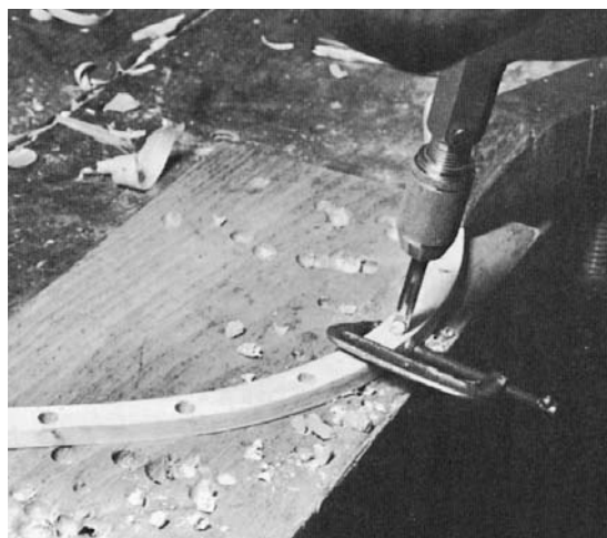
BORE THE CORRESPONDING SOCKETS ON either side of the center . Judge the slope and flare angles by eye, or with bevel squares.
