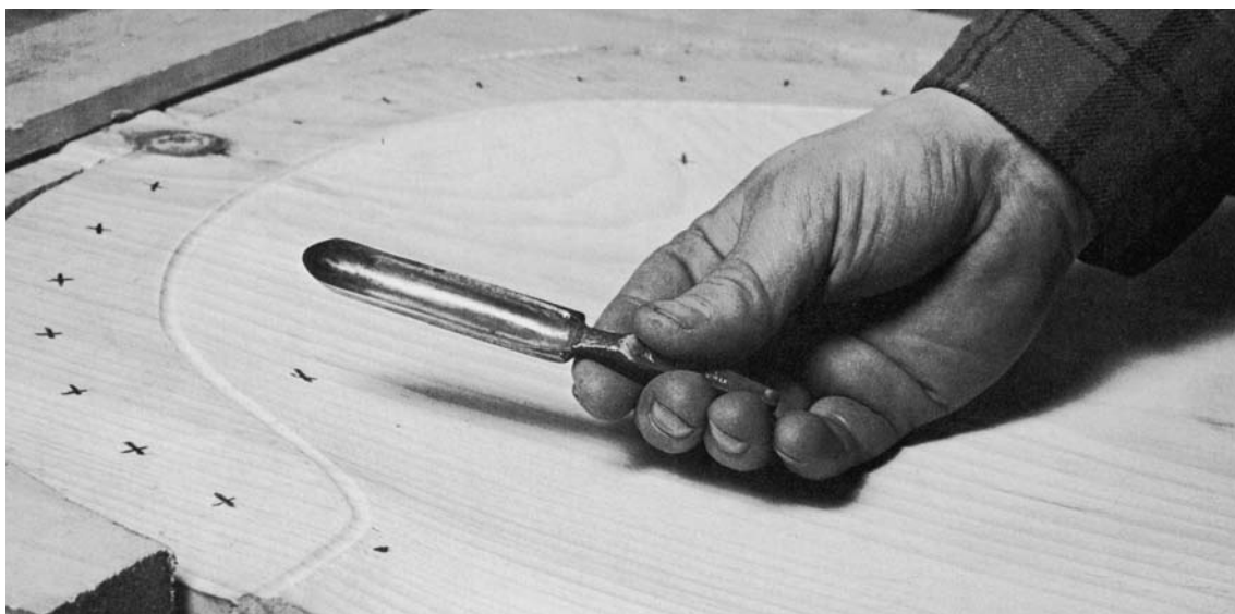
SPoon BITS ARE IDEAL FOR Windsor chairmaking . The semicircular end is sharpened, and does all the cutting.
