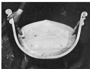
PUT THE FIRST SOCKET OVER its stump, and position the arm for marking the second socket. The arm and seat edge should form symmetrical arcs.
