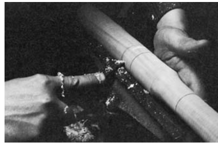
CUT THE SIDES OF A bead with a skew then, round by scraping.
