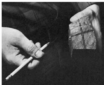
AFTER REMOVING THE BARK AND pith from a billet, sketch out the blanks on an end for riving. Hold the billet vertically and rive the back blanks with a hatchet driven by a wooden maul. Always split so there are pieces of equal mass on each side of the hatchet.
