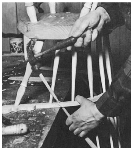
REST THE ARM ON THE bench top to wedge the ends of the bow. Shave the spindle ends flush with the bow.
