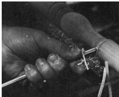
USE A SMALL GOUGE TO cut the cove that ends the major vase. Make the cove's stop with a small skew; use your free hand to control vibration. Shape the bottom of the vase and its wafer with a skew.
