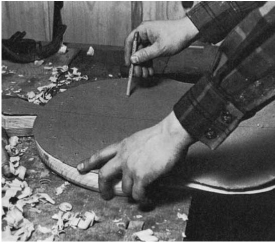
MARK THE POSITIONS OF THE seat sockets through holes drilled in the pattern.
