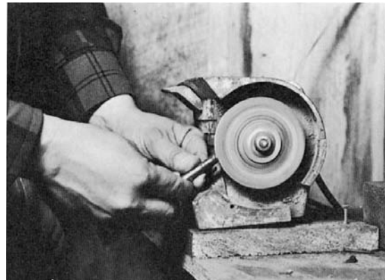
USE A DIAMOND DRESSER TO true the edge of a grinding wheel.
