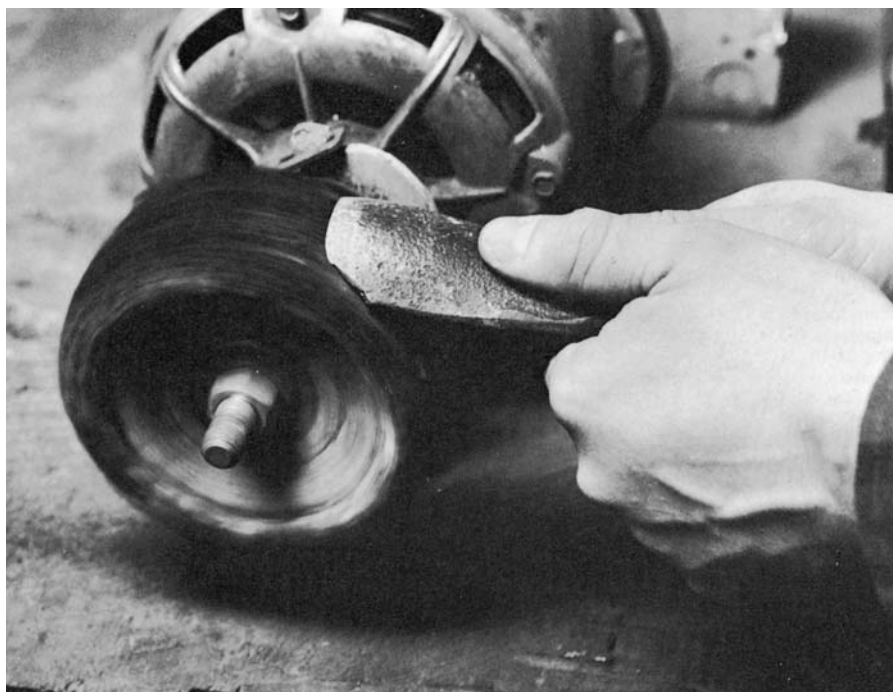
SHARPEN A GUTTER ADZE BY honing the cutting edge with an India gouge slip and buffing inside and out.
