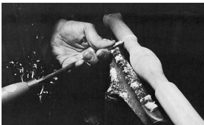
SHAPE THE BOBBIN WITH A large gouge. Clean up the surface with a planing cut. Cut a cove at the beginning of each arrow with a small gouge. Turn the arrows with a large gouge; make the tapers slightly concave.
