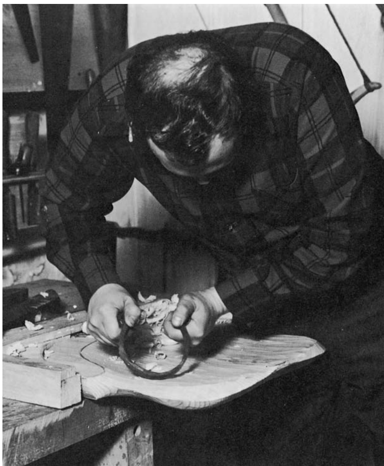
THE SMOOTH SURFACE AT THE back of the seat (below) has been worked with the scorp, after the entire saddle has been adzed roughly to shape. When smoothing, work the scorp from the back to the center of the saddle.
