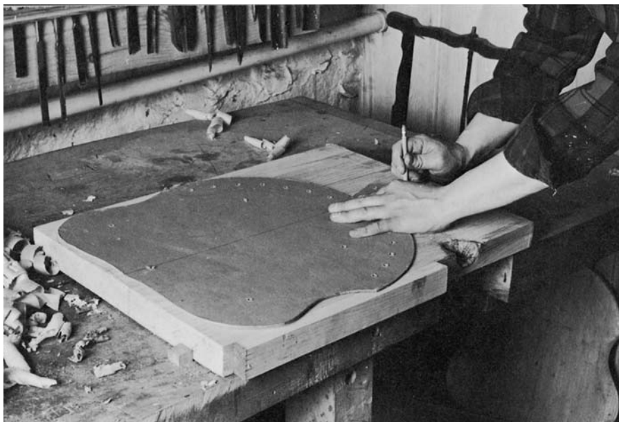
MAKE A PATTERN FOR THE seat out of \frac{1}{4} " luan plywood. If possible, position the pattern so that knots and other blemishes are located out of the area to be excavated.
