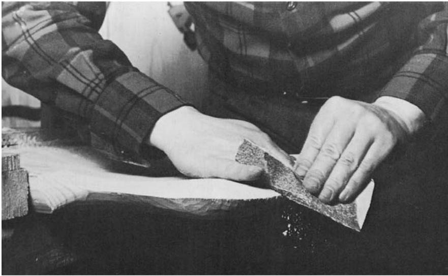
CARVE THE CHANNEL THAT SEPARATES the excavated saddle from the flat surface at the back of the seat with a 1/4" veiner (top). Sand the seat with #50-grit sandpaper. Don not lose the shapr arris on the edge.
