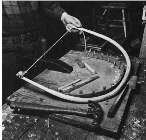
WHEN THE ARM OR BOW is cool to the touch, tie its ends together with string. The part will retain the shape, and you can use the form to bend the other part.
