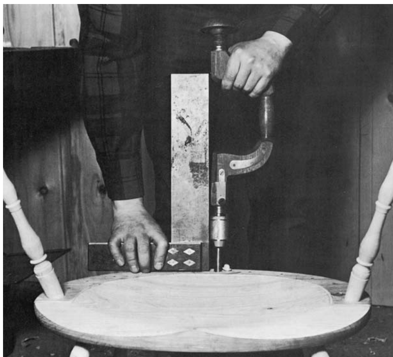
BORE THE SOCKET FOR THE center spindle first. Viewed from the front, it is perpendicular to the seat.
