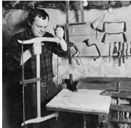
A 25" BOW SAW MAKES short work of cutting out the seat. Clamp the blank securely to a corner of the bench. Saw with the full length of the blade and use your whole body, not just your arms, for the strokes.
