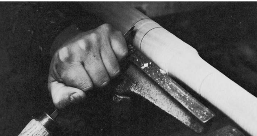
CUT THE SIDES OF A bead with a skew then, round by scraping.
