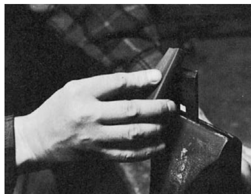
HONE THE CONCAVE CURVE OF a forkstaff plane blade with a concave India gouge slip.
