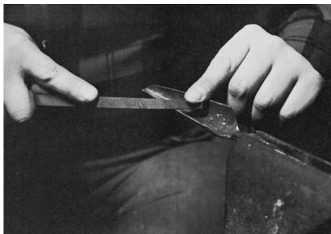
WORK THE NOSE OF A spoon bit to a perfect radius on an India gouge slip. Buff the shaped spoon bit inside and out to finish the cutting edge.
