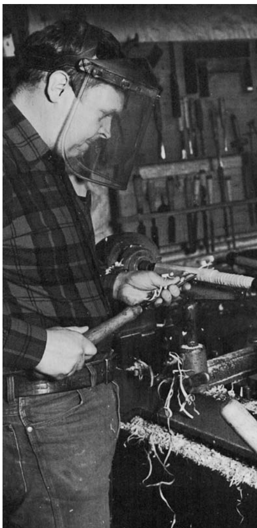
SHAPE THE SHORT SPINDLES WITH a large gouge to a continuous sweep from end to end.
