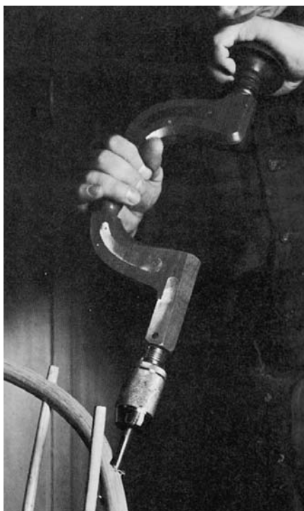
THE FINAL TWO SPINDLE SOCKETS are the riskiest. Start the bit at a right angle to the bow. Bore slowly and raise the brace to the correct angle as the hole deepens. Whittle a point on each outside spindle to make assemble easier.
