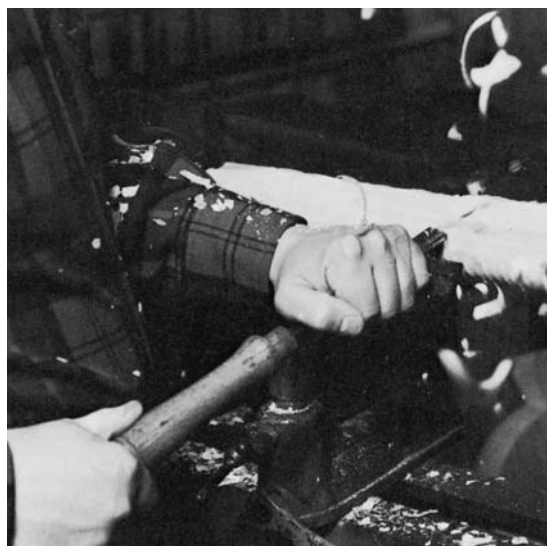
ROUGH THE LEG BLANKS TO the diameters of the major and minor vases on the legs . While the blank is spinning, mark the position of the bead and cove above the major vase, and the wafer above the minor vase with a pair of dividers. If you do not have a model leg, determine these points by measuring from a full scale pattern.
