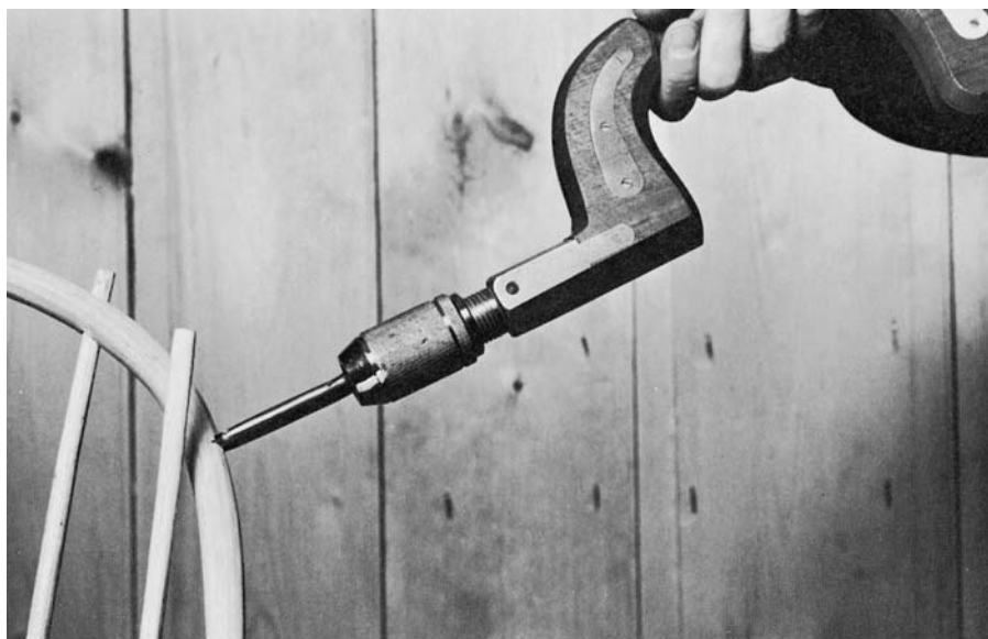
THE FINAL TWO SPINDLE SOCKETS are the riskiest. Start the bit at a right angle to the bow. Bore slowly and raise the brace to the correct angle as the hole deepens. Whittle a point on each outside spindle to make assemble easier.
