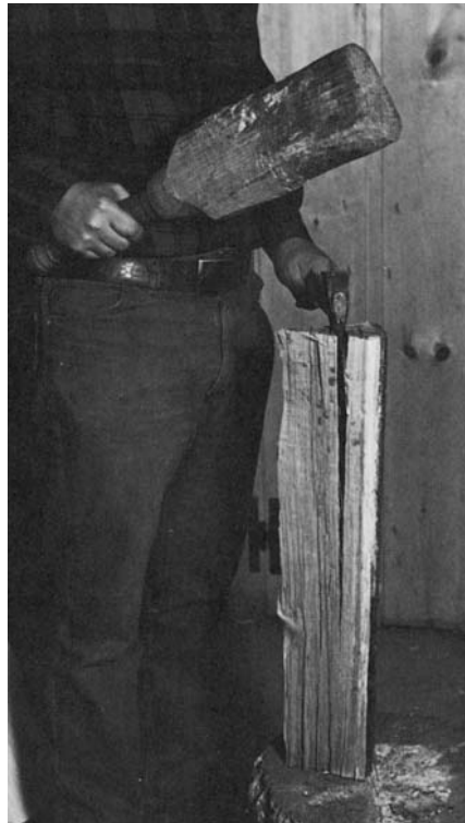
SPLIT 1" SQUARE SPINDLE BLANKS with a hatchet and wooden maul. Be sure to plan the riving sequence so you are always splitting pieces of equal mass.
