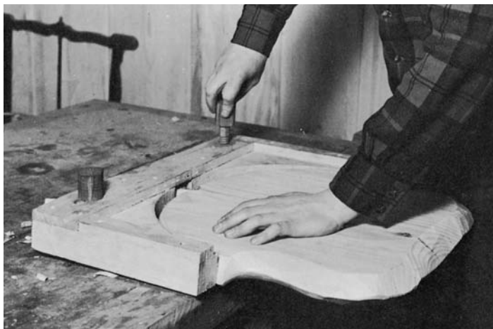
A SIMPLE WOODEN FRAME WILL hold the seat on the bench while shaping. Two threaded wooden screws fit through the back of the frame into the bench top. Bore and tap a series of holes in the bench top so that the frame can be positioned for several different jobs.
