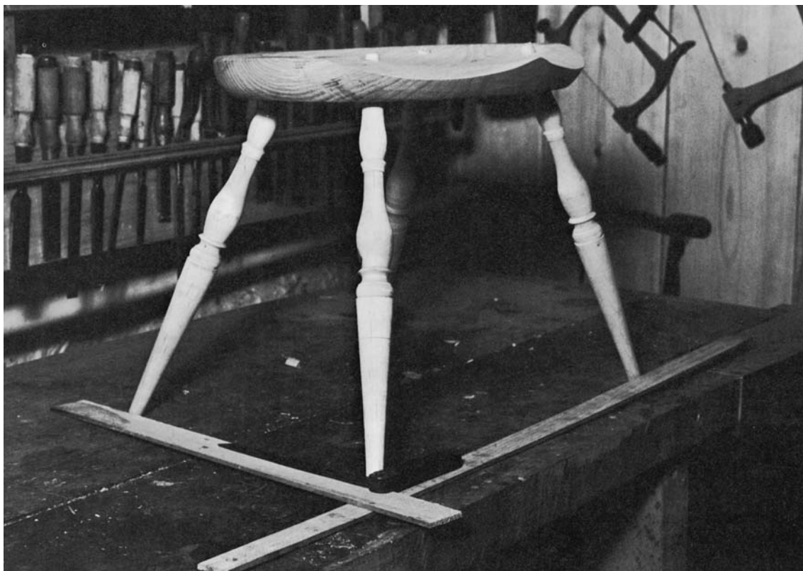
DETERMINE THE ANGLE AT WHICH the center stretcher meets the side stretchers with two straight edges.
