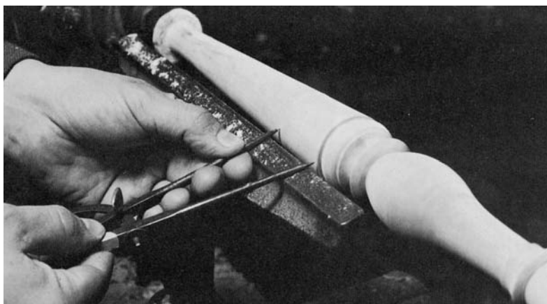
SCRIBE A RING ON THE tapered foot to locate the stretcher socket .
