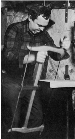
A 25" BOW SAW MAKES short work of cutting out the seat. Clamp the blank securely to a corner of the bench. Saw with the full length of the blade and use your whole body, not just your arms, for the strokes.
