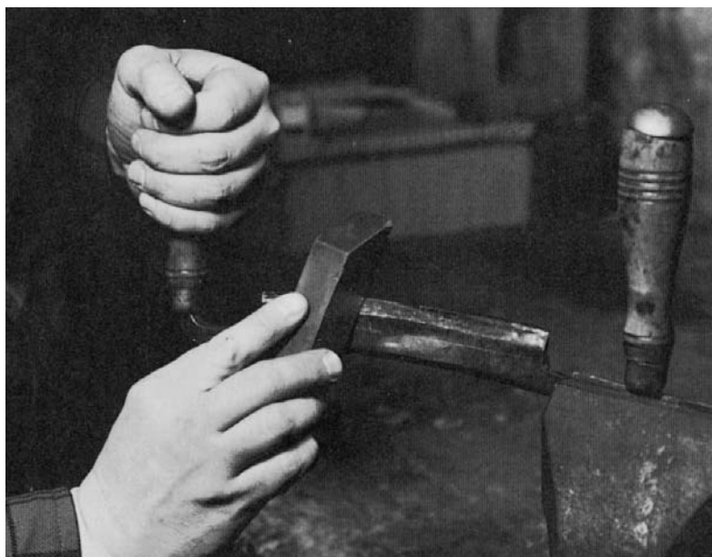
HONE THE CONCAVE CURVE OF a forkstaff plane blade with a concave India gouge slip.
