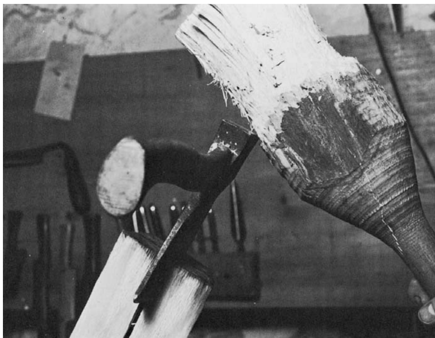
AFTER REMOVING THE BARK AND pith from a billet, sketch out the blanks on an end for riving. Hold the billet vertically and rive the back blanks with a hatchet driven by a wooden maul. Always split so there are pieces of equal mass on each side of the hatchet.
