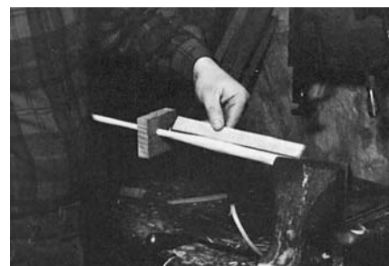
SACK BACK SPINDLES ARE MADE in the same way as those for a continuous arm chair. However, they must fit tightly where they pass through the arm. Make two gauges to ensure that the spindles are the correct diameter at the correct height. After the spindles have dried, remove stains and whittling marks with a cabinet scraper.
