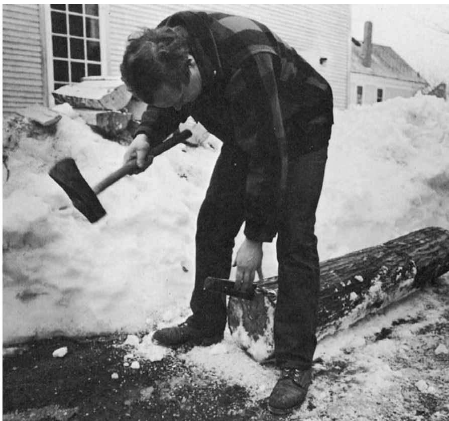
TO SPLIT A 5-FT. LONG red oak log for chair backs begin the split by driving a wedge into the edge of one end. Add a second wedge near the heart.
