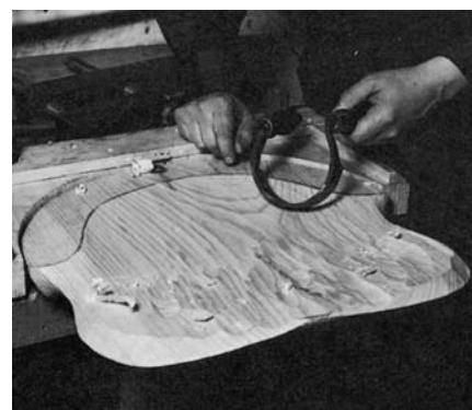
THE SMOOTH SURFACE AT THE back of the seat (below) has been worked with the scorp, after the entire saddle has been adzed roughly to shape. When smoothing, work the scorp from the back to the center of the saddle.
