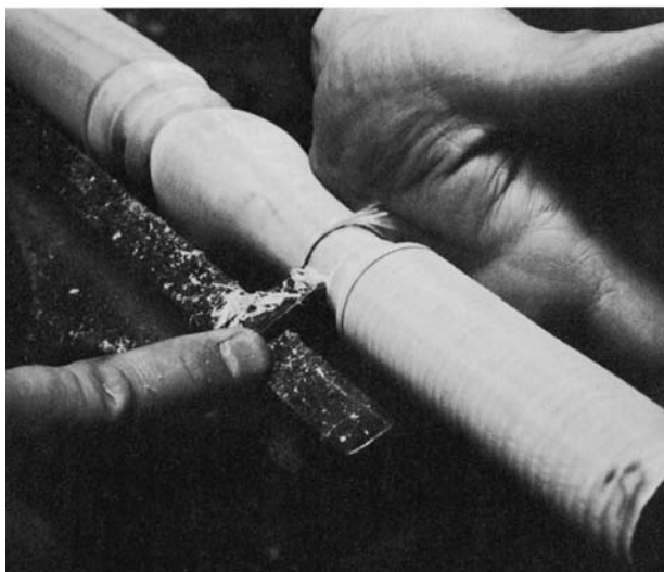
USE A SMALL GOUGE TO cut the cove that ends the major vase. Make the cove's stop with a small skew; use your free hand to control vibration. Shape the bottom of the vase and its wafer with a skew.
