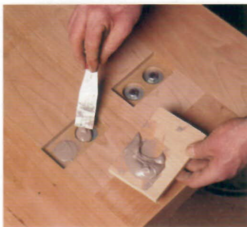
BOLTS AND BOND. The tabletop is secured to the legs with 6-in. lag screws, then covered with auto-body filler. More common wood fillers might shrink, leaving depressions in the tabletop.
