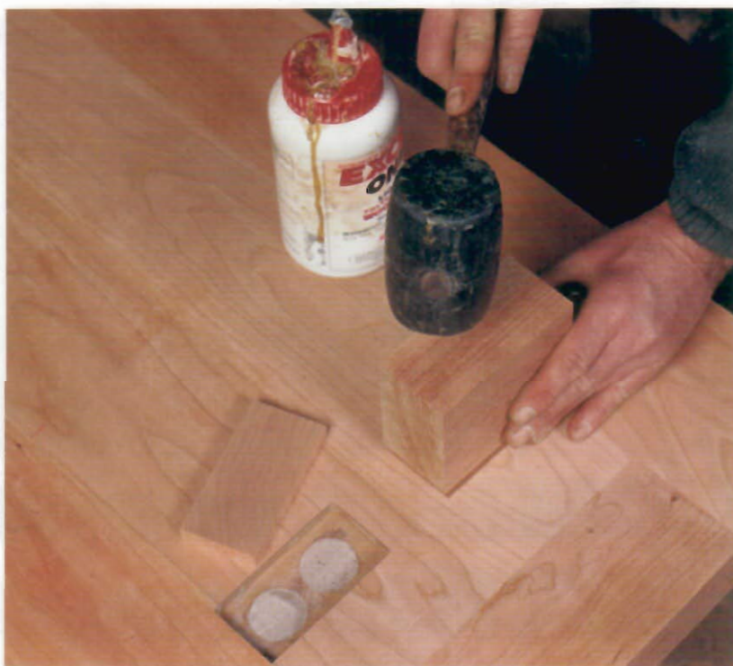
FAUX LEG ENDS. End-grain inserts are coated with polyurethane glue and then tapped into place. ■
