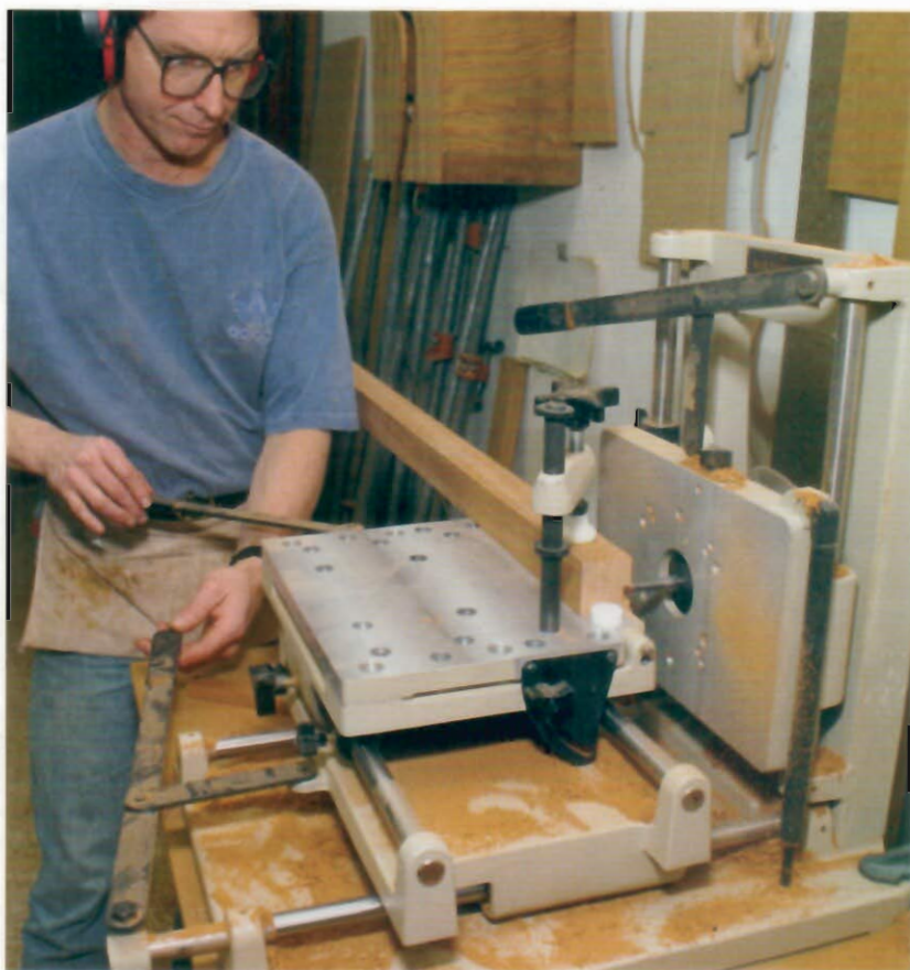
ROUTER JIG SPEEDS AND SIMPLIFIES JOINERY. The author used a Multi-Router to rout all the mortises and tenons on this sideboard. Grooves, dadoes and dovetail slots were done on a router table or with a handheld router. Dovetails were cut by hand. ■
