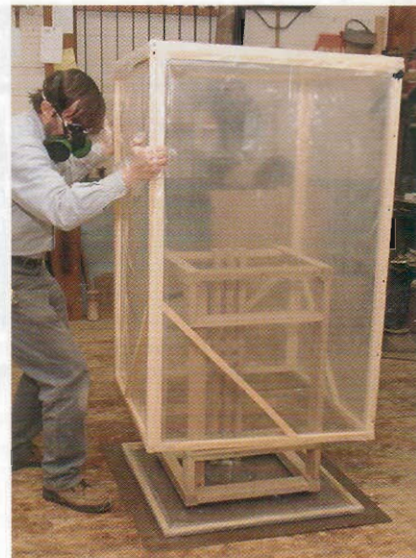
AQUEOUS AMMONIA IS POURED INTO A GLASS CONTAINER placed at the bottom of the fuming chamber (left). Then the top of the chamber is lowered quickly onto its base (above). Protective gear is essential.
