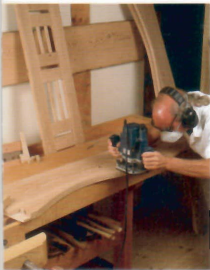
TEMPLATES AND A ROUTER HANDLE SHAPING AND MORTISING. Vogt made a plywood master template so he could form the shelves, complete with tenons, using a straight router bit and a rub collar. The other templates are for shaping the slats, mortises and wedges.
