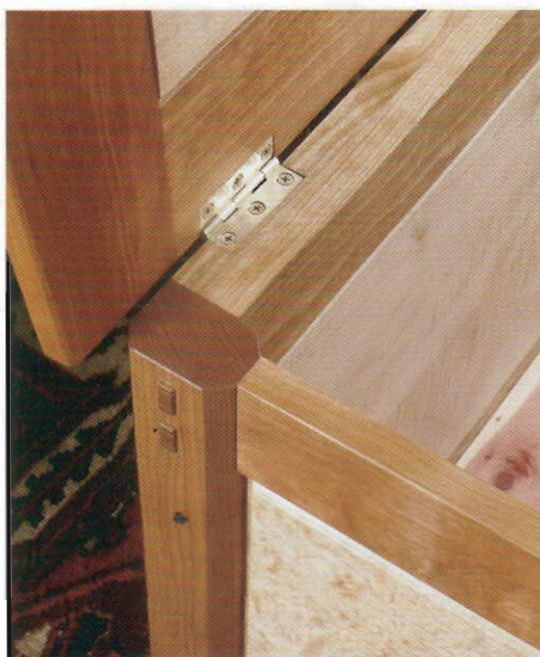
A FILLER STRIP HOLDS THE HINGES. The strip is glued to the rear top rail and butts against the rear legs, whose inside back corners remain unchamfered.
