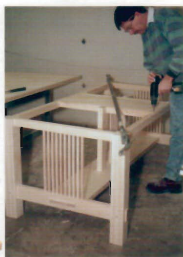
SCREW AND GLUE SUBTOP TO RAILS. The author squares up a slight misalignment in the base using a pipe clamp, then glues and screws the subtop in place.
