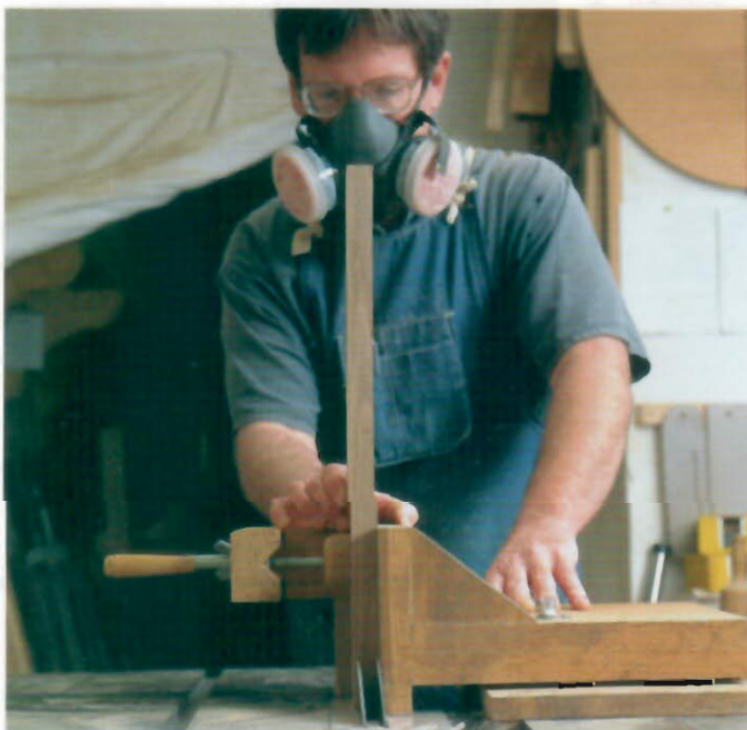
DOUBLE-BLADE TENONING ON THE TABLESAW. With a custom-made jig, the author cut angled tenons for the side stretchers and side seat rails. Sawblades were set at a 4° pitch to the surface of the saw table and separated by a \frac{1}{8} -in. spacer.
