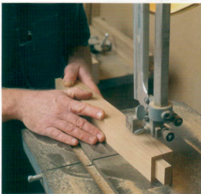
CUTTING THE CURVED BACK SLATS. Convex and concave cuts from 8/4 lumber yielded \frac{1}{4} -in.-thick slats, after the surfaces were scraped clean. These slats are the only curved pieces of the chair.
