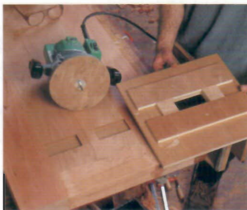
MORTISES THAT MATCH. A small-diameter straight-cutting bit and a simple template make easy work of cutting the mortises in the tabletop.
