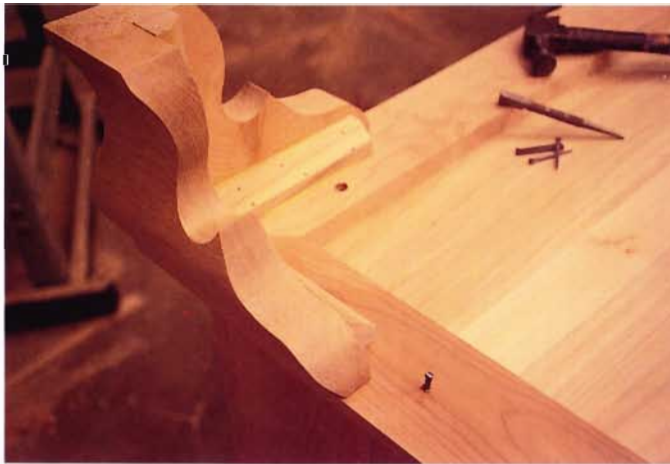
13 After the foot base has been completed, invert the lower case unit and attach the foot assembly to the case bottom with No. 8 x 1 1/4" screws in the front frame. Use nails to complete the assembly. Nails allow slight movement over time, which helps keep the piece from splitting. Notice the corner blocks on the feet.
