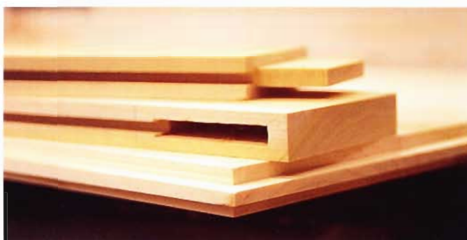
27 Mill, cut to size and assemble the top and bottom panels as well as the two shelves. All are made in the same fashion, with the front and back pieces being the stiles and the ends being the rails.
