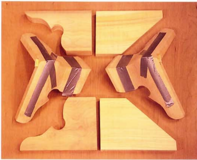
11 Make the ogee-bracket feet. (See the sidebar “Ogee-Bracket Feet” later in this chapter.)
