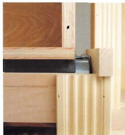
23 Assemble the TV lift box, install it on the TV lift and raise the lift to its fully elevated position. Double-check all measurements for the top of the center cabinet. One of the side strips for the top has been placed on the top of the center cabinet to show the relationship of the edge trim to the TV lift box. The top of the bottom panel of the TV lift box will be flush with the top of the cabinet.
