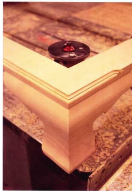
12 Sand the foot base frame, then fit the ogee-bracket feet to the frame with glue and corner blocks. Rout the profile on the edge of the frame.
