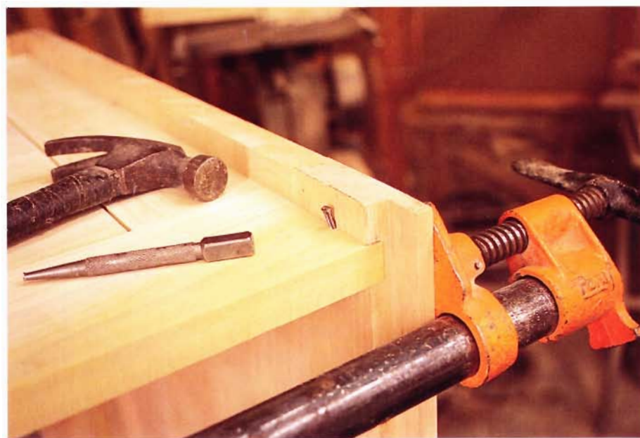
26 When set, glue the front face frame to the other leg of the L-corner, creating the quartered column area.
