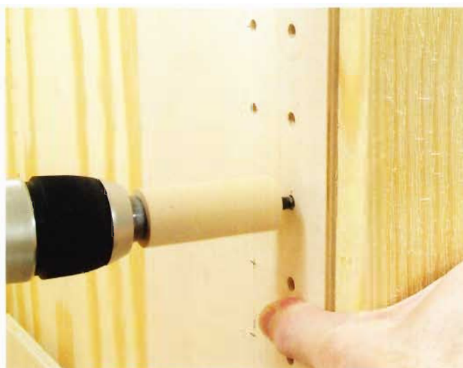
15 Drill the holes for the shelf pins using a homemade drilling jig. Using a \frac{1}{4} "-thick piece of scrap plywood, make the jig by drilling a straight line of holes 1\frac{1}{2} " apart. Place the bottom of the jig on the bottom of the cabinet and hold it firmly against the side of the cabinet. Start and stop the line of holes 6" from the bottom and top of the side of the cabinet. Use a stop on the drill so you won't drill through the cabinet side.
