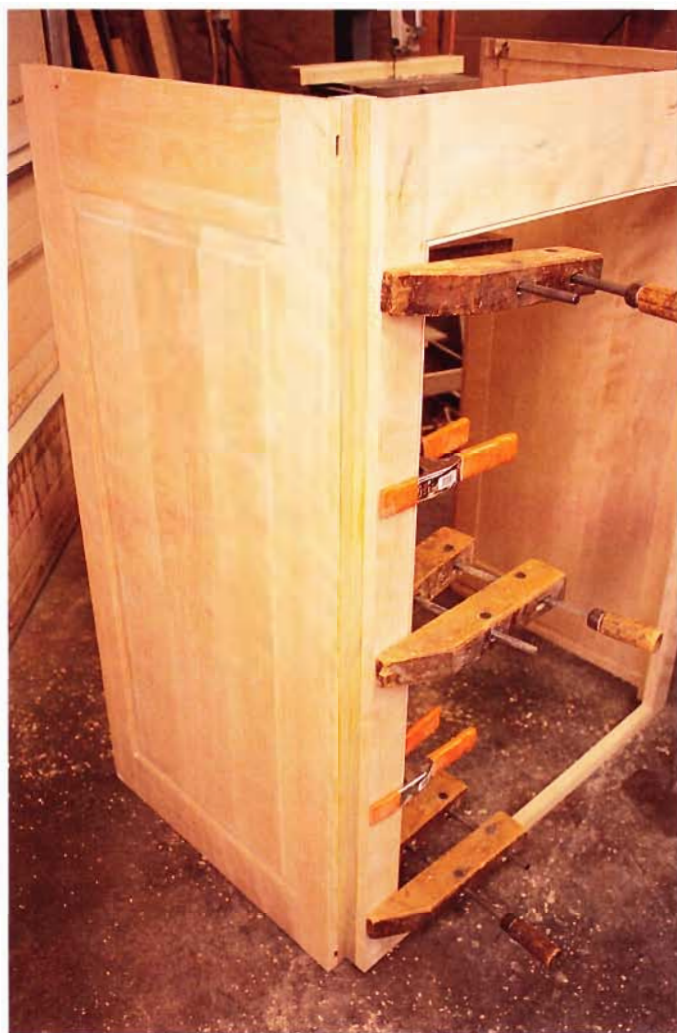
26 When set, glue the front face frame to the other leg of the L-corner, creating the quartered column area.
