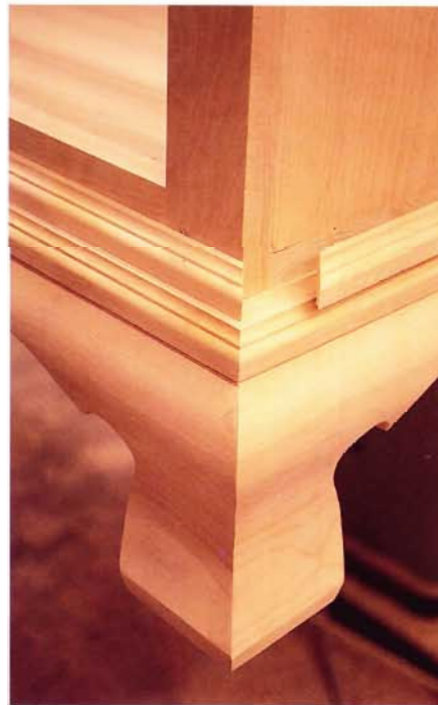
14 Next, mill and install the base moulding that covers the exposed case dovetails.
