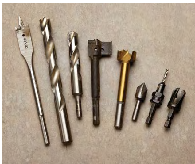
At top, a brace and eggbeater drill. At bottom, from left-to-right: A flat, or spade bit, brad tip, twist bit, expansion bit, Forstner bit, countersink, twist and countersink combination and a plug cutter.
