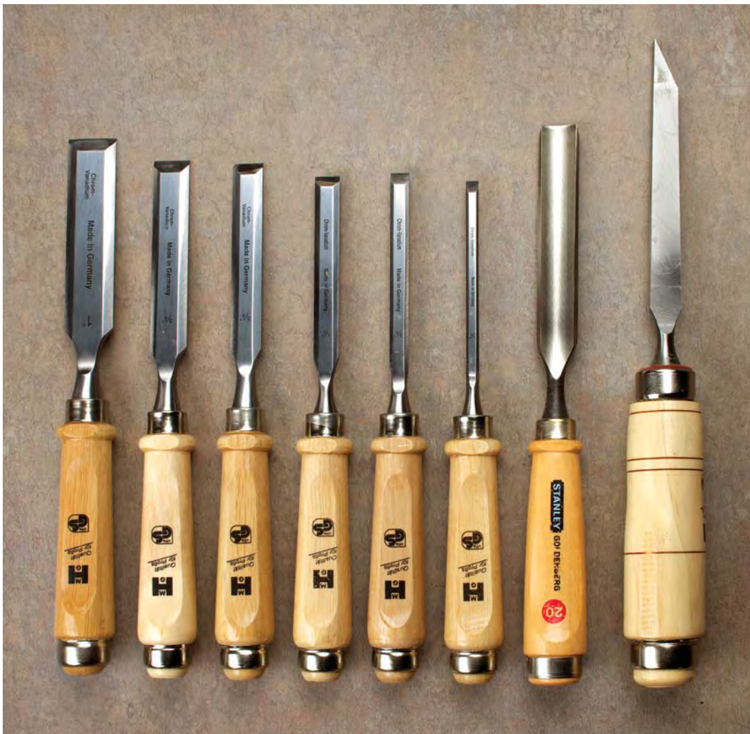
From left, a set of wood-handled bevel chisels, ranging in size from 1" to \frac{1}{8} ". The metal banding at the top of the chisel handle makes it possible to strike these wood chisels with a mallet. Next to the bevel chisels is a \frac{5}{8} " gouge, and at the far-right a \frac{1}{8} " firmer chisel (seen from the side).
