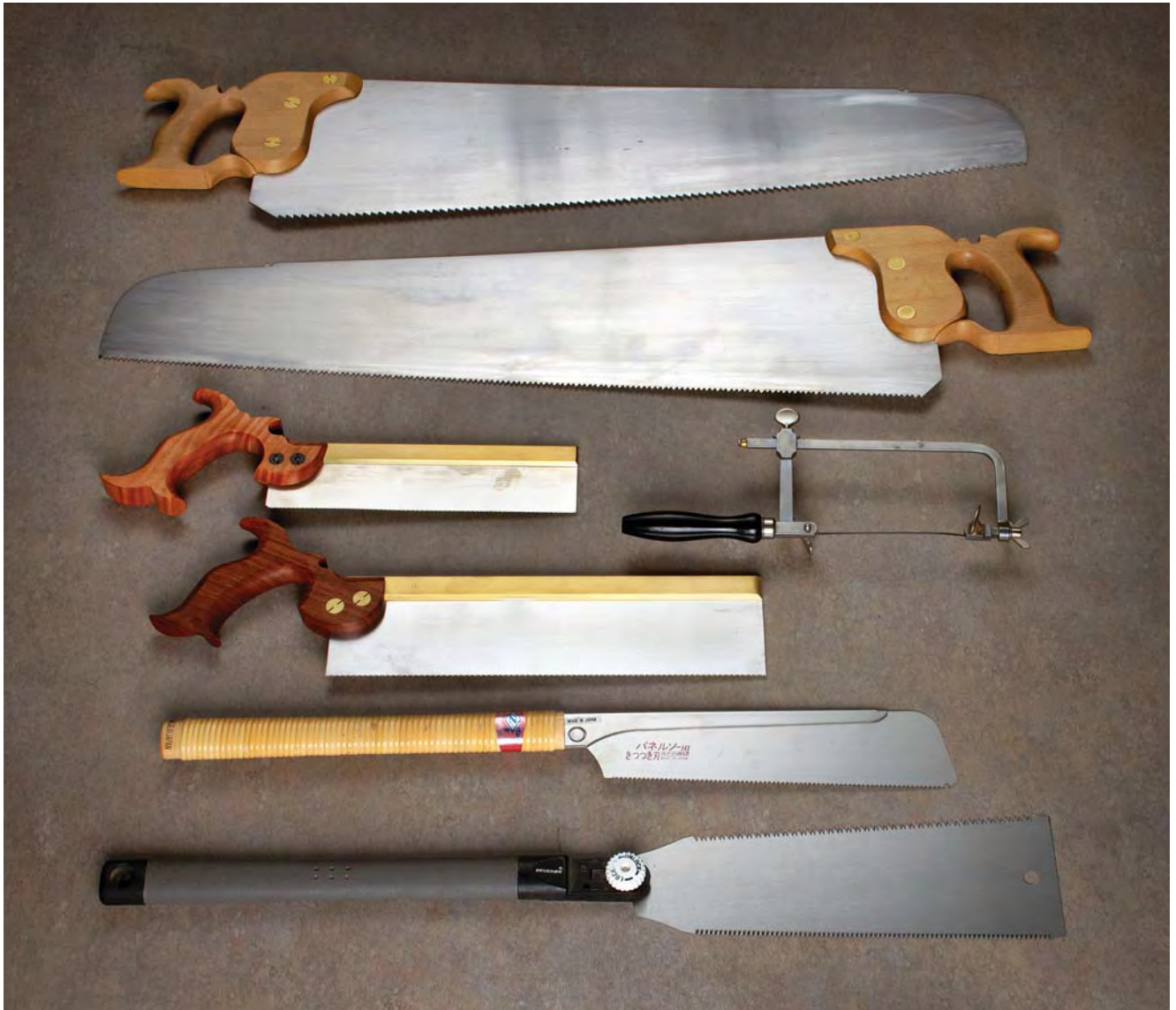
Handsaws, from top to bottom: rip; crosscut; dovetail; coping (right); backed saw; traditional Ryoba Japanese saw, and a contemporary Dozuki Japanese saw.
