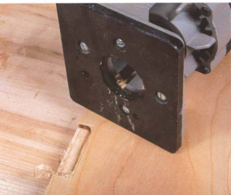
PHOTO C: When routing the waste from the mortise, stay \frac{1}{16} in. or so inside the scribed lines.
