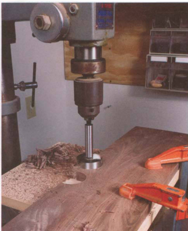
PHOTO K: To create each drawer front hand hole, drill two holes with a 2-in.-diameter bit; then saw between the lower quadrants with a jigsaw or bandsaw to complete the cutout.
