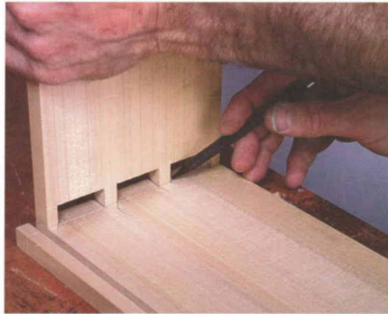
PHOTO E: The tails are marked from the completed pins. Afterward, layout lines are extended squarely across the end of the tail board.
