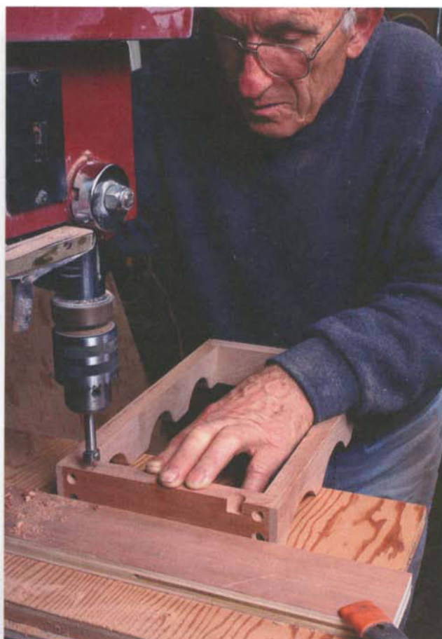
PHOTO C: Schneider uses a \frac{5}{8} -in.-diameter Forstner bit to drill the shelf-support notches in the undersides of the bottle rack side holes.
