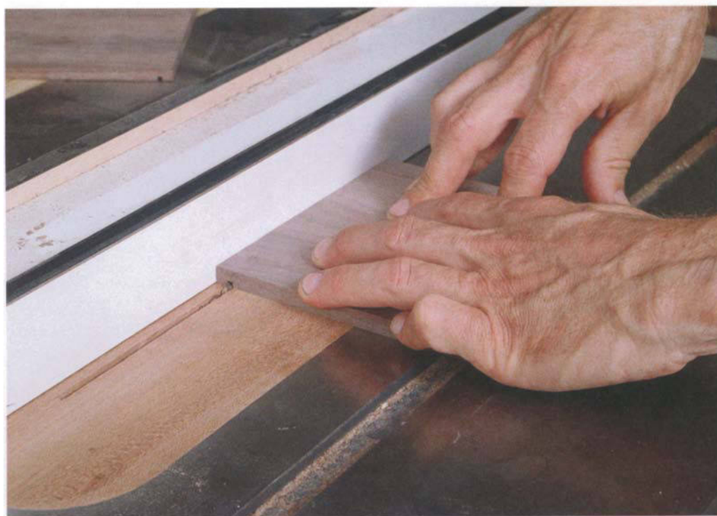
PHOTO A: Press the stock firmly against the saw table to ensure dadoes of consistent depth.
