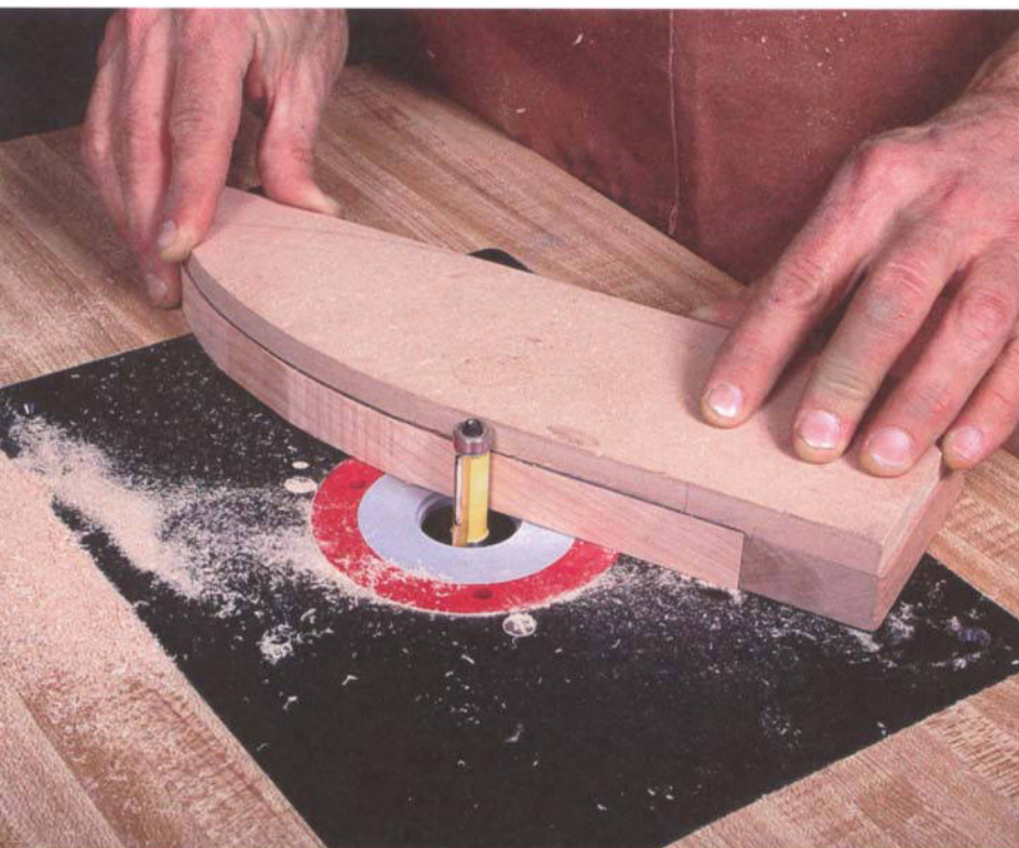
PHOTO J: Turn the template jig upside down for template routing the convex curve. Feed the workpiece right to left against the bit.
