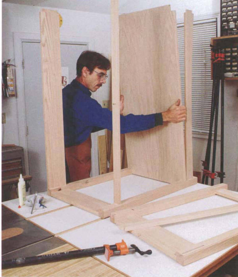
PHOTO E: After gluing up the two side assemblies and notching the platform, glue and insert the rear apron, lower rail, and stretchers to one side assembly. Then slip one end of the platform unglued between the legs, and glue on the opposite side assembly.
