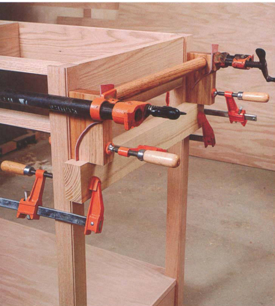
PHOTO I: To attach the bar brackets, set them on a length of thick scrap clamped to the legs. Clamp the lower section of each bracket using the curved offcuts. Thick leather scraps protect the finish.
