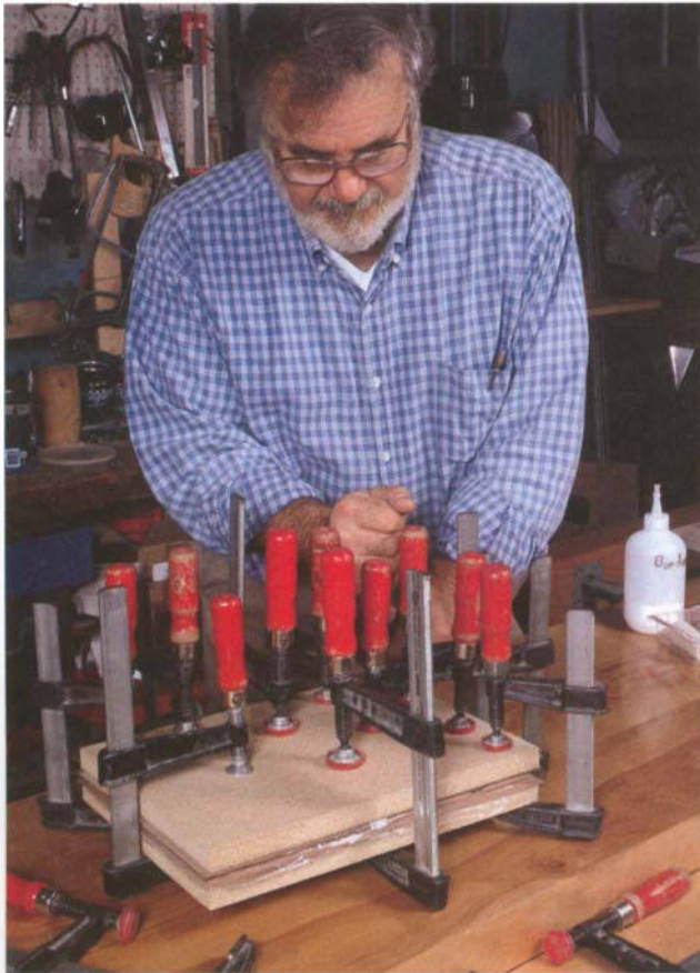
PHOTO A: Spooner glues the veneer to both faces of the top panel, covers the veneer faces with plastic wrap, and clamps the assembly between MDF cauls.
