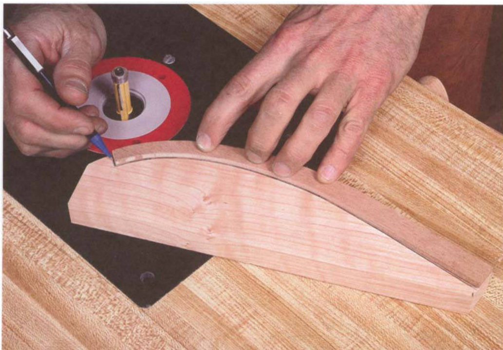
PHOTO K: After template routing the convex edge, line up the plywood slat pattern with the bottom of the blank and trace the concave edge and top onto the blank for bandsawing.
