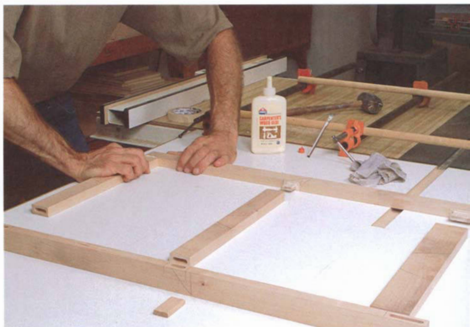
PHOTO B: To ease assembly, connect and align one half of the face frame before the glue sets up tack. Then glue on the other stile. The \frac{3}{4} -in.-diameter dowels center the clamp pressure on the stiles, preventing them from buckling under clamp pressure.
