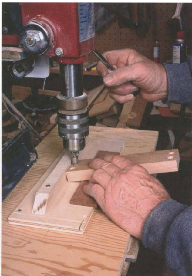
PHOTO B: Drill and countersink clearance holes in the end rails of the bottle racks for attachment to the front rails. To angle the holes, rest the workpiece on a \frac{3}{8} -in.-thick shim set back 1\frac{1}{4} in. from the drill press fence.
