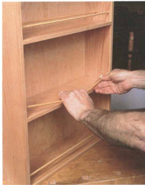
PHOTO B: After gluing on the slightly long shelf edging, nip it off ¼ in. from the end. Use the rip fence as a stop.
