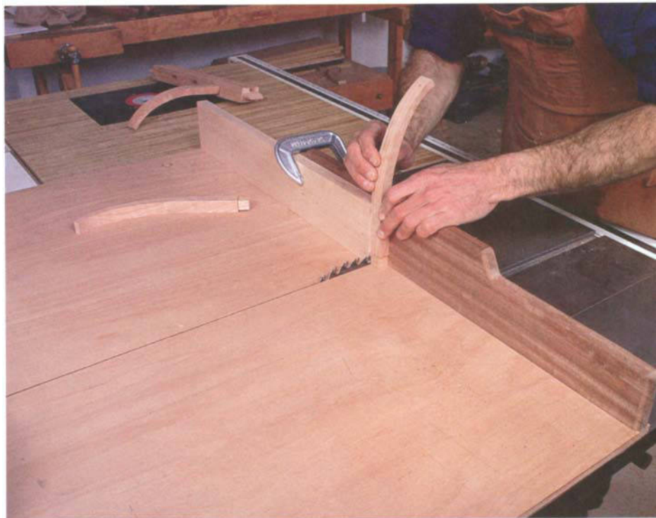
PHOTO M: Support the slat against a stop block clamped to a crosscut sled to cut the tenon cheeks. Afterward, pare to the tenon shoulders with a sharp chisel.
