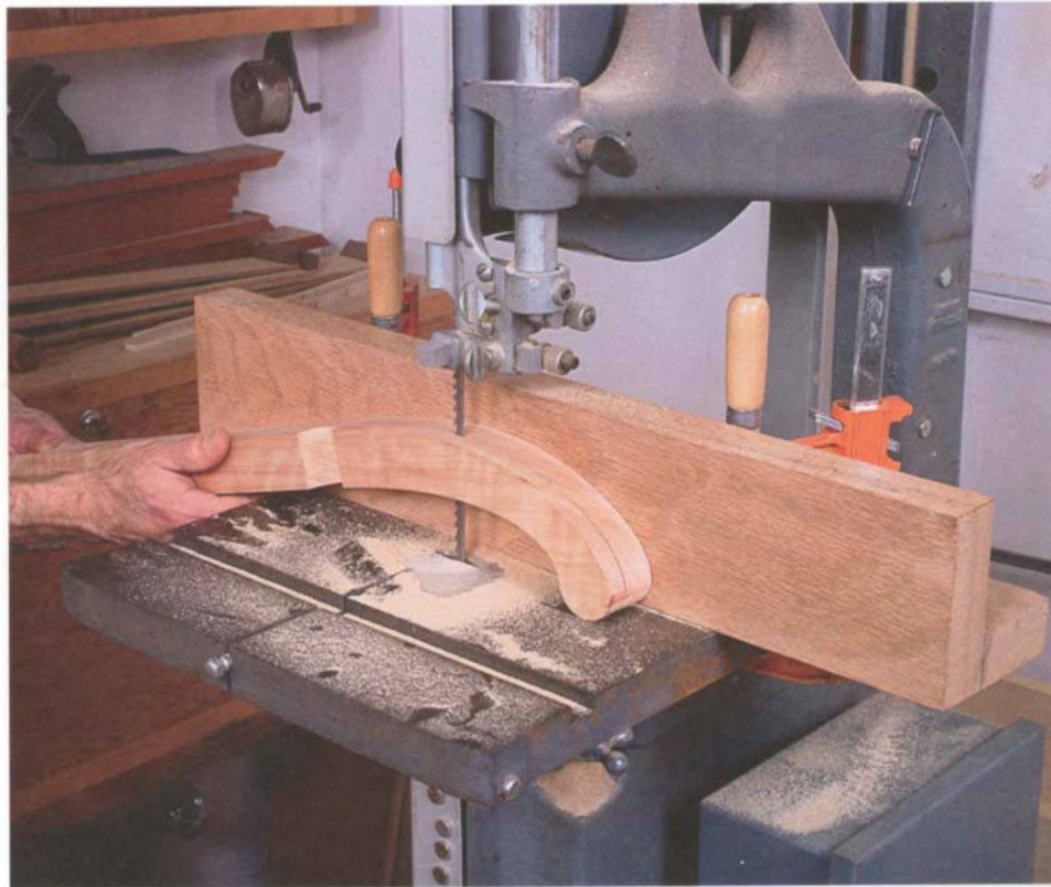
PHOTO G: After drilling the curve in the inner face of the leg, use a bandsaw fence to guide the straight cut at the top of the leg.
