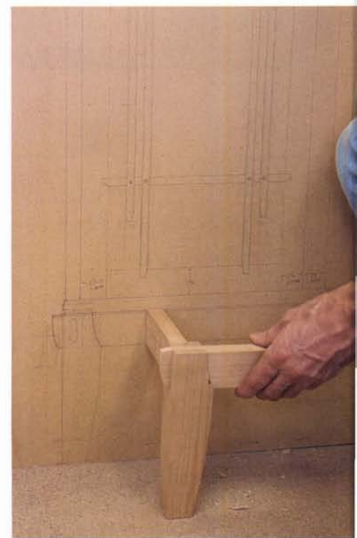
Making a mock-up. A good way to see whether your design works is by making a partial mock-up out of poplar or alder.
