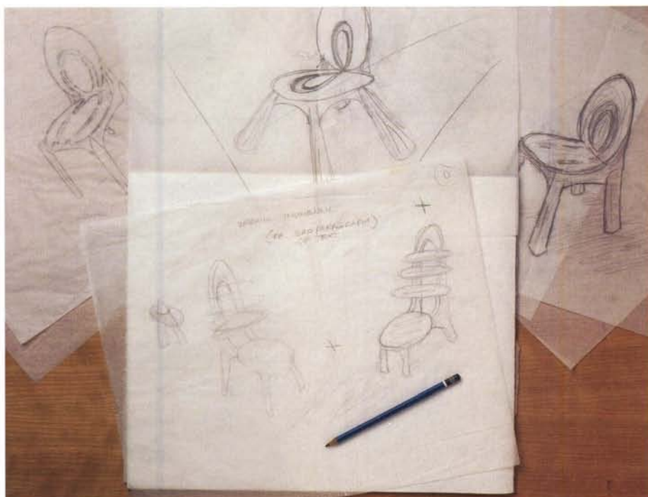
A transparent exercise. By tracing and redrawing your original sketch on a succession of pieces of tracing paper, you can develop a design in an efficient and controlled way.
