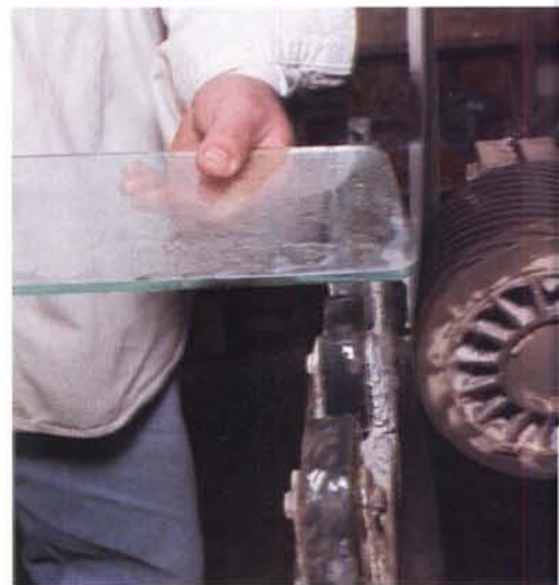
Taking the edge off. An upright sander in a glass shop can round the edges of glass or shave away a sixteenth of an inch.
