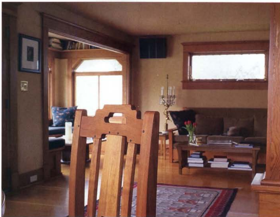
Less graceful Greene and Greene. Peart deliberately made the chairs less sculptural than the originals, designed for Greene and Greene's Gamble House, thickening the side posts and crest rail to avoid seeming too delicate in contrast with the surrounding furniture.
