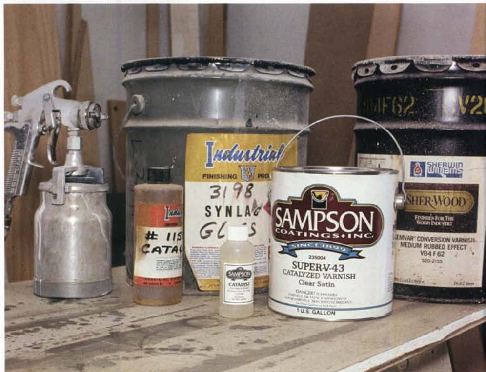
Catalyzed finishes are a two-part mix. Catalyst and resin are mixed and then sprayed on to form a tough, durable finish. Both lacquers and varnishes are available.
