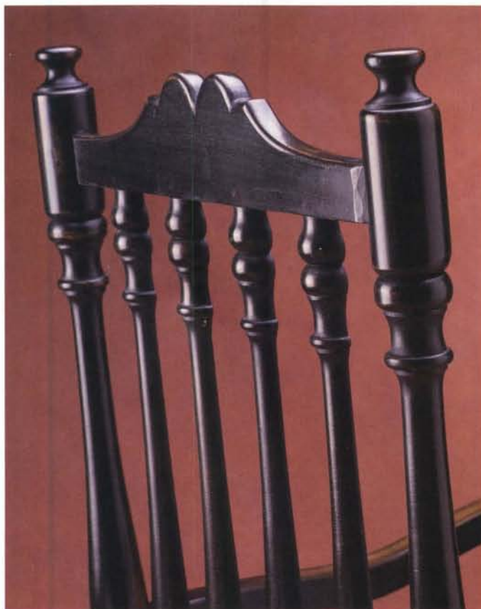
Splitting the spindle. The spindles are made by gluing together two maple blanks with paper in between, turning them as a whole, and then splitting them apart into identical pieces. The profile of the split spindles matches that of the back legs.
