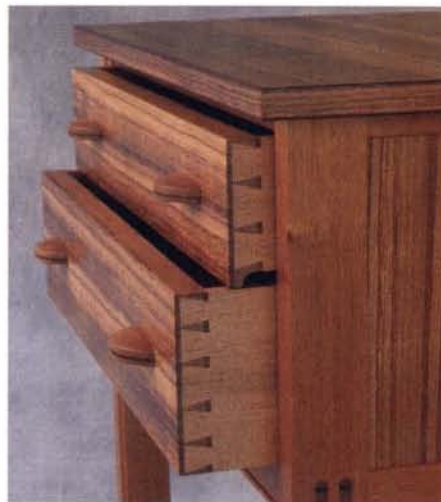
Sliding on paraffin. Nothing but paraffin comes between these drawers and the drawer pockets they slip into. The insides of the drawers are lightly finished with shellac.
