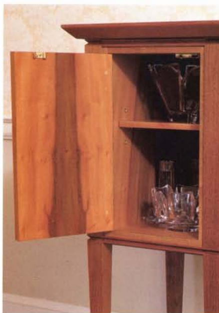
Hidden hardware. Touch latches and concealed hinges keep the sideboard's exterior free of hardware.
