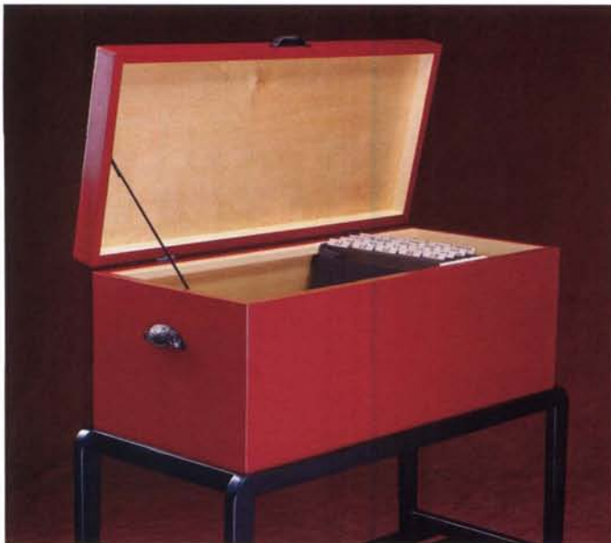
Detailed files. Poplar guides hold the hanging folders. The lid is held open by a single black, braided cord.
