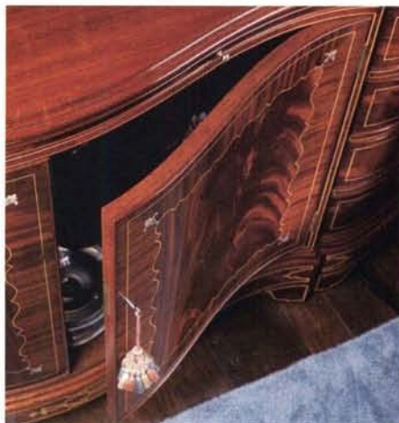
Improved, not just new. The serpentine doors were the only feature made in a new way. To keep the veneer from cracking, the doors were laminated rather than coopered out of solid wood.
