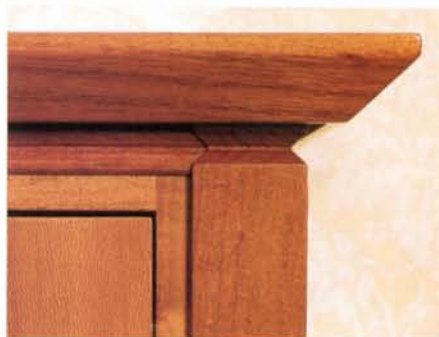
Grooves that bind. Legs and molding stand proud of the doors and panels but a V-groove (above) provides a visual binding to the carcass.
