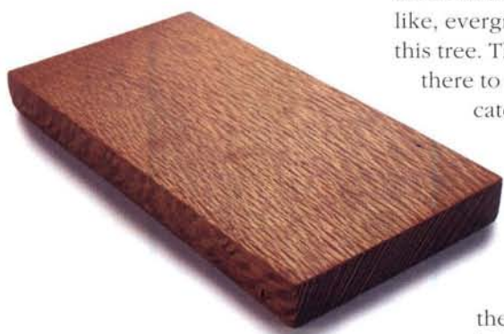
Rife with ray fleck. Lacewood's prominent rays are evident any way you slice it.
