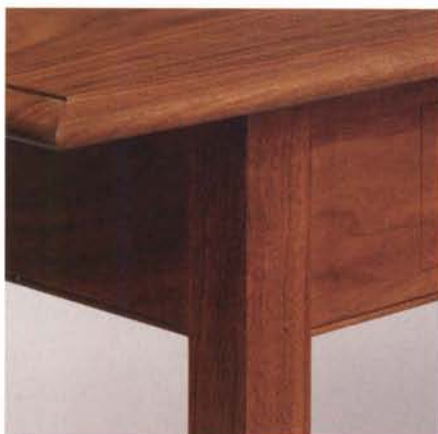
Leg with linear figure. By carefully laying out the leg stock, each side of the square portion of these turned legs has straight, consistent figure.
