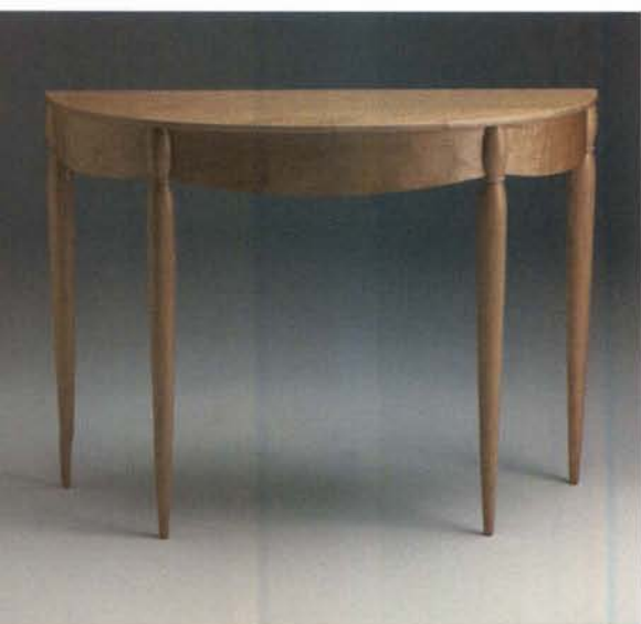
All done with dividers. The height of this curly maple demilune determined the other proportions. The turned rings on the legs are meant to support the swag of the aprons.
