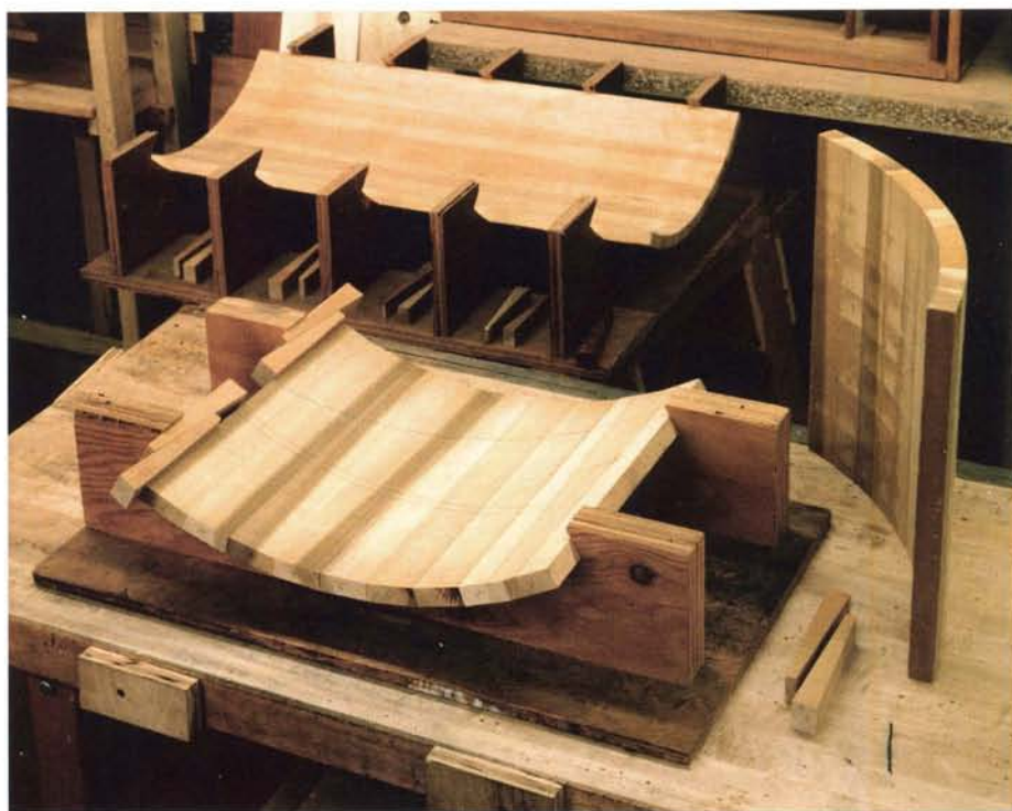
The cooper's art. Coopering is taken from the craft of making wooden casks and tubs. Coopered doors for the sideboard (left) were made in a simple, two-station form (below).
