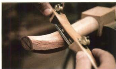
Dressing the foot. The author uses a spokeshave to give each foot its final shape.
