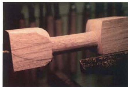
Foot is off center. The center part of the splayed leg is turned on the lathe. The rest is cut out on a bandsaw and shaped by hand.
