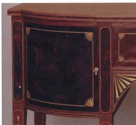
The cooper's art. Coopering is taken from the craft of making wooden casks and tubs. Coopered doors for the sideboard (left) were made in a simple, two-station form (below).
