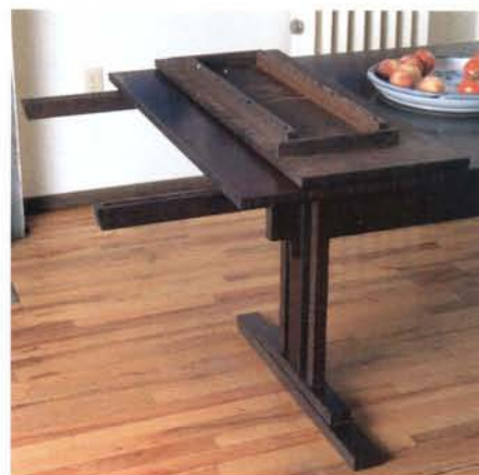
Simplified table leaves. The leaves on this table drop into slots in the sliding aprons to make the table longer.
