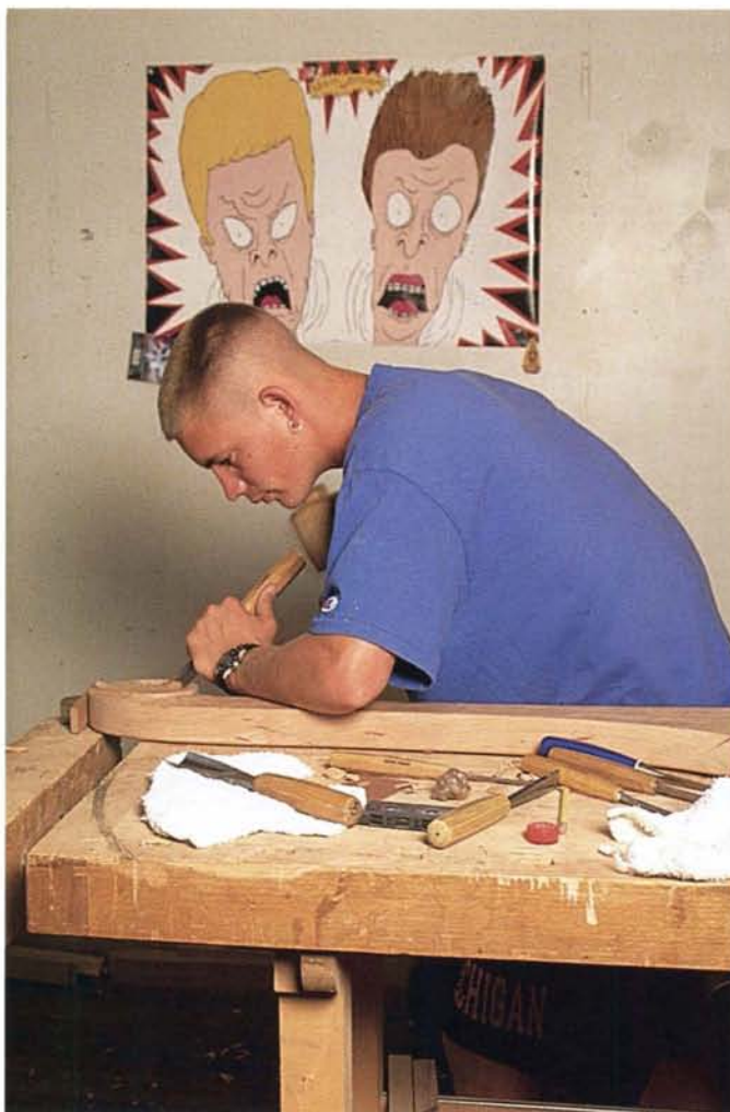
Handwork is the essential ingredient. Bill Tastleton, 20, carves the trademark curl in the headboard of a sleigh bed. "Furniture should be fun to make," Shackleton says.
