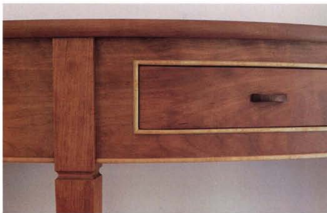
Skirt fitting. Maple cockbeading dresses up the skirt and balances the cove on the leg.
