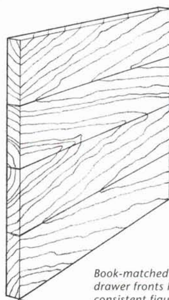
Boards are rotated so that top and bottom pairs of drawer fronts are book-matched.
