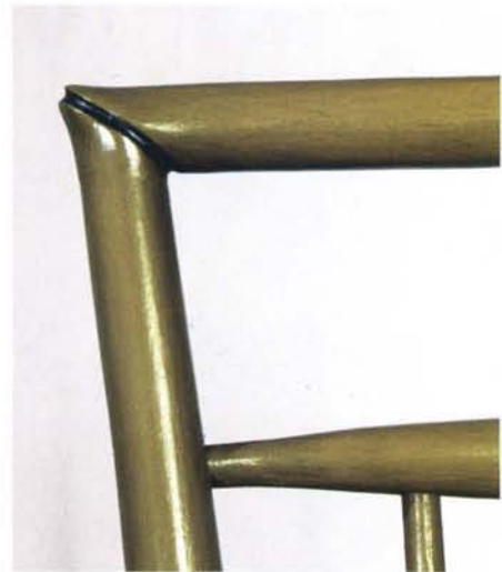
Pucker up. The false miter joint between the crest rail and the post is carved in a grooved and puckered shape called a duck bill.
