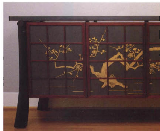
Cabinet draped in linen. Linen was glued onto this plywood cabinet before it was painted, giving texture to the surface.
