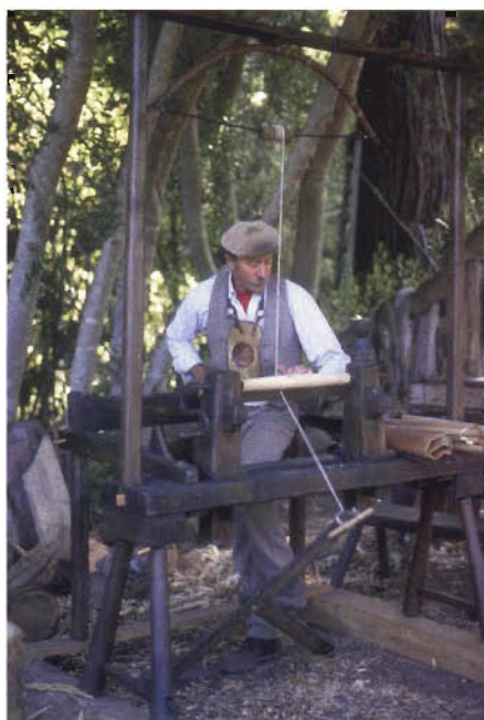
Ancient tool. Don Weber used a pole lathe to turn his chair parts.
