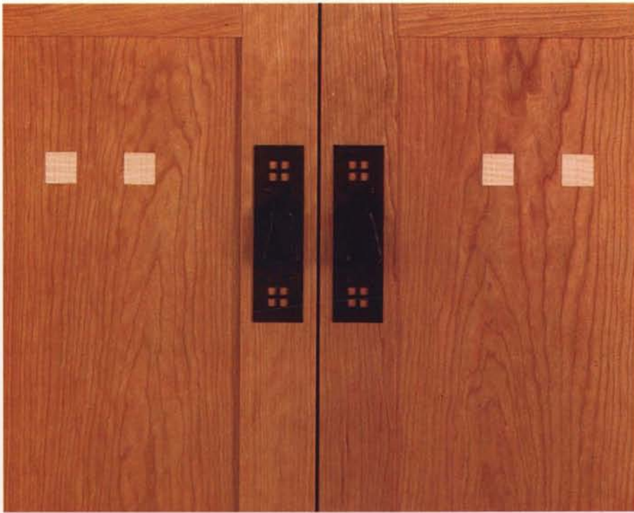
Period pulls cinch an already tight design. The motif of four squares in the pulls, picked up in the long stretcher, also determined the size and location of the inlaid maple squares.
