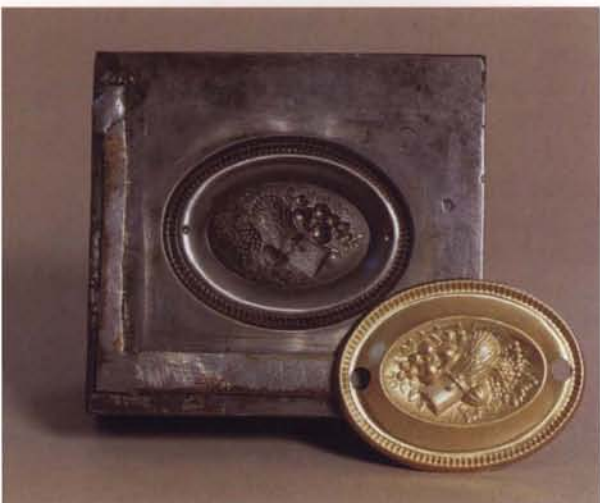
Reproductions can capture original details. This hand-carved die and the Hepplewhite-style backplate made from it by Horton Brasses show the level of detail possible in brass reproduction hardware.
