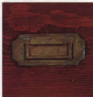
Campaign-style pulls are mortised flush with the face of the chest.
