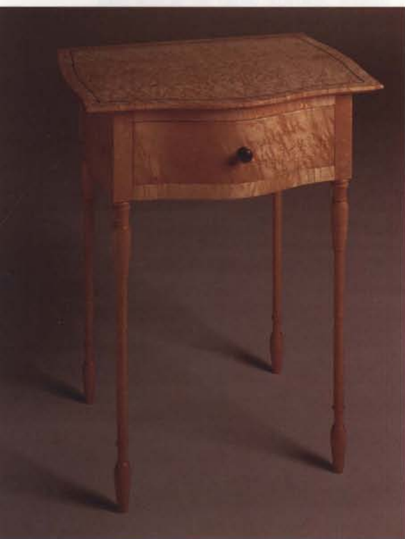
A serpentine side table. The gentle serpentine curves of this table, built by Lou Giorgio of Barrington, R. I., show the variety that can be achieved by manipulating arcs of a circle.
