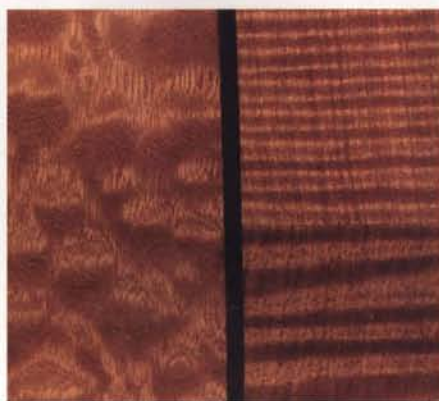
Highly figured veneers. Pommel sapele and fiddleback makore are both African hardwoods. Pommel, meaning rounded or knob-like, accurately describes the figure of the sapele veneer, shown at left.
