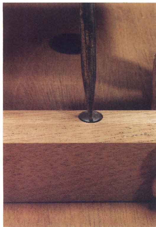
Screw in place with no glue. Be sure the screws are the correct length, so they don't come through the top of the table.
