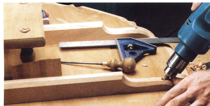
The batten is attached to the table top with three screws, one in the center, and one about 1 1/4" from the end. The end screws are angled slightly in. Put a piece of veneer or 1/16" poster board between the batten and the birdcage as a spacer, and drill pilot holes.
