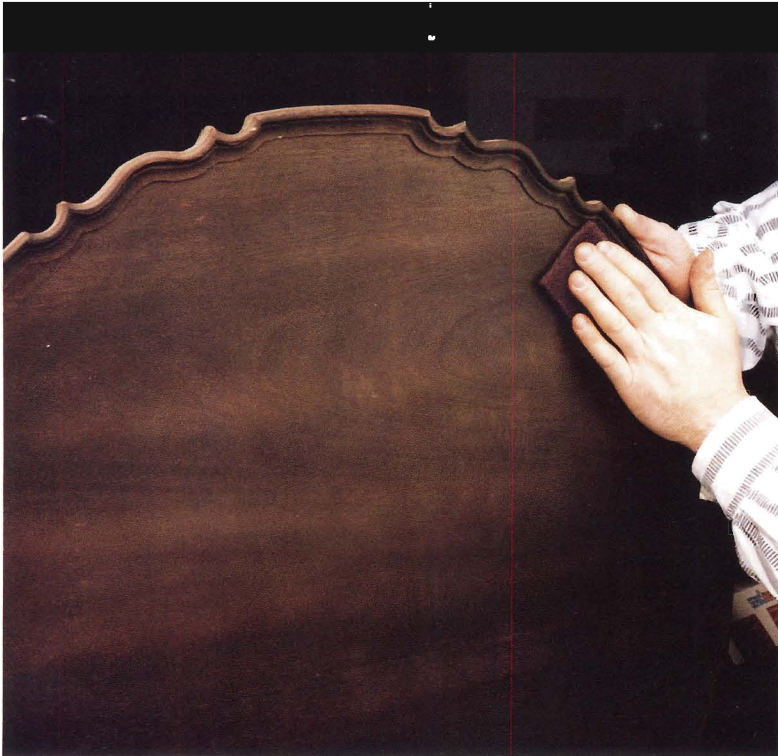
This is rubbed down with a fine pad of Scotchbrite™.
