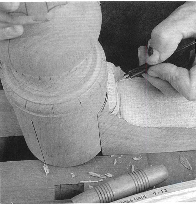
Test fit the leg. There is a little gap on this side that will need adjustment by a slight trimming of the dovetail.
