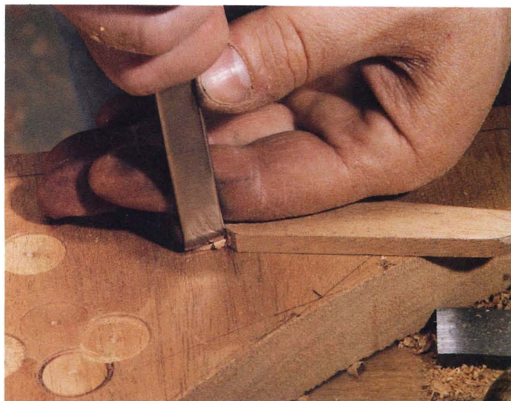
Cut the key on the bandsaw from a piece of 1/4" mahogany and clean it up with a chisel and sandpaper.
