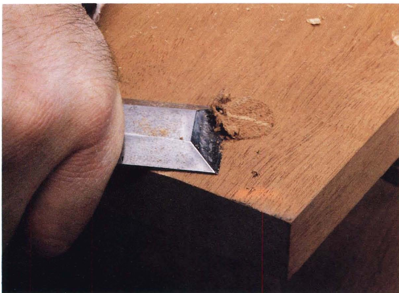
and smooth them with a chisel. Then you can prepare the surfaces of the birdcage for finishing.
