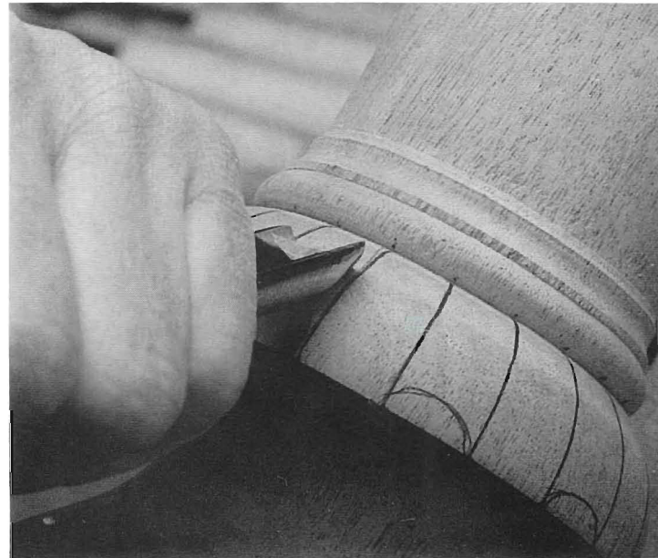
Starting part way up the concave segment, work your way up. By starting here you relieve the pressure on the wood and get a cleaner cut.
