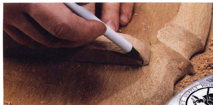
Lay the batten in place and mark where the outside edge of the end needs to be rounded off. Shape it with chisel or rasp.
