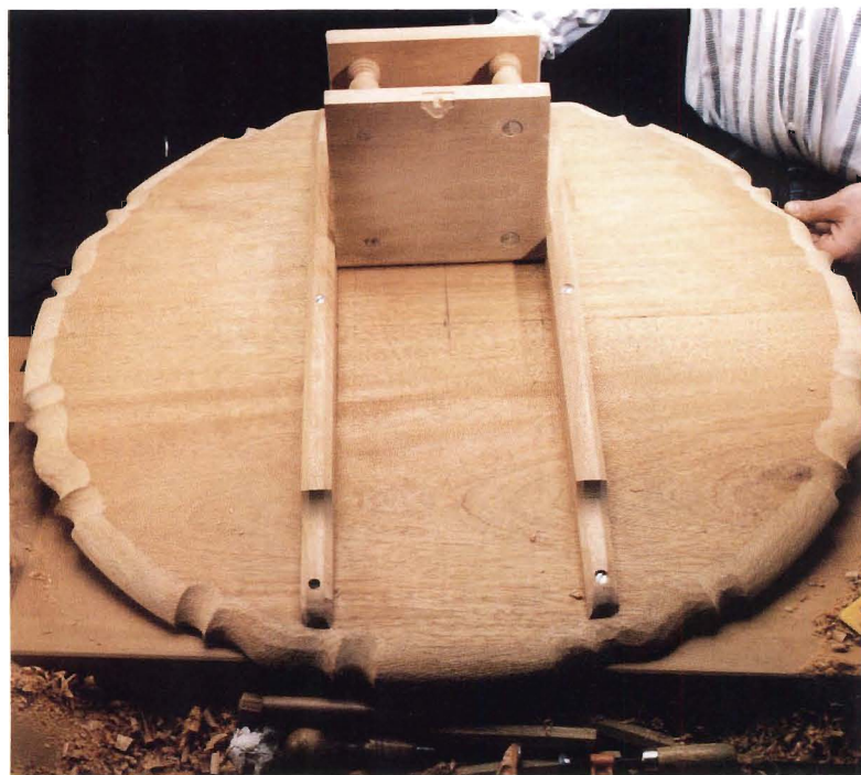
The batten and birdcage assembly in place.
