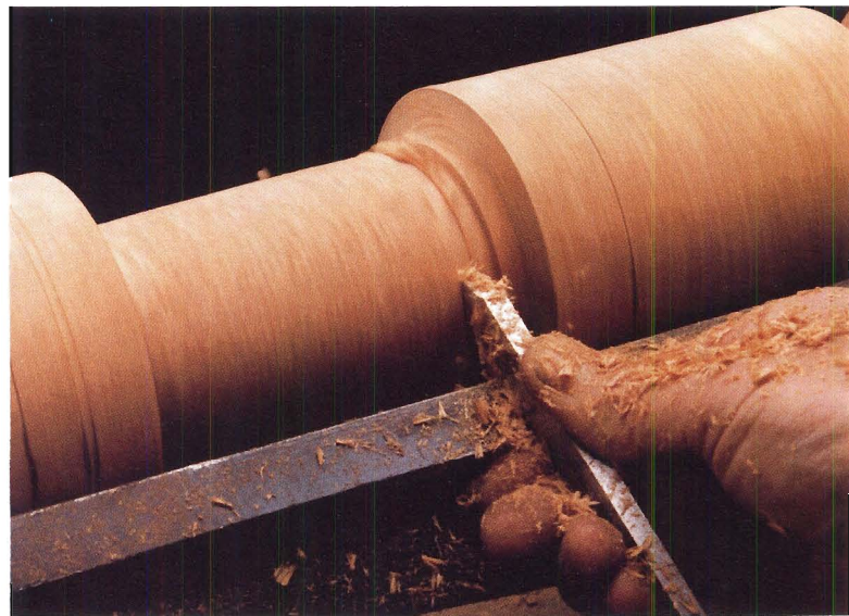
Establish the base of the flat area above the cove at 2\frac{1}{4} ".
