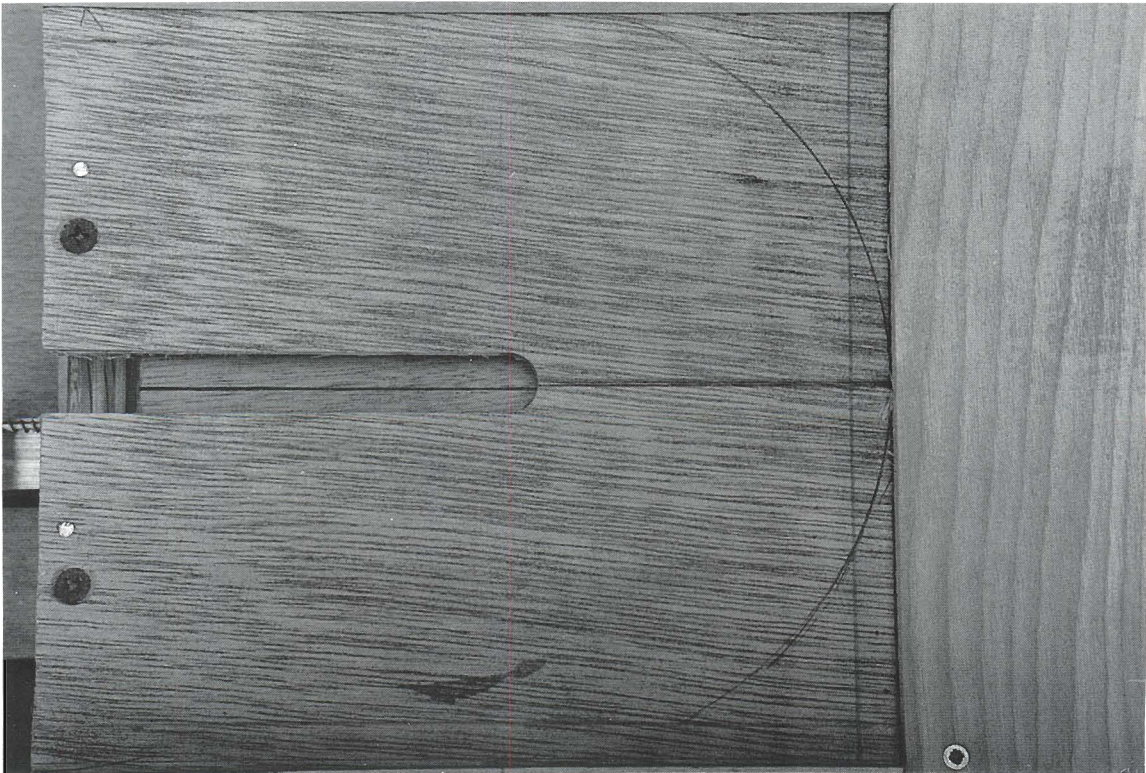
The line on the jig aligns with the line we drew on the base of the table pedestal.
