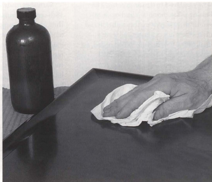
The final step in finishing is to polish the surface. Here, a linseed-oil polish has been applied and buffed off.
