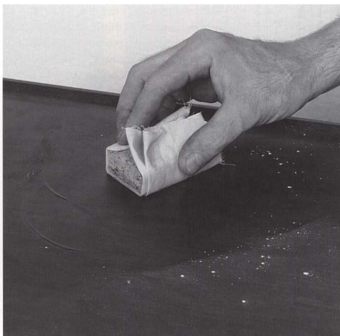
Period cabinetmakers leveled the surface of the finish by rubbing it with pumice and linseed oil using a pad backed by a cork block. The modern equivalent is to use steel wool or a waterproof silicon-carbide sandpaper.
