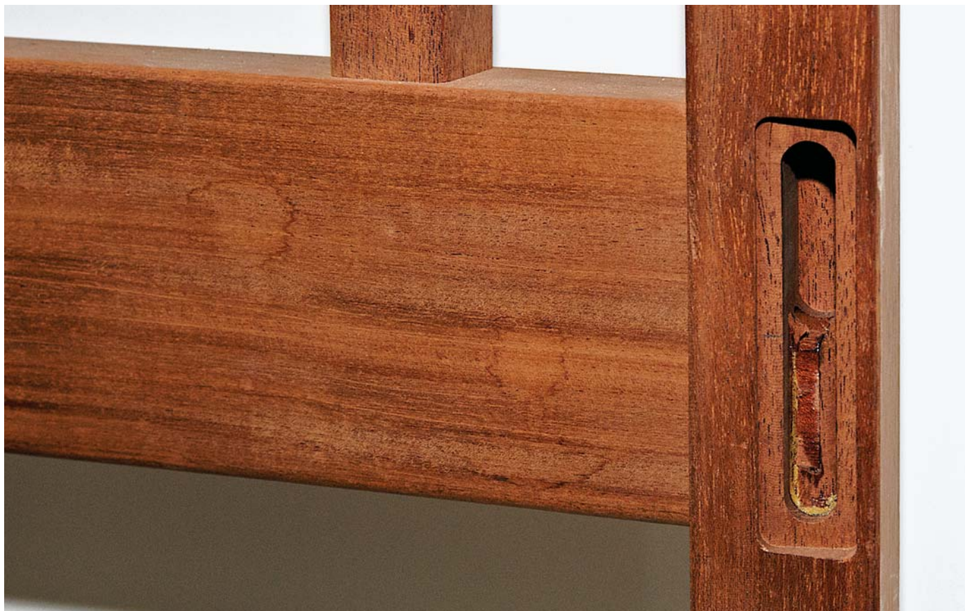
ABOVE A modern housed mortise on a recreation of a Blacker dining room chair. It creates significant additional labor in the name of aesthetics. Detail, mock-up of dining room chair, Jim Ipekjian.
