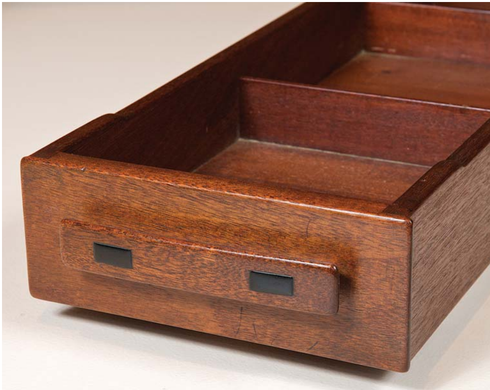
LEFT A simple, effective joint that remains tight after 100 years. On this drawer, the sides are stepped both front and back. Detail (full view on p.128), drawer from bedroom desk, 1907-09, Robert R. Blacker house.
