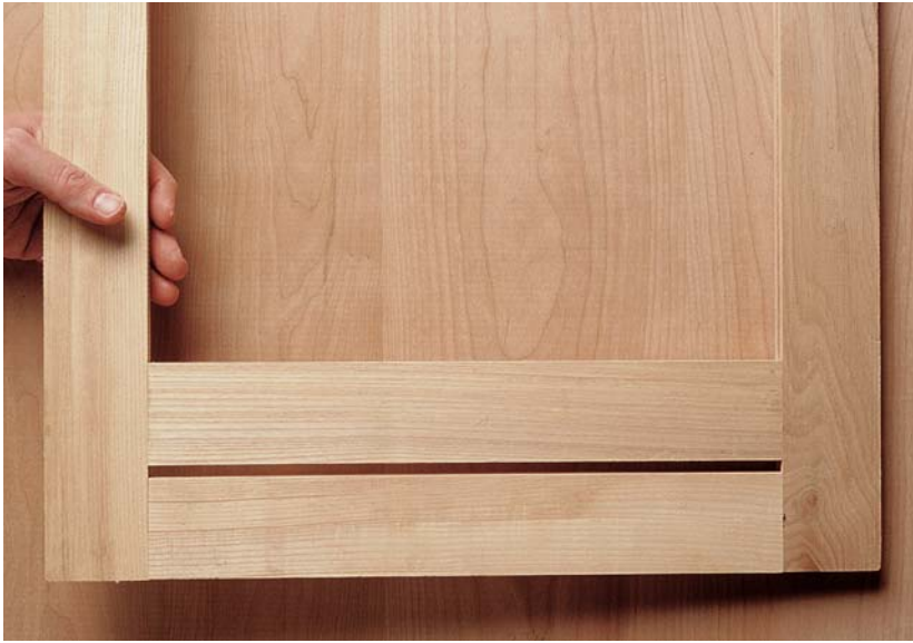
Photo F: Doubled-up stiles on the inner frames prevent the wood movement problems you might experience with a single wide stile.
