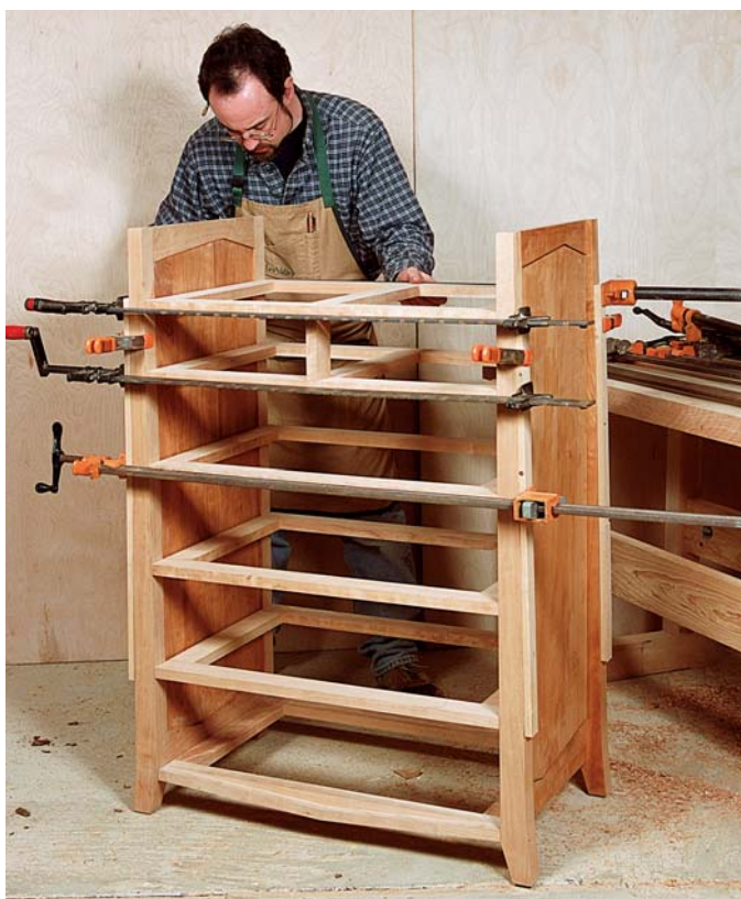
Photo L: After the second side is seated, right the unit and apply clamps parallel to each web frame, across the front and the back. The spring clamps hold pad strips that protect the posts.
