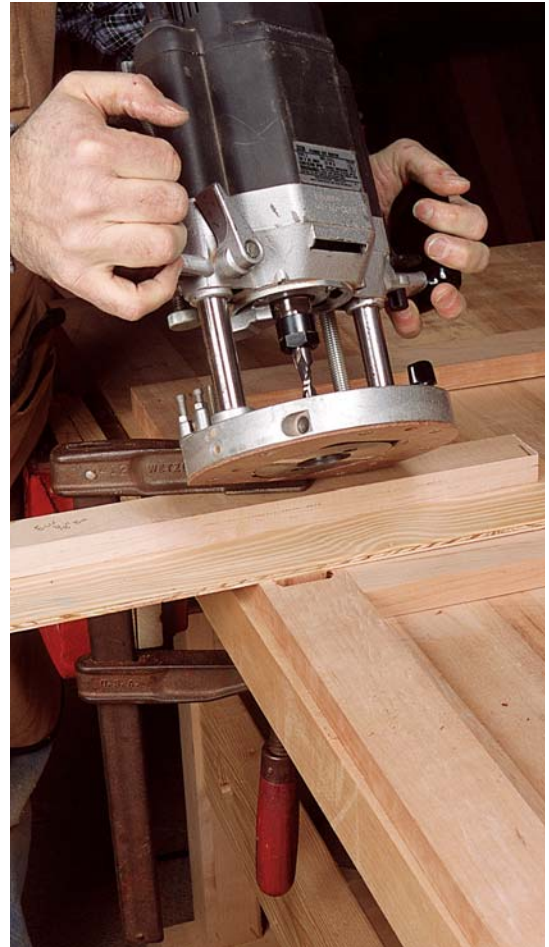
Photo J: The vertical drawer dividers are joined to the web frames with mortises and loose tenons. Rout the mortises after the frames are glued up.
