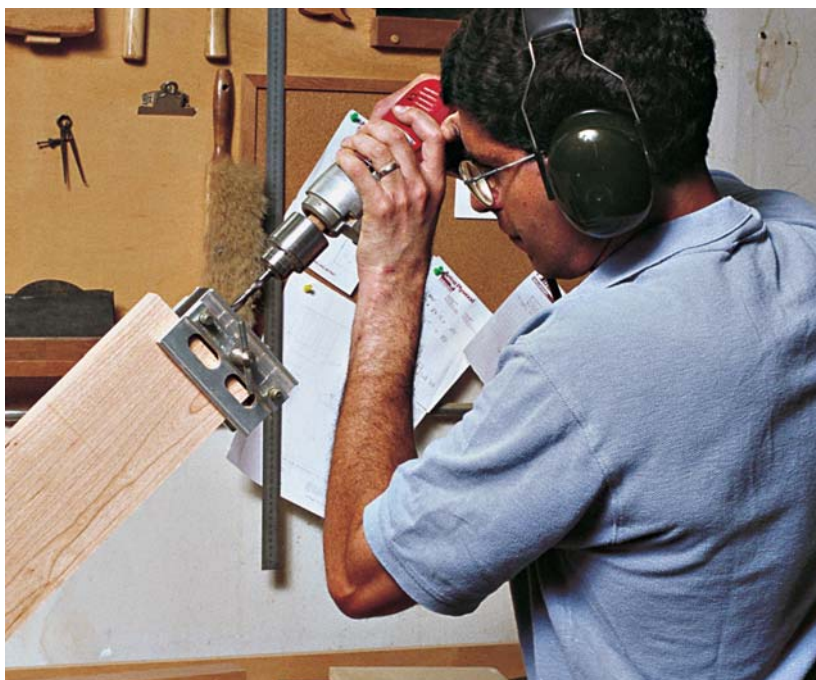
Photo F: Drill the \frac{3}{8} -in. bolt hole in the side rail with a self-centering doweling jig. It centers the hole well and is simple to use.
