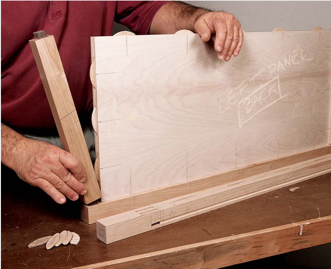
Photo E: Glue tenons and biscuits into the legs, and biscuits into the panel ends. Fit a rail and the panel to a leg. Add the second rail, and the second leg.
