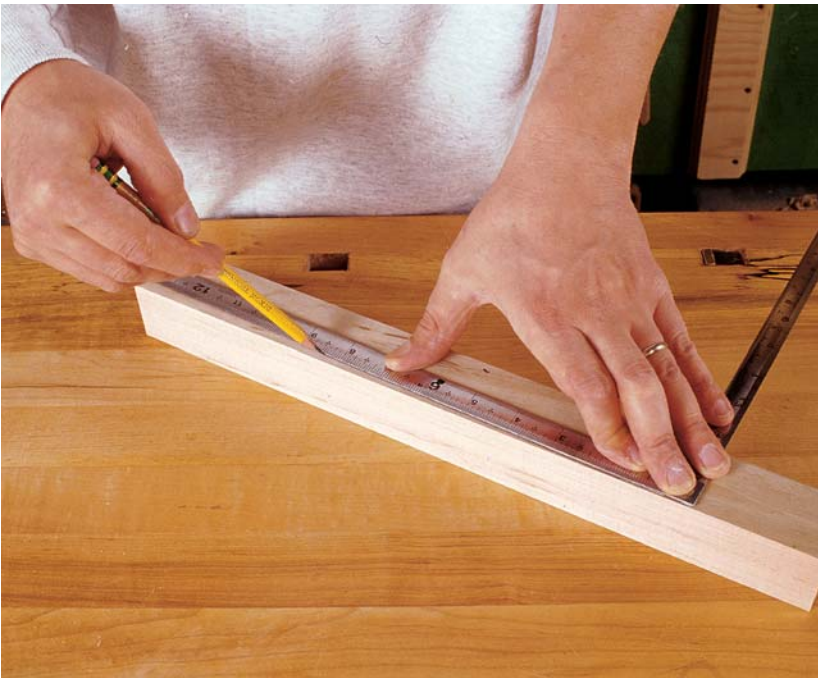
Photo D: The tapers on the inside faces of the legs begin 4 \frac{1}{8} in. down from the top and diminish to 1 \frac{1}{8} in. at the foot.
