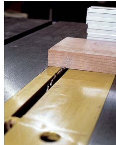
Photo K: The apron piece is positioned so that the edge of the blade meets the mark you made with the knife.
