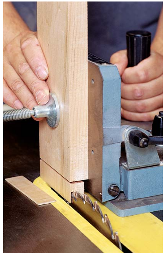
Photo M: I use a commercial tenon jig to cut faces, but a shopmade jig will work as well.
