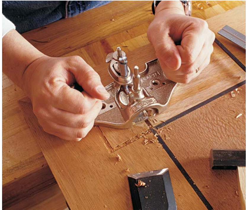
Photo F: Using a router plane fitted with a sharp \frac{1}{4} -in.-wide blade, plane out the waste between the groove walls. Take light passes, adjusting the blade downward as you go.
