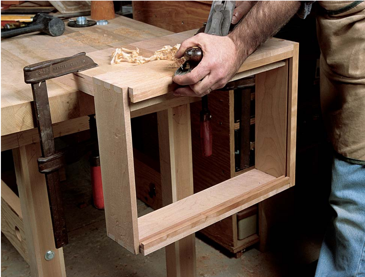
Photo R: With the pins deliberately cut a hair short, the sides are just proud of the pin ends in the assembled drawer. Burton can quickly handplane them flush with the pins.
