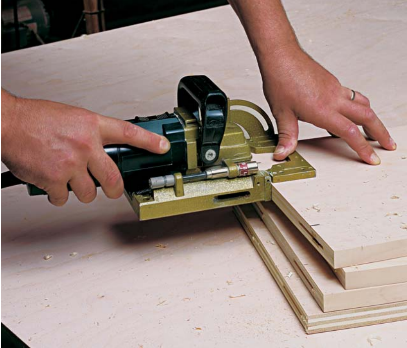
Photo B: Cut biscuit slots in the ends of the fixed shelves and at the top of the sides.
