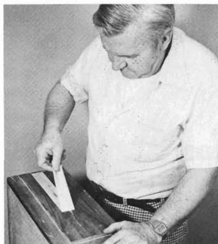
Now pull off the masking tape. The butted pieces should fit tightly together. You can see the joint — but just barely. The finishing process will hide it completely.
