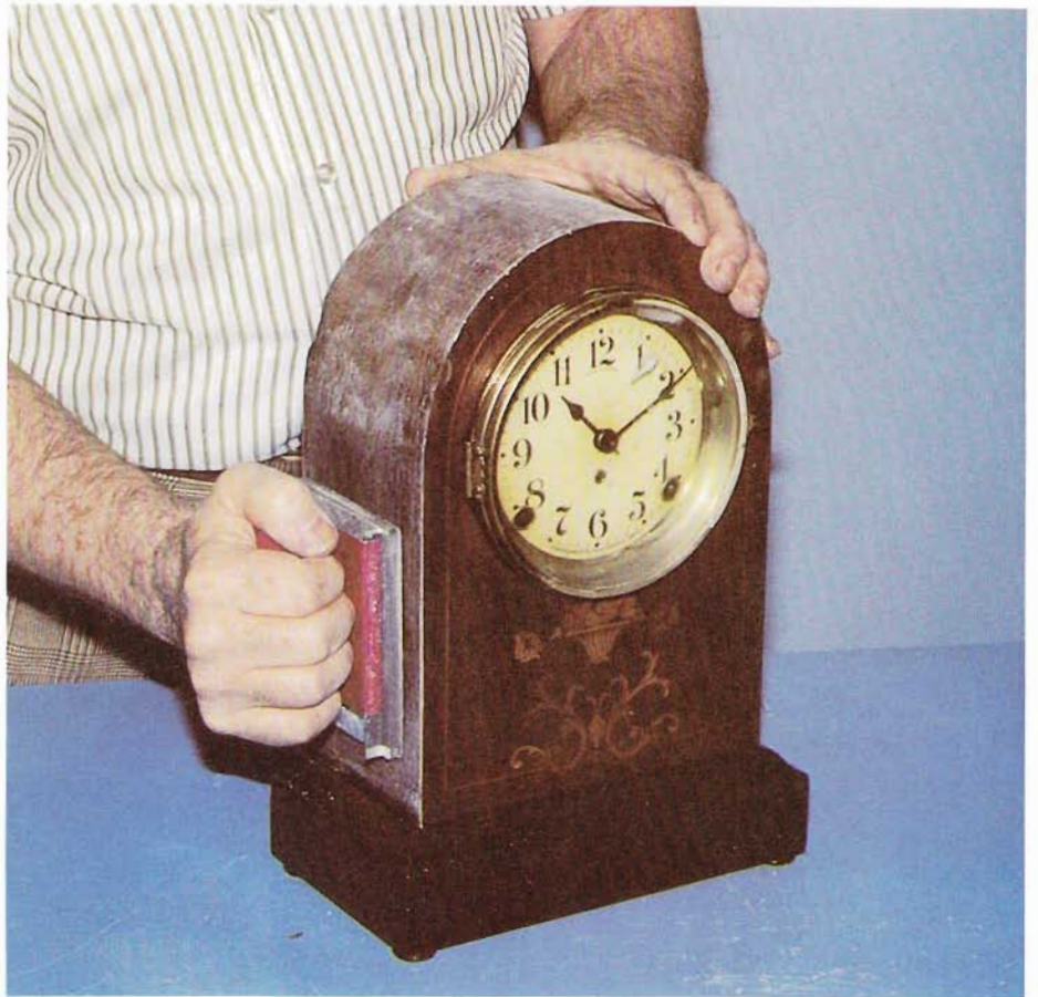
9 Shellac will fill sandpaper quickly so keep a toothbrush handy to clean the paper frequently.
