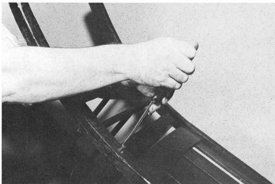
If you damage or break the plug in getting it out, you can buy a new plug to replace it. Be careful not to damage the wood frame.
