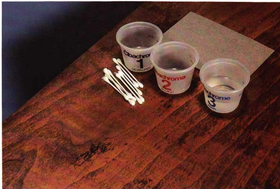
1 The black marks on this surface were caused by water. They are in the wood, not just in the finish. To get rid of them, you need these materials for bleaching: a two-part wood bleach you can buy at your home center; some vinegar; a lot of cotton swabs; and three little cups. The cups we use came from a photo developing kit and are numbered. This makes it easy to remember where each chemical is.
