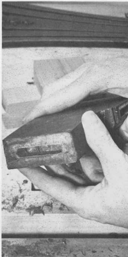
8 Here is the mortise with the tenon removed.
