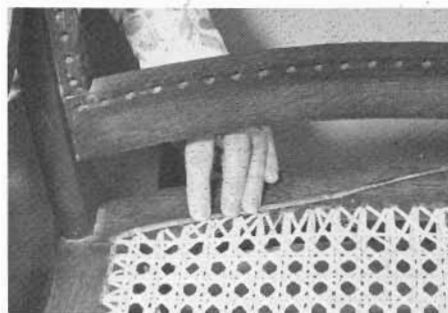
To make a neat binding tie at each hole, hold the binding cane flat and directly across the hole as the weaving cane is drawn tight.
