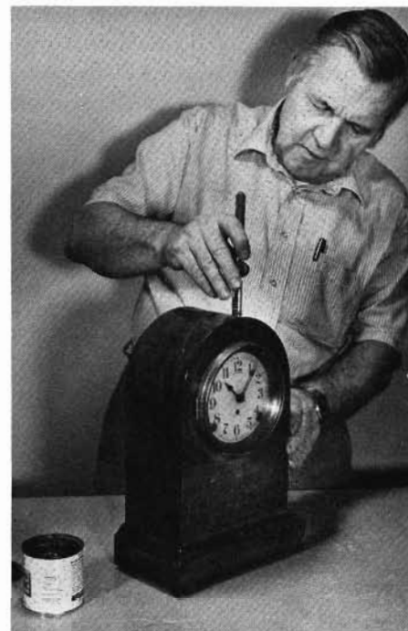
Shellac should be applied carefully to avoid air bubbles. The material is laid down, as is varnish. Be sure that the brush marks overlap.
