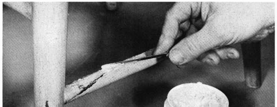
To repair splits and dents, try latex wood filler — probably the easiest repair product on the market. It accepts stain well, does not shrink much, and can be sanded when dry.
