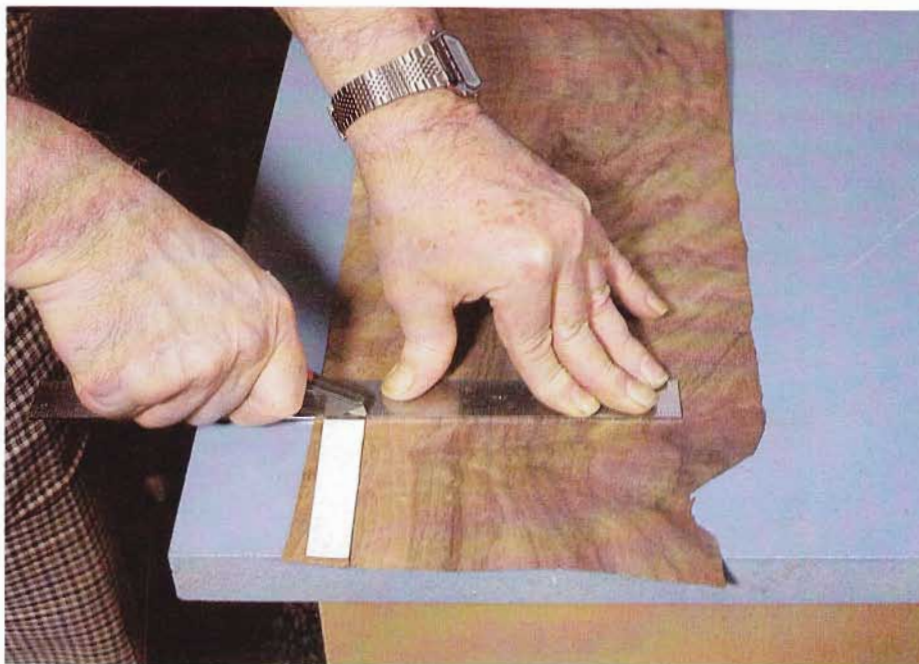
7 The next step is to cut a small cardboard pattern. Cut and fit until the cardboard is an exact fit in the repair area. Use the pattern to cut out the patch. Move it around the veneer sheet until you find an area where the grain of the new veneer closely matches that of the veneer remaining on the old surface. Now use a straightedge and either a veneer saw or a craft knife to cut out the patch, carefully following the cardboard pattern as you cut.
