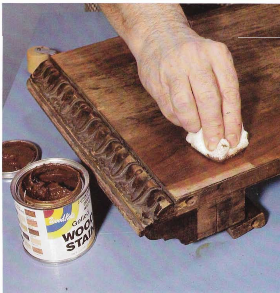
10 After the contact cement has set for a couple of hours, you can apply stain to the patch and the area around it. This is a demonstration project. If you were working on this table insert, you would have stripped the entire surface, and now would stain the whole surface so that the color would be even all over.
