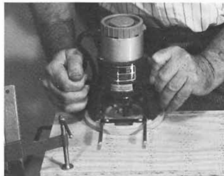
Cut sides for each drawer; we used 1 inch oak. The bottom fits into a groove at the bottom of each side; cut this with a router and a \frac{1}{4} inch dado bit. Trace dovetails on drawer fronts.
