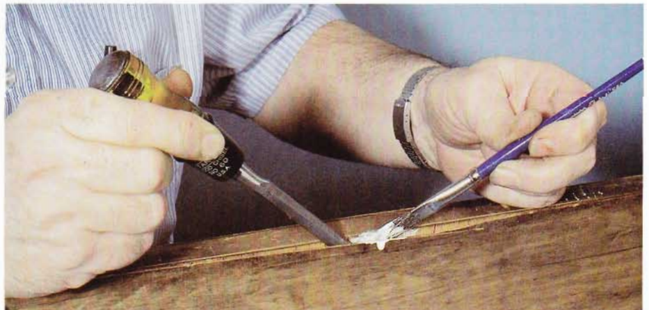
13 Examination shows the veneer to be lifted for only an inch or so in from the edge. The repair consists of working white glue into the opening. Use a brush. Hold the work vertical and apply plenty of glue so that it can run to the depth needed.
