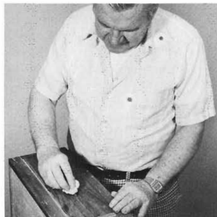
Use contact cement solvent to clean all contact cement and any gum from the masking tape off of the veneer. Caution: Test the solvent on a sample of the veneer before doing this, especially when veneering exotic woods. In rare cases, the solvent may cause the coloring in the wood to run.
