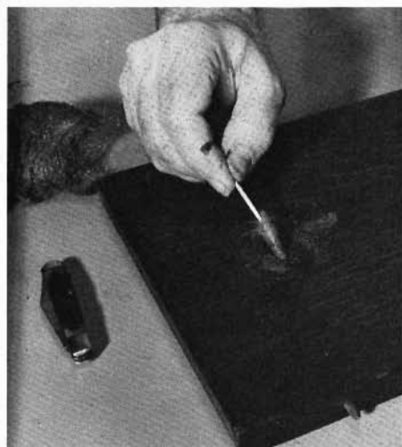
Another handy tool for making repairs in a finish is the abrasive swab — a small wad of steel wool wrapped around the toothpick.
