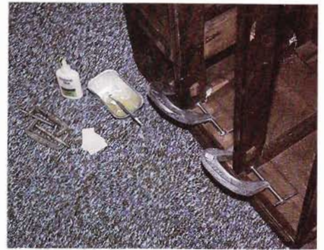
8 Now we reglue those frame members which need it, using a brush to apply the glue that has been squeezed into the aluminum dish.
