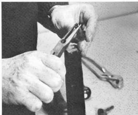
The end of the socket is slitted to form several "wings." Bent inward, these wings hold the caster up in the leg. Those shown have bent outward and no longer grip the caster. Use a pliers to bend them inward again.
