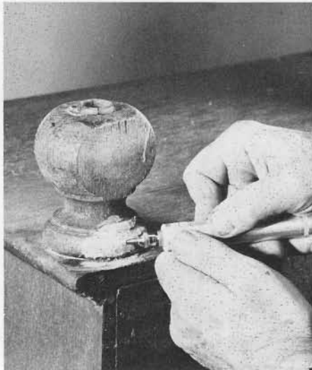
Next, using a Dremel Flex-Tool with a high-speed carving bit, we carved the new wood to match the original shape.
