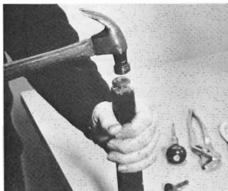
Reinsert the caster socket. Drive it all the way in; the teeth on the socket collar will dig into the wood of the leg.
