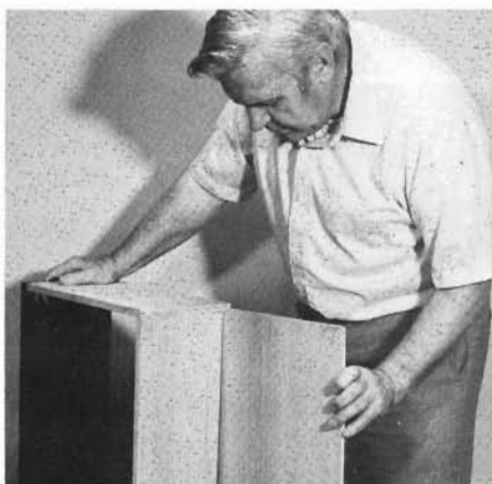
Drawers are assembled with new side and back panels and new bottoms made of \frac{1}{4} inch hardwood plywood, ordinary plywood or Masonite.
