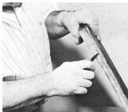
If all the glue is not removed, the two pieces will not fit together properly when they are reglued. Scrape away all excess glue.
