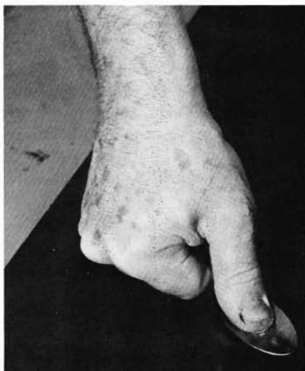
To determine the brittleness of a finish, press hard on the bowl of a spoon as you draw it across the surface. If the finish is brittle, it will crack and flake along the line you draw.
