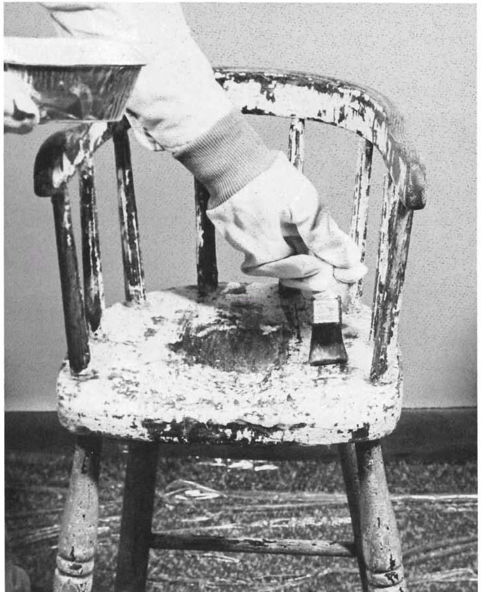
The stripper is laid on with a brush in a thick layer, and allowed to stand for perhaps 15 minutes. The material will cause the paint to blister and wrinkle.
