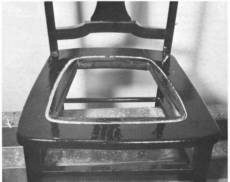
Now that old spline has been removed from this boudoir chair, and the chair has been refinished, it is ready to receive new prewoven cane.
