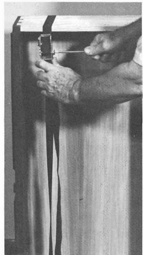
Whenever a piece is glued, it must be clamped securely and left to dry as long as necessary. This is a strap clamp.
