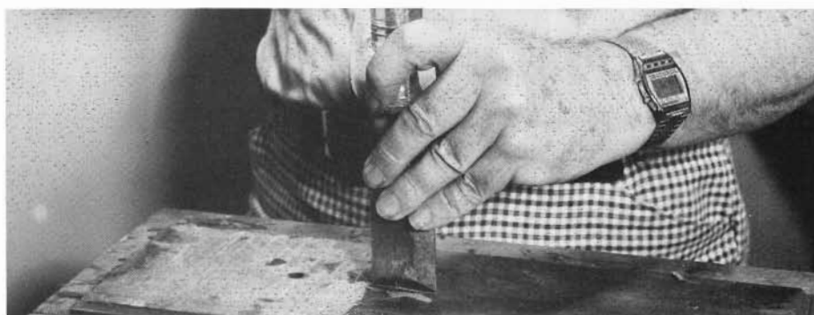
In some areas, the old glue still held. To break through, hold the chisel vertically and tap to make cuts through the veneer. When you make several cuts near each other, the old glue will loosen and release the veneer. Again, try not to cut into the base wood.
