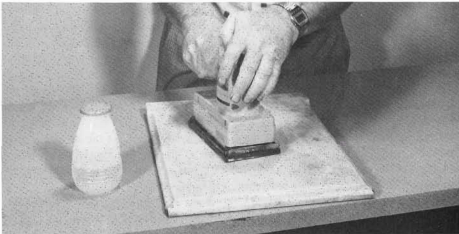
Start with the 120 grit paper in the sander and work it back and forth over the marble under fair pressure. Keep sprinkling water every few minutes to keep the surface wet. A white paste will form as the marble dust mixes with the water. Keep an eye on the scratches and pits on the marble surface, and as they disappear, change to finer sandpaper grits. The final polish should be done with a 400 grit or finer paper.
