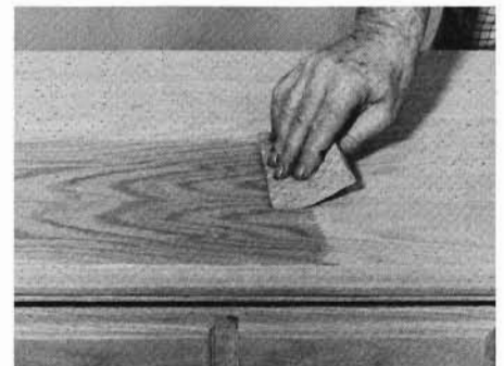
To raise the grain of an open-faced wood deliberately, first apply water, as shown here. The raised grain is then sanded smooth.
