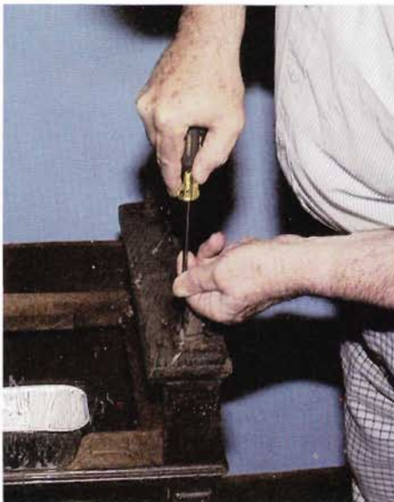
2 Next we took off the casters. There is a hole under each, indicating that these were not the ones used when the dresser was new. The hole accommodated the neck of the original. We will try to find substitutes for the old ones.
