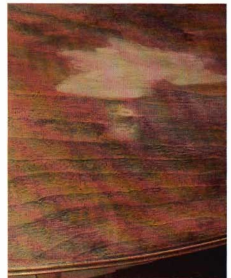
7 Here are the newly bleached areas. Bleaching also can be used to remove stains which have soaked deeply into the wood.
