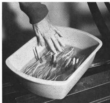
The caning is gathered into loops held by spring clothespins and soaked in a solution of warm water and glycerine for at least 15 minutes before use. (An hour is better.)
