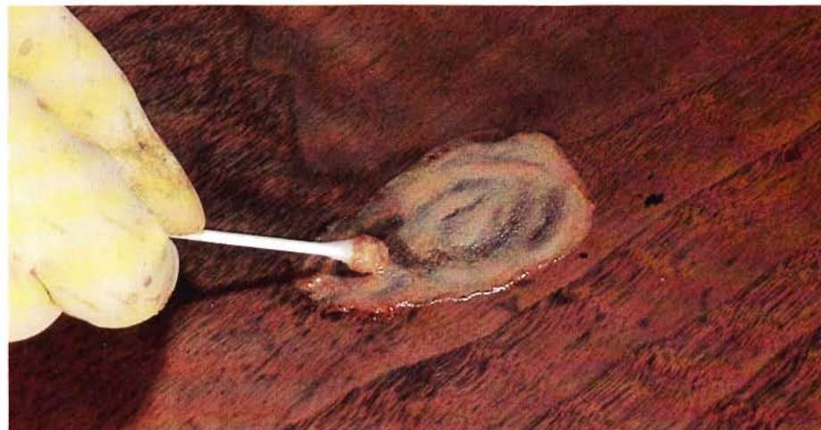
3 After the specified time, use a cotton swab to apply Chemical B from the kit. There will be a white foaming action.
