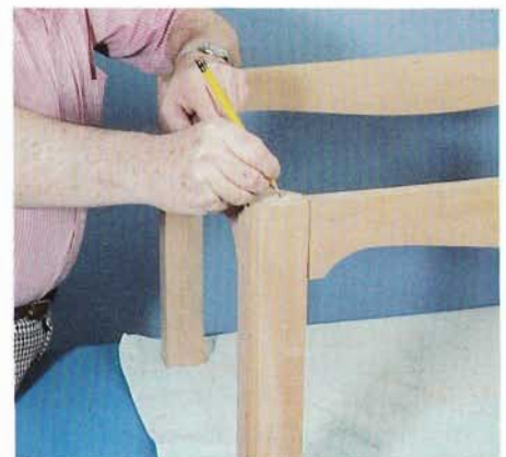
7 Now each leg and rail is numbered, so that when they are reassembled for gluing, you will get each tenon in the mortise.
