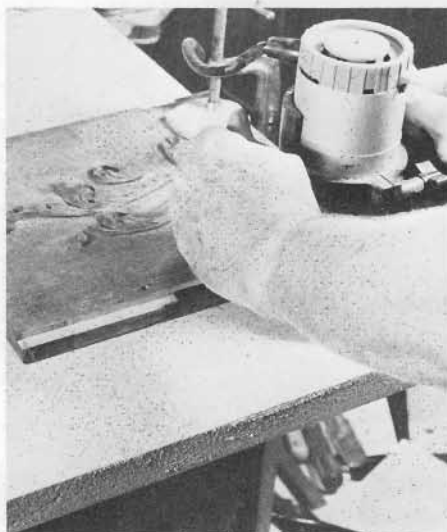
The first step in the edge repair is to cut away the splintered edge with the router, using a 1/4-inch rabbet bit.
