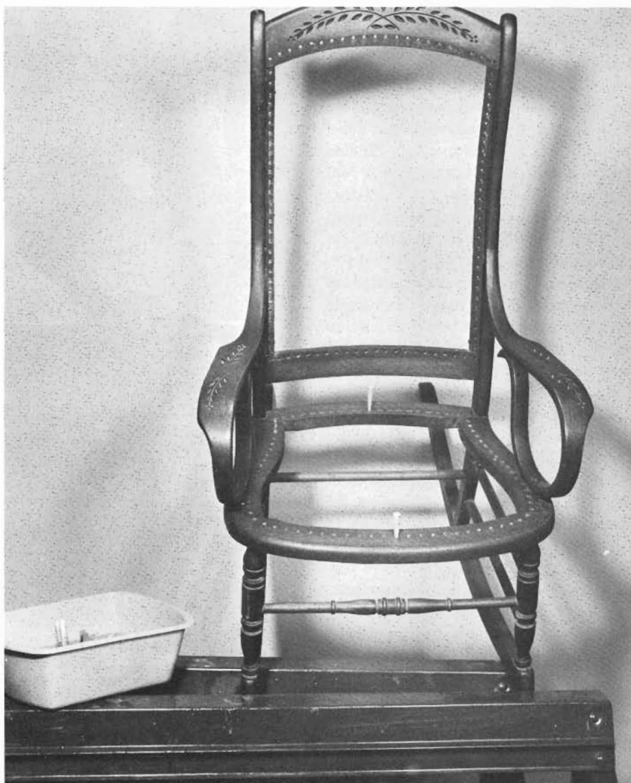
Repaired and refinished, the rocker is ready for caning. We set the piece up on metal sawhorses tilted against a wall, to bring the work to a convenient height. If you work in an uncomfortable position, you will end up with fatigue and sore muscles.
