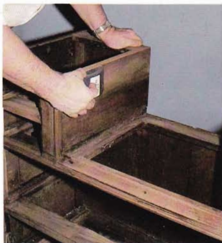
2 After taking off the old finish, the piece is sanded with fine paper. Old wood is dry and sands quickly, so don't overdo it. Watch the surface as you work to check progress.
