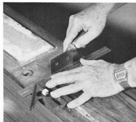
We deliberately cut these veneer panels slightly oversize so they could be trimmed in place. Use the veneer saw and a straightedge.
