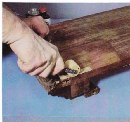
9 After the contact cement has dried for at least an hour and is no longer sticky, place the patch in the repair area and roll it down. Apply plenty of pressure as you roll.
