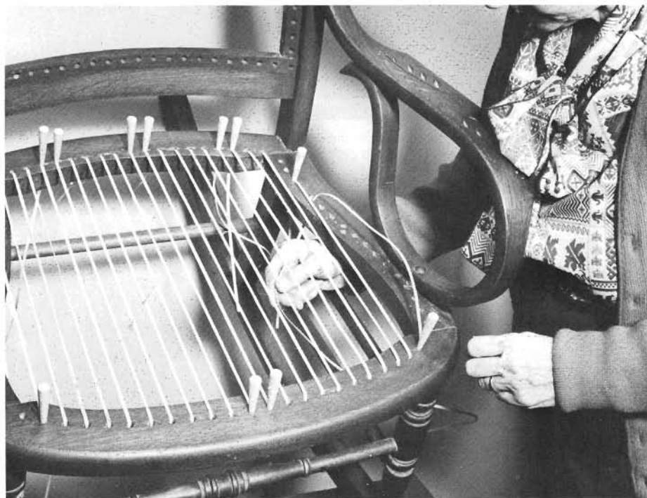
The shield shape of this seat has made it necessary to weave shorter strands at the left and right sides. When you must use strands that start along the side rather than at the back, employ the side holes that will keep the strands parallel with those already in place. In this case, the fourth hole from the back along each side proved to be the right one. Also, when inserting short strands, use a separate strand rather than continuing the longer strands.
