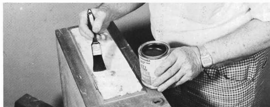
Apply contact cement to the drawer face. Use an inexpensive paint brush; evenly coat the entire surface.
