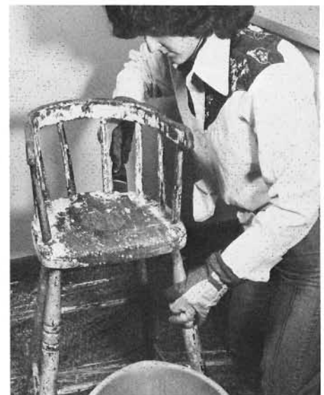
Slowly the old paint comes off. Under the white, there is a light brown and a darker brown coat, which are difficult to see here.
