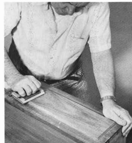
Before finishing, sand the veneer face thoroughly to eliminate saw marks in its surface. Use coarse, then medium, then fine and very fine paper to get the veneer ready for a stain and the finishing coats of varnish.
