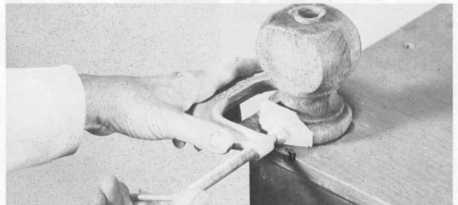
We began the repair by gluing new wood, cut to the size needed, to the leg "collar."
