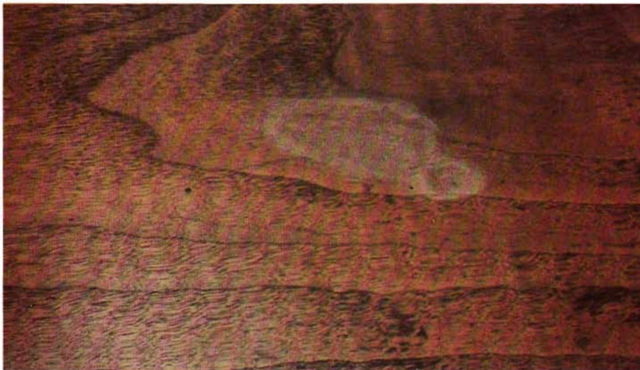
5 Here is the spot after drying. You can see that the black marks have disappeared. There was stain on this surface and it, too, is gone. Your first refinishing step will be to stain this spot first to bring its color level up. Allow it to dry, then apply a coat of stain to the whole top.
