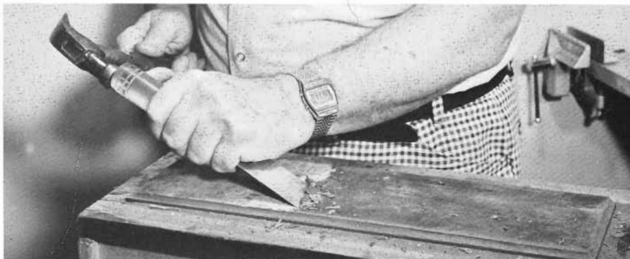
Remove the old dried and cracked veneer before applying new. The best tool for the job is a sharp, wide wood chisel handled carefully. Get under the old veneer, but do not damage the surface of the drawer. If you do, the new veneer will not lay flat.
