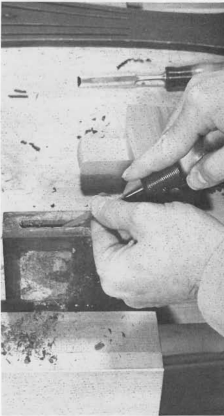
7 To clean out the ends, use a narrower chisel (here \frac{1}{4} in.) and drive the chisel down at either end of the mortise, then pry upward. This should bring up what remains of the tenon.
