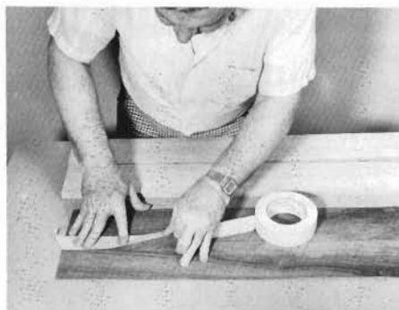
Now that the edges of the veneer match perfectly, use a strip of masking tape to hold them together. Be sure the sheets butt perfectly as you tape.
