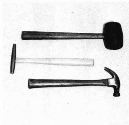
Three hammers will serve you in furniture work: a rubber mallet, a magnetic tack hammer, and a small (7½ oz.) claw hammer.
