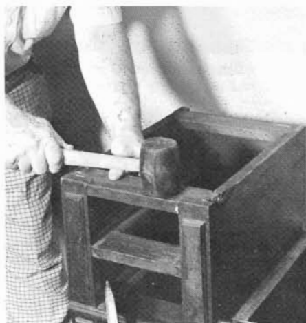
This frame member is tapped firmly but gently into the dresser with the rubber mallet. Do not damage the wood as you work.
