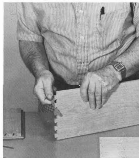
The pieces of fine wood kits are manufactured carefully, but because of humidity changes, you may have to do some sanding.
