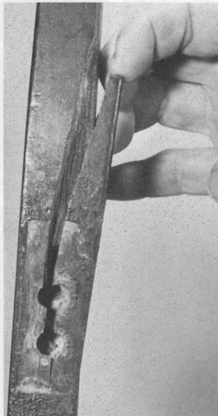
11 We found that not only was the tenon cracked, but the chair back rail was cracked through the mortise.
