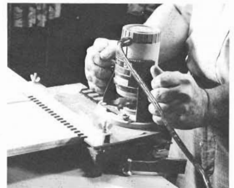
Cut a blind dovetail joint with a jig and a router holding a dovetail bit. Drawer side is at jig back; drawer back is in front of the jig.
