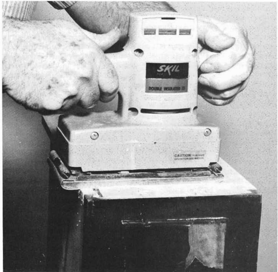
An electric sander simplifies the job of sanding. Avoid using sanding discs in a portable electric drill; always use a straight or orbital sander similar to the one shown.
