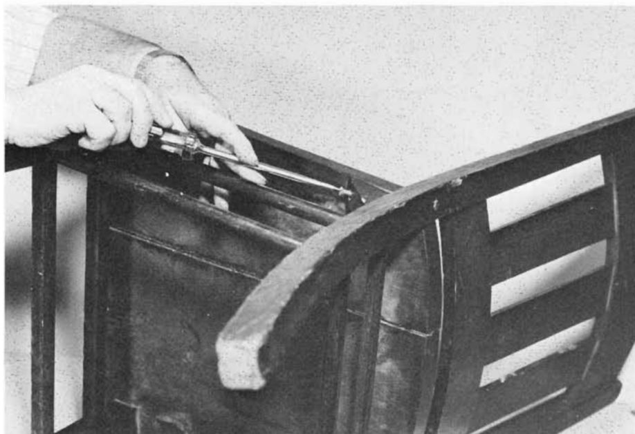
Look for screws in corner blocks, and also at the back, holding the seat to the back. Screws sometimes are hidden under wood plugs. Pry up the plug; remove the screw beneath it.
