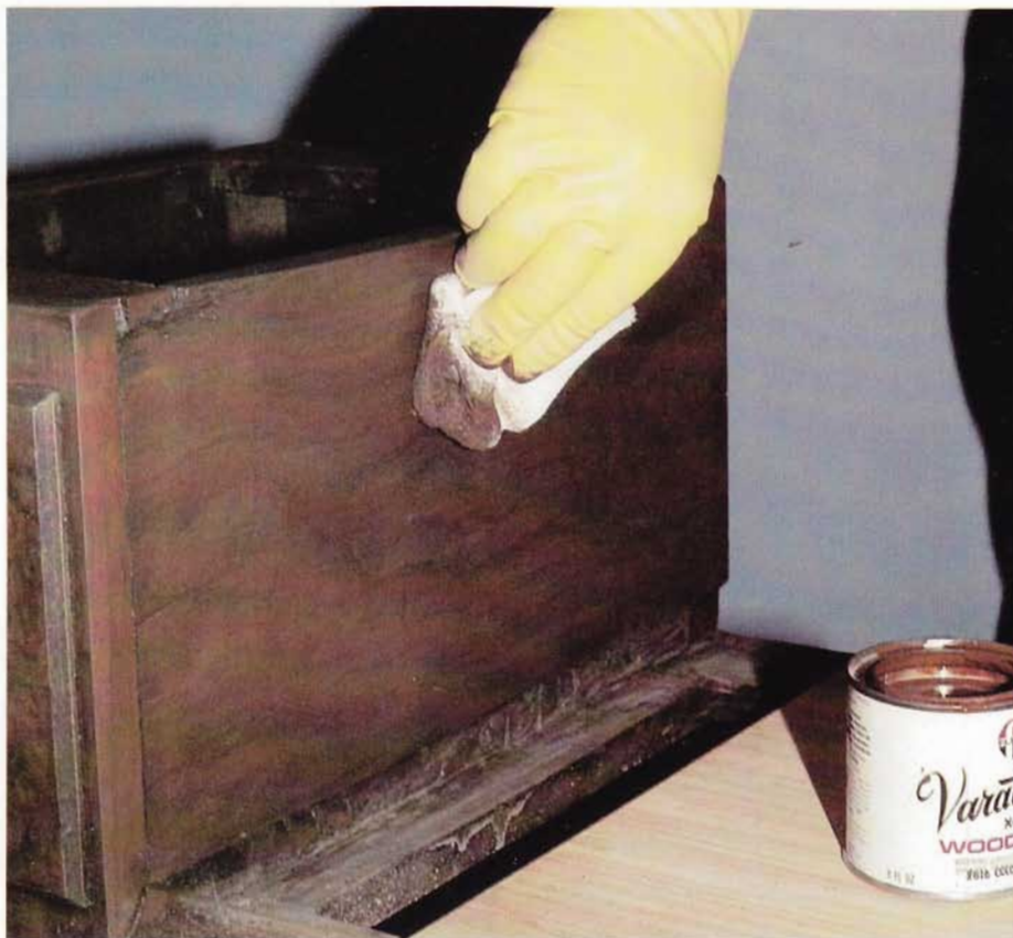
5 Next, wipe the stain thoroughly to expose the grain of the wood and achieve the proper color. Allow the stain to dry overnight before putting on the final finish.
