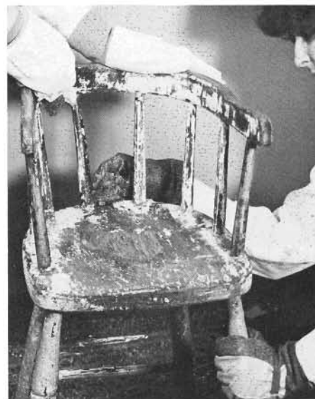
After the stripper has worked on a layer, and after scraping, use steel wool to remove the paint and break up the next layer.
