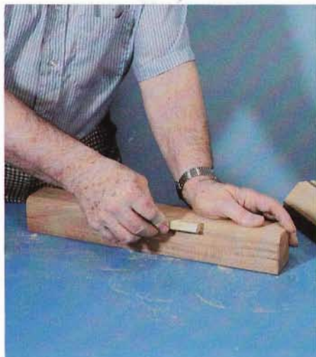
3 To sand the small grooves on the front corners of the legs, we made a sanding block and did the job by hand. The sanding block is a piece of wood that fits the grooves.
