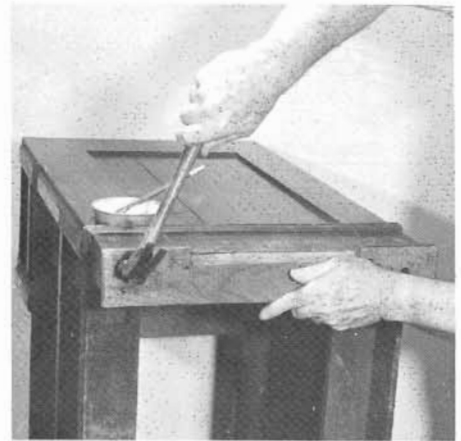
The square nails are now hammered into place as the baseplate is reglued. Two clamps hold the plate as the glue dries.
