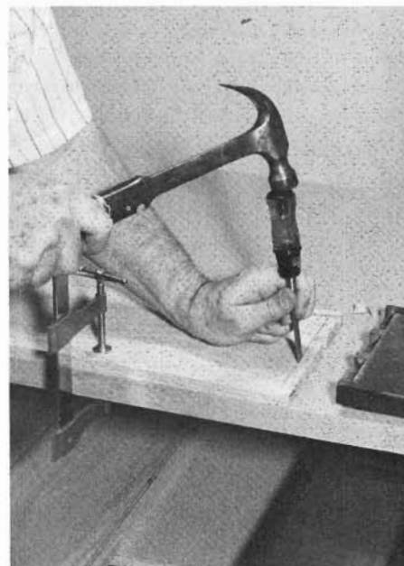
The wood chisel at work. If you plan to do much furniture work, practice with the chisel to learn how to control your cuts.
