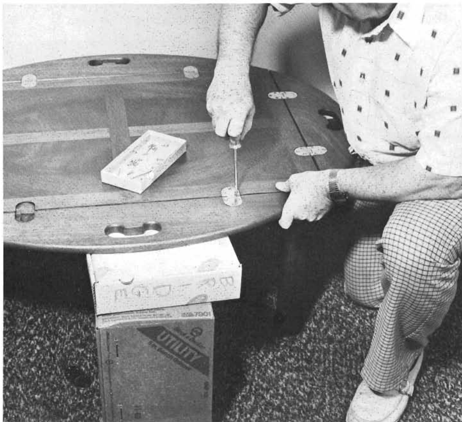
One mark of the better kits is the fine quality of the hardware. If your kit is inexpensive, upgrade it by replacing lesser pieces of hardware with fine brass ones.
