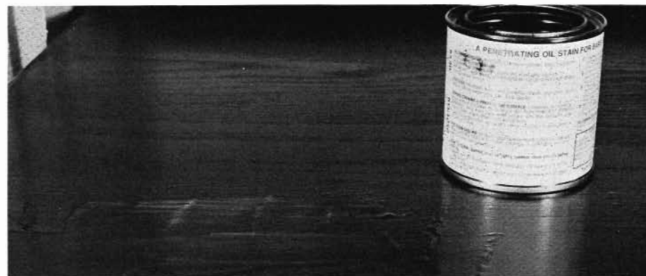
Penetrating resin is an especially good finishing material for softwoods such as pine. The material is absorbed into the surface and protects it from dents and other damage.
