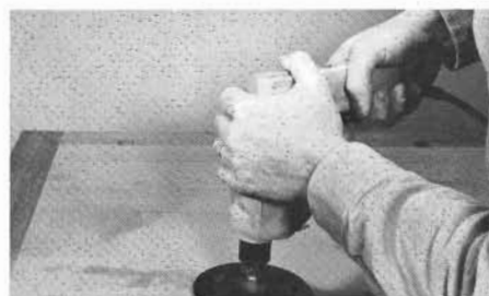
5 After cutting to the general shape you want with a wood chisel, use your drill with a sander attachment and coarse paper to continue the shaping. Change to finer grades of paper as you work until the rocker is shaped, smooth and ready for finishing.
