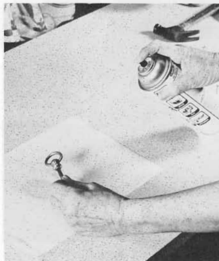
After bringing the brass to a lovely glow, we sprayed each piece with clear lacquer to protect it from dirt and hard use.
