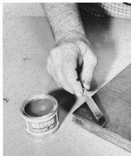
Use the spatula blade to smooth out the shellac. On an edge repair, also use it to shape the shellac to the same shape as the edge.
