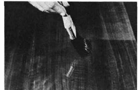
The patterned approach is one way to apply varnish. In this method, you have alternate varnished and unvarnished stripes. Then fill in.
