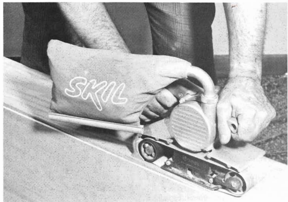
A belt sander is a fast worker, great for removing material fast. But be careful of it. You can dig trenches in the surface with it if you work too carelessly.
