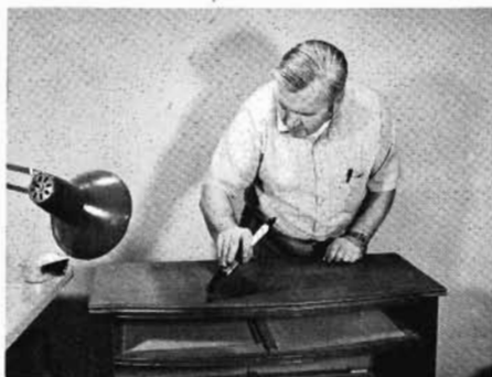
Varnish is laid down, not brushed out. The material then smooths out by itself. A light opposite you helps highlight missed areas.
