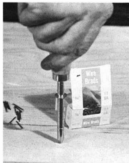
Shown here is a brad driver, a tool especially designed to drive the small fasteners. Brads are used for fastening wood trim.
