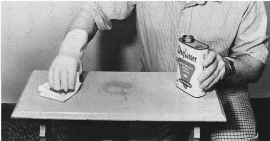
Applying enamel is similar to applying varnish. If you are recoating a piece already enameled, remember that the new coat will not adhere properly to the old glossy surface. Either sand the old surface or use a "deglosser" liquid on it so the new coat has tooth.
