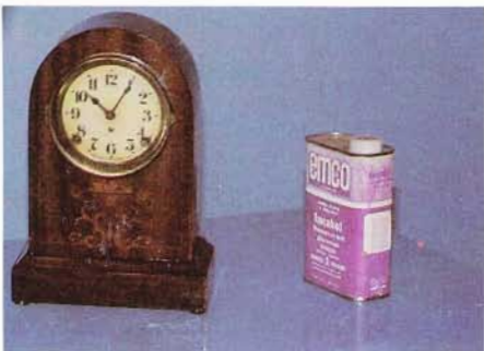
8 We have decided that time (some 75 years) and the realignment have resulted in a finish that is too thin. We decide to apply a new shellac finish. We first sand the old finish with fine paper to remove any blemishes.
