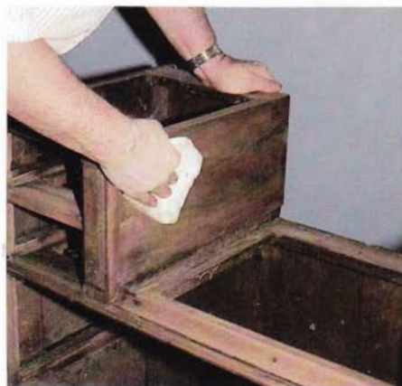
3 Remove all traces of sanding dust by wiping with a tack rag. Press hard to get all dust out of the wood grain, and keep wiping until the tack rag stays clean when you wipe an area.
