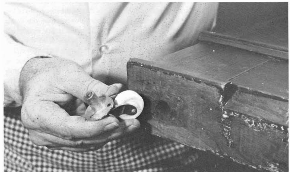
A plate caster is one that screws to the bottom of the furniture instead of being inserted into a socket. A small shaft fits up into a hole in the leg to hold the caster steady.
