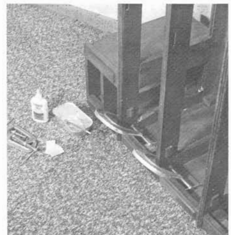
Here is another view of the frame of the dresser, showing how the joints were reglued. Clamps of various sizes were required.
