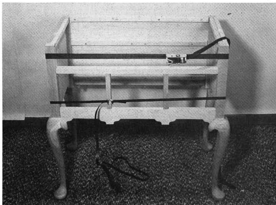
You can avoid many problems if you use glue carefully. Don't apply too much, and clean away any excess before you stain. Clamp the drying pieces firmly.
