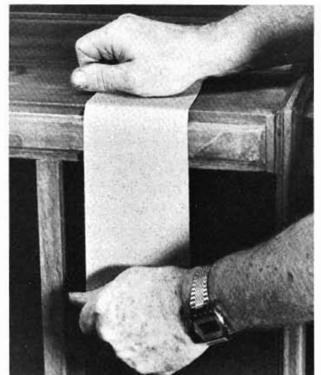
New sandpaper is stiff; soften it to make it last longer by running it back and forth, face up, across a table edge.
