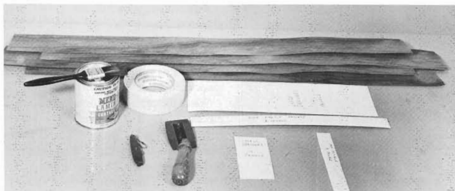
These are the veneering tools and materials: sheets of rosewood veneer, cardboard patterns of the areas to be veneered, contact cement, masking tape, a veneering saw and a small craft knife. You also will need some brown kraft paper.
