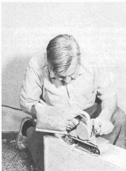
Use a belt sander to smooth the new wood and to sand new joints. A smooth drawer, with all corners slightly rounded, operates easily.
