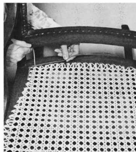
Now a length of weaving cane is used to tie the binder cane in place. The end of the weaving cane is tied to a loop under the rail. The other end is brought up through the second hole.
