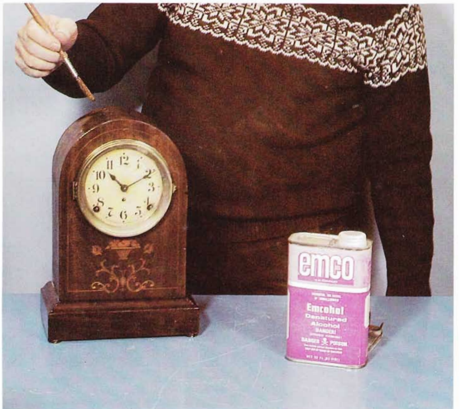
10 When shellacking, use a top quality brush and gently lay the coating on. Don't brush it out, as you would with paint. Here, a 3-pound cut of shellac is used straight from the can, and we plan on 4 coats. If you use a 1 or 2-pound cut, increase the number of coats.
