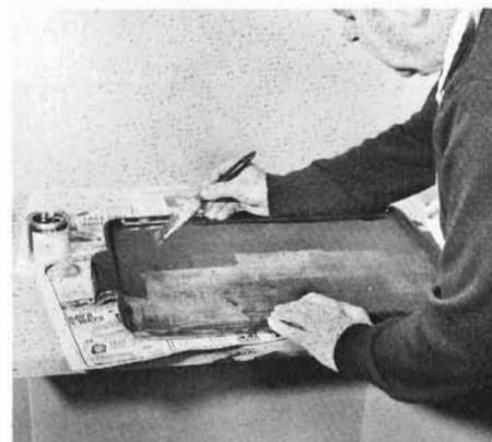
Next, we applied a coat of varnish to the damaged area. When this dried, the entire tray was varnished to fully restore the tray.
