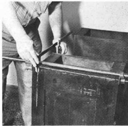
The newly glued crack can now be clamped for drying. Wipe the excess glue from the surface as soon as those clamps are in place.
