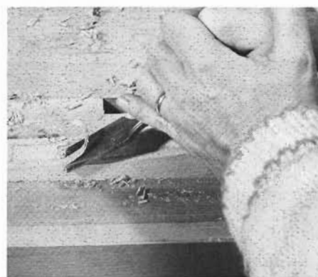
4 The glue has dried and the rocker is ready for shaping. Use a wood chisel to level high spots and to make the rocker shape you need.
