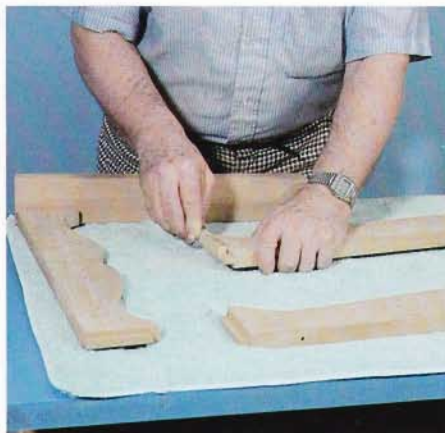
4 All of the table joints are mortise-and-tenon. After you have finished sanding all parts, the base is assembled dry. During this assembly, you probably will have to sand the tenons a bit to make them fit. Note that we have placed a soft bath towel on the workbench to protect the sanded parts as we work.
