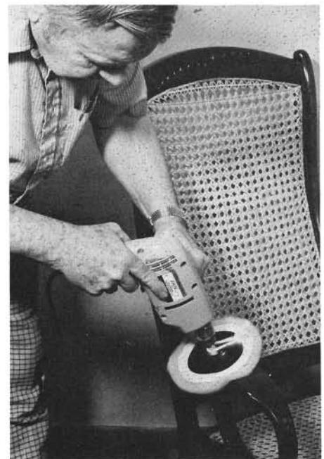
Now the wax is buffed to a high shine with a lamb's wool buffer in the electric drill.
