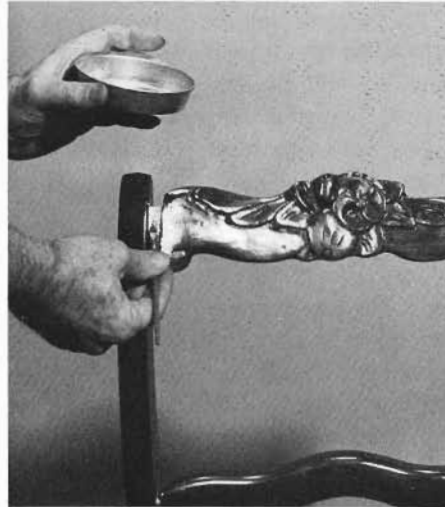
Sometimes you can reglue furniture without dismantling it. Here a brush is used to paint glue into a loose chair joint.
