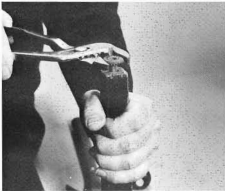
Lift the socket slightly with the awl, then use a pliers to turn and lift it.
