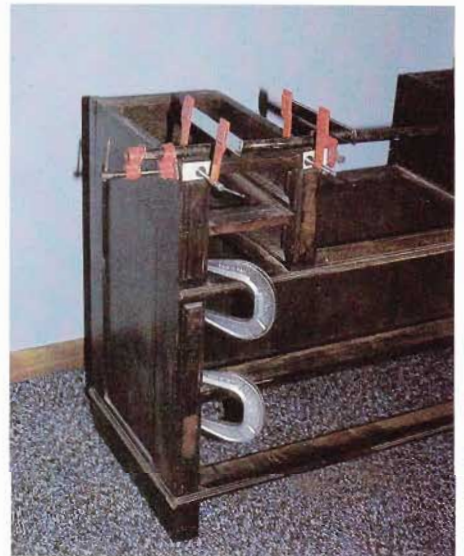
9 We need a variety of clamps to glue the dresser joints together. Notice the small wood pads that protect the finish of the dresser from the jaws of the clamps.
