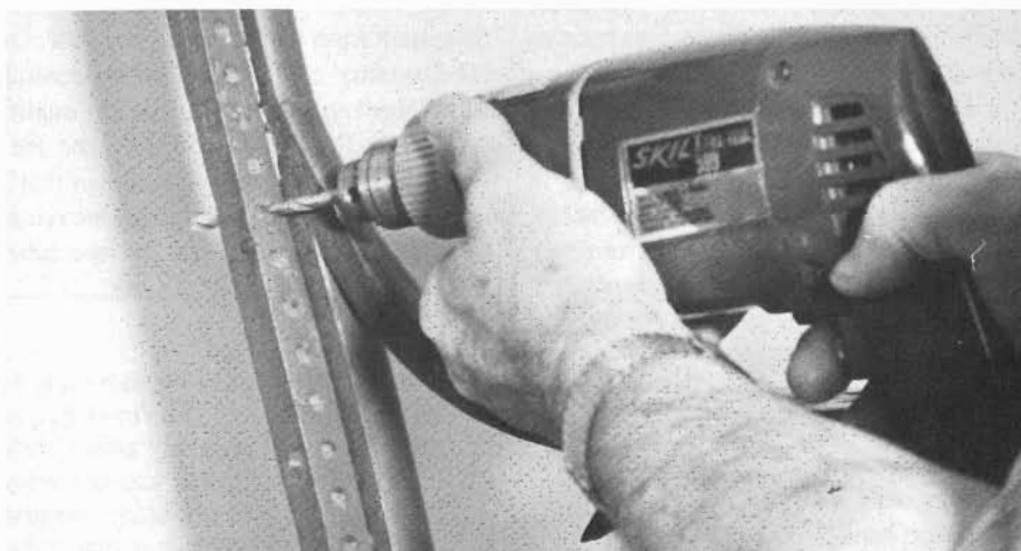
Before recaning an old chair, make sure the holes are free of dirt and old finishing material. The best way to do this is to redrill each hole with a bit that is the size of the hole. It only takes a few minutes to run the bit into each of the holes.
