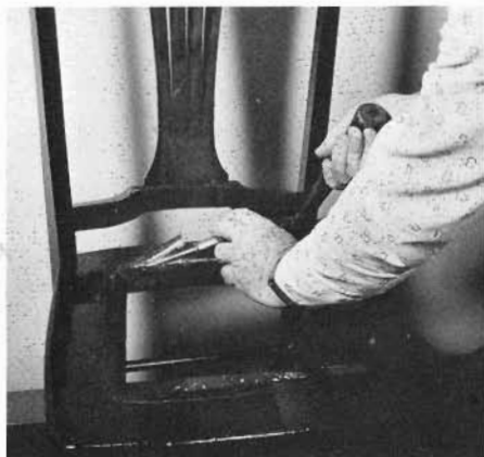
To remove the old spline from the groove around the seat, dig through the old spline and get a small chisel or narrow screwdriver under it.
