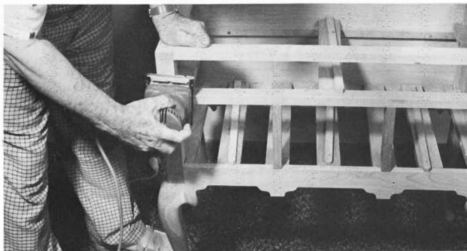
Once the glue has dried, sand all the pieces thoroughly. No brand of unfinished furniture comes in a condition that is ready to stain. Your sanding should be thorough.
