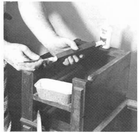
Now we must reglue any frame members that need it, using a brush to apply the glue that has been squeezed into the aluminum dish.
