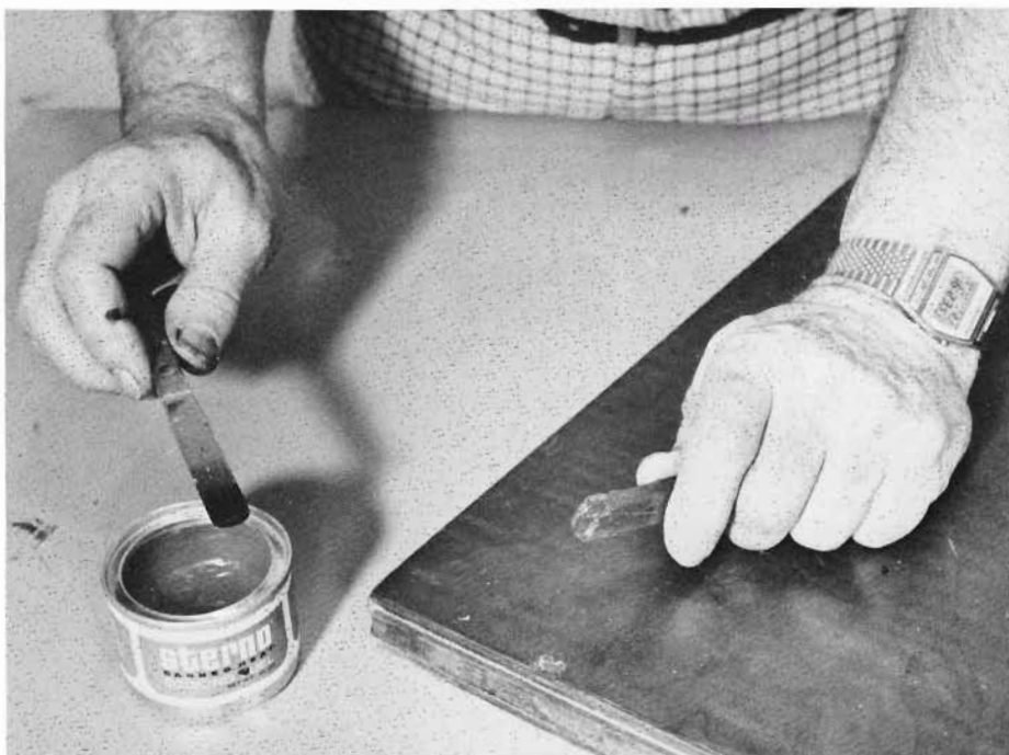
Select the color closest to the color of the finish. Light a can of Sterno or use an alcohol lamp to heat the blade of a spatula. (Do not heat by candle flame, as this will deposit carbon on the blade which will discolor the stick shellac.)
