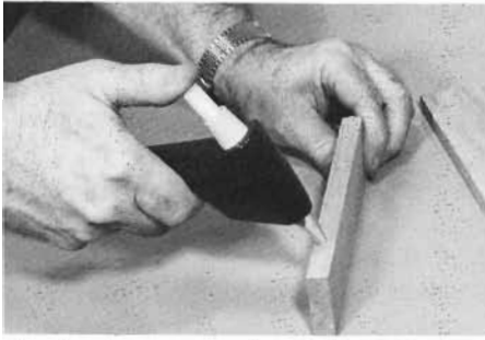
Electric glue guns can be used only in certain furniture applications. Here a gun is used to apply a bead of glue to an edge.
