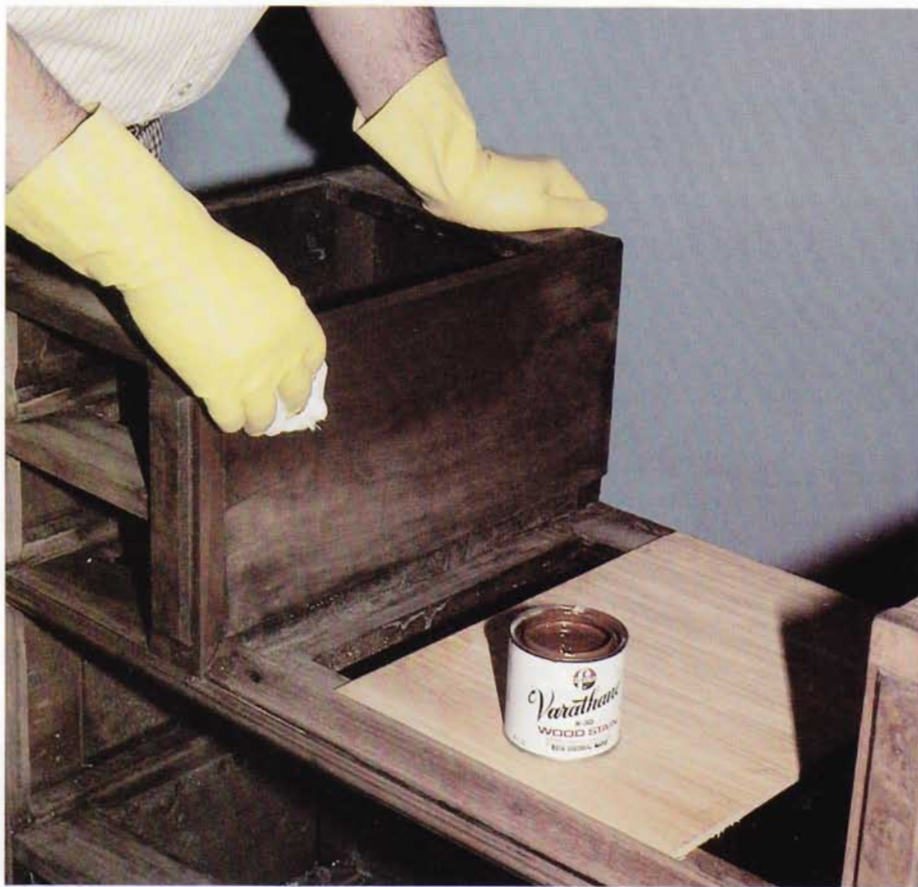
4 We chose a liquid wiping stain for this job but could have used a jelled stain. The first step is to apply a light coat of stain to each part of the piece and allow it to stand for ten minutes.
