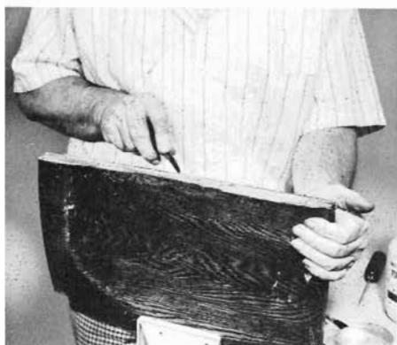
After the glue has begun to soften, use a pen-knife to dig clots of glue out of crevices and to scrape the surfaces clean.
