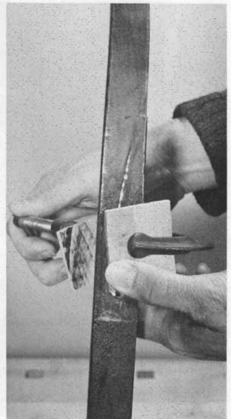
12 Repair of the crack is a simple glue-and-clamp procedure. Don't attempt to reassemble the chair until all glue has dried thoroughly.
