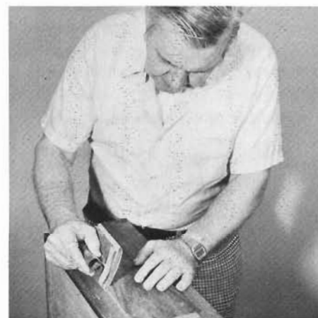
After giving the contact cement a couple of hours to set, sand the edges. The edge of our hand sander was a perfect fit for this job. If it hadn't been, we would have made a small hand sander of the right size and shape from a block of wood.
