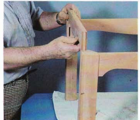
6 Assemble the table base without glue. Here the last side rail goes into place after the tenon was sanded to fit.
