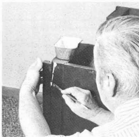
The upper part of the back frame had a long crack in it. Using a brush, we put glue into the full length of the crack.
