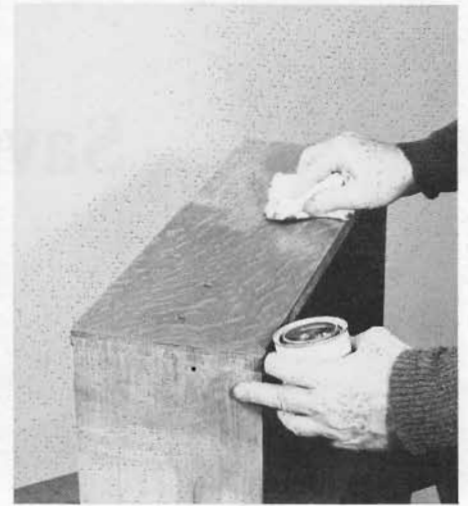
This drawer has been stripped of the old finish. The old stain is sound, but it had faded, so we applied a new coat of stain to bring up the golden oak color.
