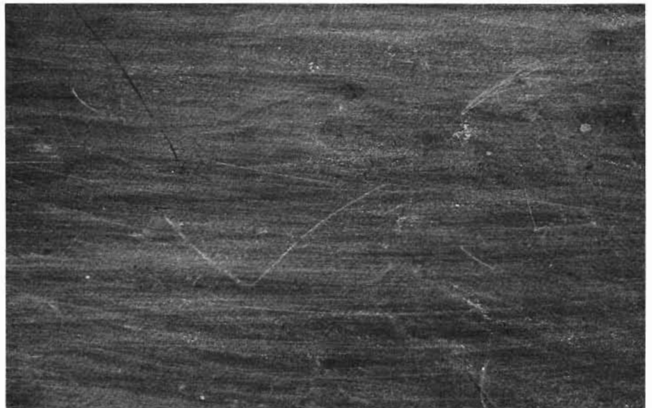
A surface covered with scratches need not be totally refinished. Before you take drastic measures, try reamalgamation. Apply new varnish to the scratch. Then reamalgamate.
