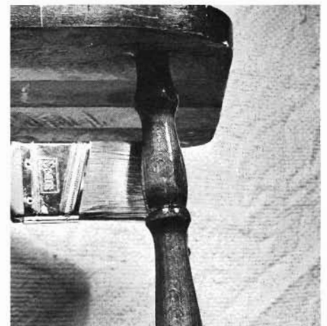
To prevent runs when you varnish round parts such as legs and rungs, apply less thick a coat than you do on a flat surface.
