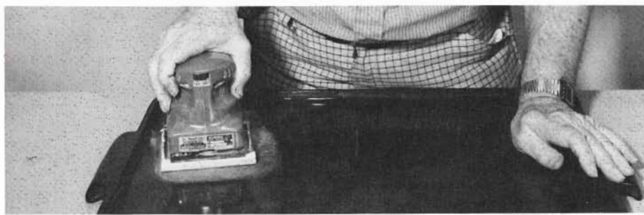
We tried finish remover on the bad spot but it didn't work. The finish appears to be a heavy coating of polyurethane varnish. Our only choice now is to sand out the bad spot as far as necessary to remove any discolored wood. Fortunately, not much sanding was required, so the surface of the wood remains unharmed.
