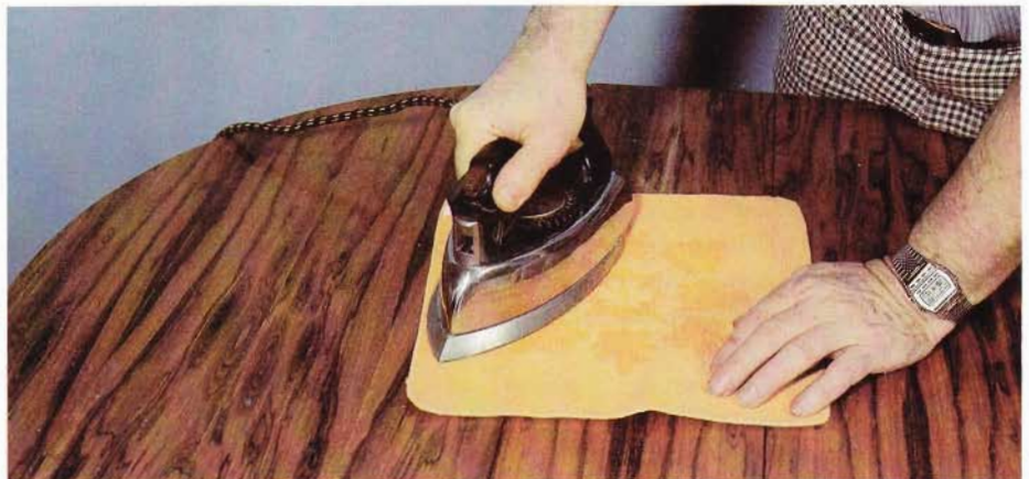
15 Once in a while, veneer will bubble up in the center of a veneered piece. Many times, a simple repair can be achieved by applying a hot iron to the bubble. Place a dry wash cloth on the bubble and press the iron to the area. Be careful not to hold it too long, as it may affect the finish.
