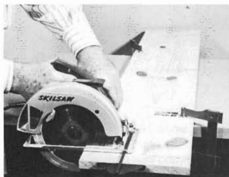
A circular saw is useful for straight cuts. Always use it with an edge guide.
