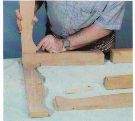
5 Sand each tenon carefully so as not to change its shape or the face of the adjoining wood, then fit it into its mortise.
