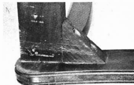
Corner blocks (left) reinforce joints. To remove glue blocks (above), tap a chisel at one edge.
