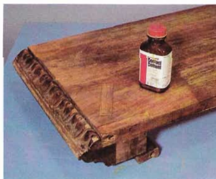
8 Check the veneer patch for size by placing it in the repair area. When it is perfect, coat the area to be repaired and the underside of the veneer patch with contact cement. Allow both to dry for at least an hour.
