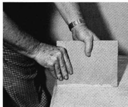
Wood filler is a creamy paste which you paint over an open-grained wood to fill the grain. Allow it to stand until it suddenly loses its gloss.
