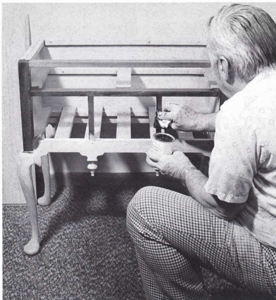
All surfaces should be finished. We finished the butler's table when assembly was completed. However, this low-boy has interior spaces that we finished before the top was installed.
