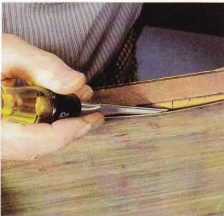
12 Another common veneer problem is when the veneer lifts from the base wood, as it has here. This table leaf was soaked during a flood and now must be restored.
