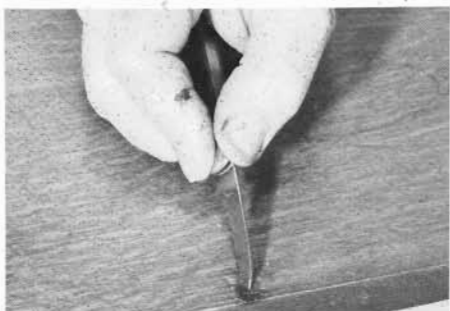
A cigarette burned the edge of this table leaf to make a black char about 3/4 in. long. To repair it, scrape with the sharp blade of a pocket knife.
