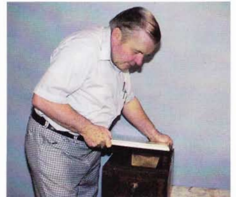
4 Before restoration can begin we must disassemble the dresser. After removing the screws beneath the marble top, we can lift off the section. The marble pieces need minimal work.
