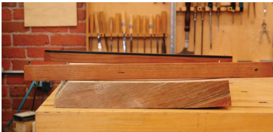
This twisted board illustrates just how a four-legged piece can also twist. There are two opposing high sides vs. two low ones. The winding sticks show what's high and low.
