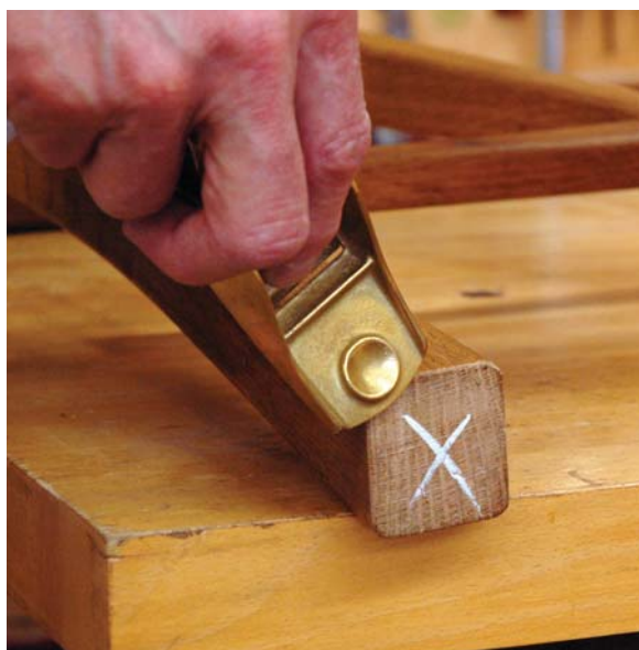
Truing legs with a block plane requires time and ingenuity to make sure the piece stays stable and doesn't tear out as you attempt to trim it to length.
