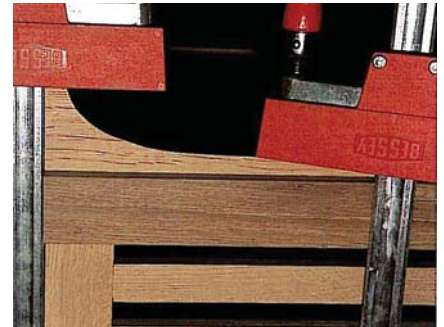
Gluing on the corbels is fairly simple, but watch for glue squeeze-out.
