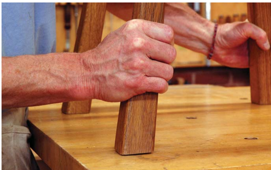
Check for twist using the bench as a flat reference surface. Pushing on opposing corners will identify which legs are longer; mark those with chalk.
