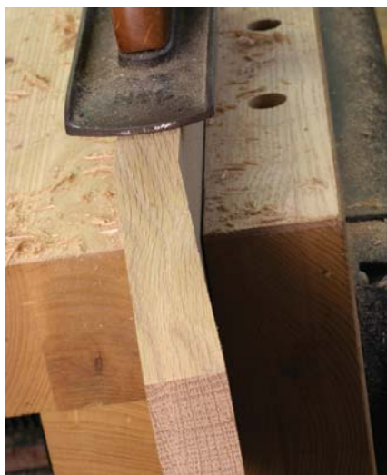
The glue line should disappear because the grain and color are the same in both pieces.
