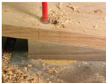
A wedge below the arm provides the proper tilt to keep the holes vertical.
