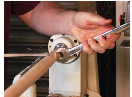
A fairly simple turning trick to get consistent sizes is to use a wrench as a caliper.
