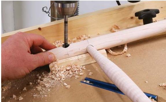
Tilt the drill press table to the proper angle using an angle layout stick.
