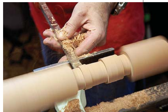
Turn the cylinder at the top of the leg with care. If your tool catches the square section above or below, game over.
