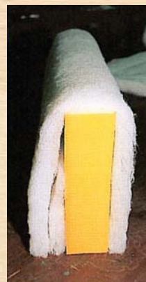
The back cushion is rectangular cut foam wrapped with fiberfill.
