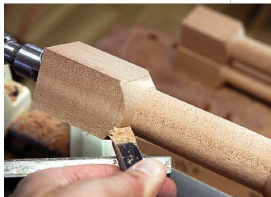
The transition between the cylinder and the square section is a snap if you ease into the cut slowly.
