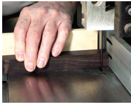
After machining a piece of ebony to 1" \times 1" \times 12", slice 16 \frac{1}{2} "-spacers at the band saw. And make a few extra, just in case.
