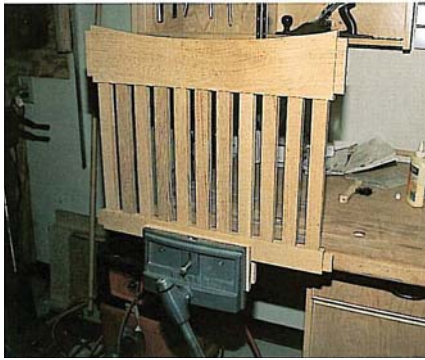
The side assemblies should fit snugly, but if you force them, you'll split the wood!
