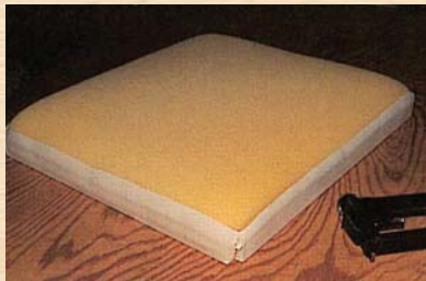
Right side up, the foam is formed by pulling and fastening muslin to give the cushion its final shape.
