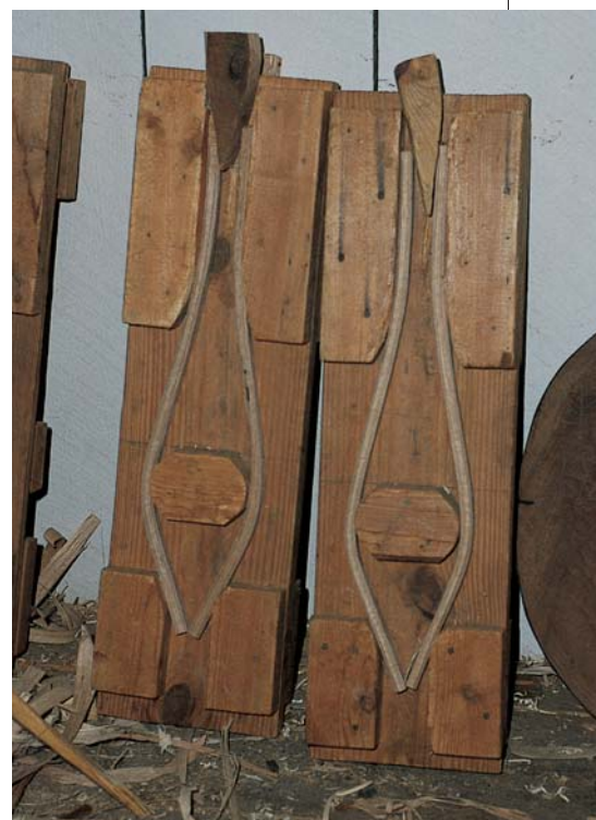
The jigs I use are fairly simple 2× material with blocks added to space and shape the pieces. Two sets of back rails are shown. The jigs for the back legs are even simpler.
