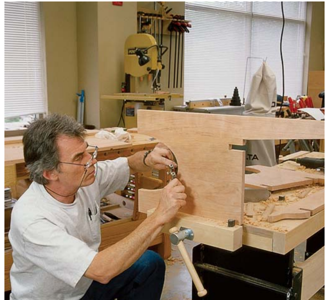
A spokeshave eases the edges the block plane couldn't reach.
