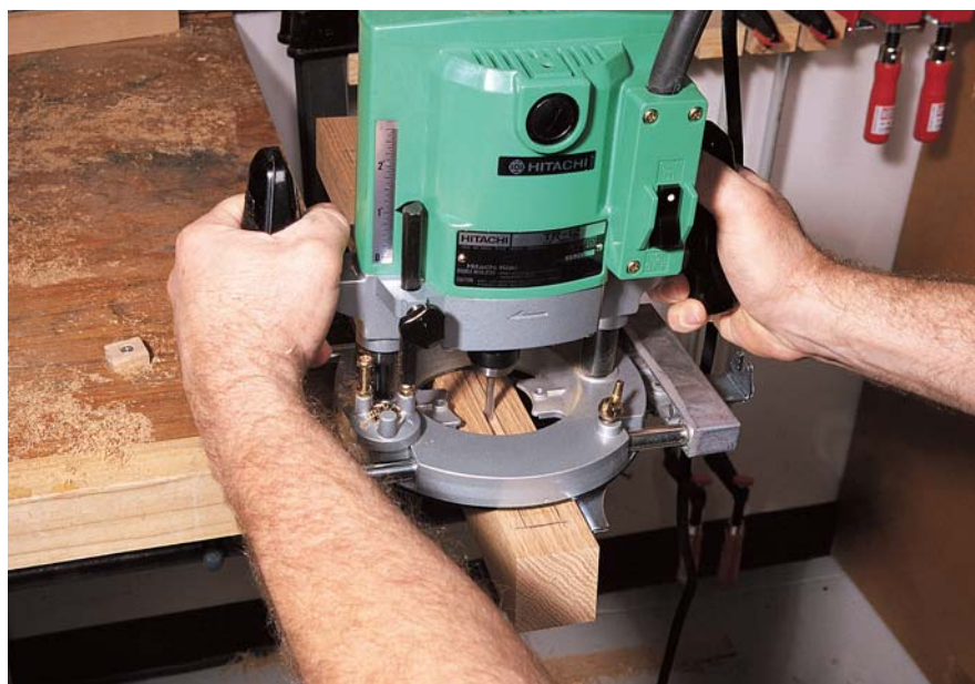
Start the inlay work on the four legs by using a router with an edge guide to rout the 1/4"-wide channels for the inlay.
