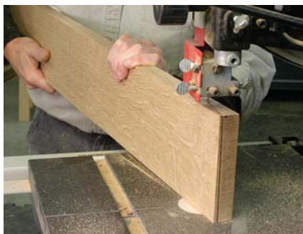
An angled wedge sliced off the end of the arm forms the bend.
