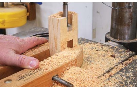
Making a jig to drill the stretcher holes can be easily done with a small piece of 2x4. Drill a 1 1/4" hole from both sides then rip the piece to 1 1/16" thick to create a trough in which to place the leg for drilling.
