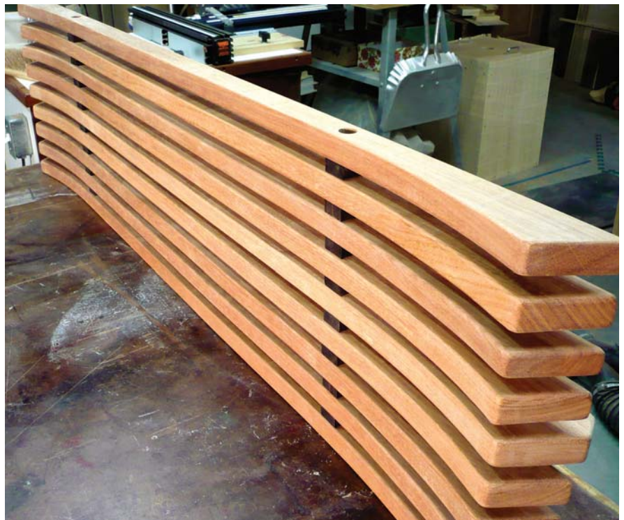
To start assembly, insert a rod through one of the outside slats so the washer and nuts are recessed in your counterbored holes. Slide on a spacer. Repeat.
