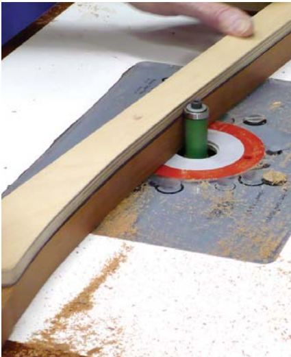
Jatoba is very brittle and prone to splintering, so attention to grain direction while routing is essential to avoid tearout.
