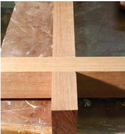
Strive for a snug fit between the stretcher and lower rail.
