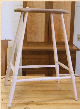
Rough assemble the stool and trim the tenons close so the wedge placement can be marked.
