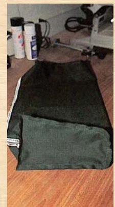
The upholstery fabric is stapled in place using the same method as the muslin. A layer of fiberfill is simply placed between the foam and fabric to give the cushion loft and smooth and irregularities. Fit the fabric in the corners neatly.
