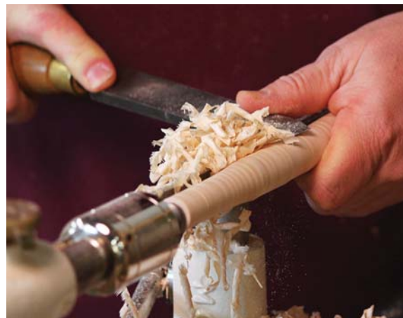
After turning the leg blank to a 1¼"-diameter cylinder, use the layout stick to plot the top and bottom, and the middle of the swelled part of the leg.
