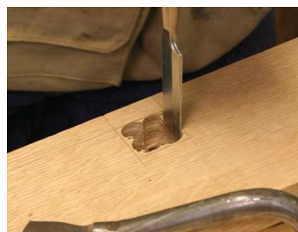
The same wedge is clamped between the arm and the bench to pare down the walls of the through-mortise.
