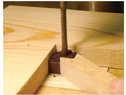
Drill \frac{5}{16} " holes in the center of the spacers. I made a simple bird's mouth, along with a 90° jig, to secure the spacers during this operation.
