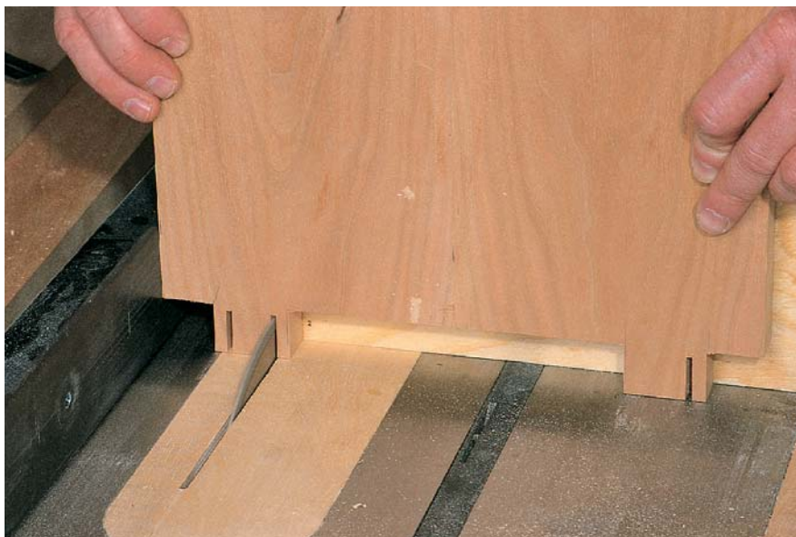
Cut the tenons to the actual width on the table saw. Set the blade to 1" high, defining the length of the tenons. After marking the depth with a gauge, cut the waste out from between the tenons. Set the saw to \frac{7}{8} " high for cutting the slots that accept the wedges used to hold the table together. See the diagram for the actual size of the outer parts of the tenon. Use a backing board on your miter gauge to hold the boards upright
