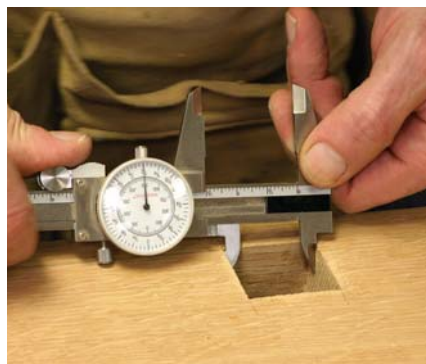
Check the size frequently with calipers as you work on the mortise, and compare it to the tenon.
