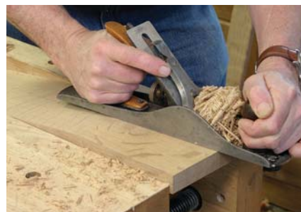
Planing out the band saw marks leaves a smooth surface on the top and bottom of the arm.
