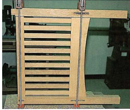
When attaching the legs to the side assembly, the best grain should face outward.
