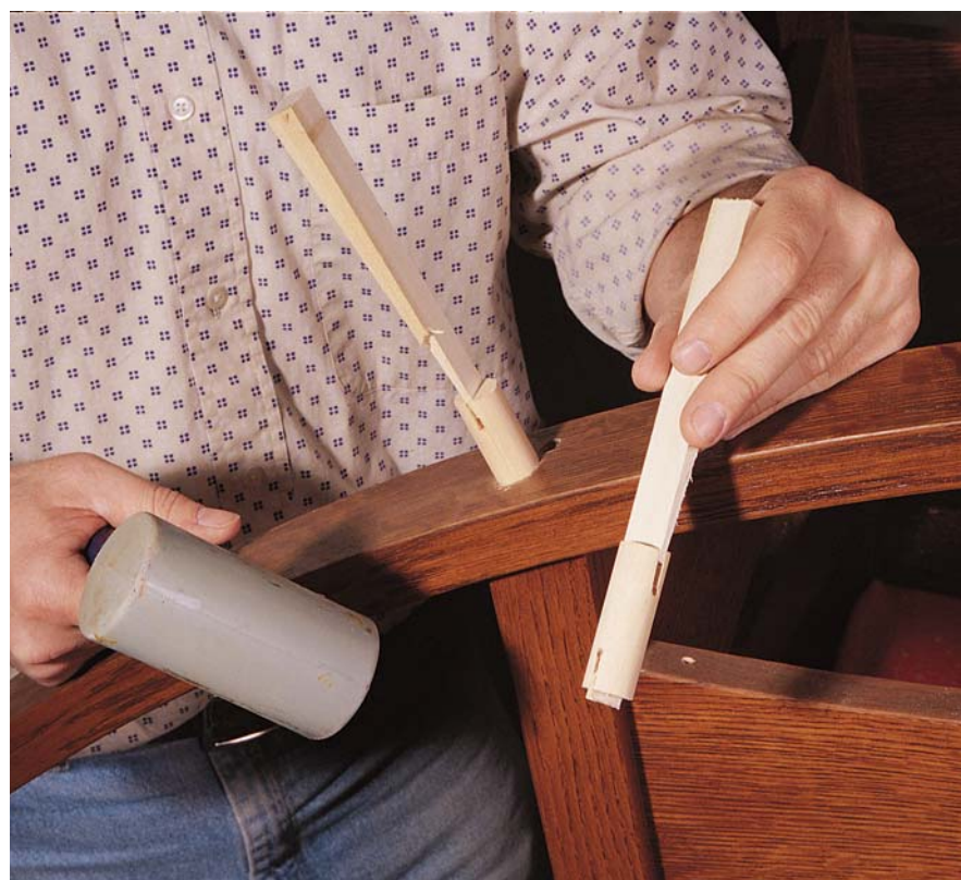
A \frac{3}{4} " dowel with slots and wedges will hold the rockers in place for many years to come.
