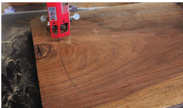
Careful placement of the pattern allows the seat to be defect-free. The band saw makes short work of roughing out the seat blank.
