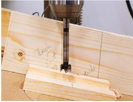
Tilt the drill press table to the proper angle using an angle layout stick.
