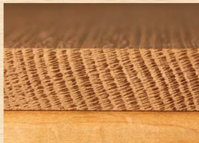
Quartersawn oak has near vertical end grain.
