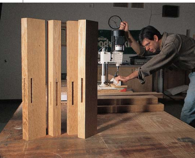
Make the mortises in the legs before you shape the curve near the bottom or make cutouts on the top.
