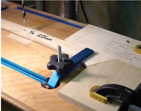
Set up to drill \frac{5}{16} " holes in the slats. Both ends of the slats are secured with hold-downs for this critical operation.
