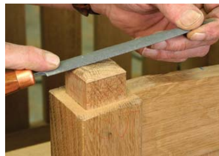
Mark the intersection of the arm and the tenon with a pencil line and round the end of the tenon down to the edge. Stop just outside the line to maintain the fit between the two parts.
