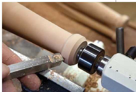
To make the astragal at the foot, turn 45° chamfers on the corners. Then turn chamfers on the arrises of the chamfers. Then turn arrises on those chamfers until you get an astragal.
