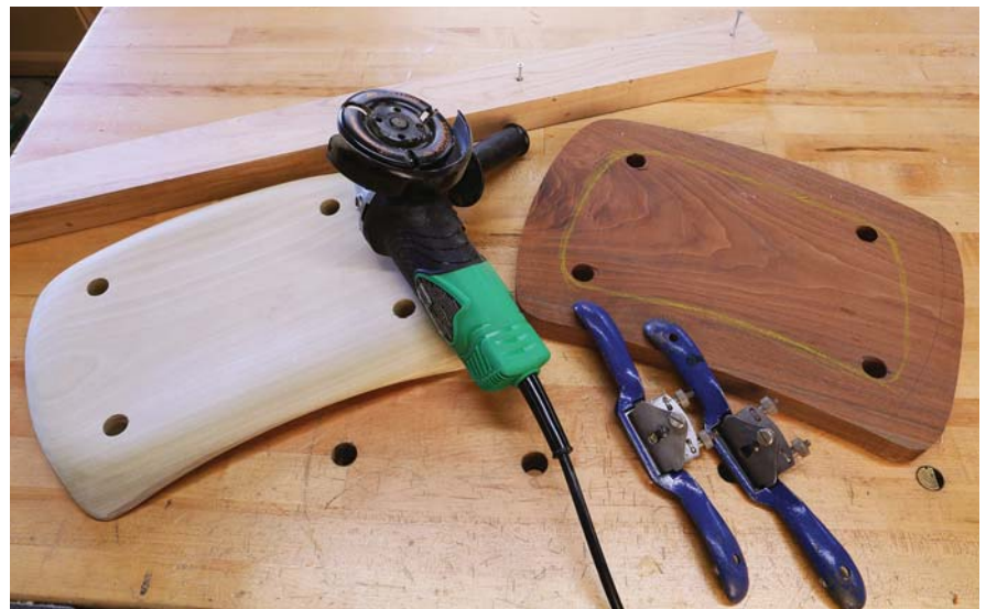
Attach the seat topside up to a stick with a couple of screws through it. This allows you to secure the work in a vise for grinding and shaping with hand tools.
