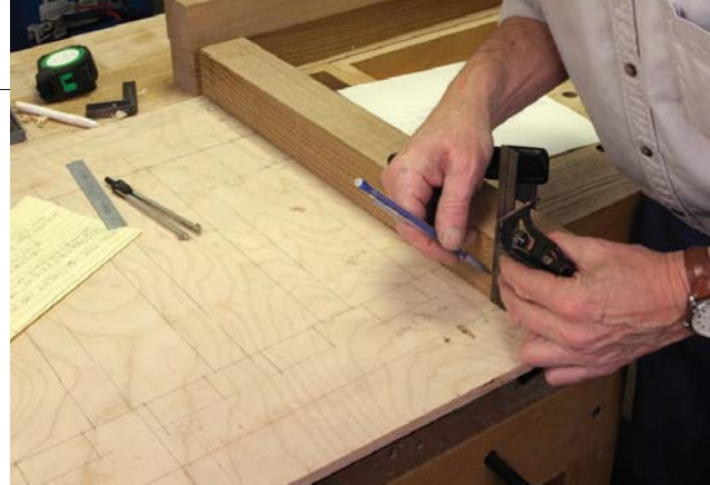
A full-scale drawing provides a reference for most parts of the project. It saves time, and prevents measurement and layout errors.
