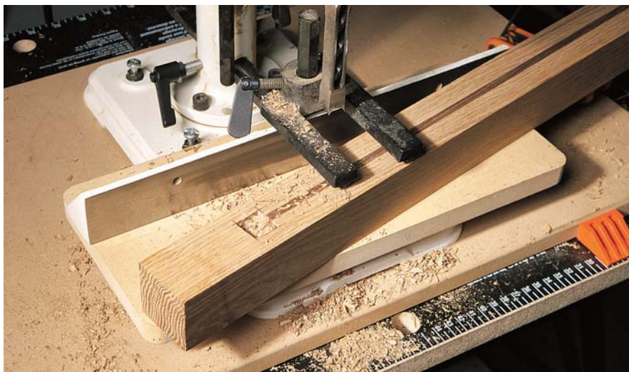
The square ends of the inlays can be done with a mortiser, as shown here, or you can use a router with a template and use a chisel to square out the corners.
