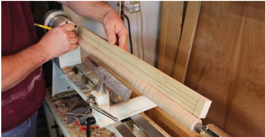
After turning the leg blank to a 1¼"-diameter cylinder, use the layout stick to plot the top and bottom, and the middle of the swelled part of the leg.
