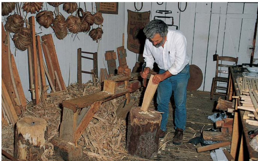
Most woodworkers don't list a hatchet as part of their tools, but when I'm chopping out the shape for the top slat it's my best friend.
