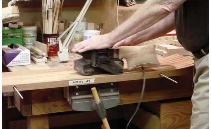
I use my ancient (and very loud) belt sander to level the slats. This operation requires a light touch and good hearing protection.
