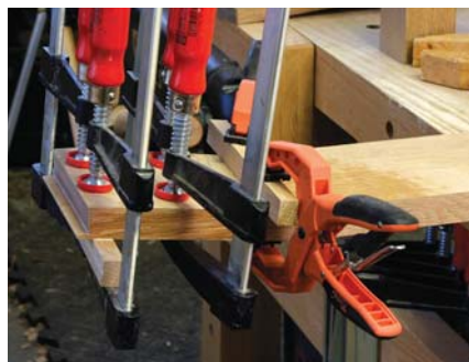
The wedge is glued to the underside of the arm, smooth face to smooth face.
