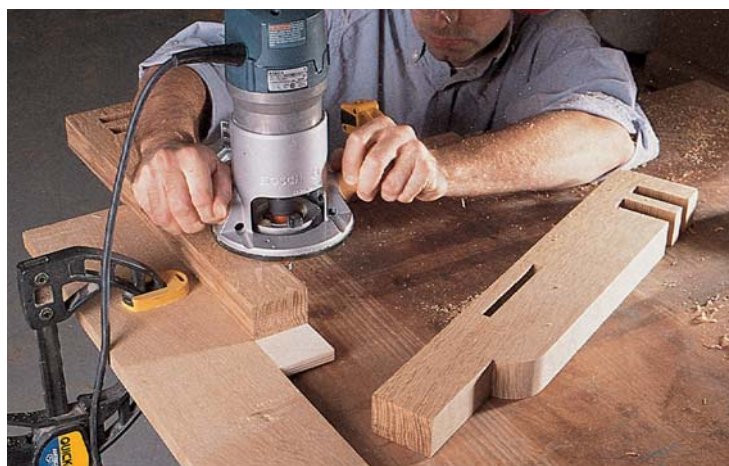
When pattern-routing the curve on the legs, make sure you have the work firmly clamped in place. I have the pattern and leg wedged between two pieces of oak (the pattern is on the underside of the leg). Then the leg itself is clamped to the table. You also could perform this operation on a router table with a starting pin for pattern-routing.
