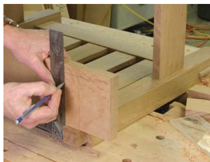
Balance the arm on the base assembly and mark the location of both the front and back tenons without moving the arm.
