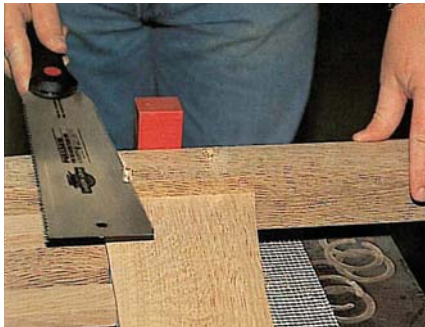
Keep the saw blade parallel to the leg surface while cutting the peg flush.
