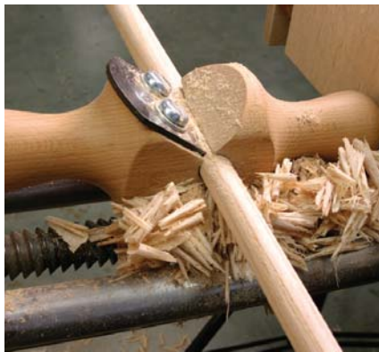
This rounding plane by Ray Iles excels at turning down your sticks to the right dimension.
