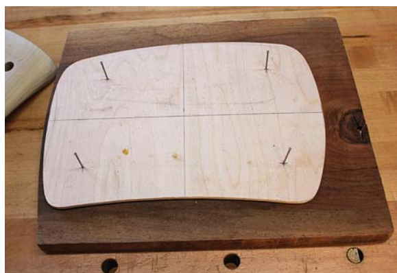
Choosing your figure and grain direction is crucial for a sturdy stool. The nails in the pattern help locate the center of the leg holes.
