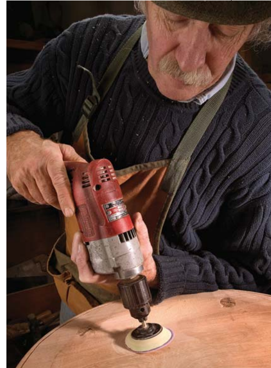
The final step to smoothing the seat is to fair out the saddle with sandpaper stuck to a foam pad, which will follow the seat's complex contours.
