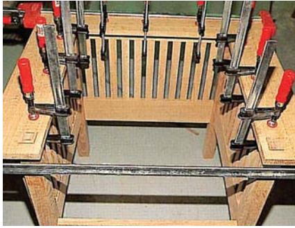
Gluing the arms in place is another chance to adjust the chair for square.
