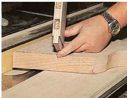
A featherboard provides stability and safety while cutting the tenons.
