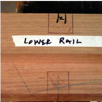
Carefully mark the notches for the rails. Here, a lower rail blank is lying on top of the stretcher blank.
