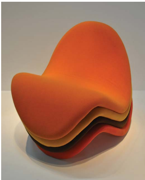
Figure color-12c Stacked Tongue 577 chairs, designed by Pierre Paulin (1967), tubular steel armature surrounded with rubber webbing and expanded foam, upholstered in polyester stretch fabric. Manufactured by Artifort. 33½ inches wide; 35½ inches deep; 24 inches high; 13½ inches seat height (85 cm wide; 90 cm deep; 61 cm high; 34 cm seat height). Photography by Jim Postell, 2011.
