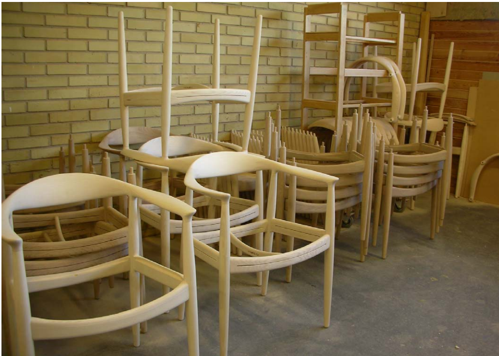
Figure 9.25 “The Chair,” wooden frames in production at PP Møbler, Denmark. Photography by Jim Postell, 2006.
