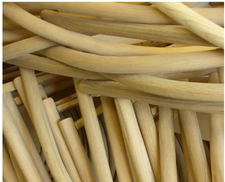
Figure 7.12 Turned and steam-bent wood—cut with the grain. Photography by Jim Postell, 2006.
