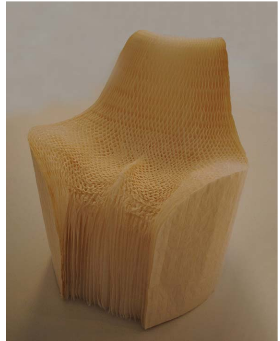
Figure color-13d Honeycombed paper (made from layers of glassine) used in the Honey-Pop armchair, designed by Tokujin Yoshioka's (2000–2001). Photography by Jim Postell, 2011.
