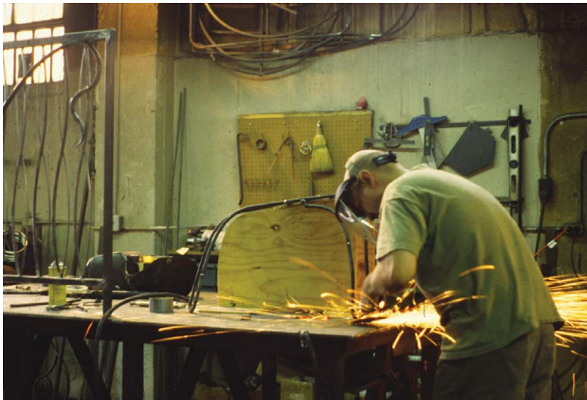
Figure 8.55 Student grinding a metal weld. Photography by Jim Postell, 2006.
