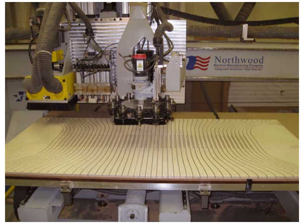
Figure 4.110 CNC fabrication—photograph of paths being CNC milled into 48 × 96-inch plywood sheet. Production model. Photography by Greg Lewis, 2006.
