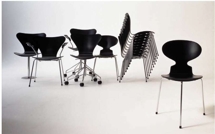
Figure 2.36 Ant and Series 7 fabricated using molded beech plywood. Stacking chairs, designed by Arne Jacobsen (1952.1955), manufactured by Fritz Hansen, Denmark. (Ant chair). 19 inches wide and deep; 30¼ inches high; 17¼ inches seat height (48 cm wide and deep; 77 cm high; 43.8 cm seat height). Photography courtesy of Erik Skoven and Fritz Hansen, Denmark.
