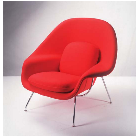
Figure 2.10 Womb chair, designed by Eero Saarinen, (1946–1948). Manufactured by Knoll International, upholstered in molded latex foam over a fiberglass, reinforced plastic shell, supported by slim, chrome-plated steel rod legs and base. 40 inches wide; 34 inches deep; 35½ inches high; 16 inches seat height; 20½ inches arm height (101.5 cm wide; 86.5 cm deep; 90 cm high; 40.5 cm seat height; 52 cm arm height). Photography courtesy of Knoll, Inc.
