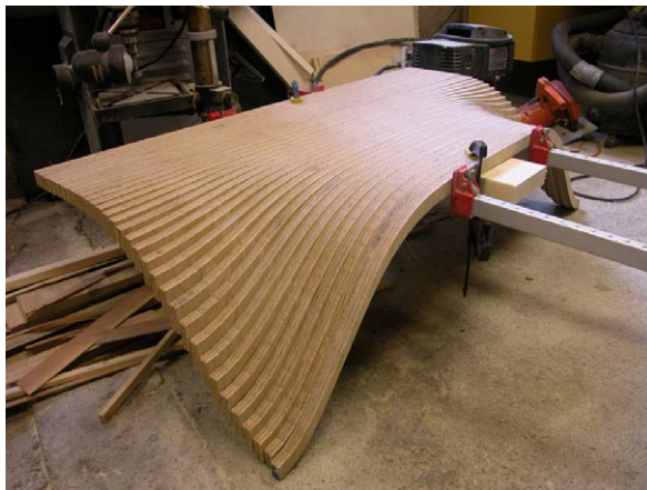
Figure 4.111 Initial parts clamping—test assembly in shop. Edge finish rough as a result of CNC water jet experiment. Photography by Greg Lewis, 2006.
