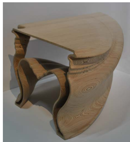
Figure 10.74 Cinderella table (2005), view showing laminated and digitally milled plywood. Photography by Jim Postell, 2011.
