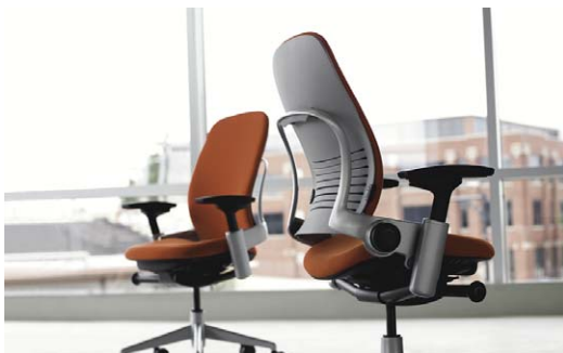
Figure 2.44 Leap office chair, designed by Steelcase and IDEO (1999), manufactured by Steelcase. The depth of the lower-back support is adjustable by turning a knob, which controls the tension of a slotted, flexing polypropylene backrest panel. Photography courtesy of Steelcase, Inc.
