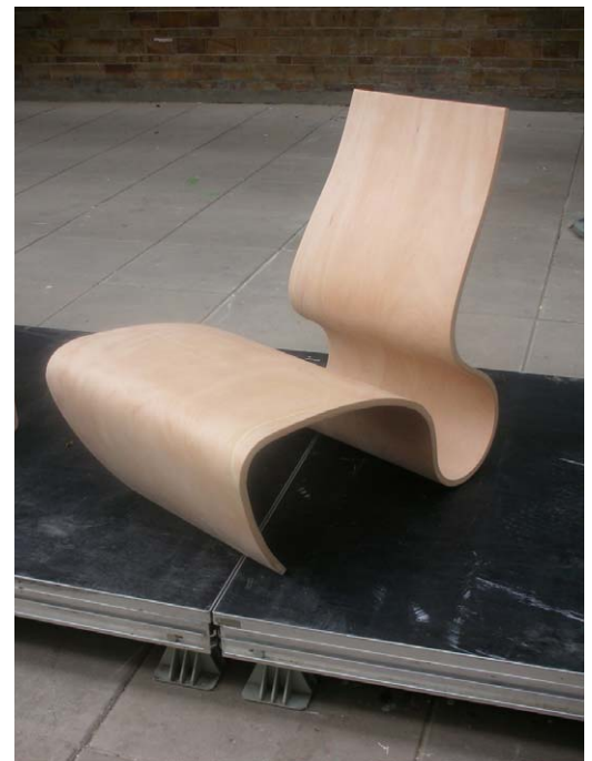
Figure 7.63 Vacuum molding and veneer-laminated seating, designed and fabricated by Jose Alberto Casas Pena (2006). Photography by Jim Postell, 2006.
