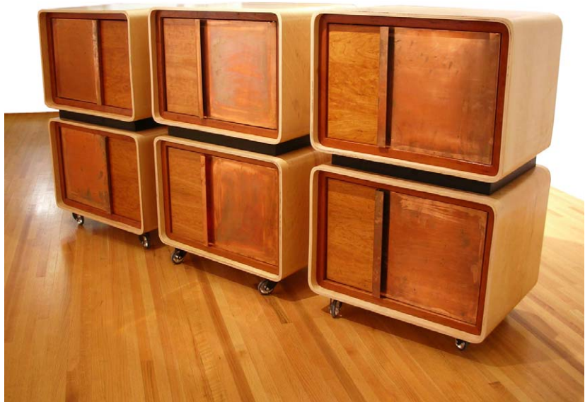
Figure 7.19 Folded copper drawer fronts with integrated copper handles inset in six Baltic birch storage units, designed and fabricated by Jim Postell (2005). Photography by Jim Postell, 2009.
