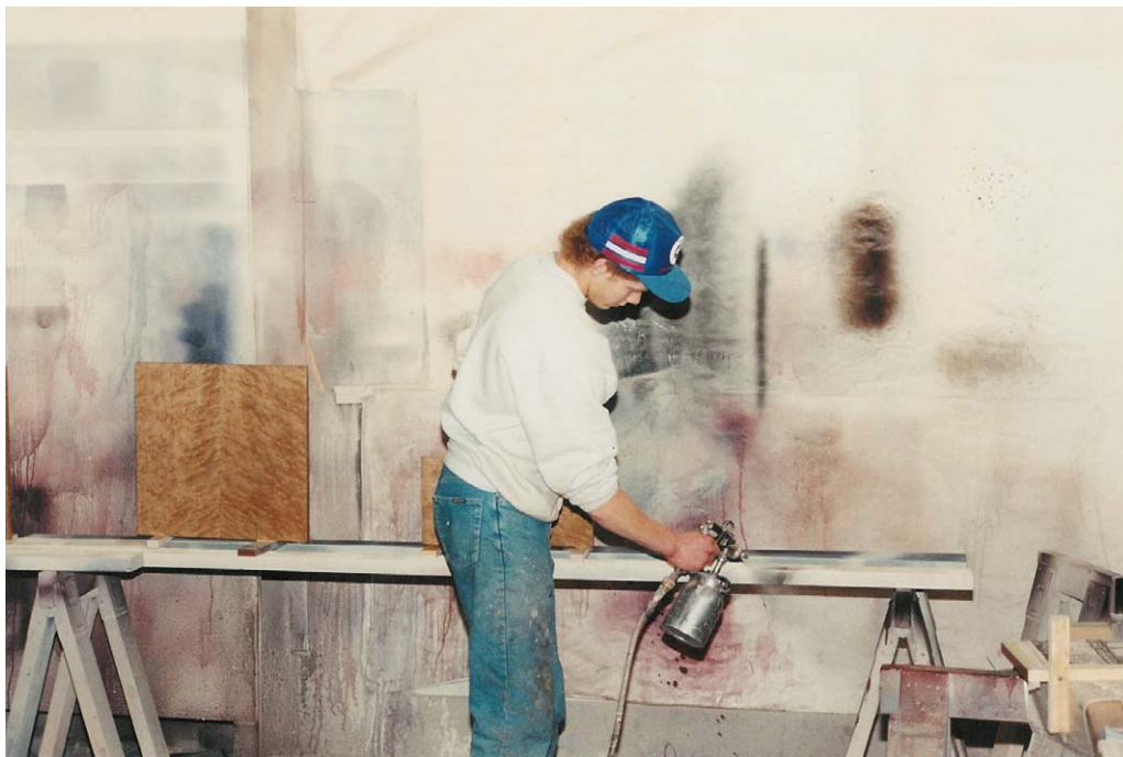
Figure 8.50 Spray finish using nitrocellulose lacquer. Photography by Jim Postell, 1994.
