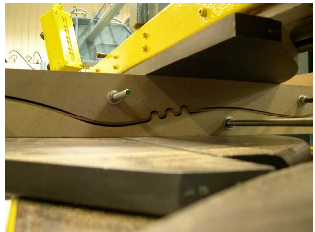
Figure 6.62 Pressing Maplex (cellulose fiber material) in a two-part press. Courtesy of Emiliano Godoy. Credit: Erika Hanson, 2005.
