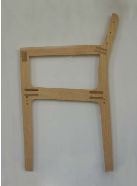
Figure 8.18 Section cut showing wood dowel connections in a chair. Photography by Jim Postell, 2006.
