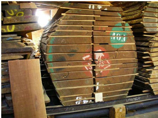
Figure 7.60 A boule log, plain-sawn mahogany lumber reassembled with spacer strips. Photography by Jim Postell, 2006.
