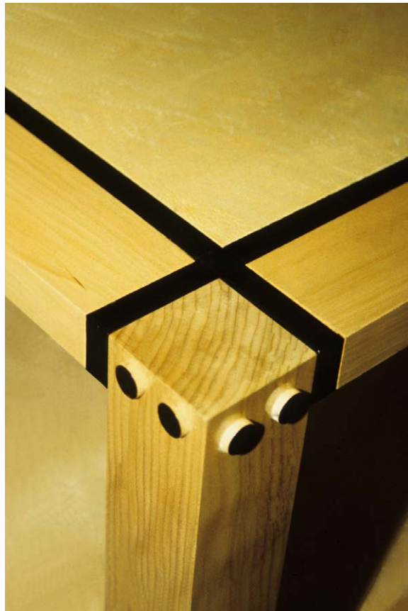
Figure 8.19 Corner detail—wood dowel connections. Photography by Jim Postell, 1994.
