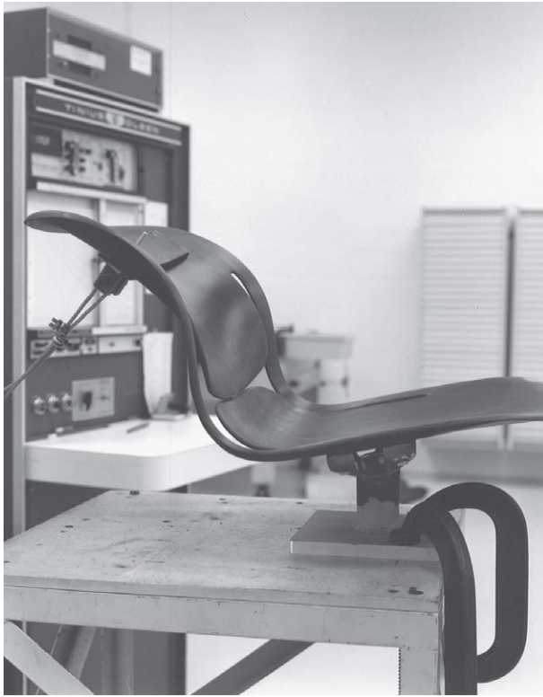
Figure 6.33 Testing the Equa chair's split shell made of glass-fiber-reinforced polyester, which permits the seat to operate independently of the side elements. Manufactured by Herman Miller, Inc. Photography courtesy of Herman Miller, Inc.
