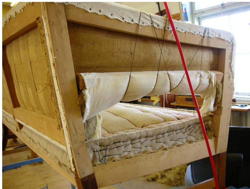
Figure 8.47 Upholstery in the making—showing various types of materials: lumber, nails, staples, and wire. Photography by Jim Postell, 2006.
