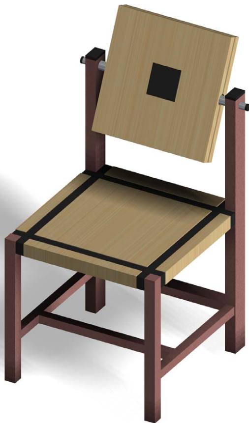
Figure 5.38 Ad quadratum geometry used to compose a chair made of Baltic birch plywood, cherry, and neoprene 80. Computer model by Jim Postell, 1994.
