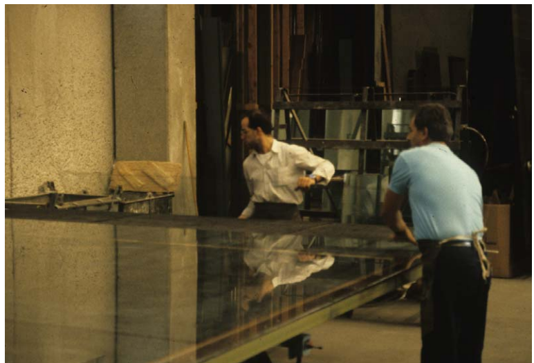
Figure 4.67 CNC device cutting 12-mm glass using very high water pressure for the Ghost chair at Fiam. Photography by Jim Postell, 1990.
