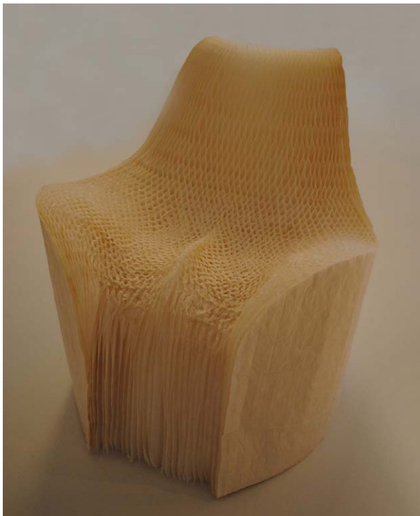
Figure 7.43 Honeycombed paper (made from layers of glassine) used in the Honey-Pop Armchair, designed by Tokujin Yoshioka (2000–2001). Photography by Jim Postell, 2011.
