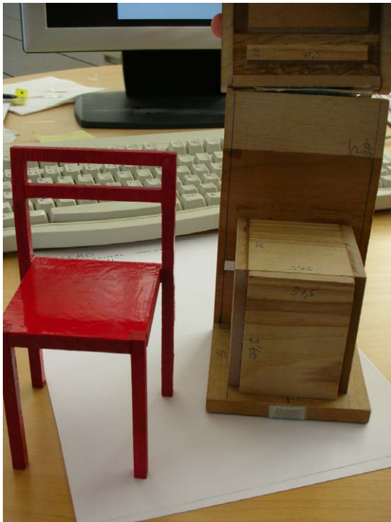
Figure 6.31 Scaled 1:5 model of a two-part form for Non Rubber. Photography by Jim Postell, 2006.
