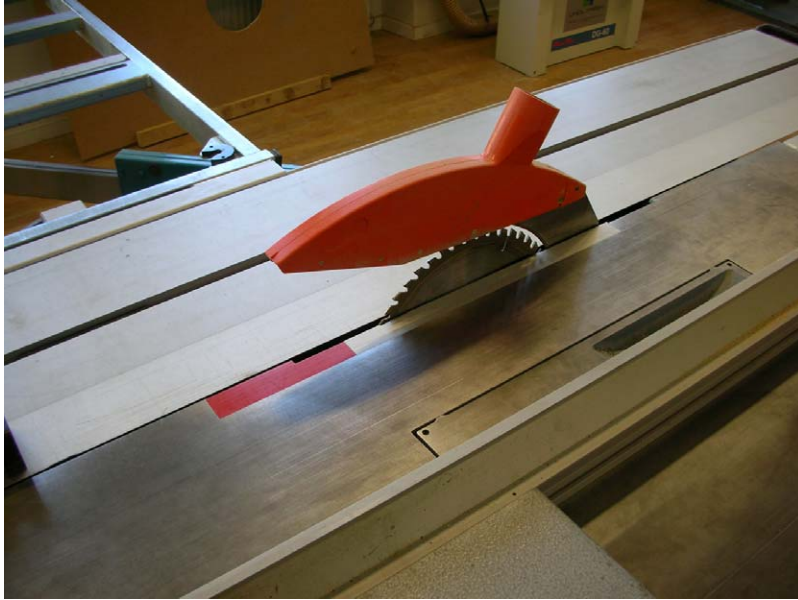
Figure 8.6 Table saw with guard and splitter (riving knife). Photography by Jim Postell, 2006.
