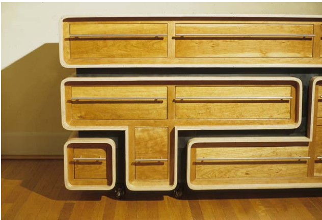
Figure 4.98 Detail—cherry, bending birch, and black neoprene 60. Photography by Jim Postell, 2005.
