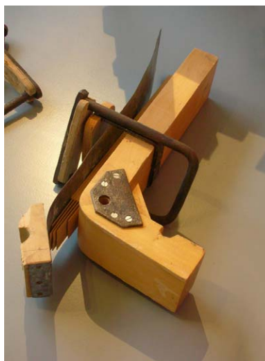
Figure 4.43 Formwork for the curved laminated birch leg—Stool 60. Photography by Jim Postell, 2006.
