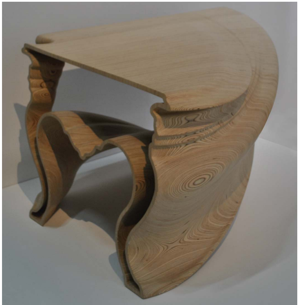
Figure color-16b Cinderella table (2005), digitally milled and hand-laminated plywood. Photography by Jim Postell, 2011.
