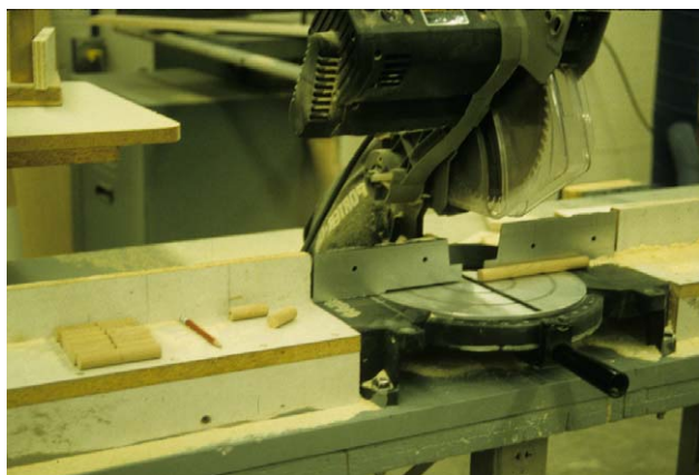
Figure 8.13 Miter saw (also known as a chop saw) is used for making cross-grain cuts. Photography by Jim Postell, 2006.
