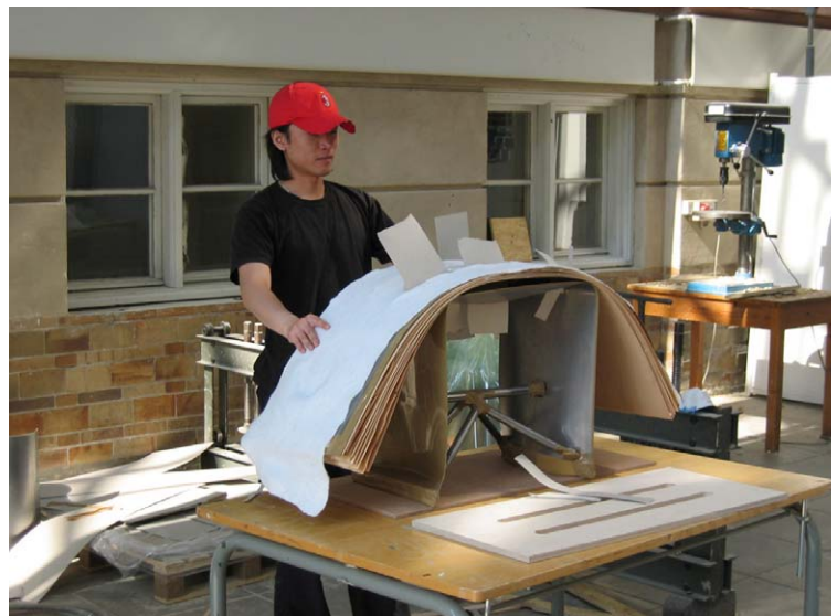
Figure 8.8 DIS student gluing wood veneers around a metal form prior to vacuum molding. Photography courtesy of Erik Skoven.
