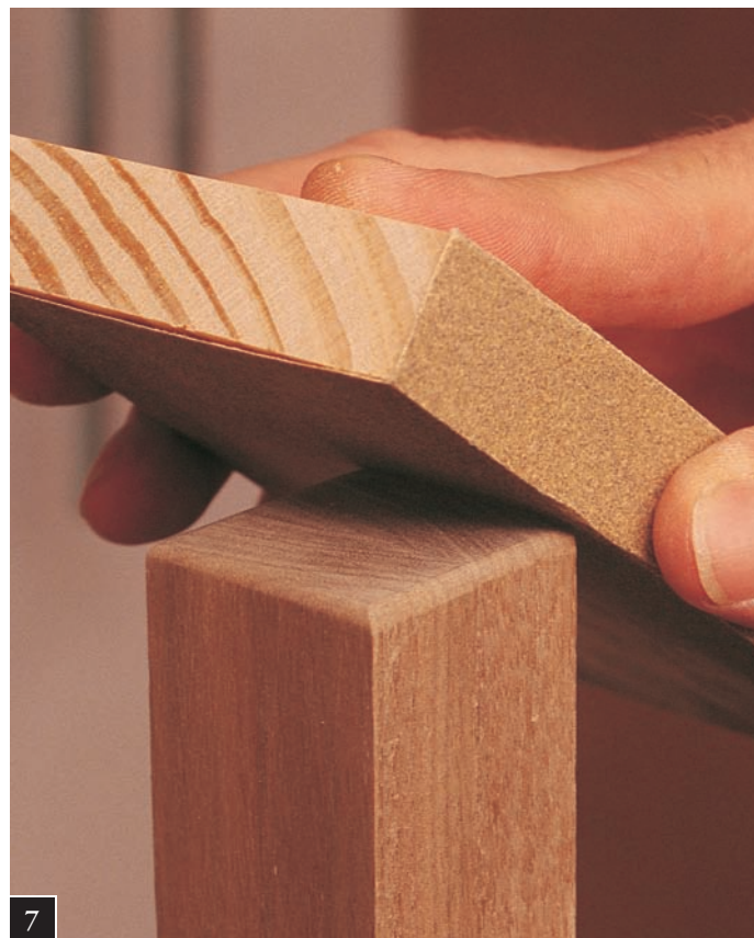
Rounding over or “breaking” the top edges of the legs is done easily before final assembly of the table.
