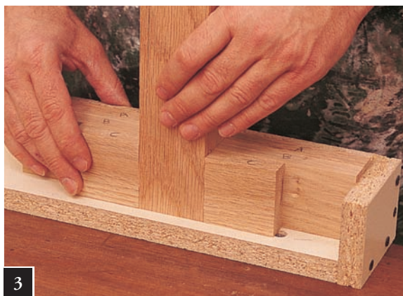
3 The leg will self-center when the two (2) A pieces are put into place with the leg. This whole assembly can be pushed against the jig side for proper alignment. Clamp in the usual way. Two (2) of these assemblies are needed.
