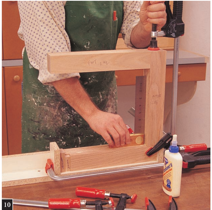
Glue-up of outer leg/foot assembly EFFG/LML to apron BDC.
