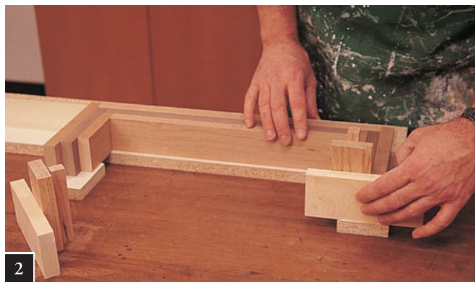
2 By using spacers at the ends of the D parts, clamp pressure is evened out.
