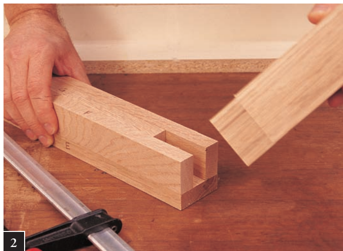
Assembly of LML foot and EFG outer leg. The outer leg pieces are glued up at this time because it is easier to capture the foot tenon in the loose parts. Two (2) assemblies are needed.
