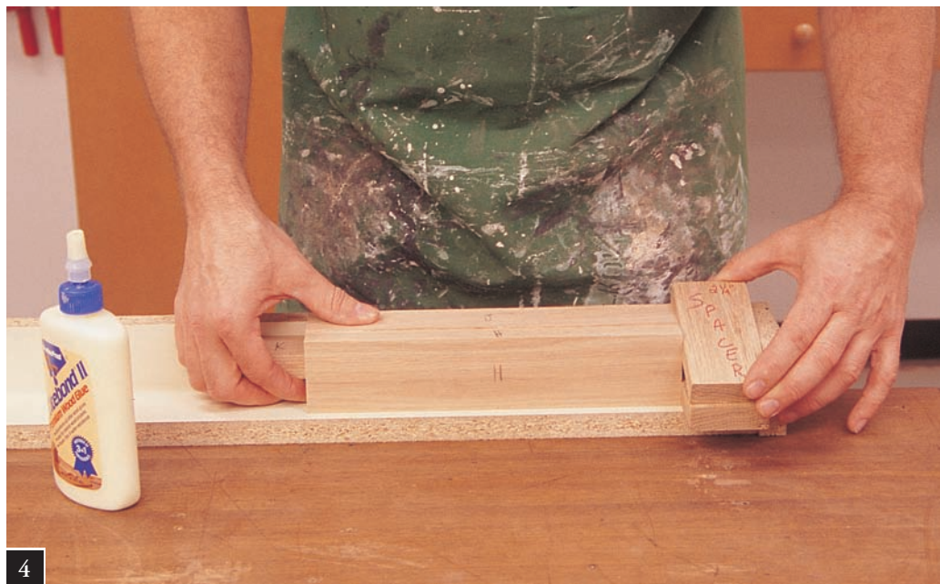
Use the 2 1/4" spacer to glue up leg HJK.
