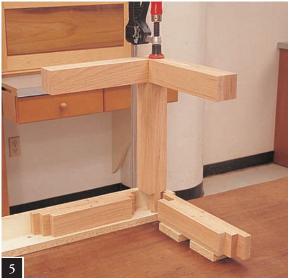
5 Setup for outer leg/foot assembly to outer aprons AEE and BDF. Aprons are loose until glue-up.
