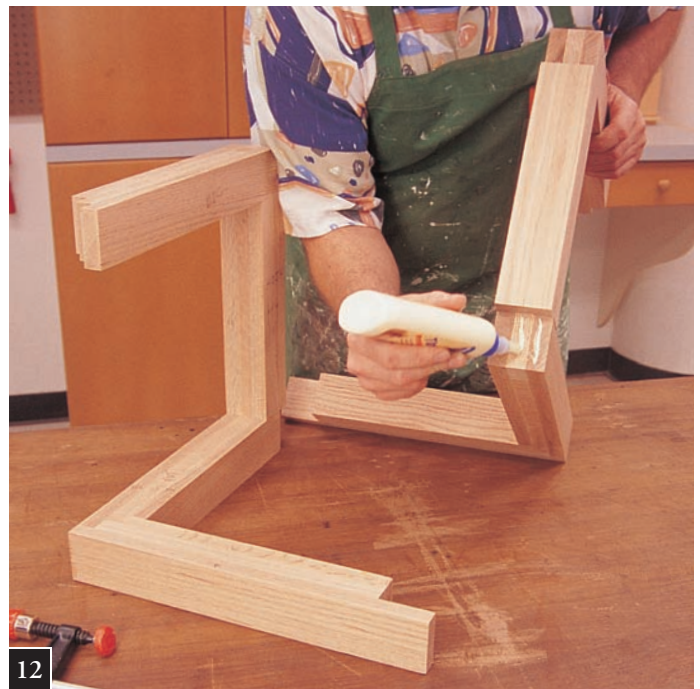
Apply glue to all surfaces of the joint that will touch.
