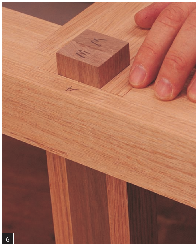
Dry fit the legs for a snug (but not too tight) fit.
