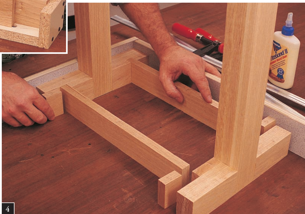
4 The two (2) leg/foot assemblies are connected with two (2) stretchers F. The two (2) D foot pieces are also attached at this time. Lay this assembly out as it will go together. Get all clamps ready, then proceed with the glue-up. (See photos 5 through 7.)
