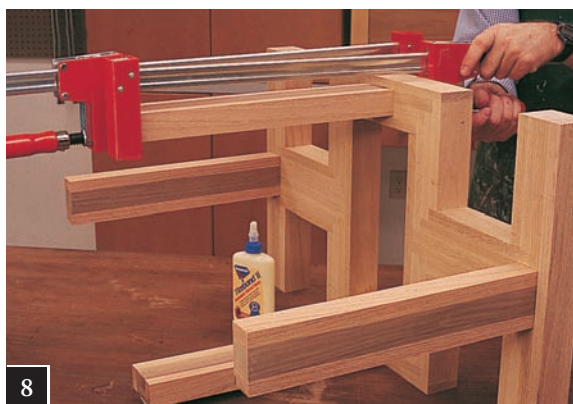
Put glue on the inside edges of the tenons on the legs and slide them into the mortises. This will keep the glue from getting all over the top of the tenons on the legs. Clamp squarely and let the glue dry overnight.
