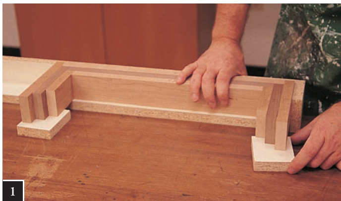
1 Setup for gluing subassembly E1E2E3 and two (2) D1D2D3. (Note the spacers to level the assembly with the jig.)
