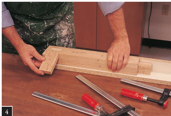
Glue-up of leg 2 (GGHK). (See the illustration for leg 2.)
