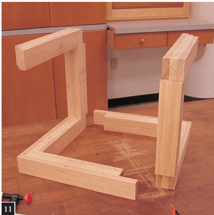
Setup for assembly of two inner leg assemblies.
