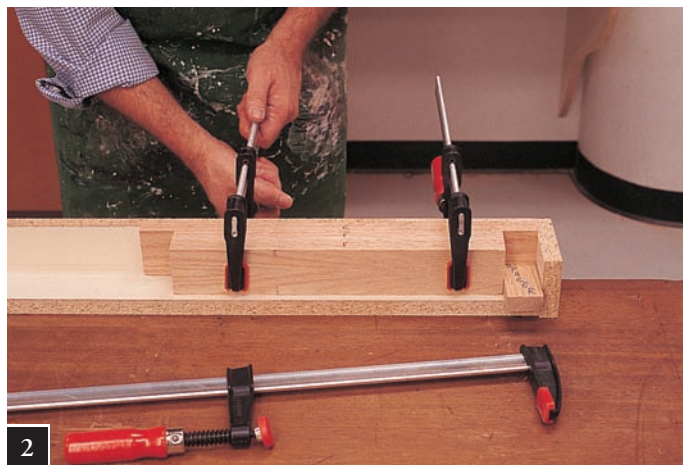
Glue-up of the top rail CFF using the 1 \frac{1}{2} " spacer.
