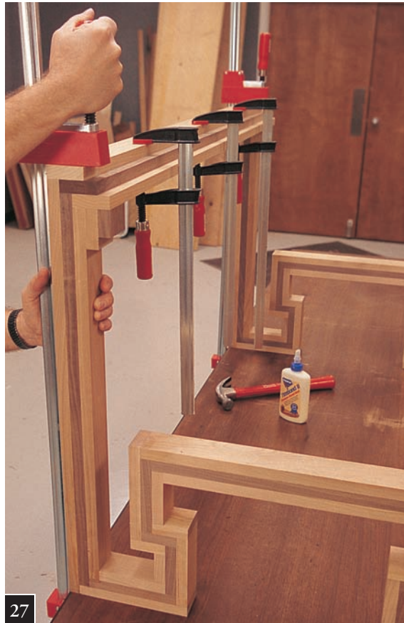
27 Clamp along the whole length of the G rail.
