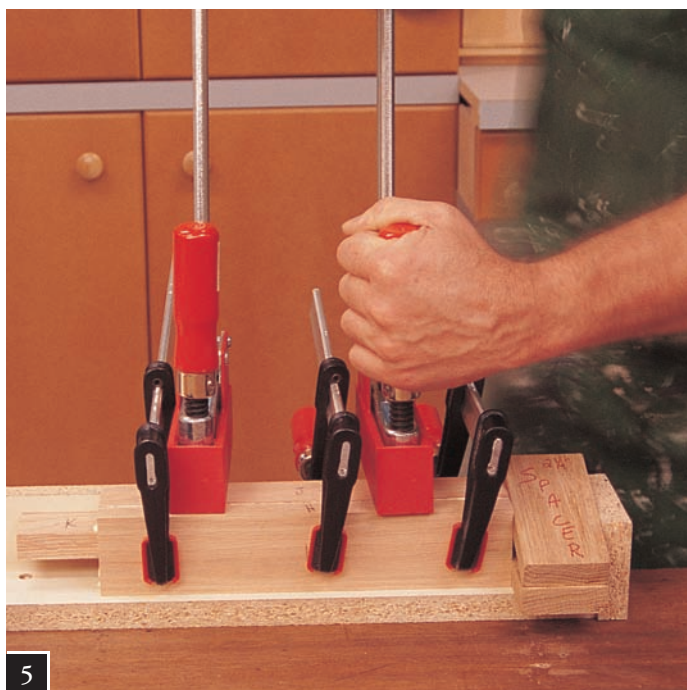
5 Final clamping of leg HJJK. (Note the vertical clamping. Pressure from two directions is important.) Two (2) inner legs are needed.
