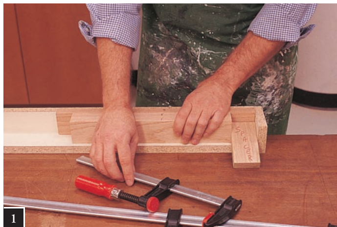
Glue-up of the top rail BFF using the 2 \frac{1}{4} " spacer.
