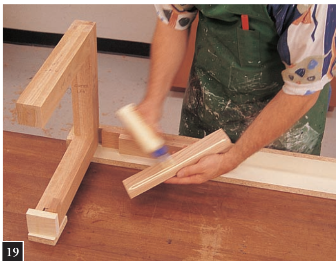
19 Setup for gluing end apron ACD to outer leg/foot/apron assembly.
