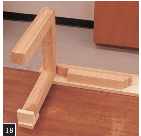
18 Setup for assembly of apron ACD to outer leg assembly.
