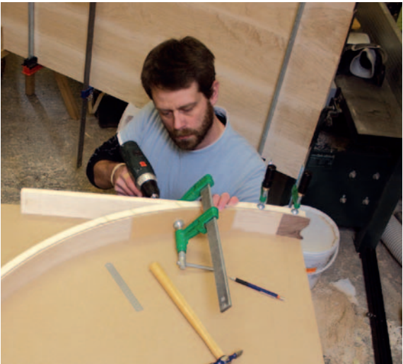
Pic.5 The straight component (C) needs to be rounded at the end to meet the inner (A) curved part of the leg assembly (above, left). These two parts can then be glued and screwed together (above). Once that is done extra laminations are glued to the top of the joint between the straight part (C) and the inner part (A) to cover the joint. The end of the straight part is then mitred (right) to join the outer leg (B)
