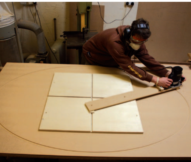
Pic.11 Cutting out the MDF template for the elliptical top. To keep the sheet stable for as long as possible, Steve routs most of the way through the MDF like this, then cuts away the waste with a jigsaw, running along the centre of the groove. This leaves a little waste left at the bottom of the 'groove'. He then uses a laminate trimming cutter, with a bearing, against the routed edge to clean it up
