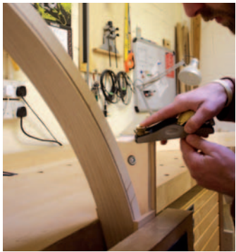
Pic.5 The straight component (C) needs to be rounded at the end to meet the inner (A) curved part of the leg assembly (above, left). These two parts can then be glued and screwed together (above). Once that is done extra laminations are glued to the top of the joint between the straight part (C) and the inner part (A) to cover the joint. The end of the straight part is then mitred (right) to join the outer leg (B)
