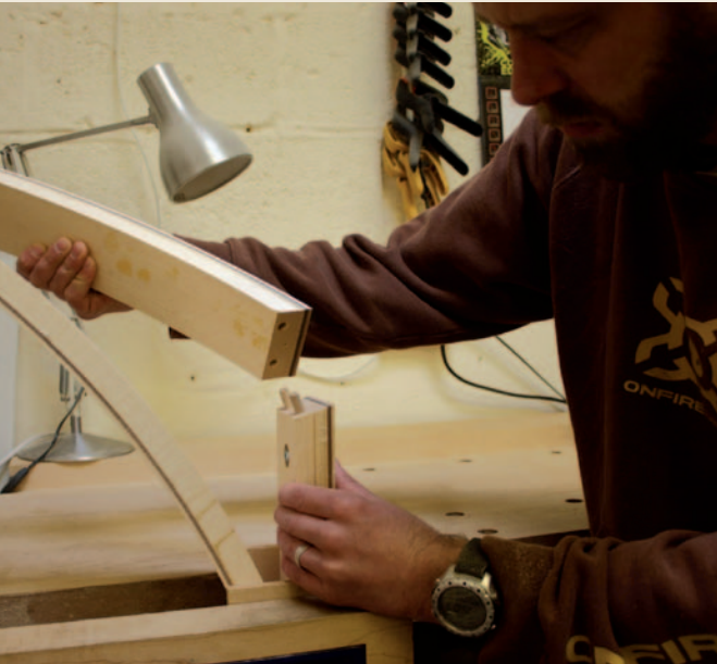
Pic.6 The dowel drilling (or dowel routing) jig is screwed to the mitred end of the straight part of the leg assembly, and then to the mitred end of the outer leg part (B). Steve makes lots of these 'instant' jigs in his work
