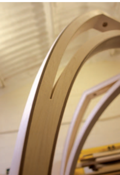
Pic.13 There is an extra layer of veneer in the joint between the curved parts to avoid a dust trap
