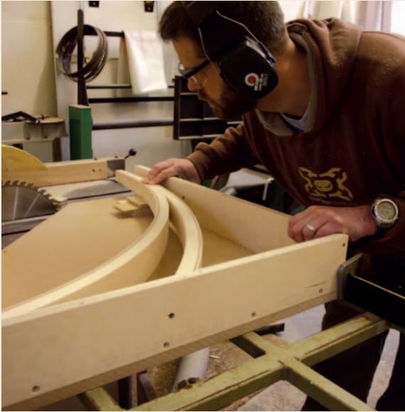
Pic.10 Having tapered the legs, the same box can be used on a tablesaw for cutting the legs to identical length
