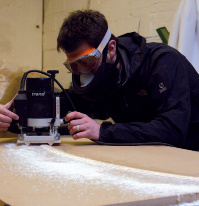
Pic.4 This is a great way of levelling the edges of laminated components, returning them to the former, but lifted a little on blocks. You then run a router over the top, with triangular section runners fitted to a sub-base. Steve used a two-flute straight cutter, but subsequently discovered the Wealden six-wing surface cutters, which would have produced a much smoother finish for this job
