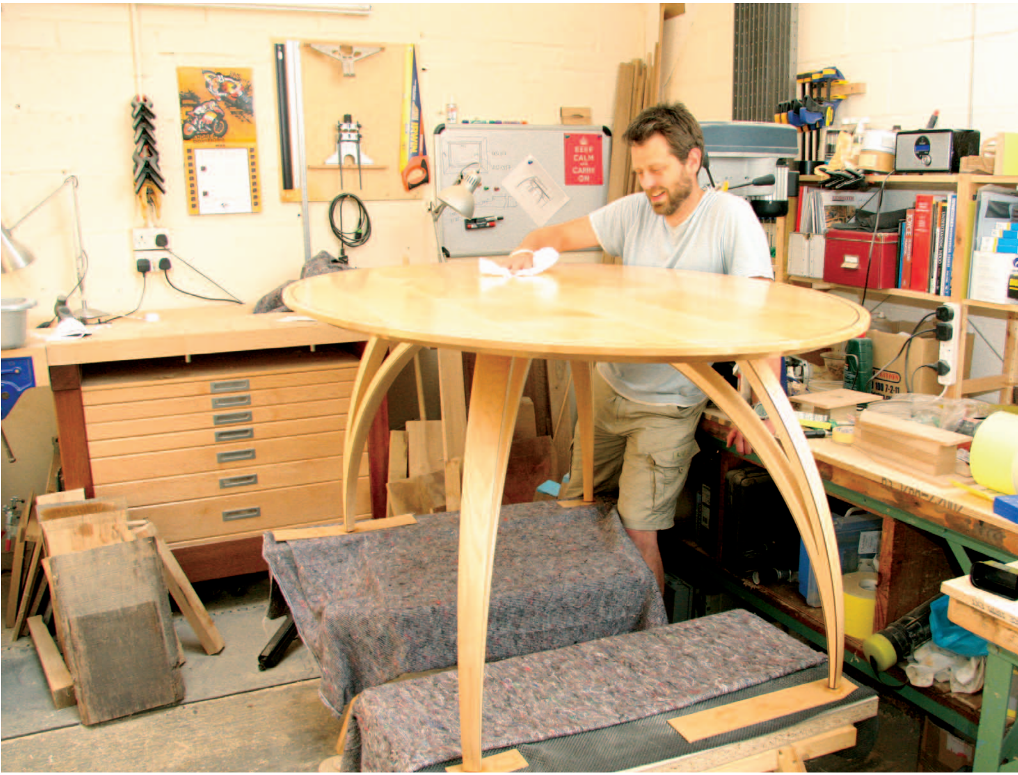
Pic.1 The four leg assemblies comprise two curved components each, which were laminated in separate formers (left)
