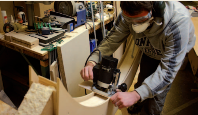
Pic.2 Skiing the inside face of the inner leg component to taper the thickness from the top down to the foot
