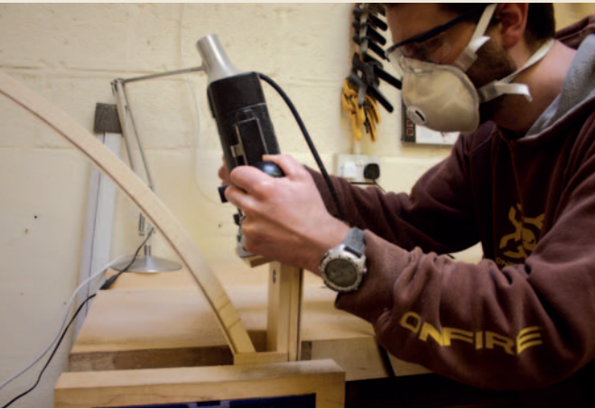
Pic.4 This is a great way of levelling the edges of laminated components, returning them to the former, but lifted a little on blocks. You then run a router over the top, with triangular section runners fitted to a sub-base. Steve used a two-flute straight cutter, but subsequently discovered the Wealden six-wing surface cutters, which would have produced a much smoother finish for this job
