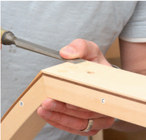
Pic.7 Paring back the dowels after trying to use screws to pull up the mitre between the outer leg (B) and the straight part (C). The leg assemblies are joined at the centre in pairs first (above right)
