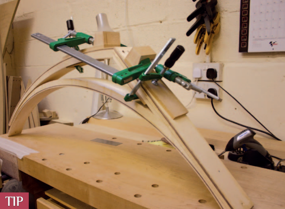
Pic.8 Using 'donkey's ears' to pull the mitred joint between the straight and outer curved components together. At this stage the two curved parts are not joined at the feet, and are flapping around. An extra layer of veneer is glued between the two curved parts so there isn't a fine dust trap
