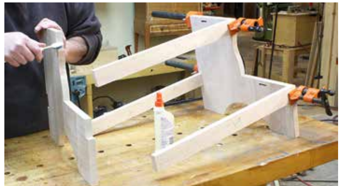
(Fig. 8) Leaving one side clamped as you work on the other makes the glue-up smooth.
