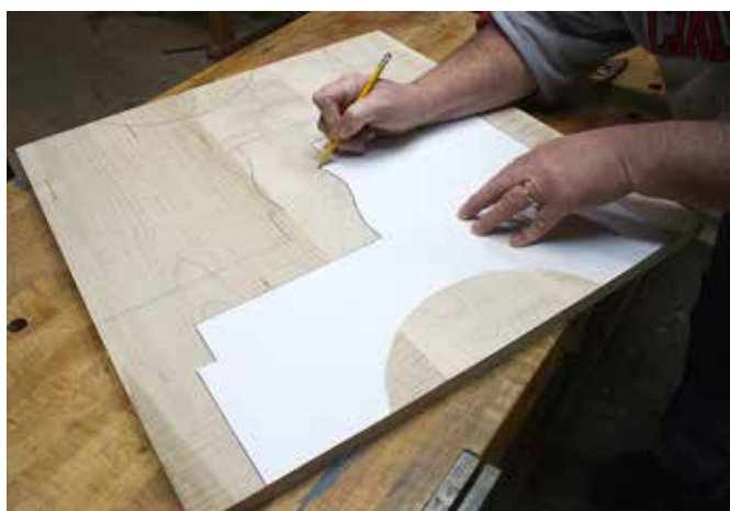
(Fig. 1) Save time by laying out both sides on a single assembled panel, and by printing and using a full-size pattern.
