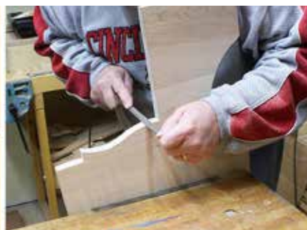
(Fig. 5) I find that smoothing the edges of the sides is both a power-tool and hand-tool operation – a spindle sander makes quick work of the arc and can only smooth a portion of the shaped design between steps. The area close to the lower steps is where a file becomes a better choice.
