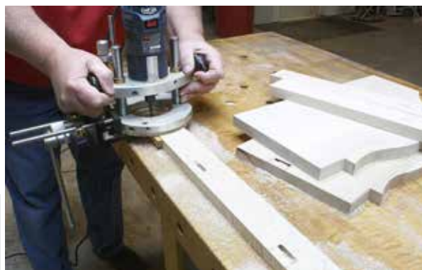
(Fig. 6) A router and 1/4" spiral up-cut router bit are great to dig out the slots for wooden clips – three along the front braces and two at the sides hold the treads secure.
