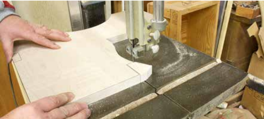
(Fig. 4) With the arc cut along the side bottom cut, it's easier to get the top brace notch cut.
