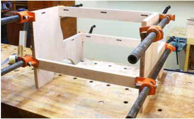
(Fig. 7) A view from the rear of the steps after a dry-fit assembly show the location of the slots for the wooden clips.
