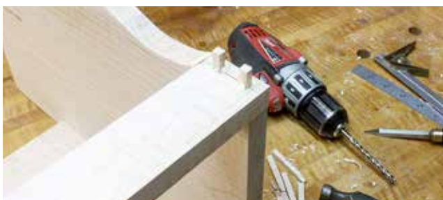
(Fig. 9) If you allow the glue to dry, it holds the ends of the braces secure as wooden pegs are driven for added support – without the glue, it's possible that the ends of the braces would split as the work was completed.
