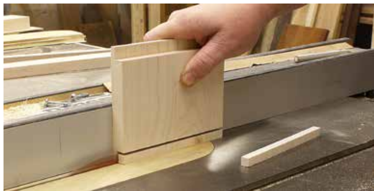
(Fig. 12) The tongue formed on the ends of a scrap have the grain orientation correct for making clips.
