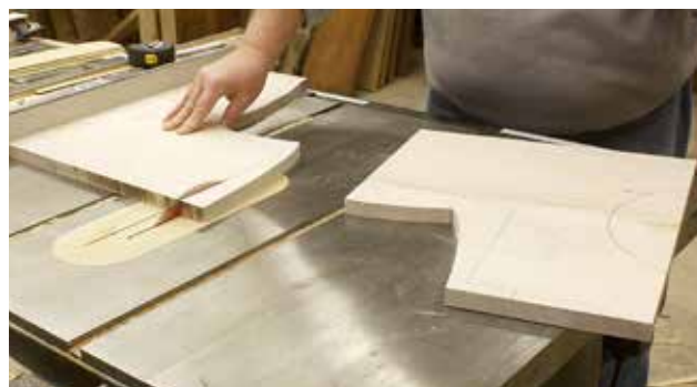
(Fig. 3) I find it better to use my table saw to trim the straight cut lines along the top, back and front of the bed step sides.
