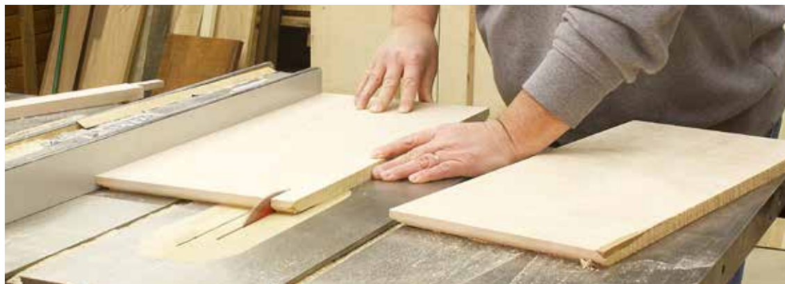
(Fig. 11) By leaving the steps over-wide as you route or shape the edge and ends, you can easily eliminate any problems, such as blow-out or those considered operator error.
