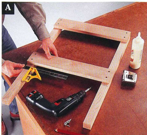
Check with a combination square to make sure the desk legs are square to the ends.
