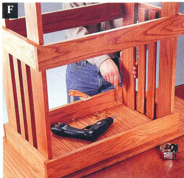
Attach the table panel to the base with corner braces.
