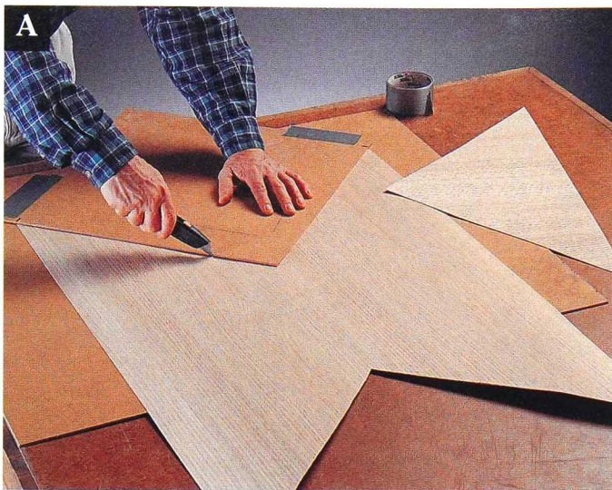
Use a sharp blade to cut the veneer pieces along the template. Press firmly to prevent the veneer from sliding.
