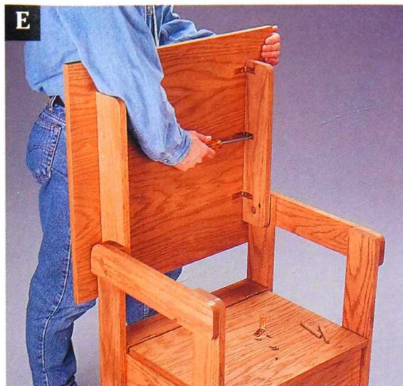
Attach the tabletop to the table cleats with brass corner braces.
