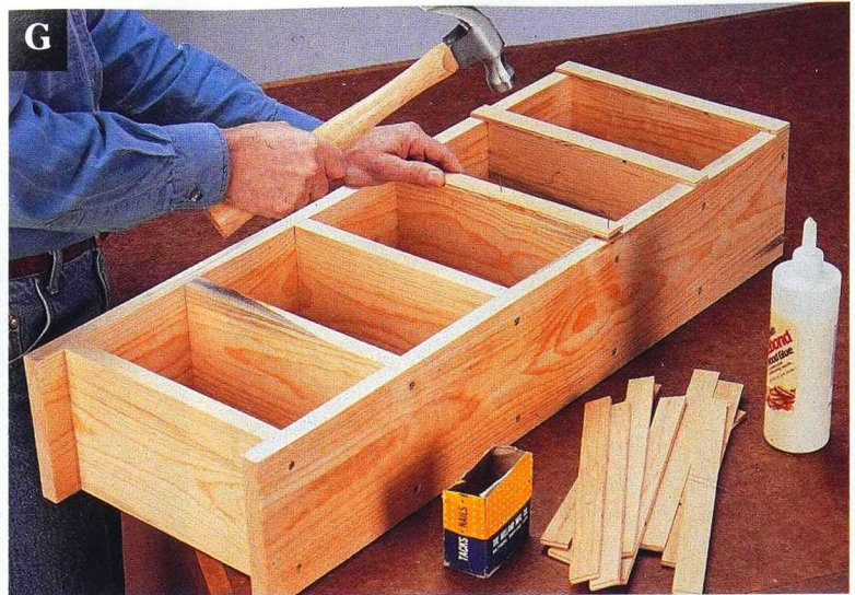
Using glue and 4d finish nails, attach the swing-out shelf sides.
