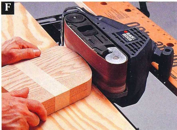
Clamp a belt sander and a scrap board to the workbench to create a stationary shaping tool.
