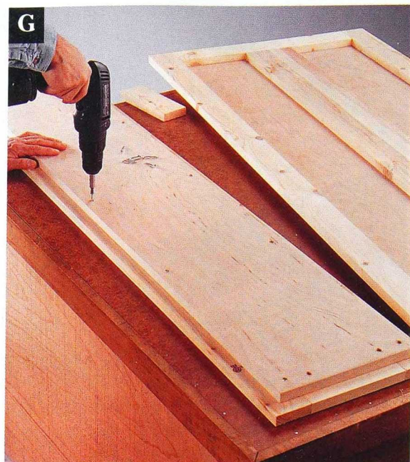
Attach strips of 1 x 3 to the fronts of the door panels to create a frame.
