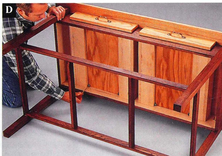
Slide the drawers into place. Then, install rubber feet at the back corners to serve as drawer stops and keep the drawers centered.
