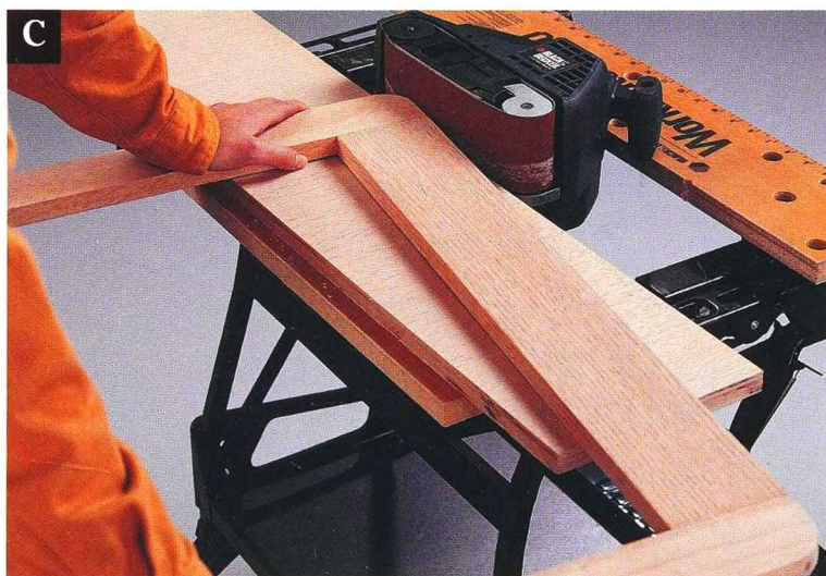
Mount a belt sander to your worksurface, and use it to smooth the roundover cuts on the frame.
