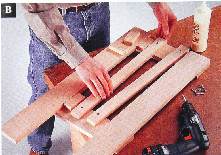
Position the base slats between the base legs, and attach them to the inside faces of the cross rails.
