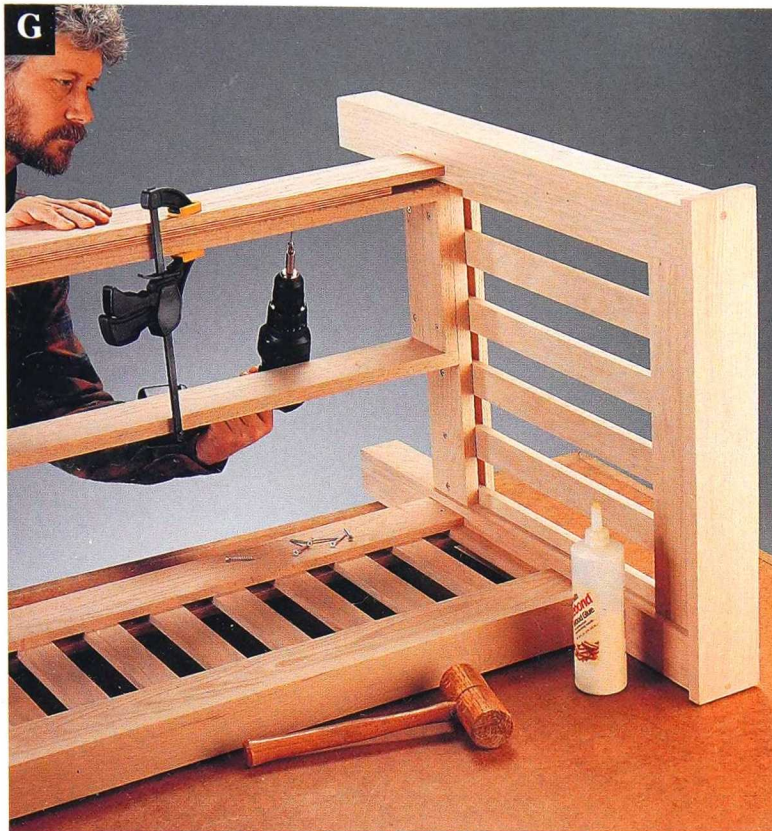
Clamp the spacer and frame face to the support frame. Attach them with glue, and drive screws through the inside of the support frame.
