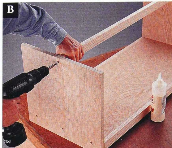
Secure the stringer in place with glue and screws.
