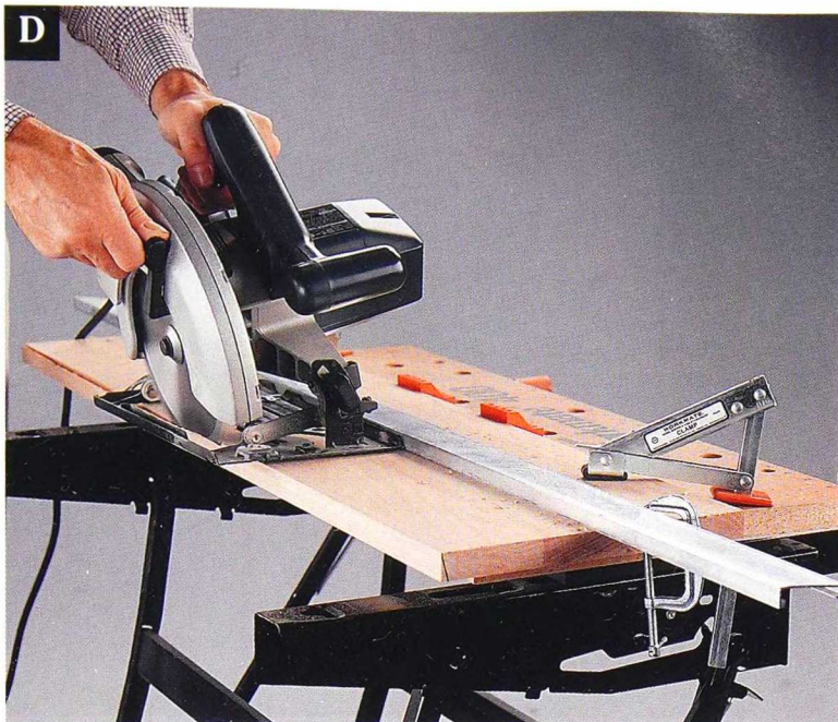
D Use a circular saw and a straightedge as a guide to make a slight bevel on the front edge of the desk top.
