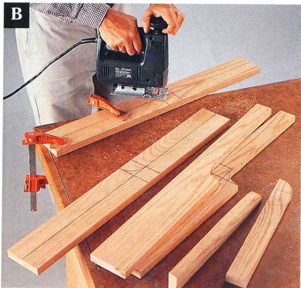
Cut the curved tapers in the legs with a jig saw.
