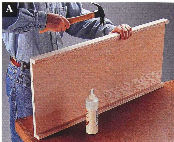
Fasten the shelf edges to the shelf panel with glue and 6d finish nails.
