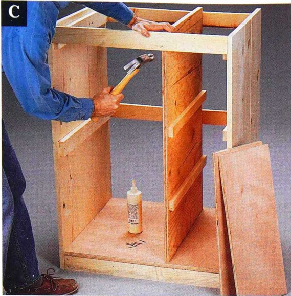
C Install the divider 9" in from the right side of the cabinet.
