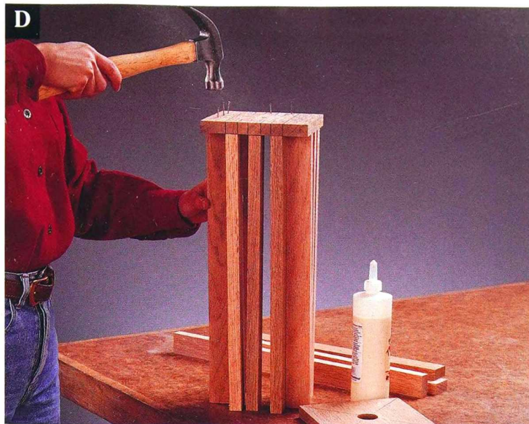
Attach the slats to the top plate with glue and 6d finish nails.
