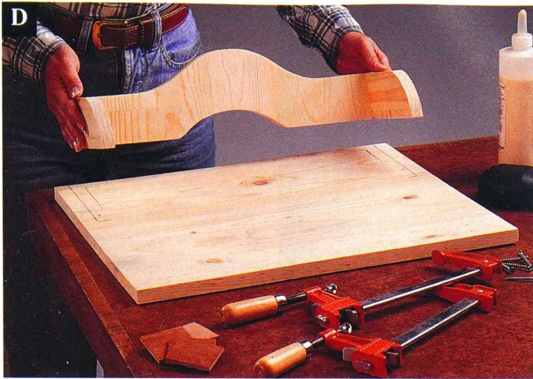
D Draw reference lines on the top. Then, drill pilot holes and attach the back rail and wings.
