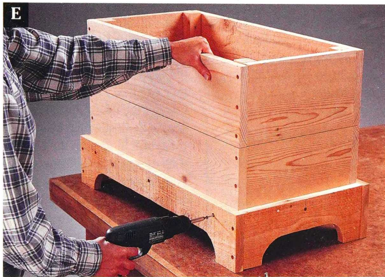
Set the box frame into the base, and fasten it with evenly spaced screws.
