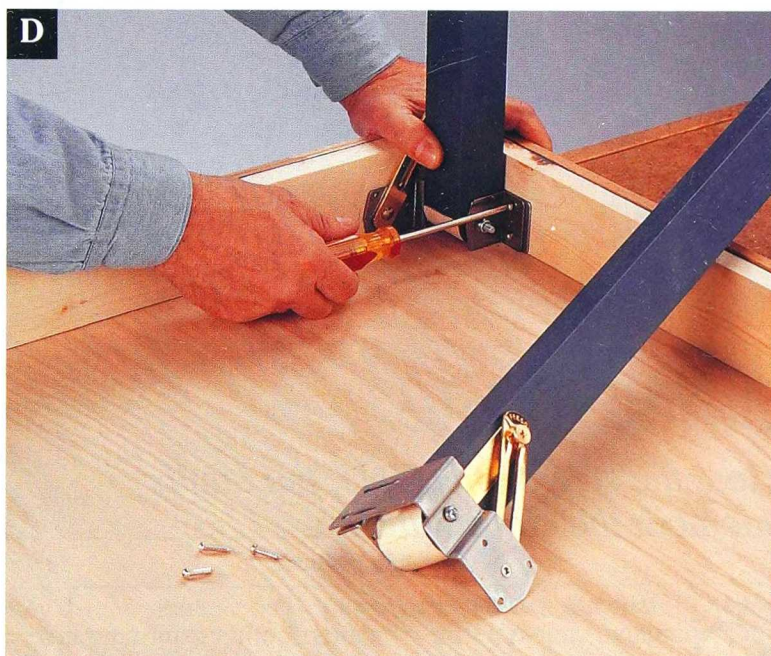
D Attach the card-table leg fasteners to the rounded ends of the legs. Then, attach them at the inside corners of the tabletop frame.
