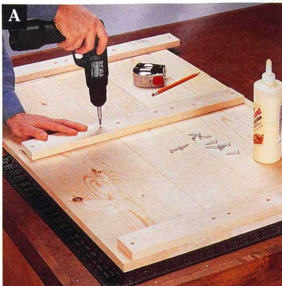
Fasten cleats to the side and middle boards, forming the cabinet sides.
