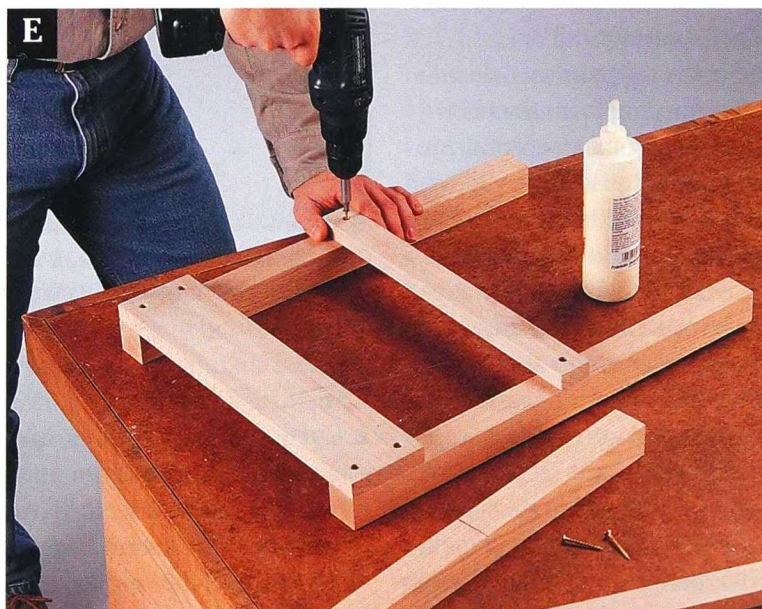
Attach the credenza ends and end rails to the legs with glue and wood screws.
