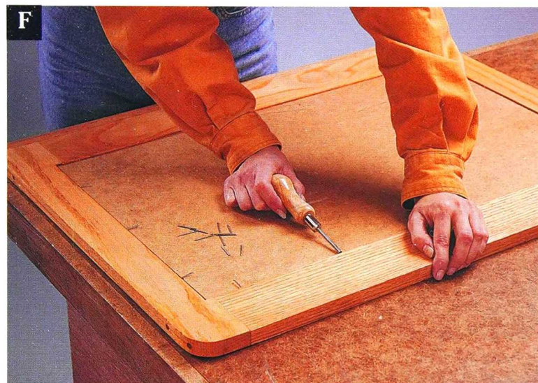
F Install the mirror and mirror back. Then, secure them to the frame with brads, using a brad pusher.
