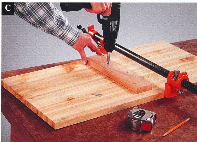
Attach the top cleat to the undersides of the tops, making sure it is centered between the ends and the sides.
