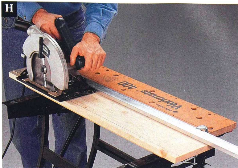
H Use a circular saw with a straightedge as a guide to rip-cut the door boards to size.
