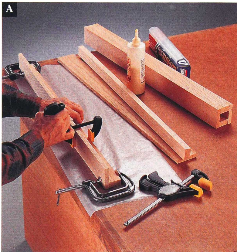
Assemble the legs with glue and clamps, using wax paper to protect your work surface.
