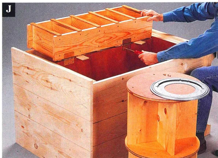
J With spacers in place to help align the parts, attach the swing-out rack to the divider with 3 \times 3 " butt hinges.
