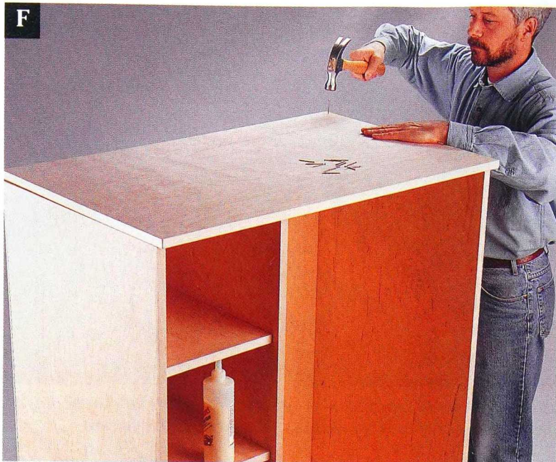
Mount the top panel so it covers the top edge of the back panel and overhangs the front edges of the side panels by \frac{3}{4} ".
