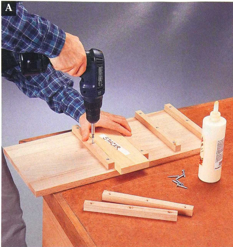
Use a spacer to keep the slats aligned properly, and attach them with glue and screws.
