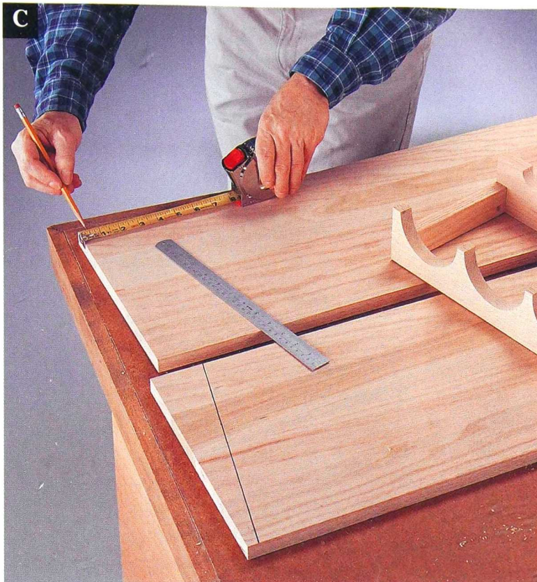
C Measure \frac{1}{2} " along the front and 2\frac{1}{2} " along the back of each side, and connect the marks for the bottom rack alignment.
