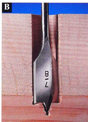
Use a scrap backer board to prevent tearout when drilling through a workpiece.
