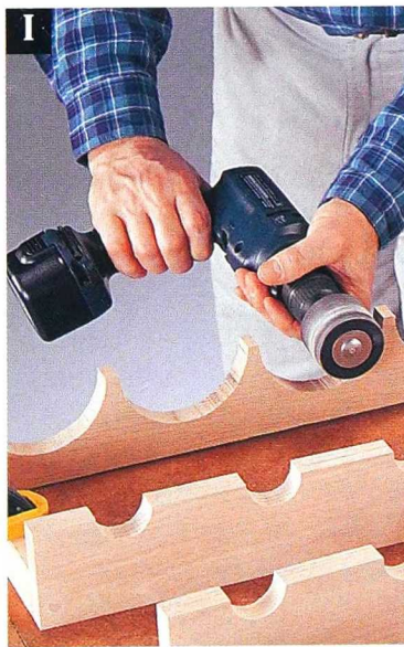
I Smooth curves and hard-to-reach surfaces with a drum attachment on your power drill.
