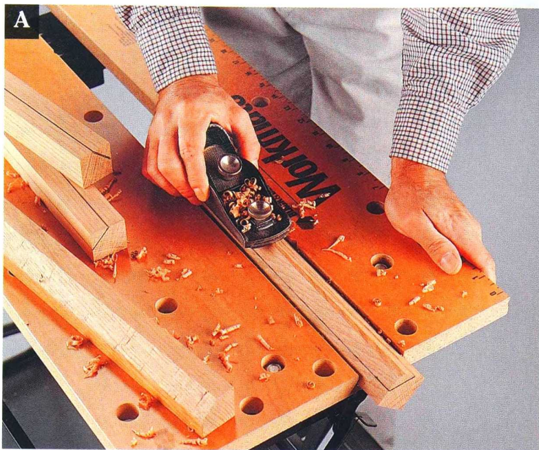
Use a plane to trim away one edge of each leg.
