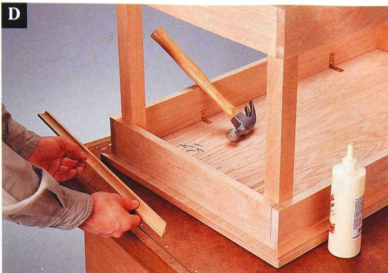
Install strips of oak cove molding along the underside of the desktop.
