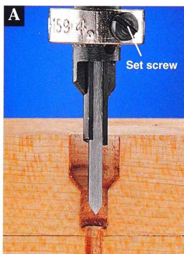
A combination pilot bit drills pilot holes and counterbores for wood screws in one step.
