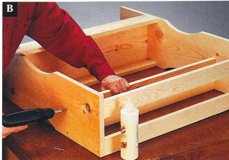
Fasten the bin stop board between the end panels to complete the assembly of the valet framework.
