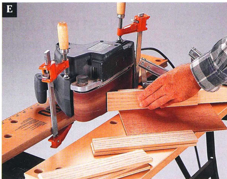
Clamp a belt sander to your workbench to make the divider bevels.
