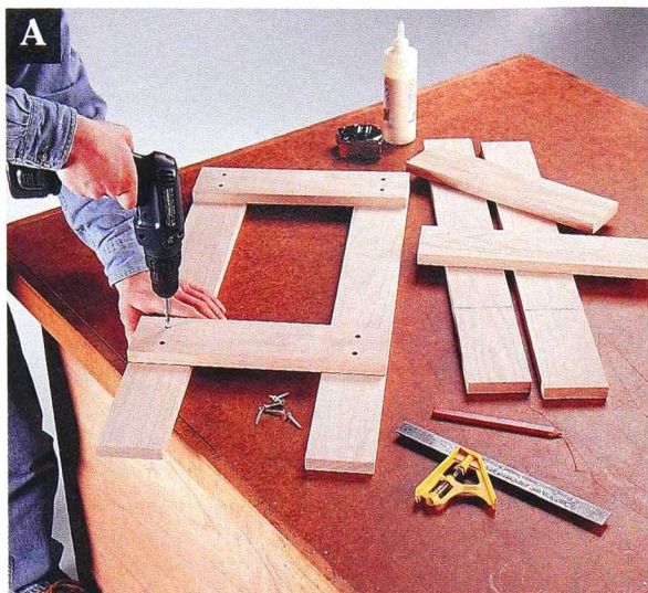
Attach cross rails to each pair of legs with glue and wood screws.
