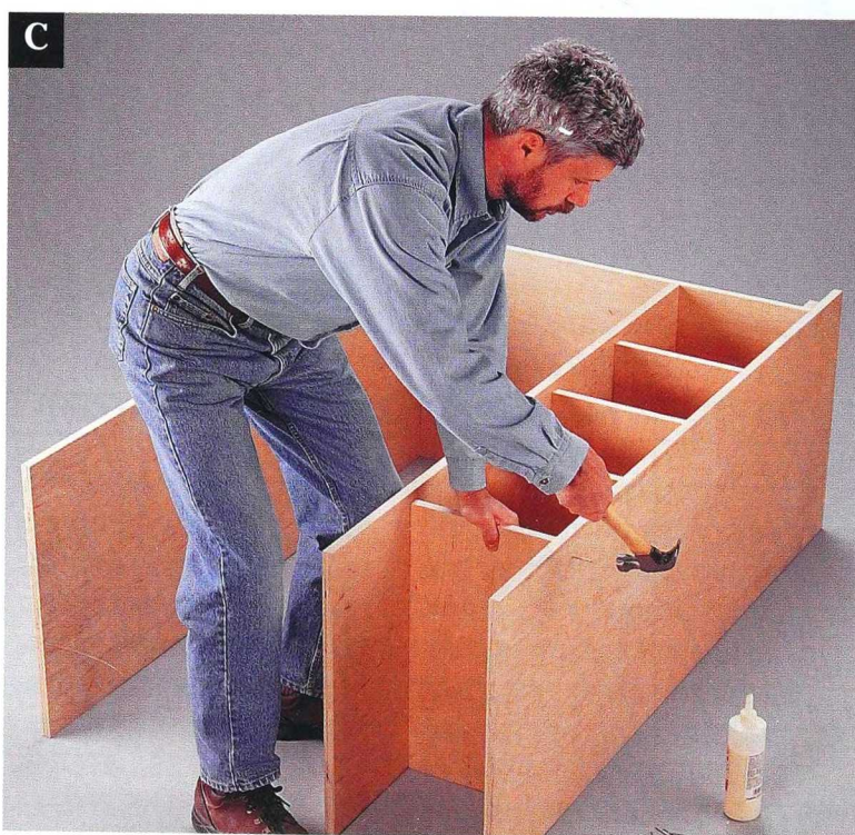
Fasten the shelves between the side panel and center panel with glue and finish nails.
