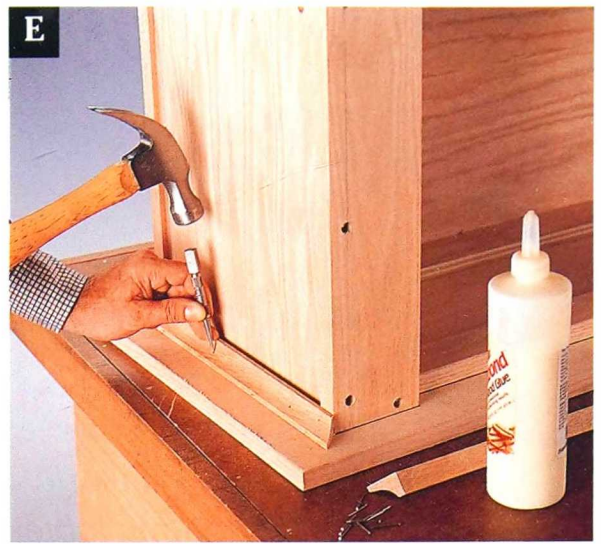
Miter-cut cove molding to cover the joint between the top panel and the carcass.
