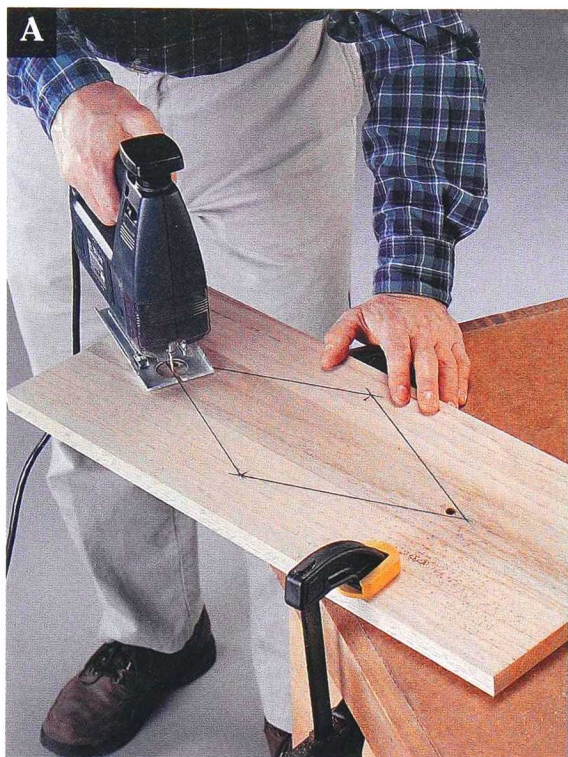
A Drill starter holes. Then, cut out the diamond shapes with a jig saw.
