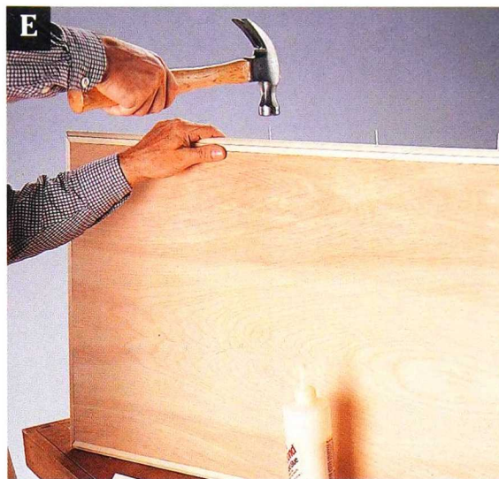
E Attach the top cap around the perimeter of the lid. Drive nails in partially before positioning the strips.
