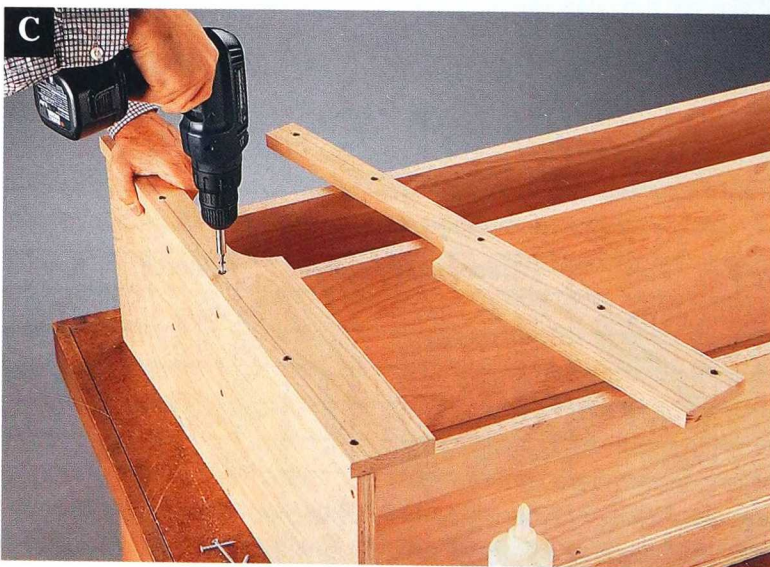
Fasten the legs to the front edges of the end panels. Make sure the outside edges of the legs overhang the end panels by \frac{1}{4} ".
