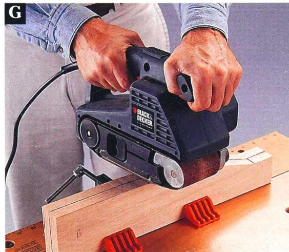
Gang-sanding is an easy method for creating two or more identical parts.
