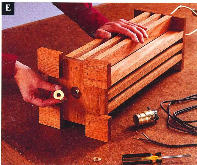
Install the threaded lamp tube, and secure it to the bottom plate with a washer and nut.
