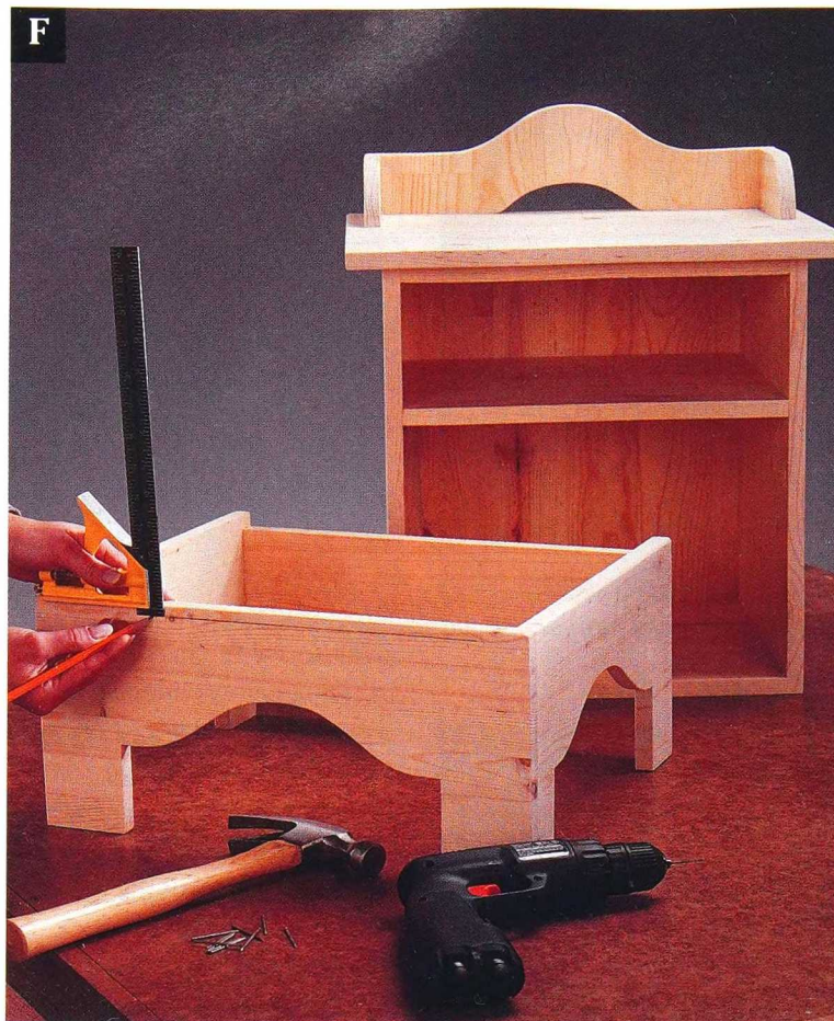
Use a combination square to mark the finish nail position on the base front and sides.
