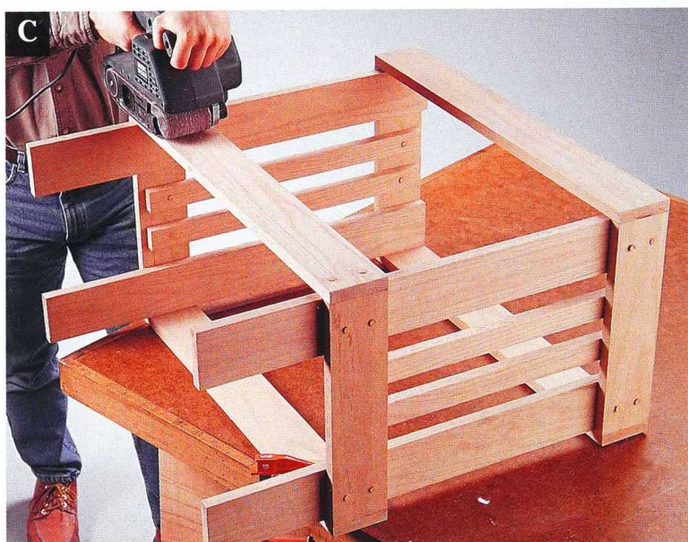
Sand the oak plugs flush with the surfaces, using a belt sander.
