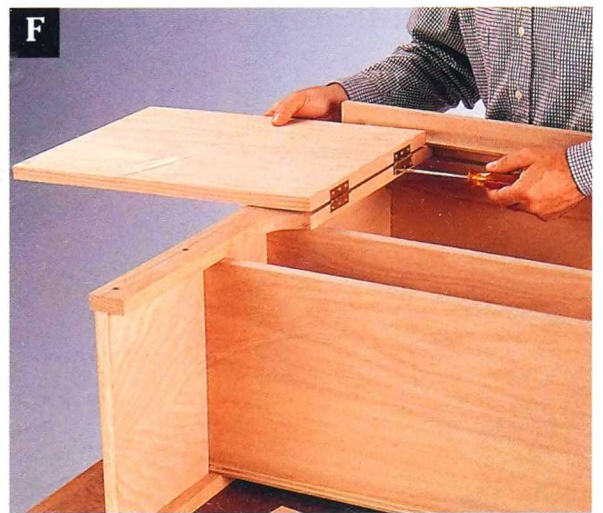
Attach each door to a leg, using 1\frac{1}{2} \times 3 " butt hinges.
