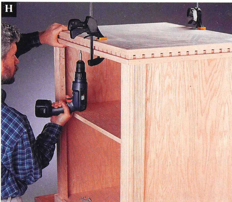
Apply glue and clamp the top in place. Then, secure it by driving screws through the stretchers.
