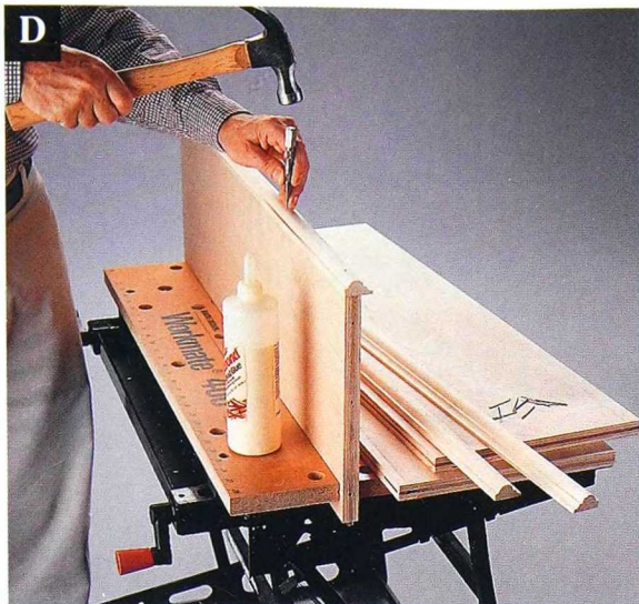
D Attach strips of panel molding to the front edges of the shelves.
