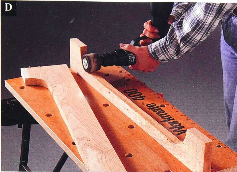
Smooth the jig saw cuts on the radius cutouts using a drum sander attachment and drill.
