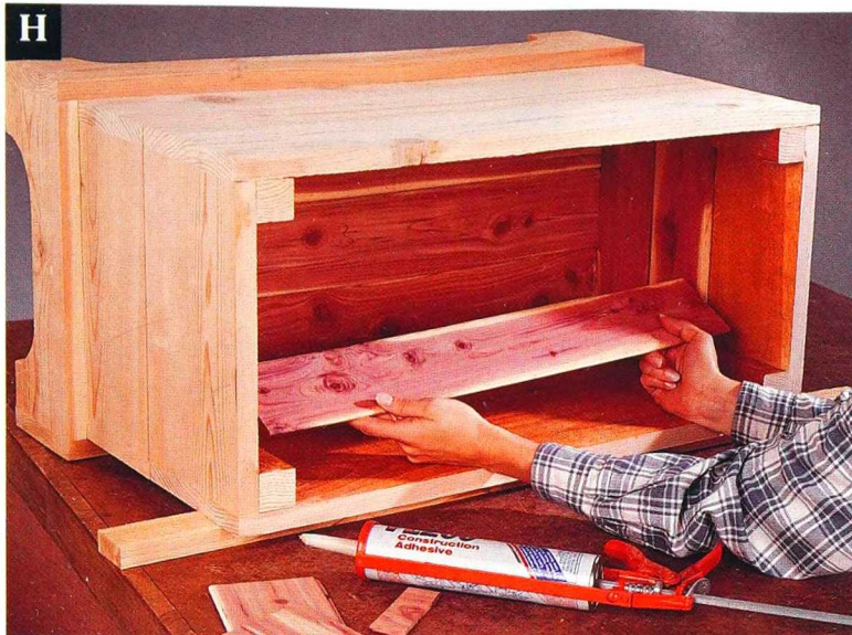
H Install aromatic cedar panels to the sides, ends and bottom, using panel adhesive and 2d finish nails.
