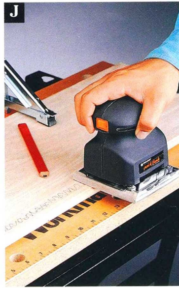
J Draw pencil marks on veneered surfaces to prevent oversanding.
