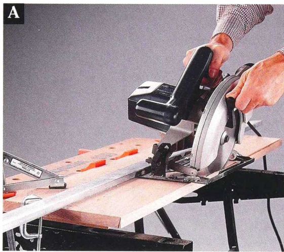
The foot of the circular saw rides along the straightedge to make straight, smooth cuts.
