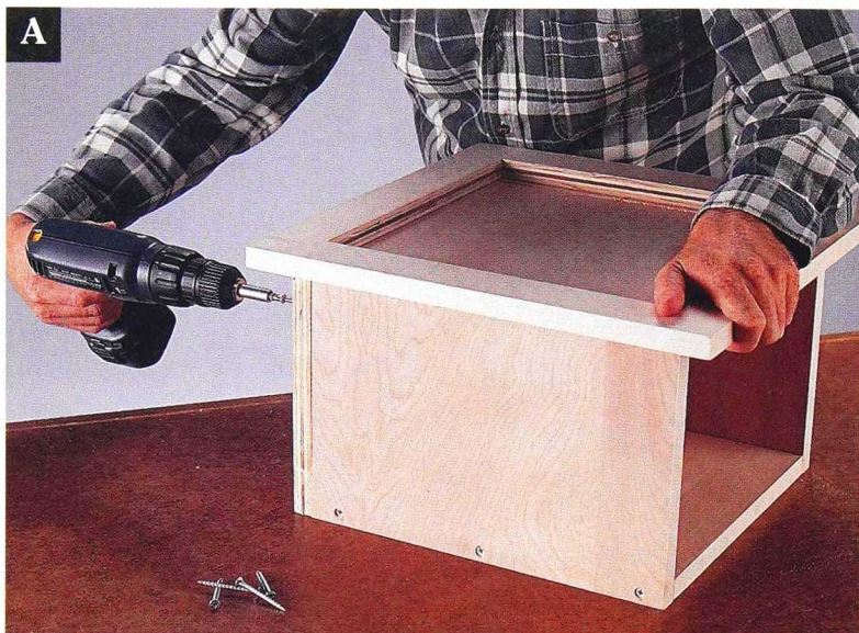
Fasten the back panel to the side and end panels with glue and wood screws.
