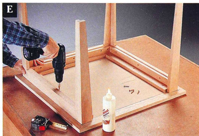
Attach the top with glue and screws driven through the stretchers and into the top.
