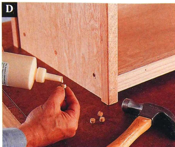
Fill all visible screw holes with oak plugs.
