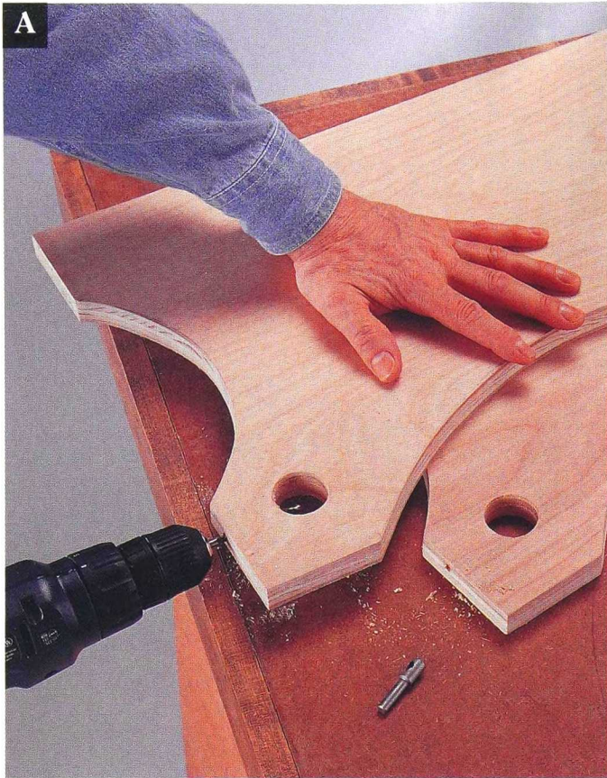
Drill pilot holes for the anchor screws through the bottom edges and into the dowel holes.
