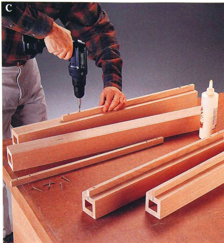
Attach the end half slats to the legs with glue and wood screws.
