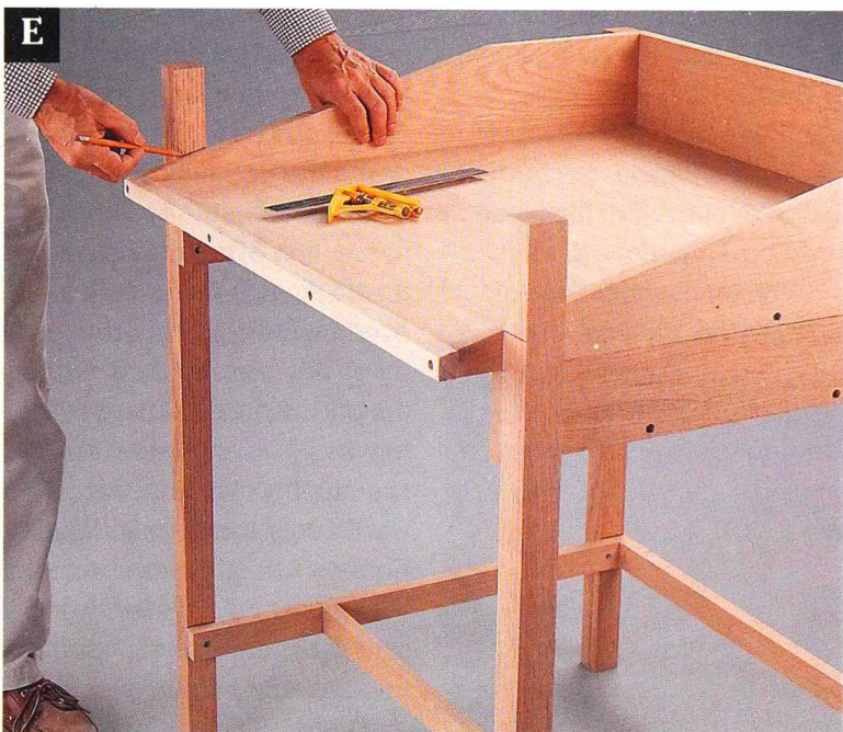
E Trace the angles of the desk sides onto the front legs. Then, trim the legs to follow the sides.
