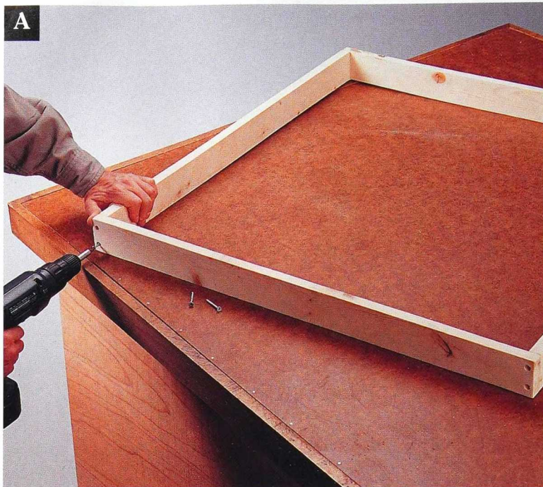
Fasten the end aprons between the side aprons with glue and wood screws to construct the apron frame.
