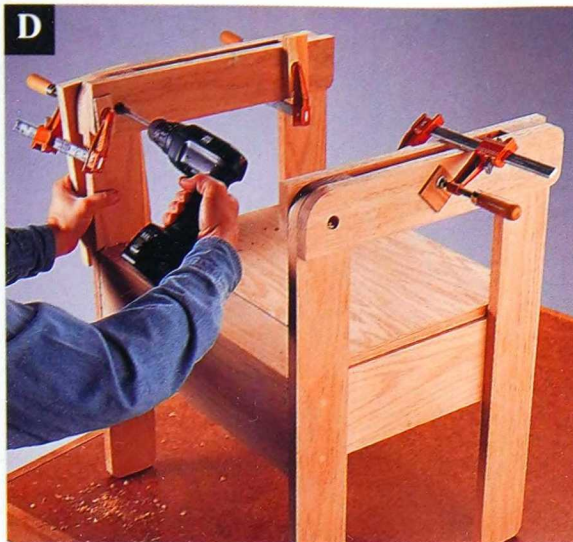
With a backer board clamped to the outside of the legs, drill guide holes for the dowel pivots.
