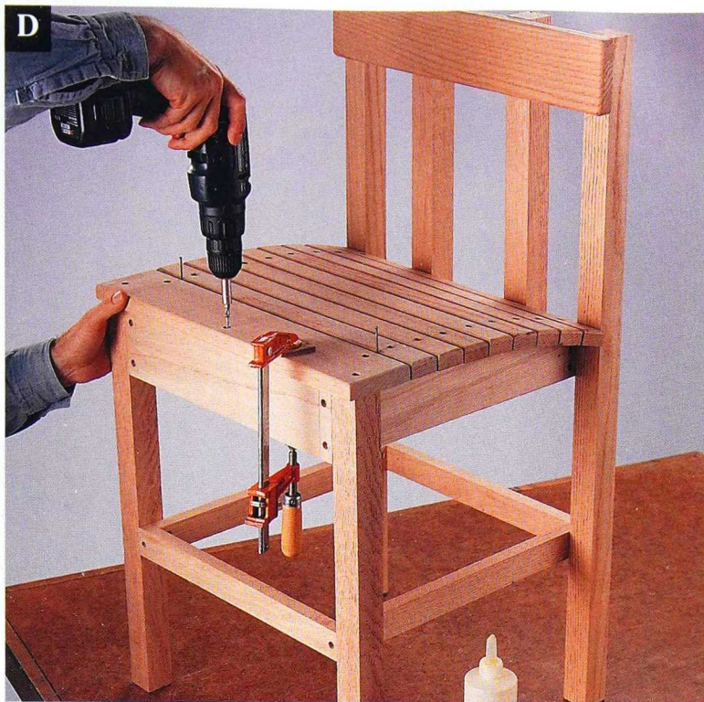
Using 10d nails as spacers, fasten the seat slats to the top of the seat frame, finishing with the front slat.
