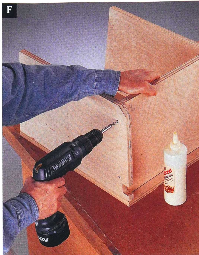
Position the bin bottom flush with the dowel notch, and attach it with glue and screws.
