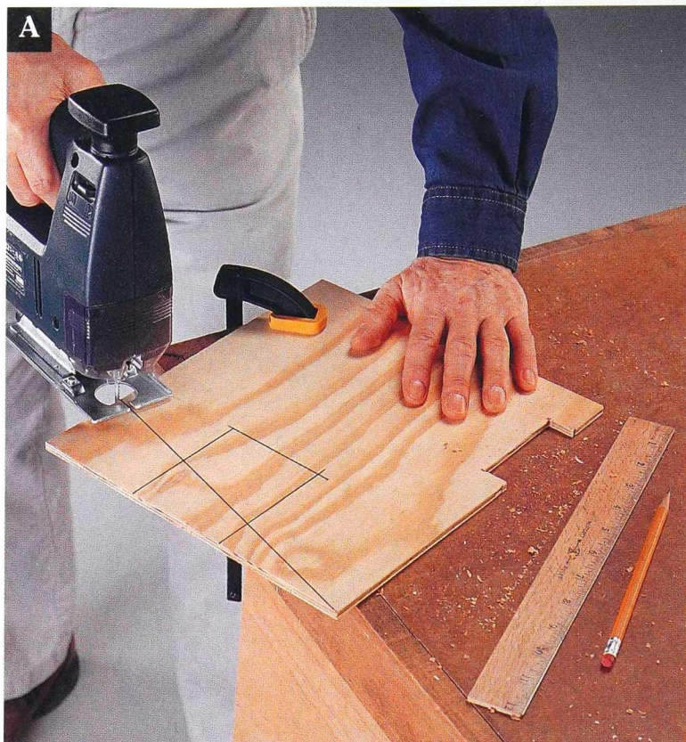
Use a piece of \frac{1}{4} " scrap plywood and your jig saw to create the mortising jig.
