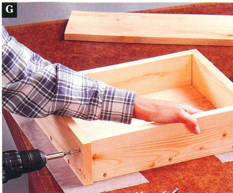
Fasten the drawer sides to the drawer ends and drawer bottom with glue and screws.
