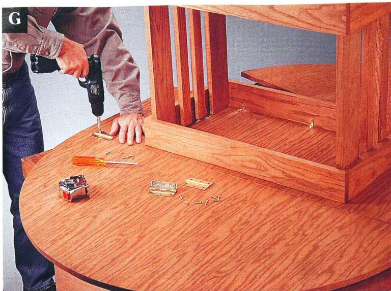
Attach the leaves to the table panel with brass hinges.
