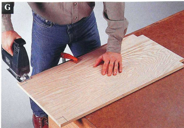
G Cut notches at each corner of the middle shelf so it will fit between the credenza legs.
