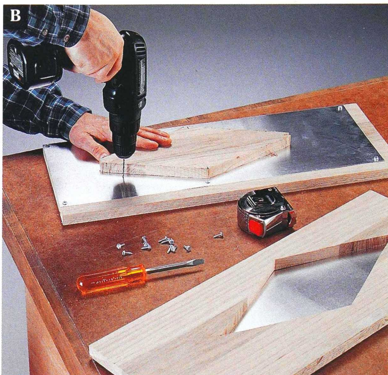
B Use the diamond cutout as a guide when attaching the tin panel around the cutout.
