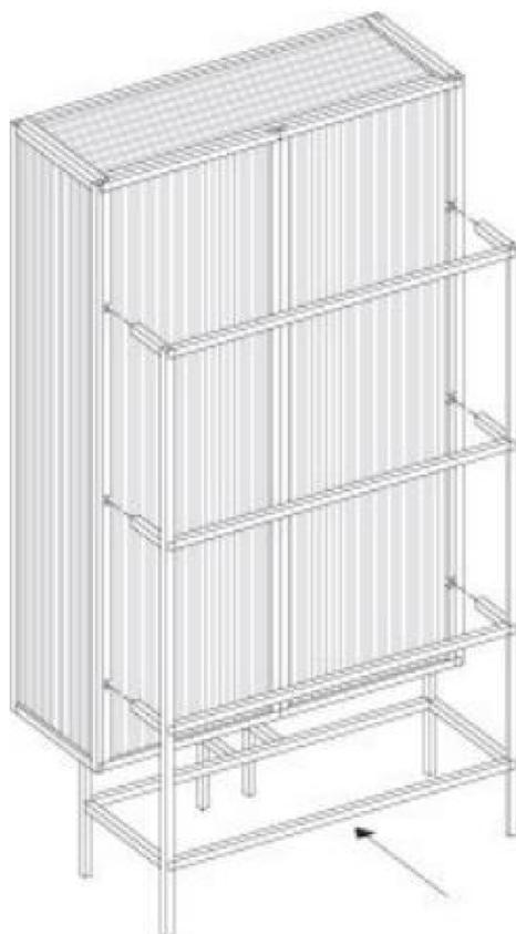
\_Put the cabinet on a block of wood to support it while you slide the frame in place.
