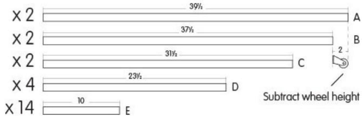
Use a saw to cut the 1 x 1in wooden battens into the following lengths:
